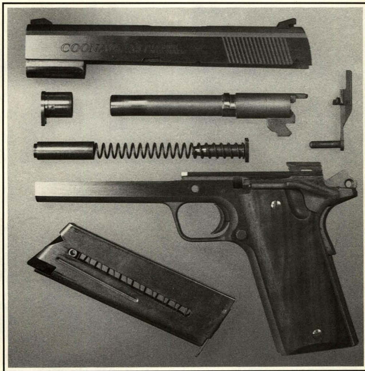
Coonan Model B field-stripped
