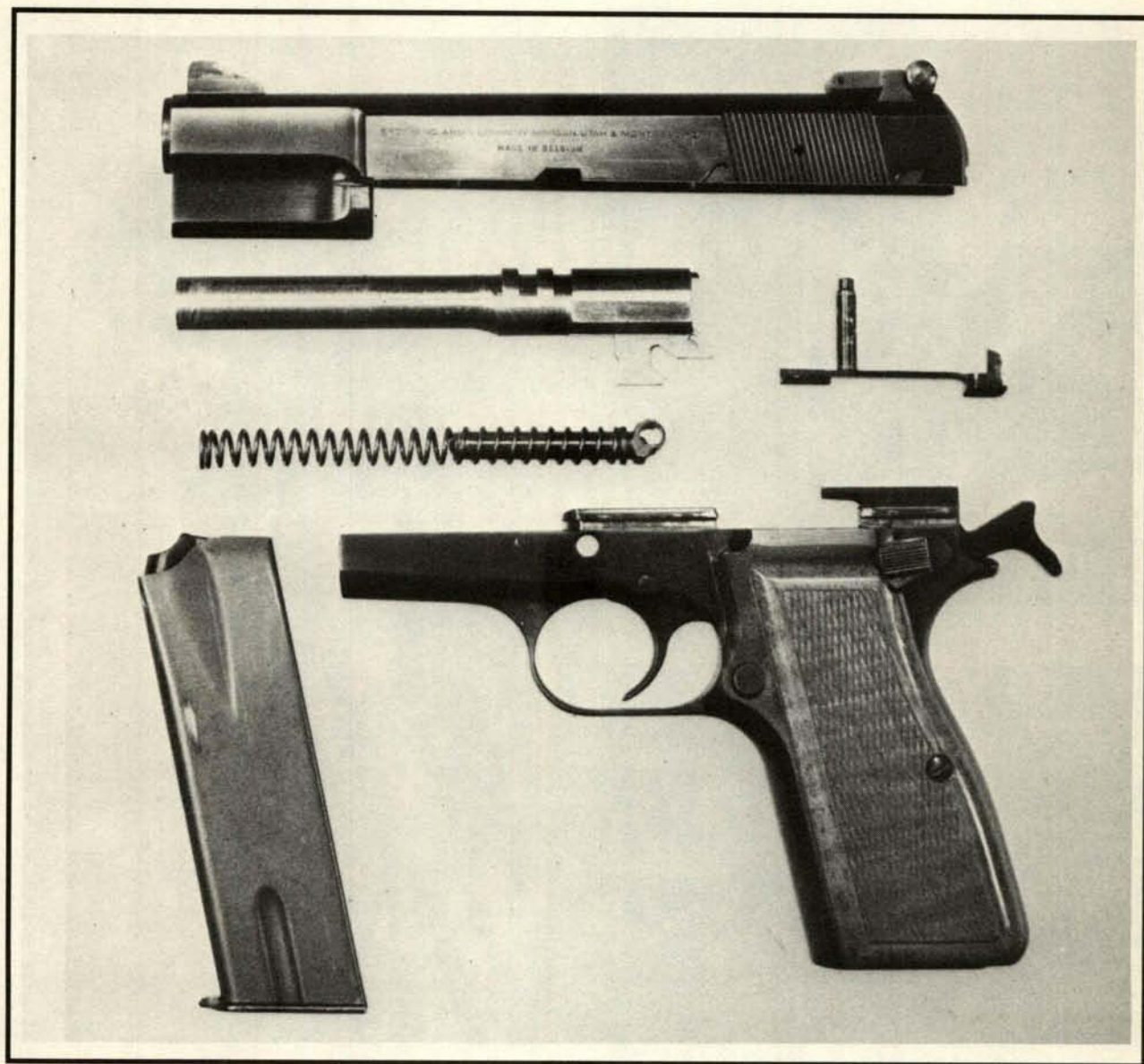
Browning Hi-power field-stripped
