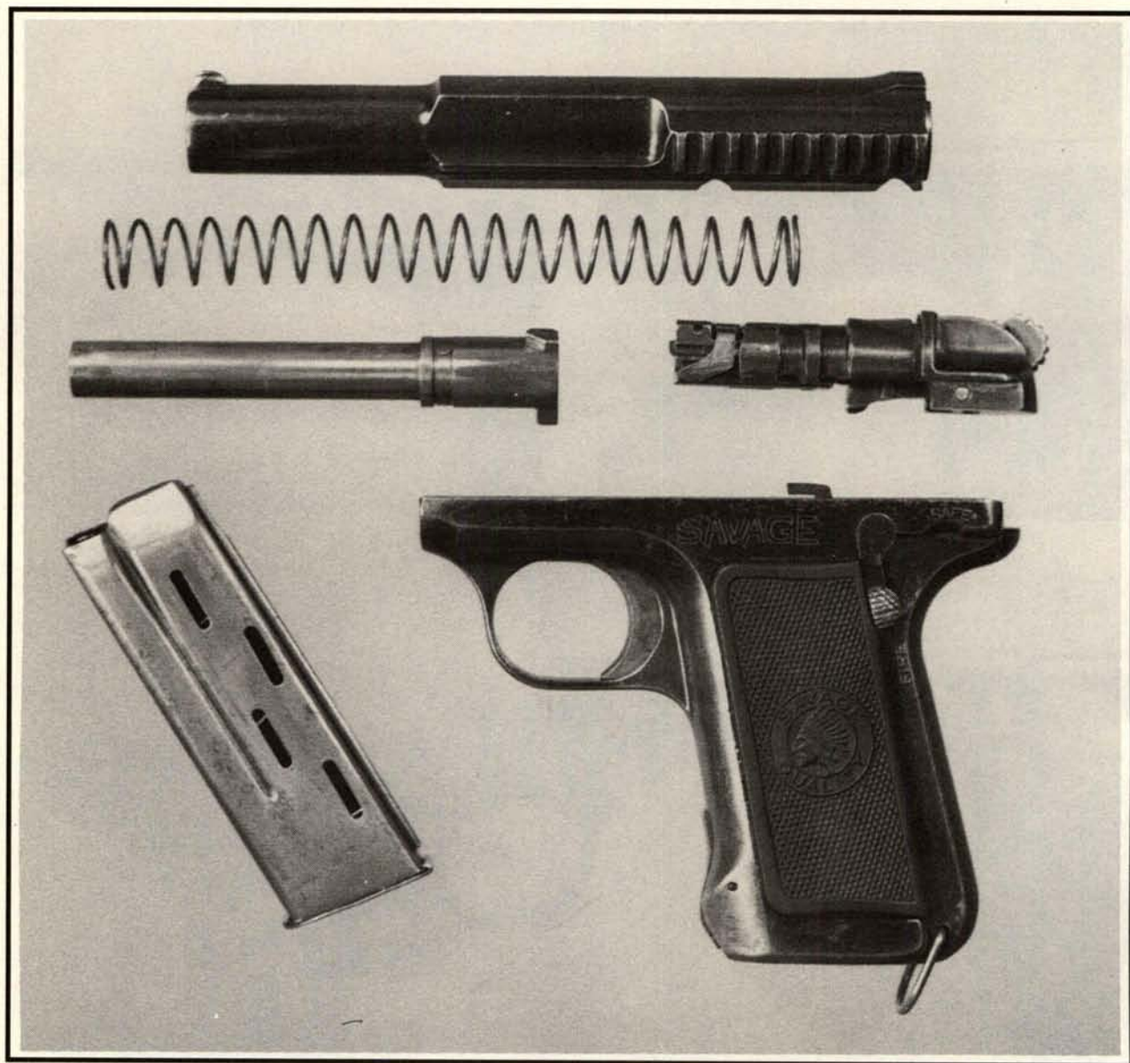
Savage Model 1908 field-stripped
