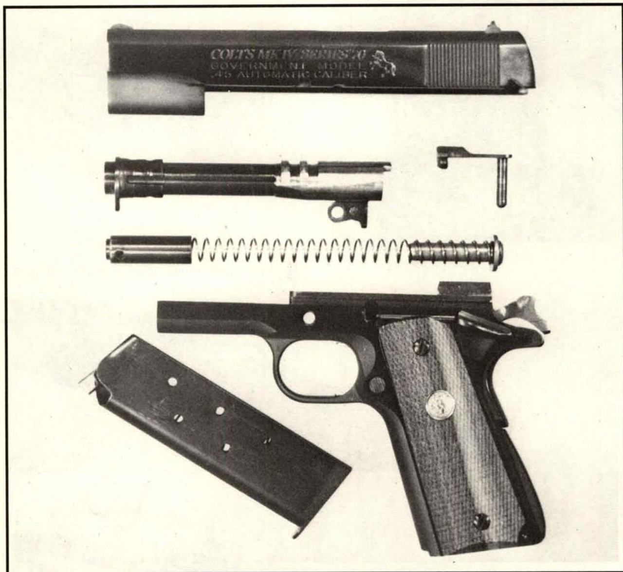
Colt Mk IV/Series 70 field-stripped
