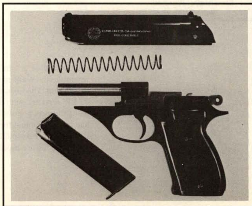
Astra Constable field-stripped
