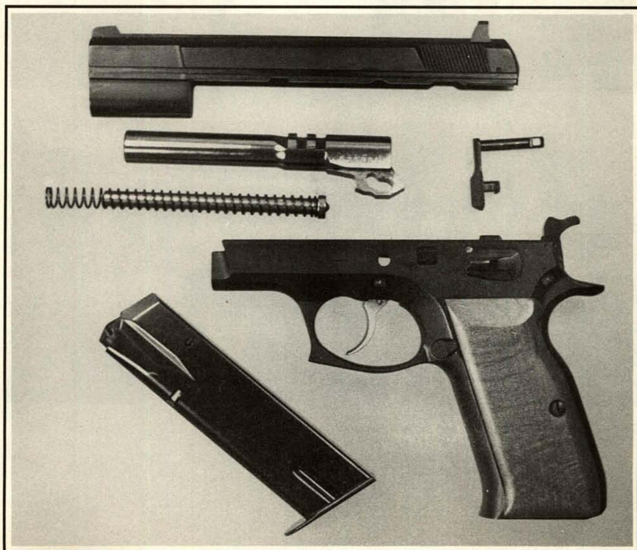
TZ75 Series 88 field-stripped
