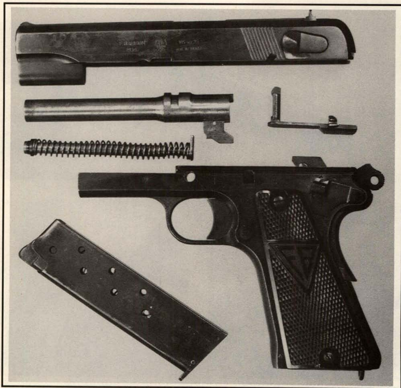
Radom P-35 field-stripped
