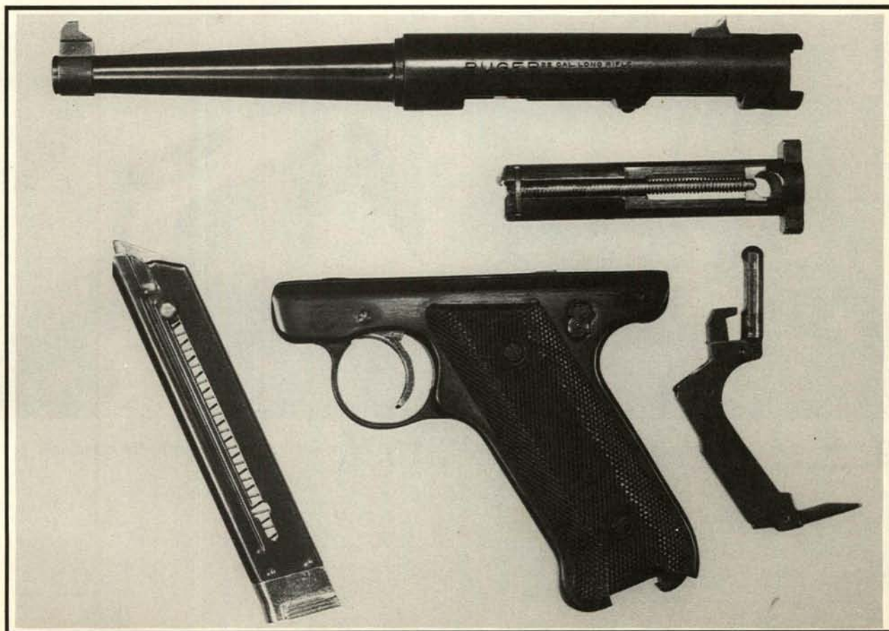
Ruger Standard Auto field-stripped
