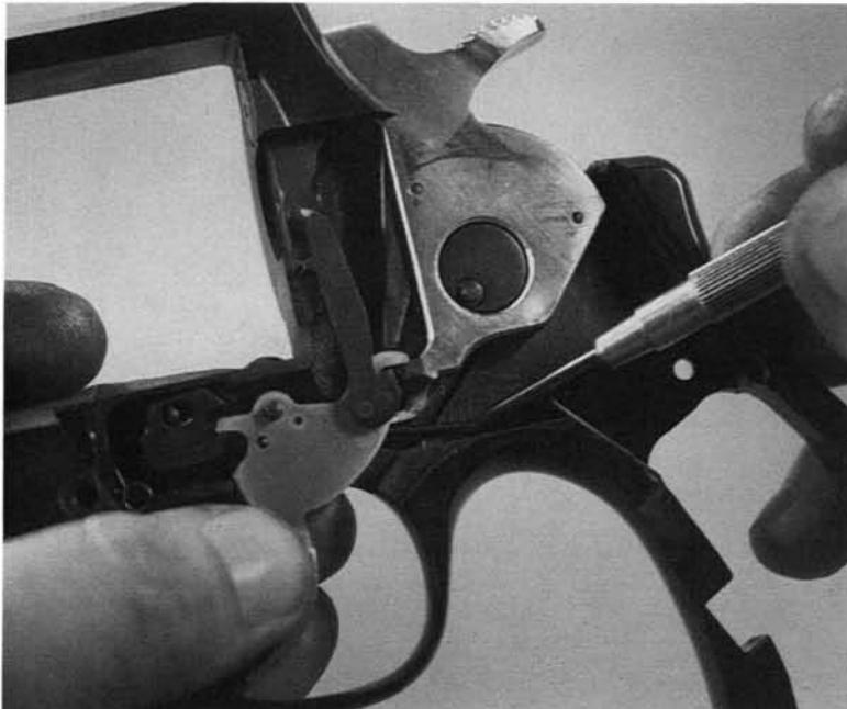
**3.** Note that the hammer spring base has four seat levels, and can be inverted, to adjust the spring tension. Whatever level is chosen, the spring unit must be located near the frontstrap of the grip frame.
