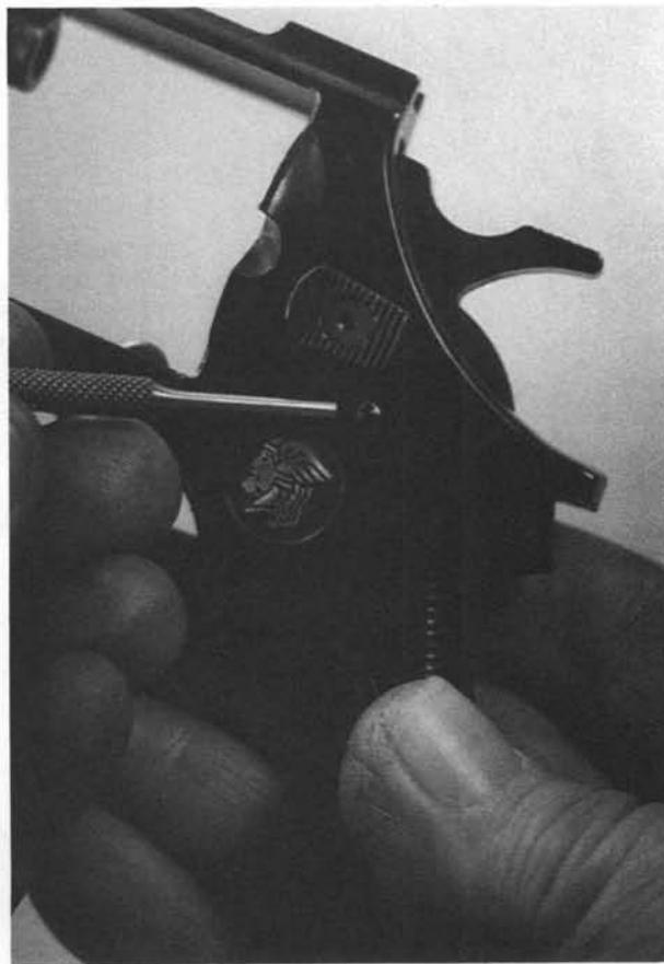
**12.** Drift out the cross-pin at the center of the frame.
