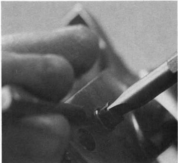
**2.** When replacing the safety, be sure the two depressions for the detent ball are on the left side, and are turned toward the ball. This can be gauged by keeping the small recess shown in alignment with the retaining screw.
