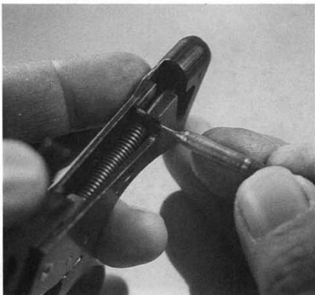
**21.** Ease the hammer down, and remove the hammer spring assembly upward and toward the rear. If it is necessary to separate the spring unit parts, wrap the unit in a heavy shop cloth and pull out the drift or paper clip.
