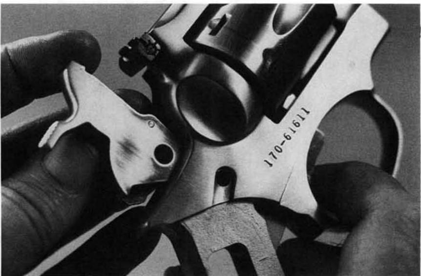
**3.** Remember that the trigger must be pulled before the hammer can be reinserted.
