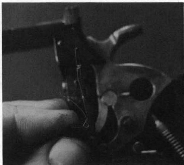
**11.** Remove the transfer bar and its captive leaf spring from its stud on the trigger.
