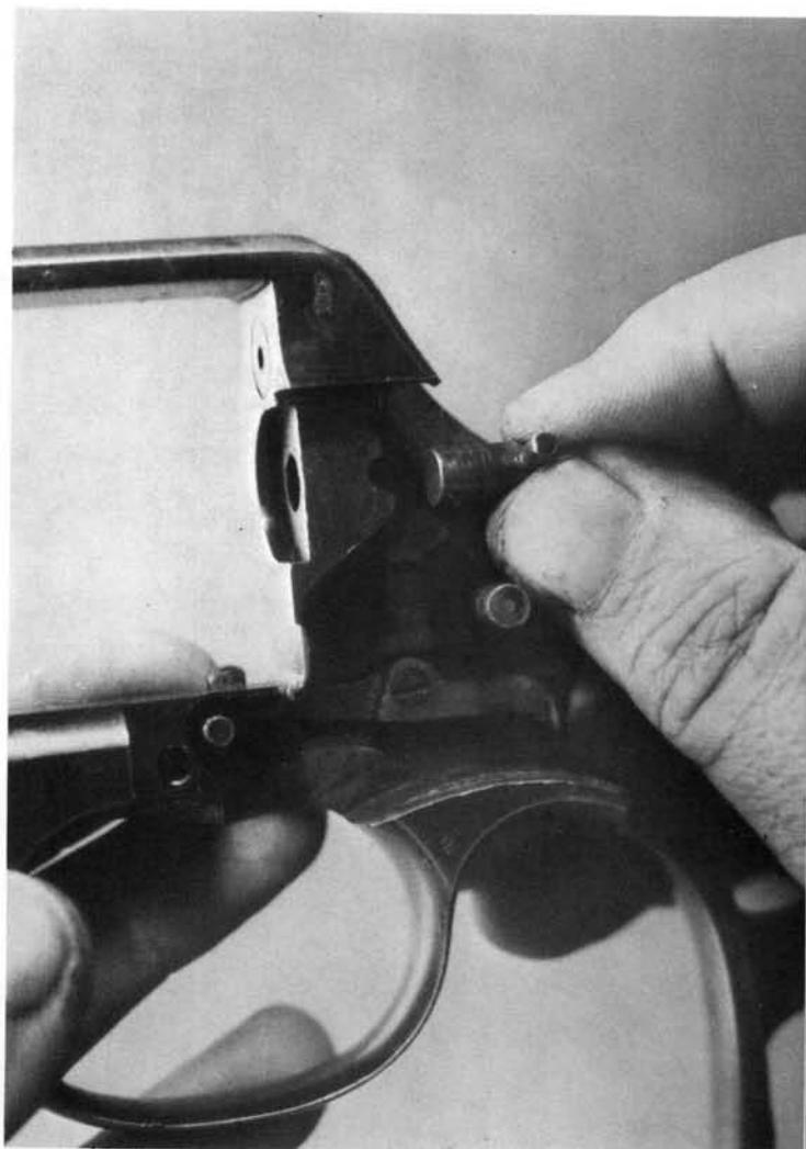
**17.** Remove the cylinder latch bolt toward the rear.
