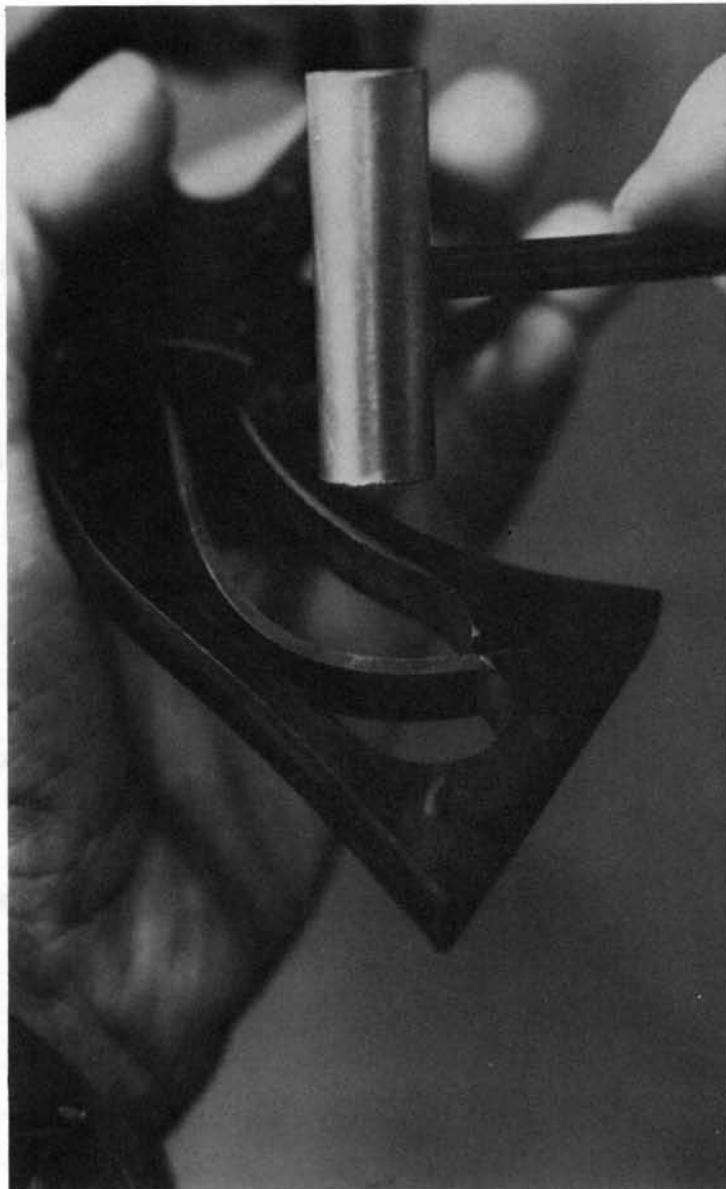
8. Remove the screw on the underside of the frame, just forward of the trigger guard. Take out the two screws at the rear of the frame, and remove the trigger guard/grip frame unit downward.
