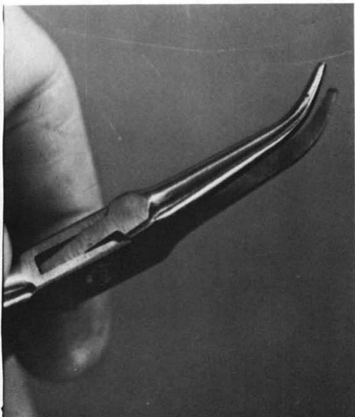
**3.** You should have at least one good pair of bent sharp-nosed pliers. These, from Brownells, have a box joint and smooth inner faces to help prevent marring.
