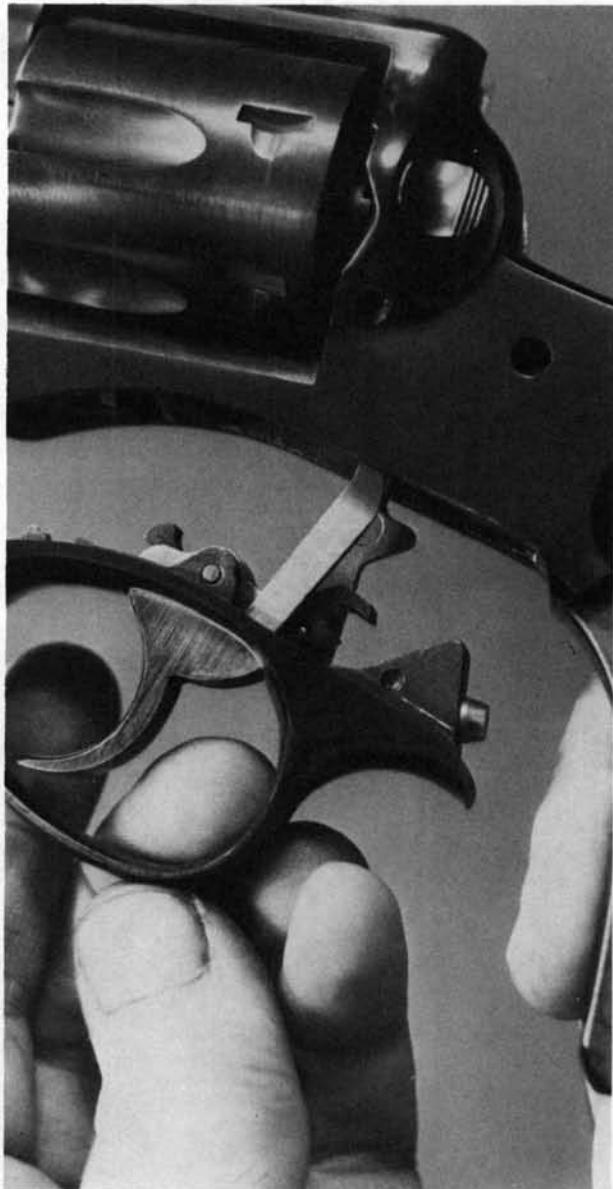
**10.** Pull the trigger slightly toward the rear and remove the transfer bar toward the left.
