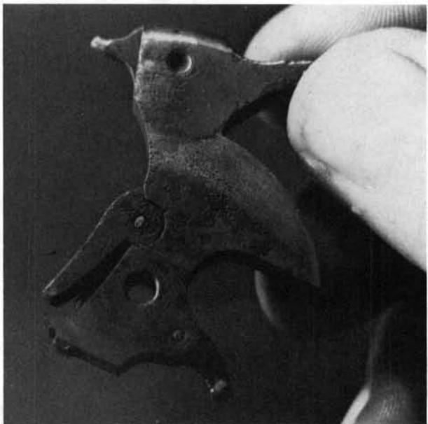
**14.** Drifting out the small pin at the front of the hammer will release the double-action lever and its spring for removal. The small cross-pin at the lower rear of the hammer retains the stirrup.
