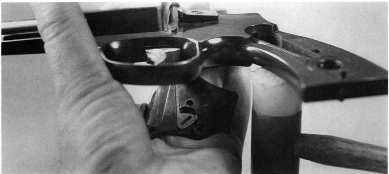
9. With the gun held as shown, tap the grip frame with a non-marring mallet until the sideplate drops into the hand.
