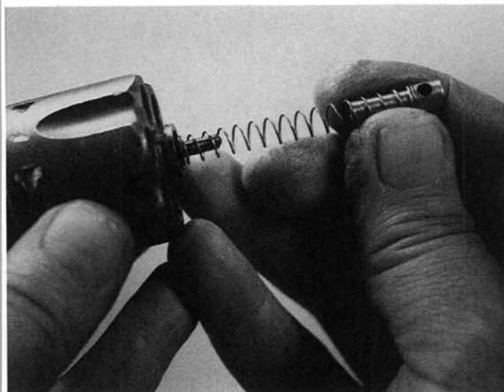
**6.** Remove the ejector/ratchet unit toward the rear.
