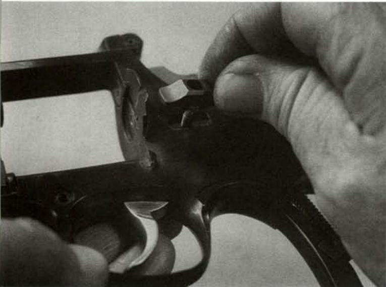
**17.** Use a tool to gently pry the lower edge of the sideplate outward, at the rear and beside the trigger. Move the sideplate slightly forward and downward, and take it off toward the left.
