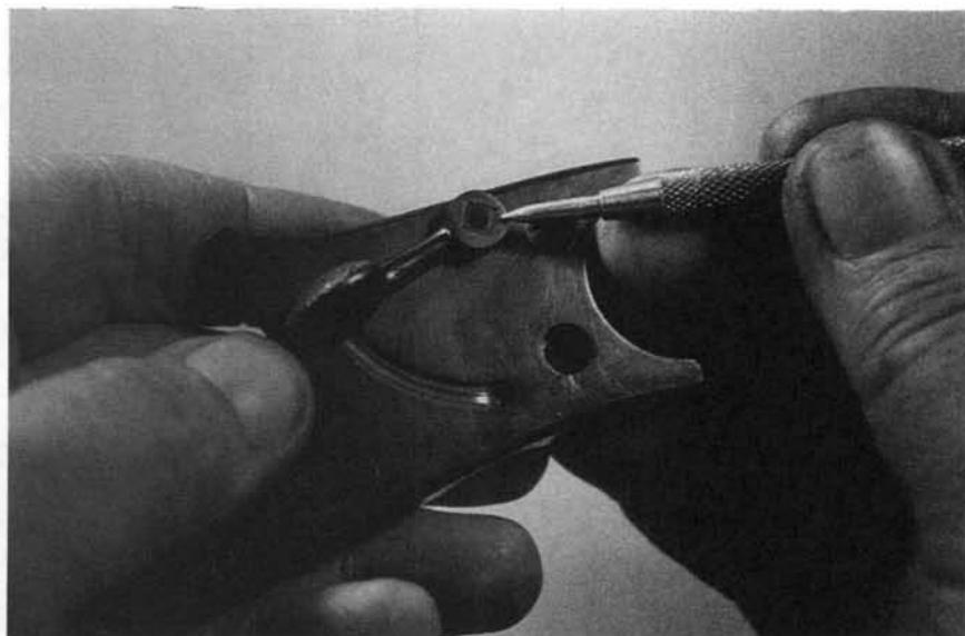
**11.** By inserting a small drift into the screw hole, and supporting the sideplate on the back, the safety shaft can be driven out of the lever. In normal takedown, it is best left in place. If this unit is taken apart, its orientation must be carefully noted for proper replacement.
