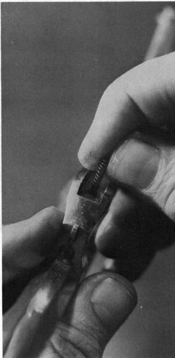
**8.** A cross-pin at the middle rear of the grip frame holds the hammer spring. After the pin is removed, the spring can be compressed with pliers and moved downward, then out toward the side.
