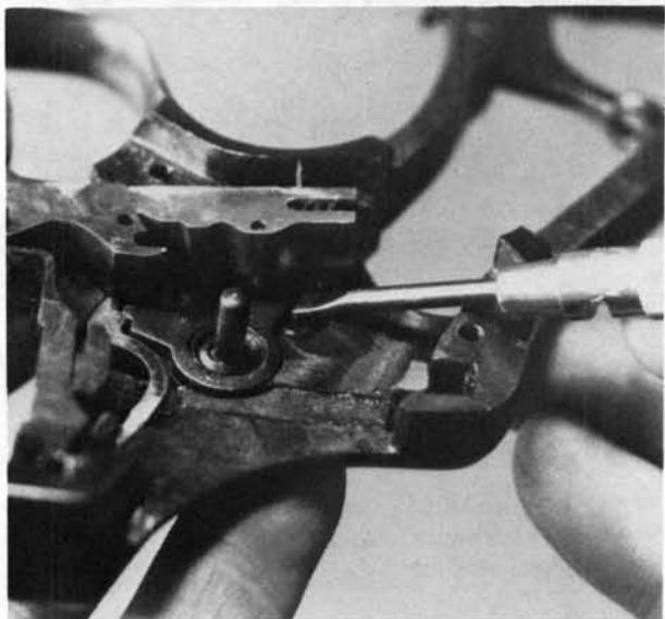
**1.** When replacing the rebound slide in the frame, be sure its inside stud engages its recess in the lower arm of the hammer block lever.
