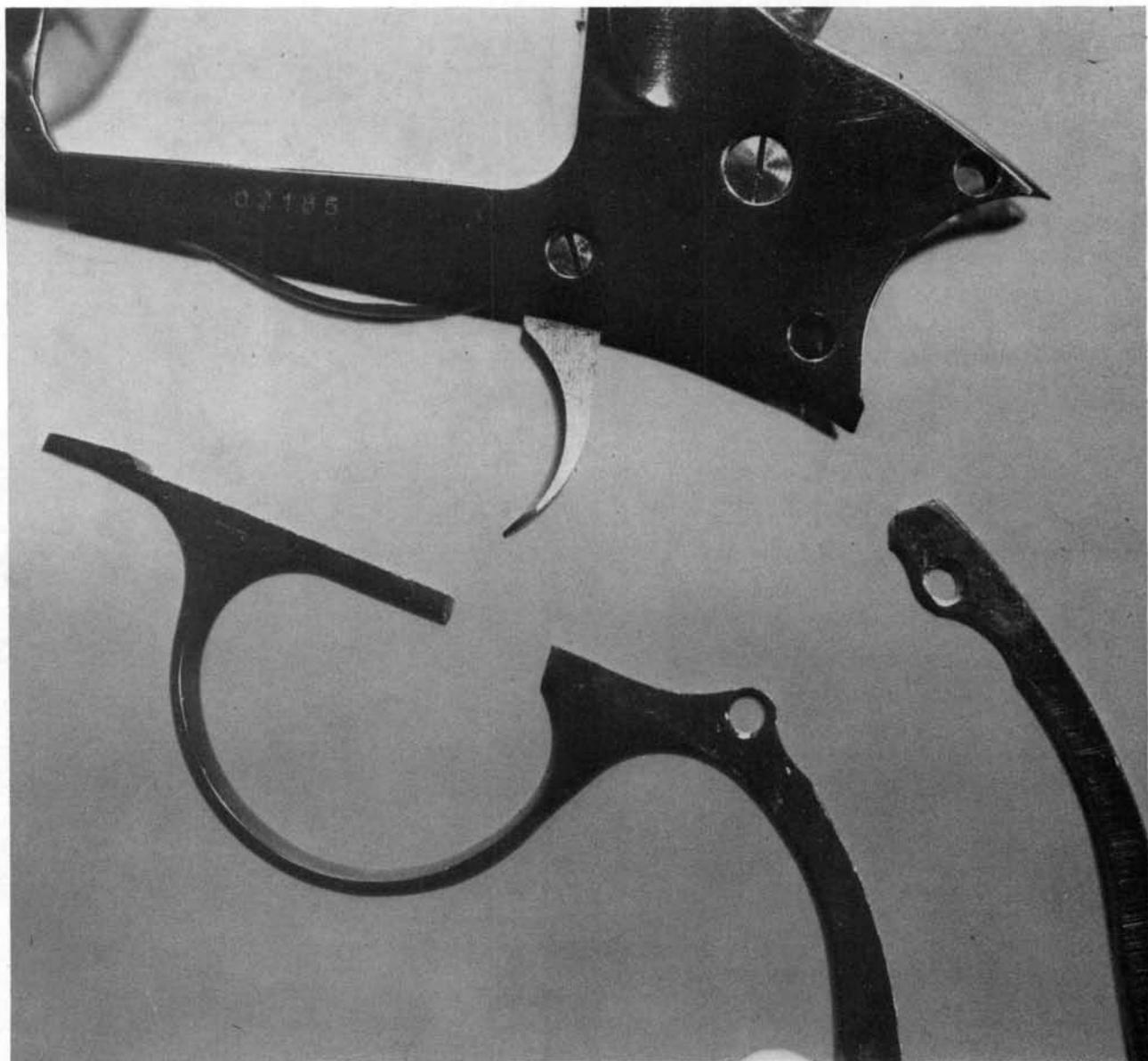
**9.** The combination spring which powers the trigger and cylinder stop will be released by removal of the guard screw. Remove the spring from the frame recess.
