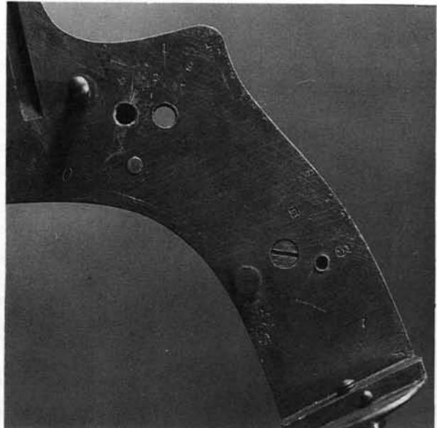
**18.** The screw in the center of the grip frame holds the right grip. Drifting out the cross-pin at the lower end of the grip frame will allow the lanyard ring to be unscrewed and removed.
