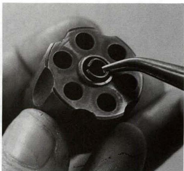
**6.** Before the crane is put back into the cylinder, remember to drop the spring ring back into the arbor tunnel, and be sure it is lying flat.
