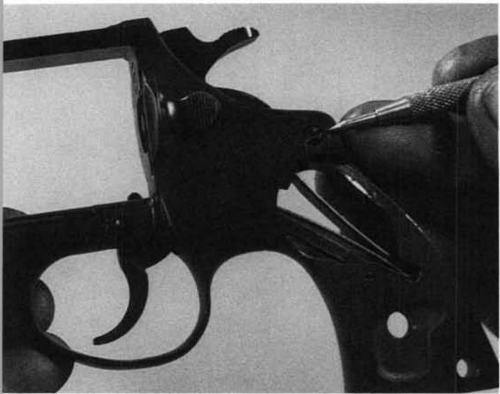
**6.** Remove the two sideplate screws on the left side.
