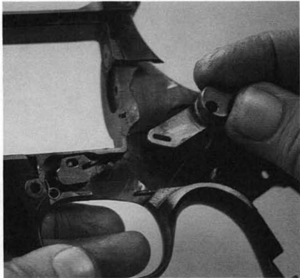
**27.** Use slim pliers to grip the cylinder stop spring as shown, and remove it toward the left.
