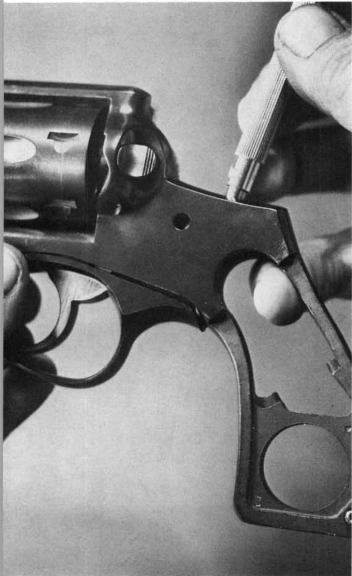
**9.** When the plunger has cleared the frame at the rear, move the trigger guard unit down and remove it from the frame.
