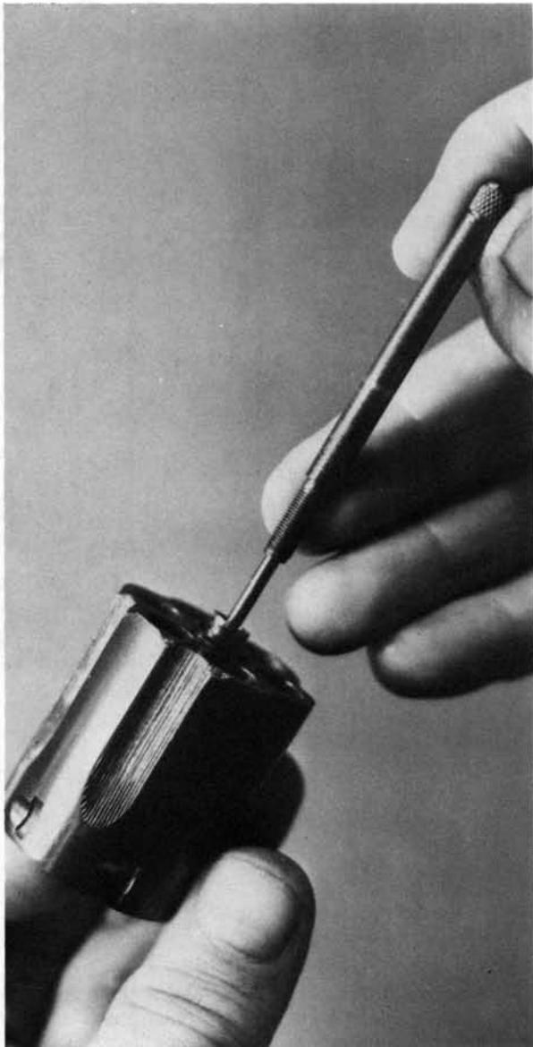
**4.** Remove the cylinder lock pin and its spring from the front of the cylinder.
