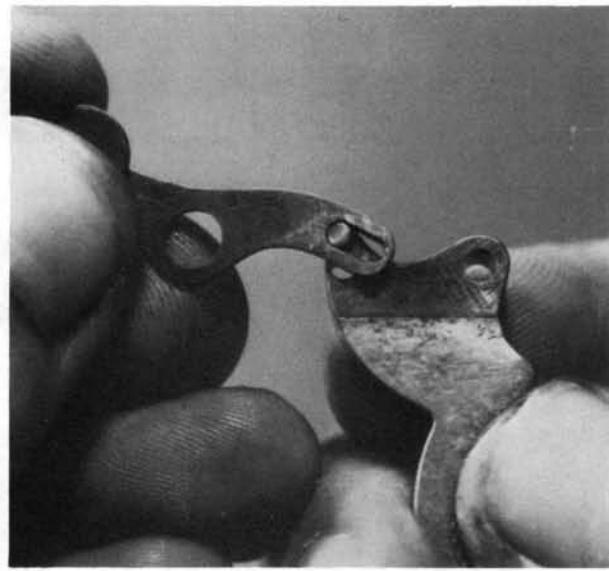
**19.** The hammer block lever is attached to the trigger by a stud on the right side, its head keyed into a slot in the lever. Move the stud back to the enlarged opening in the slot, and separate the lever from the trigger.
