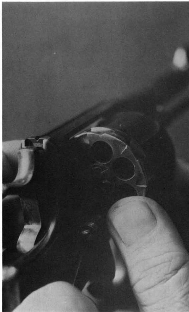
**5.** Turn the cylinder bushing until the small lug on the bushing aligns with its exit track in the front of the cylinder, and remove the bushing and spring toward the front.
