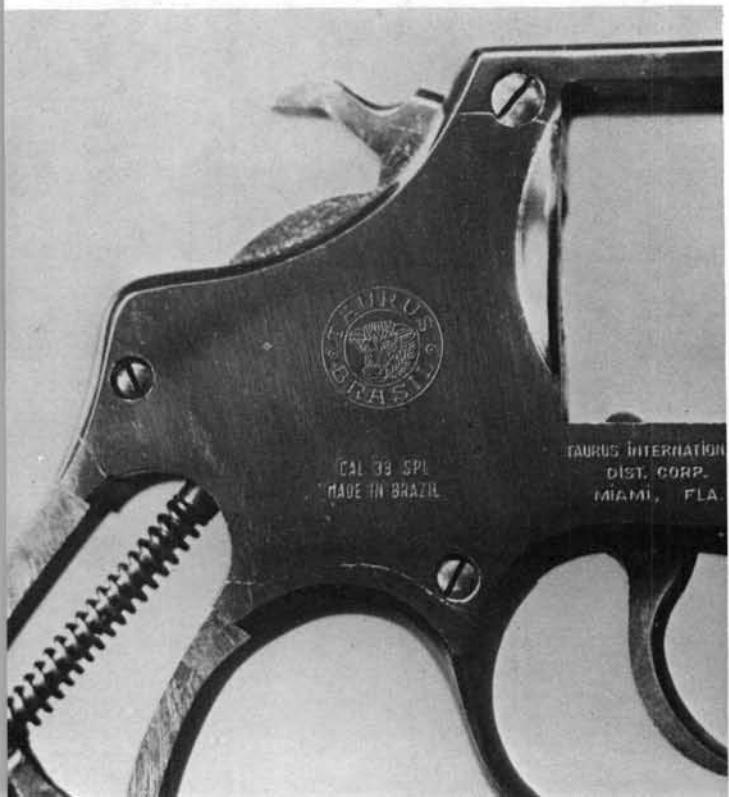
**7.** Remove the three remaining sideplate screws from the right side of the frame. Use a wider screwdriver on the upper plate screw.
