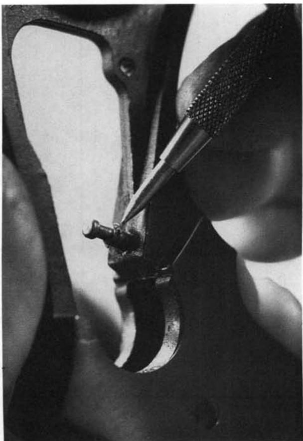
**28.** The trigger guard latch is retained in the frame by a C-clip at the rear. If removal is necessary, taking off the C-clip will allow the latch and its spring to be taken out toward the front.
