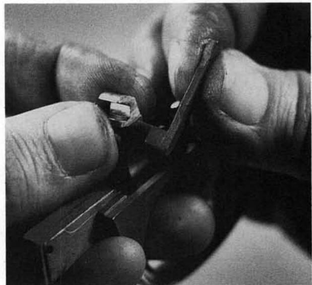
**17.** Remove the cylinder hand spring and plunger toward the rear.
