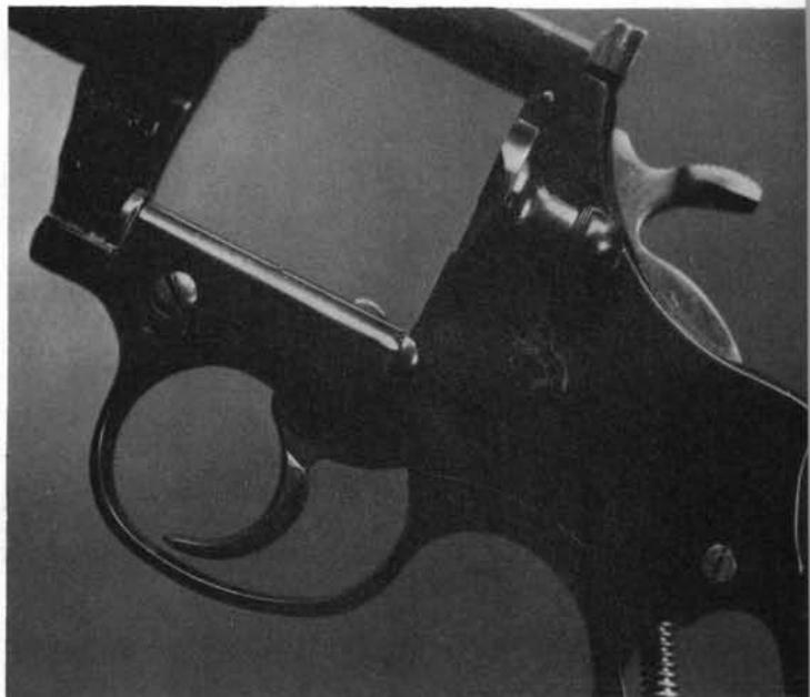
7. After the two screws are removed, hold the gun as shown and tap the grip frame with a nylon hammer or some other non-marring tool; the sideplate will fall off into the palm of the hand. Do not pry the sideplate off as this will burr the edges.
