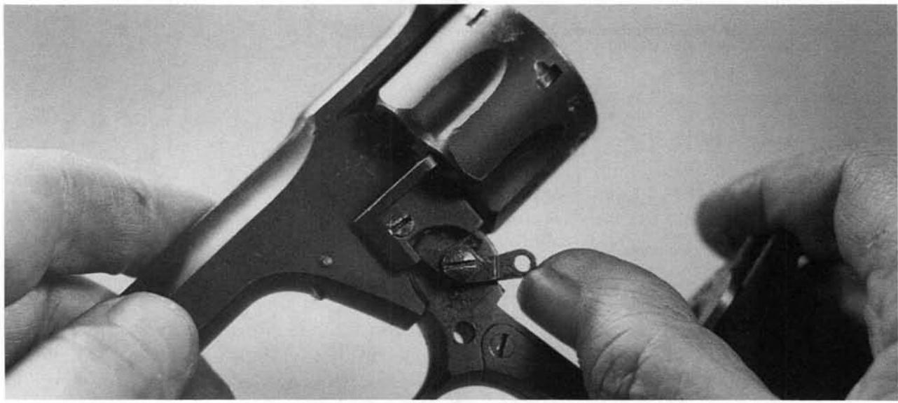
2. Rotate the lower end of the cylinder retainer lever upward until it tips the retainer out of engagement with the cylinder collar.
