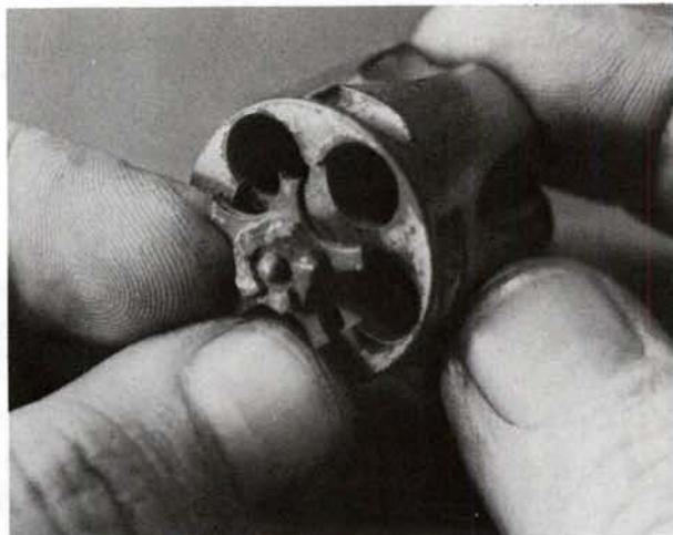
When replacing the guard in the frame, use a slave pin to hold the sear in place until insertion of the cross-pin.
