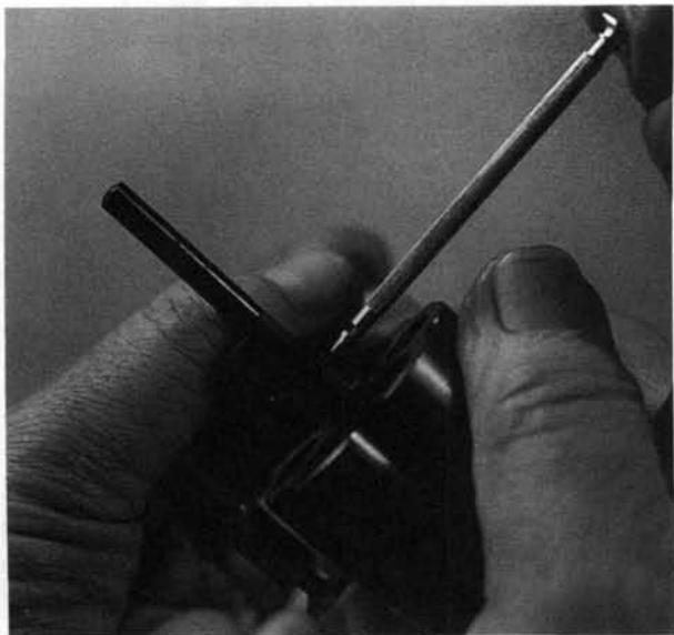
**21.** Insert a very slim tool in the hole in the top of the crane to depress the lock plunger, and push out the front latch pivot toward the left.
