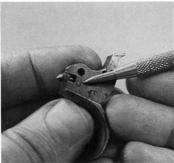
**26.** Remove the hammer block bar from its recess in the frame.
