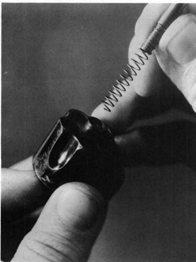
**4.** Remove the ejector/ratchet toward the rear. By using a twin-pointed tool, it is possible to unscrew the center stud and separate the ratchet from the ejector shaft, but this is not advisable in normal takedown.
