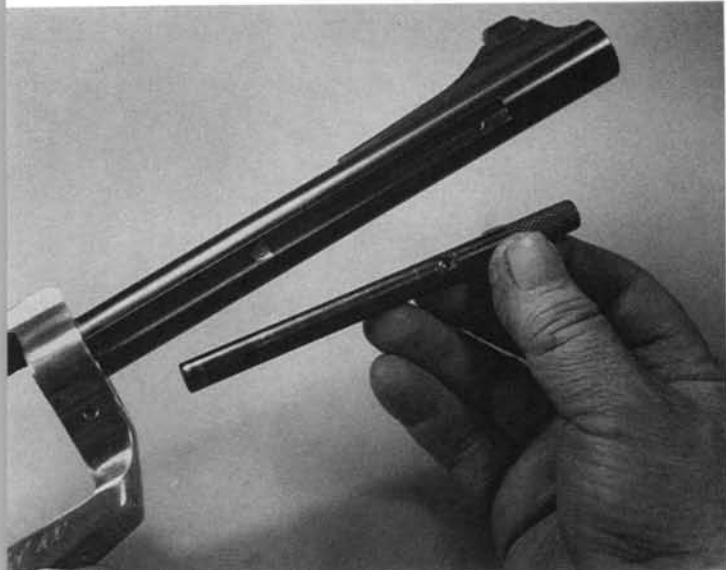
**26.** The front sight is retained by two screws. One is visible, as shown. The other is covered by the sight blade, and the blade must be drifted out of its dovetail for access to the screw. If the sight is to be taken off, drift out the blade before removal of the rear screw.
