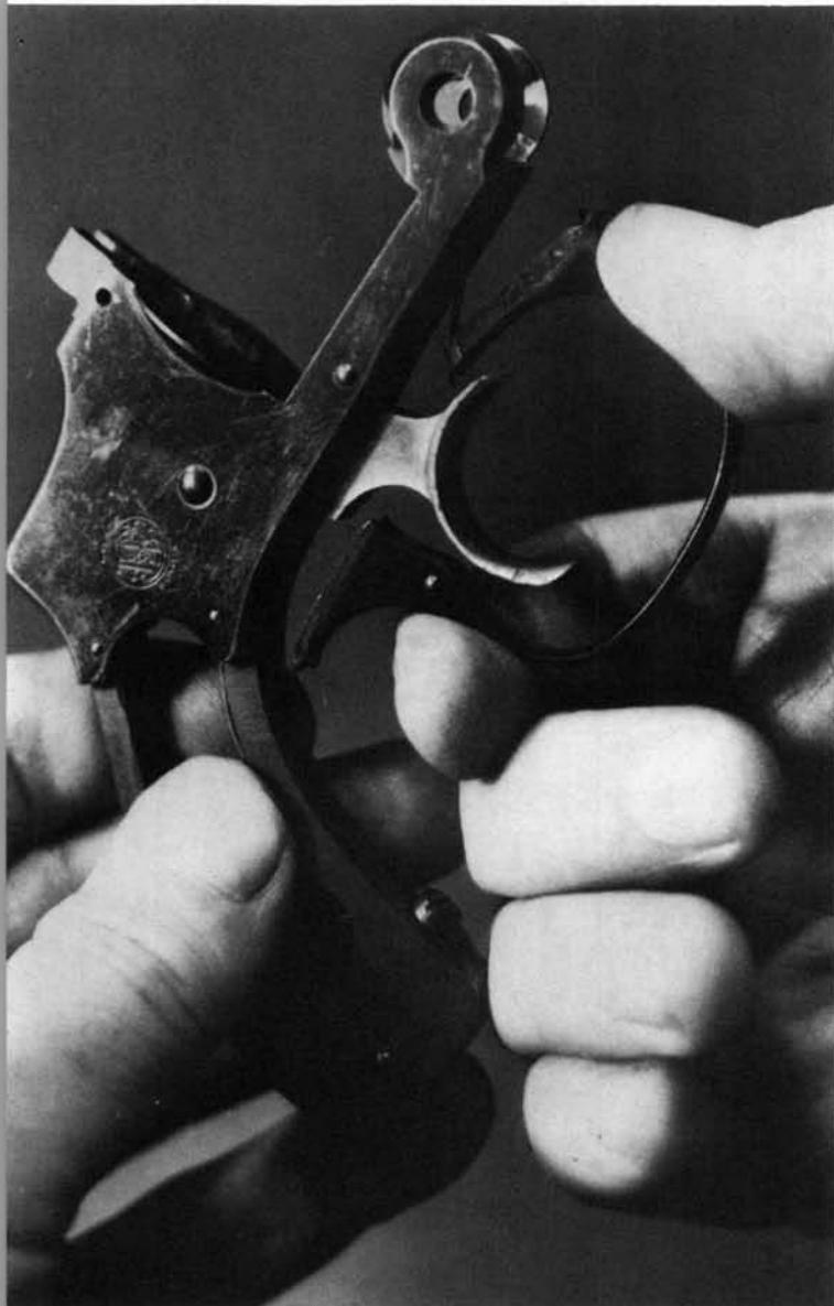
**19.** Remove the trigger spring from the lower front of the frame.
