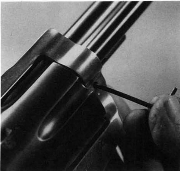
**2.** Set the hammer on the loading step ("half-cock") and move the base pin forward. It will be stopped by the ejector handle.
