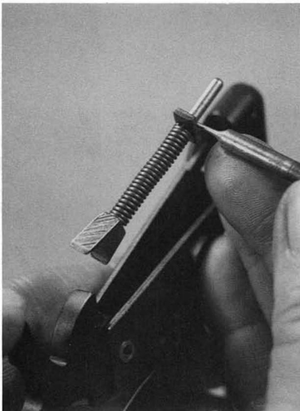
**22.** Push out the hammer pivot bushing toward either side.
