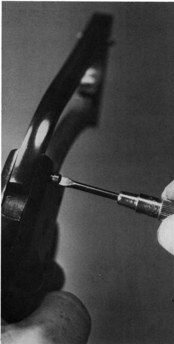
**2.** Before installing the front guard screw, use a tapered tool to center the hole in the combination trigger and cylinder stop spring.
