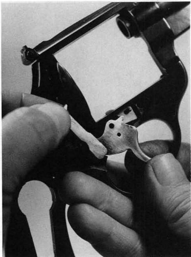
**17.** Remove the rebound slide strut from the left side of the trigger. Control the cylinder hand plunger and spring.
