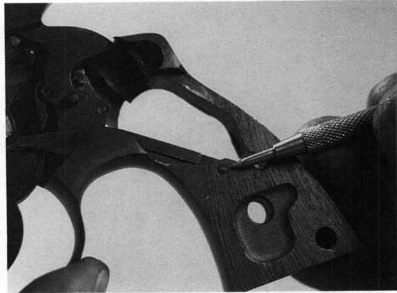
**12.** Move the rebound lever upward, out of its recess, and take it out toward the left.
