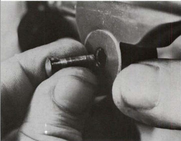
**20.** Remove the ejector cam from the frame. The ejector cam trip can now be slid out of its recess in the cam, along with its small blade spring. Take care that the spring isn't lost, and note that its concave side goes toward the cam trip.
