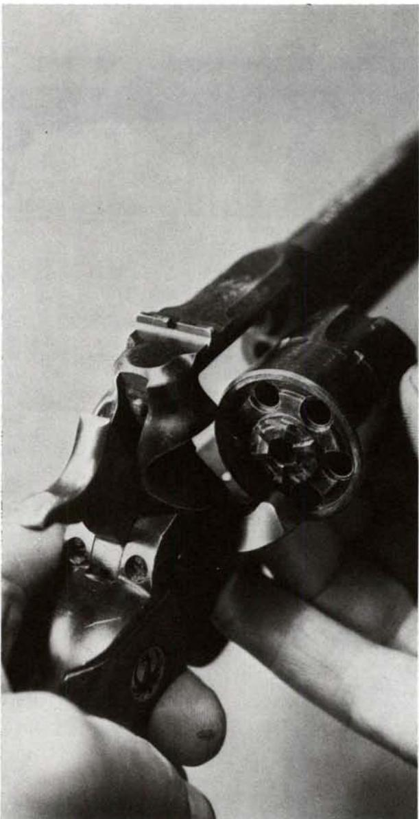
**3.** After removing the grips, cock the hammer, and insert an opened paper clip or a small nail through the transverse hole in the lower end of the hammer strut.
