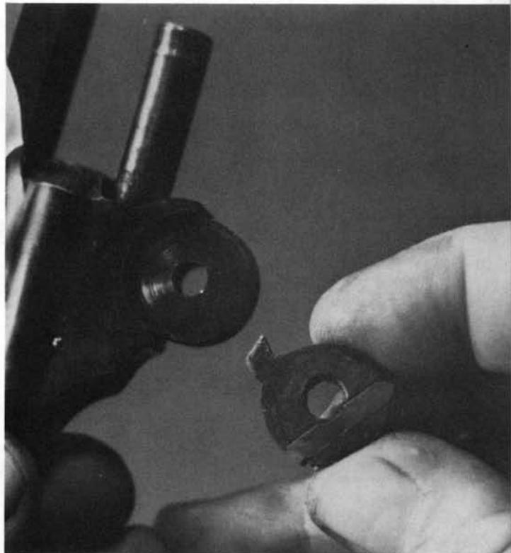
**6.** Remove the cross-screw and the limit pin beside the screw at the center of the barrel extension, and take out the barrel latch, plunger, and spring toward the rear. Taking out the small set screws in the latch knobs will allow removal of the sight leaf.
