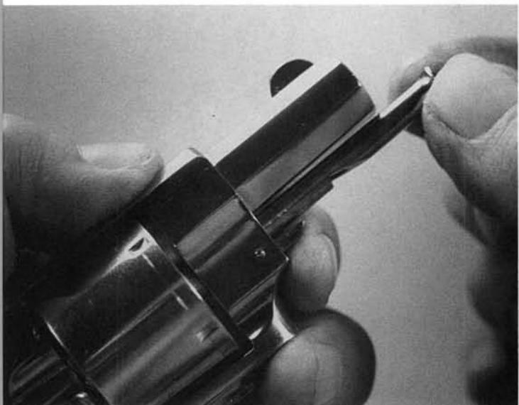
3. Remove the cylinder from the frame.
