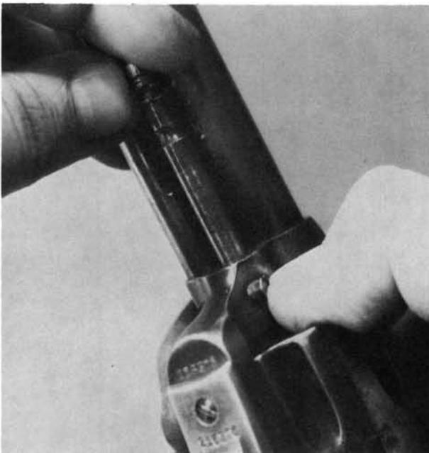
2. Open the loading gate and remove the cylinder toward the right.
