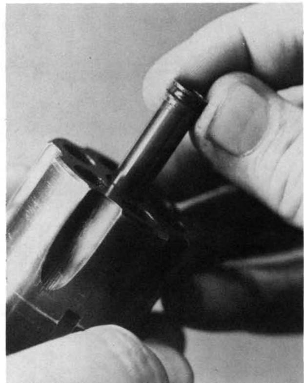
**4.** Remove the bushing from the front of the cylinder.
