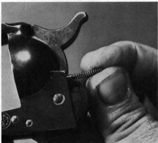
**7.** Remove the cylinder hand spring and plunger from the hole in the rear upper left of the main frame.
