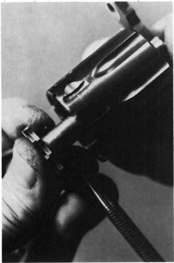
**2.** With the punch still in place, insert the ejector/ratchet into the rear of the cylinder, and insert the ejector rod and its spring into the front. Turn the rod until the small transverse hole at its rear tip is aligned with the tip of the punch, and move the punch inward to hold the assembly in place.
