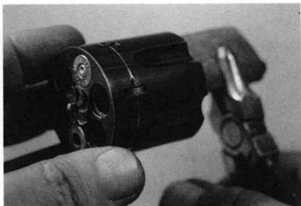
**5.** When installing the ejector rod in the cylinder, remember that it turns counterclockwise (front view) to tighten. Do not over-tighten, or the fine threads may be stripped. Place empty cartridge cases in the chambers to protect the spline.
