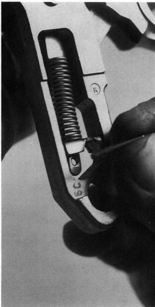
**7.** Pull the trigger and ease the hammer down. Move the spring assembly upward, tip it outward at the bottom, and remove it. If the spring assembly is to be taken apart, use caution and control the powerful compressed spring.
