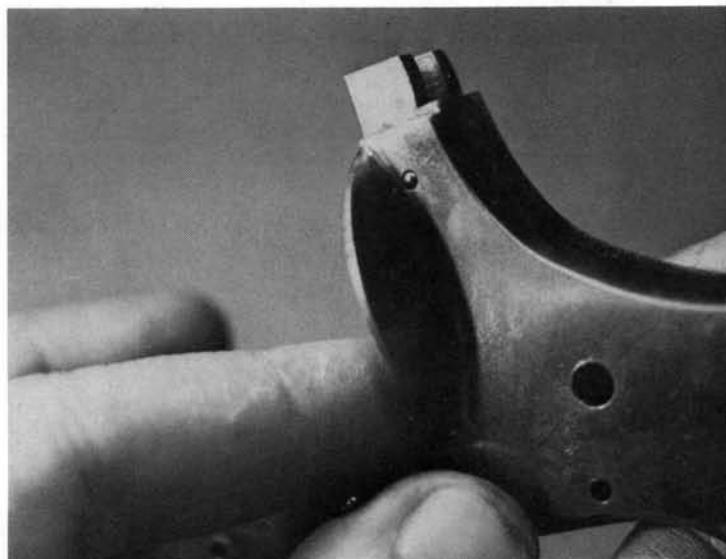
**17.** Drift out the cross-pin at the top of the frame, just below the cylinder latch posts.
