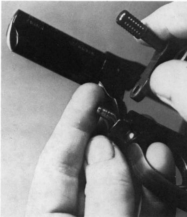
3. Remove the crane pivot and cylinder stop spring from the front of the frame.
