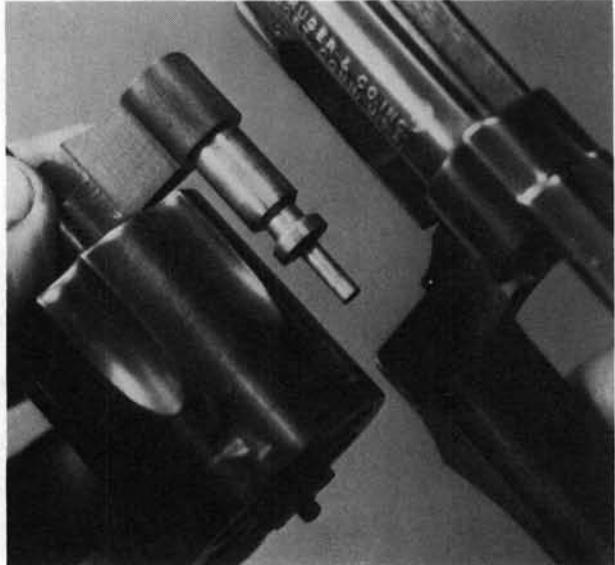
**16.** Remove the cylinder stop plunger and spring from the rear of the crane pivot.
