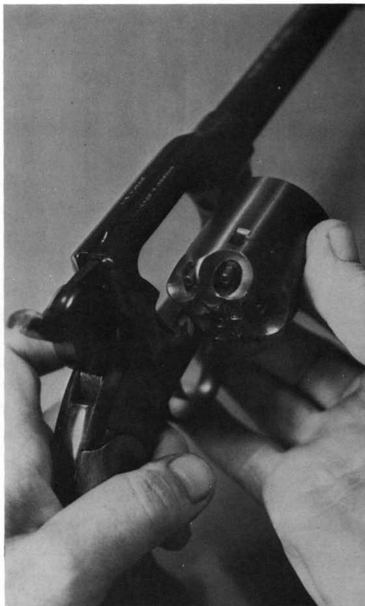
**3.** Removal of the upper screw will allow separation of the lever and the base pin. Taking out the lower screw will free the rammer for removal.
