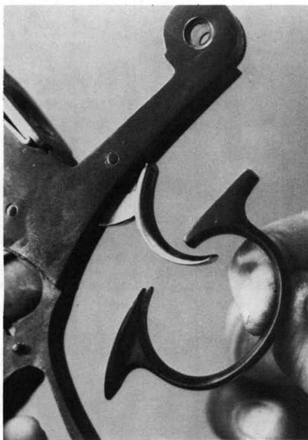
**14.** Lift the rebound lever from its pivot yoke in the frame and move it toward the rear and downward for removal.
