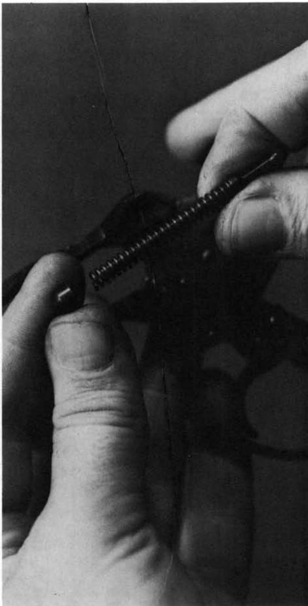
**12.** Move the cylinder latch to the rear, hold it there, and pull the trigger to tip the hammer back. Remove the hammer toward the right. Drifting out the small pin at the front of the hammer will allow removal of the double-action lever and its spring.
