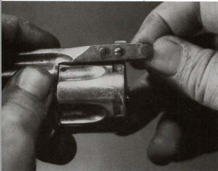
2. In this view, the retainer can be seen in its slot on the underside of the latch. Both are shown in the raised and locked position.
