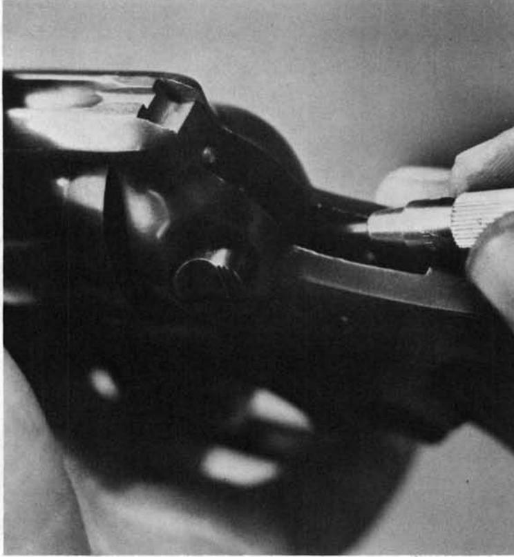
2. When moving the trigger guard unit back into the frame, insert a small screwdriver to bear against the cylinder hand, keeping it pushed toward the right as the guard is snapped into place. Otherwise, the lobe on the back of the hand will jam against the rear edge of its channel.
