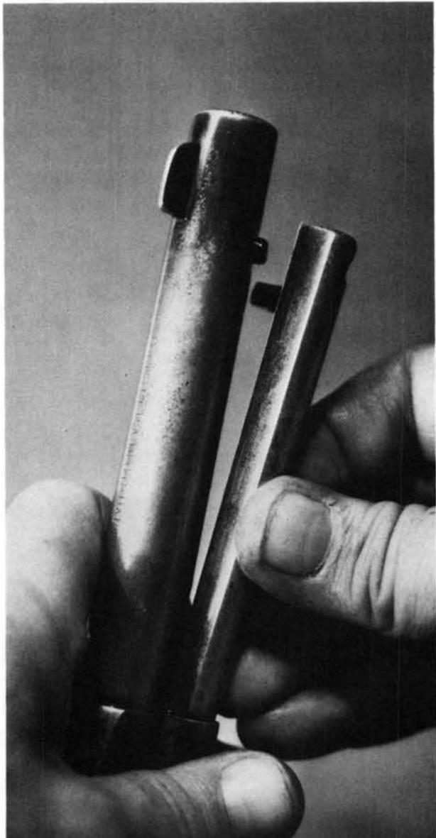
**20.** Move the ejector and its spring toward the rear of the housing, turn the ejector handle over into the exit track, and remove the ejector and spring toward the rear.
