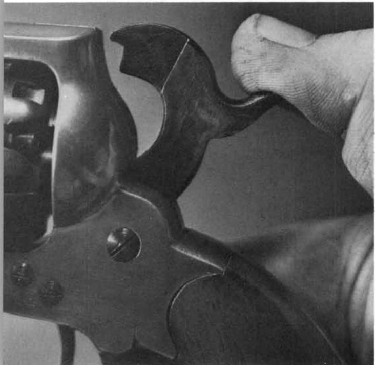
2. Give the cylinder pin retainer a half-turn. That is, turn it until its lower surface is at the top.
