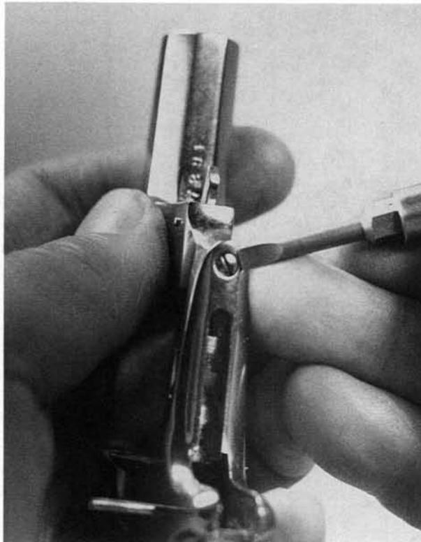
**17.** Drift out the base pin latch cross-pin.
