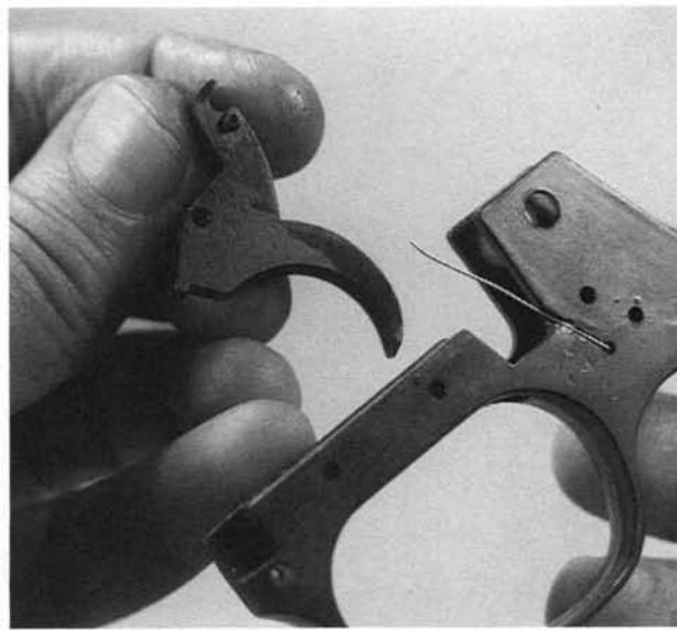
**30.** Remove the trigger upward.
