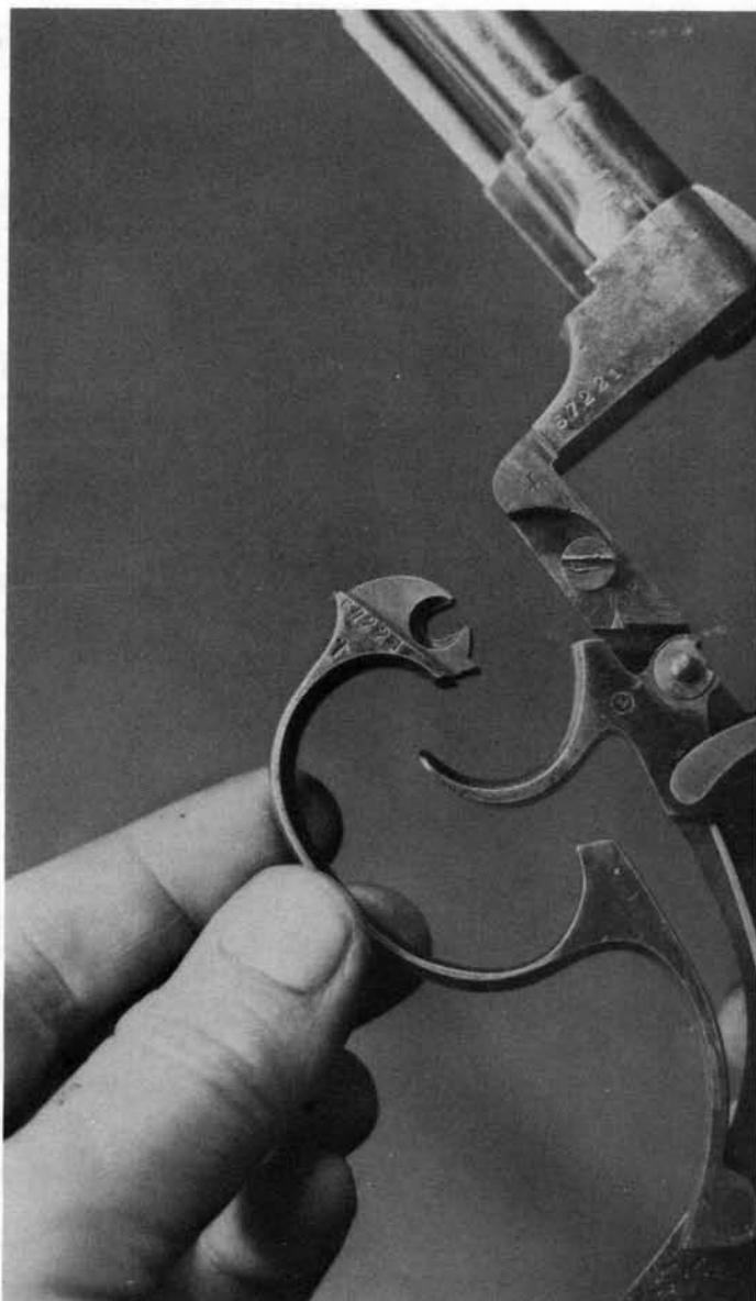
**10.** Grasp the mainspring with smooth parallel-jaw pliers, compress it slightly, and lift its rear mounting stud from the hole in the grip frame. The spring can then be removed downward and to the rear.
