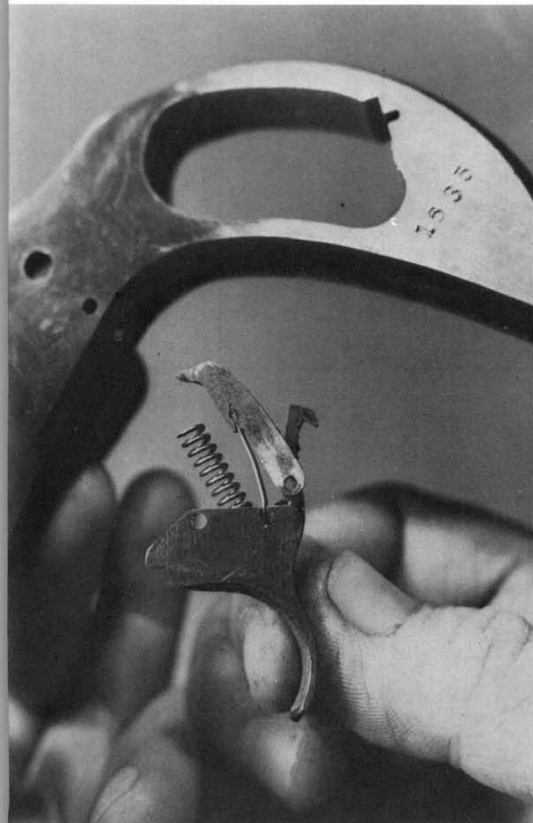
**16.** Detach the cylinder hand and its attached spring from the stud on the left side of the hammer lifter. The trigger spring is easily removed from its hole in the top of the trigger. Drifting out the cross-pin at the rear of the trigger toward the left will free the lifter for removal.
