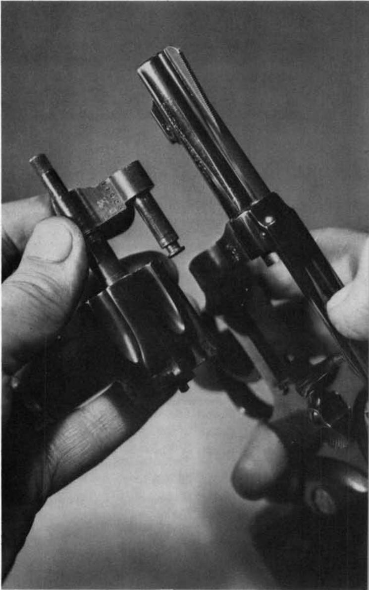
3. Remove the crane from the front of the cylinder.
