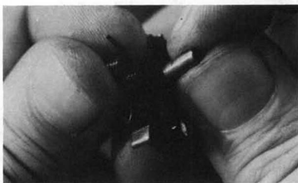
**17.** Push out the trigger pivot bushing, and remove the trigger spring from the top of the trigger.
