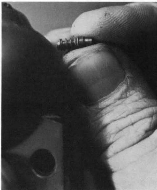
**22.** Remove the firing pin housing toward the front.
