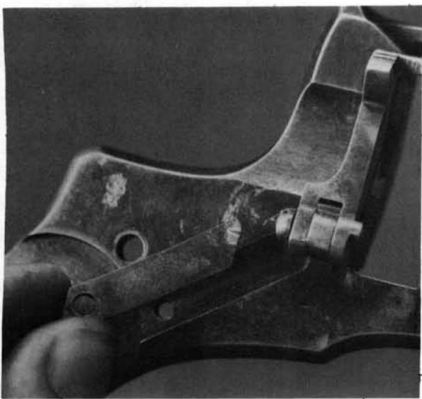
**19.** Take out the large screw that retains the loading gate spring, move the spring toward the rear and downward, then remove it toward the right.
