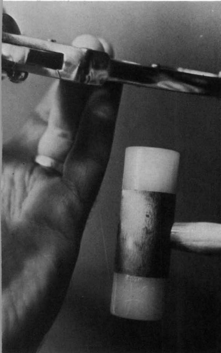
**11.** Remove the cylinder latch thumb piece and its spring and plunger from the sideplate.
