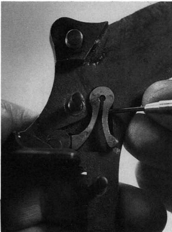
**14.** Tip the cylinder latch lever to the rear, to clear its notch at the top, and remove it toward the right.
