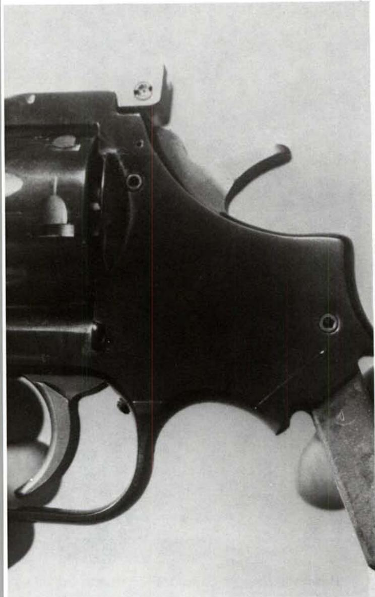
**6.** Hold the gun as shown and tap the grip extension with a nylon mallet until the sideplate falls into the hand.
