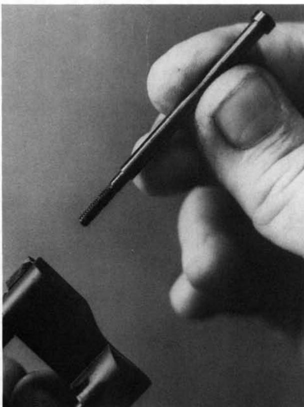
**10.** Remove the ejector rod from the front of the crane.
