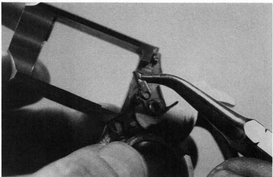
**9.** Carefully remove the tiny torsion spring that powers the cylinder hand from the hammer. Tweezers are recommended.
