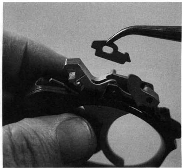
3. The cylinder stop trip goes back into its slot in the top of the trigger as shown.
