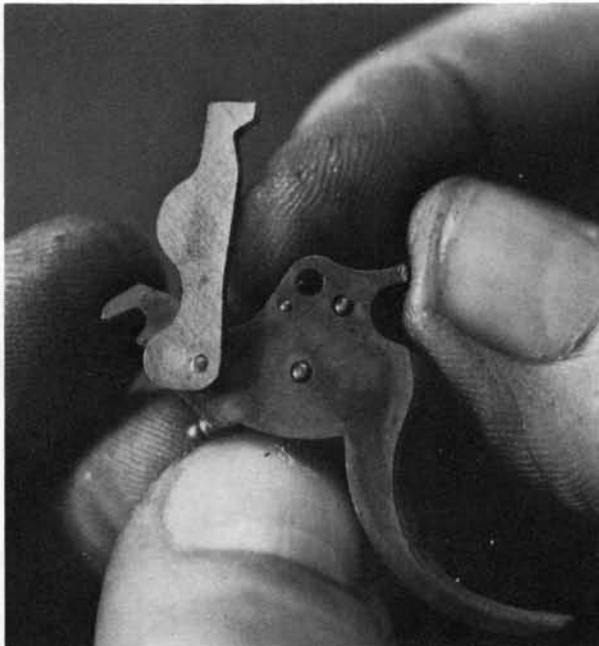
**17.** Use a small screwdriver to depress the cylinder stop at the top, and insert another small screwdriver behind the stop to nudge it out toward the right. As the spring at the front of the stop nears the edge of the frame recess, control it and ease it out.
