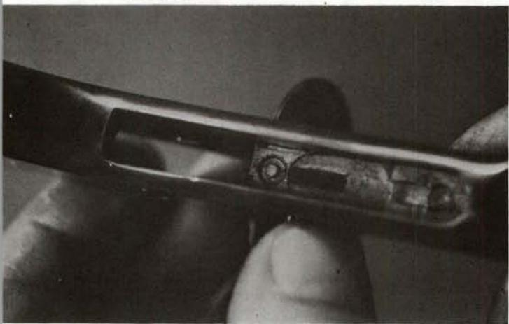
When replacing the firing pin housing in the frame, be sure the retaining groove is at the bottom, and use a tapered tool inserted through the pin hole to insure alignment before inserting the original pin.
