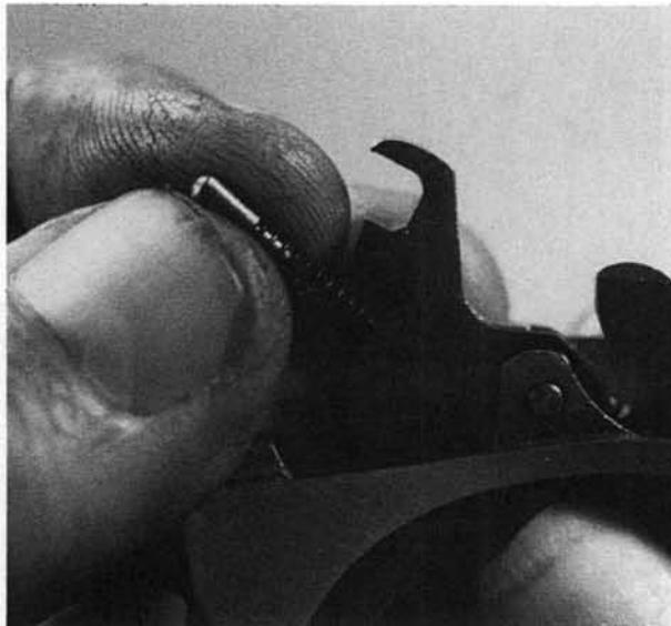
**18.** Push out the trigger cross-pin.
