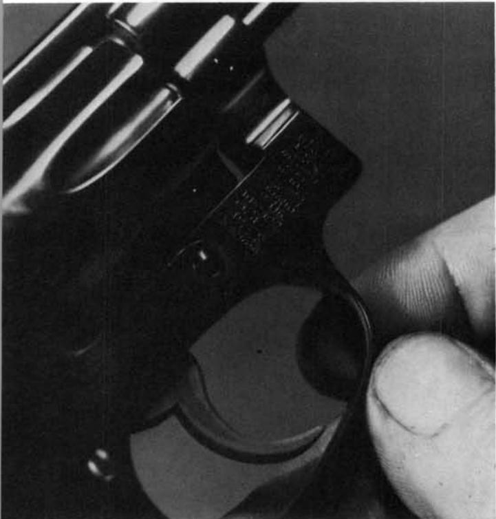
2. Move the crane forward out of the frame, and remove the cylinder and crane assembly toward the left.
