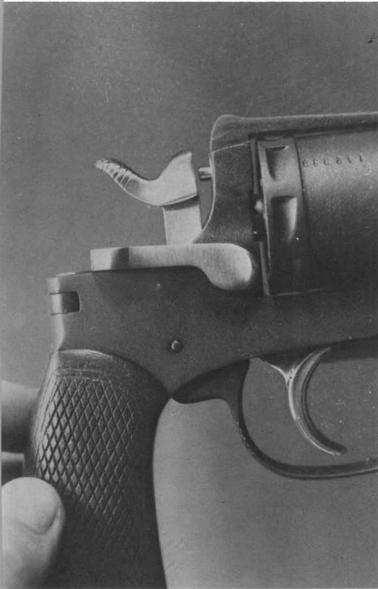
2. Pull the ejector assembly latch downward and turn it slightly, so its side lug will lock it in position.
