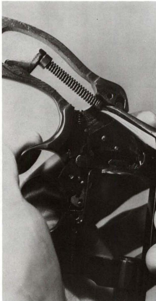
**11.** Take care not to lose the hammer spring cup, as it will be freed when the spring and strut are removed.
