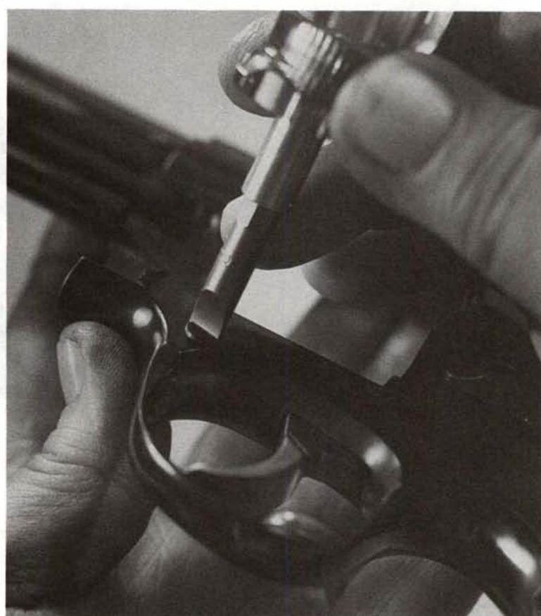
**16.** Remove the screw at the center of the cylinder latch button, and take off the button toward the left.
