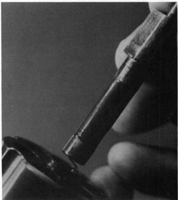
3. With leather-padded pliers, unscrew the ejector rod (turning it toward the left, front view) and remove the rod and crane from the cylinder. If the rod is very tight, pad a vise with leather or wood, insert two empty cartridge cases in opposite chambers to stabilize the ejector. Then clamp the rod into the vise, turning the cylinder by hand until it breaks free.
