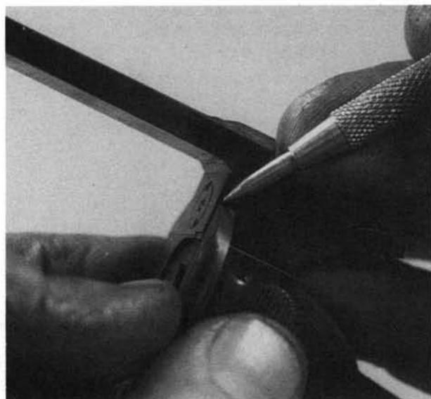
**2.** When replacing the sideplate, align the cylinder latch piece with the edge of the sideplate and the frame, so the stud on the latch plunger will enter the hole in the latch piece.
