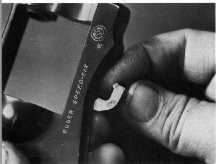
**25.** Remove the cylinder stop from the underside of the frame.
