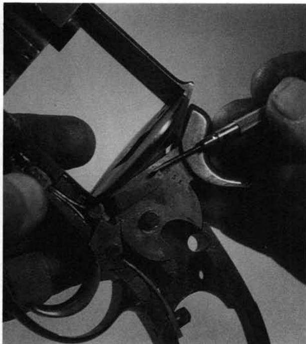
**16.** Depress the trigger, and remove the hammer toward the left.
