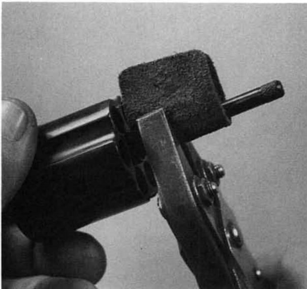
**5.** Remove the ejector rod and the ejector spring and collar toward the front.
