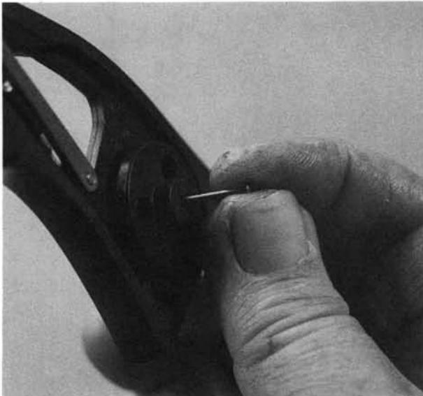
2. Cock the hammer, and insert the disassembly pin in the hole in the mainspring guide rod.
