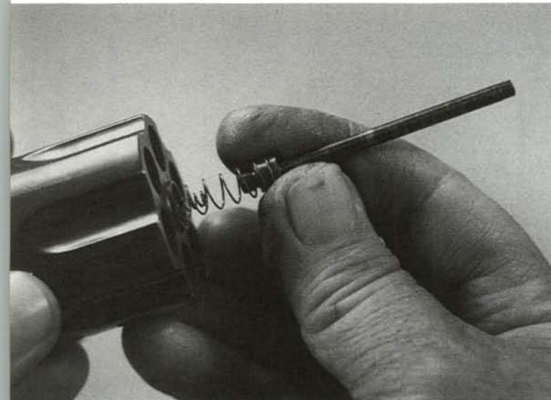
**11.** Remove the cylinder latch plunger and spring toward the front.
