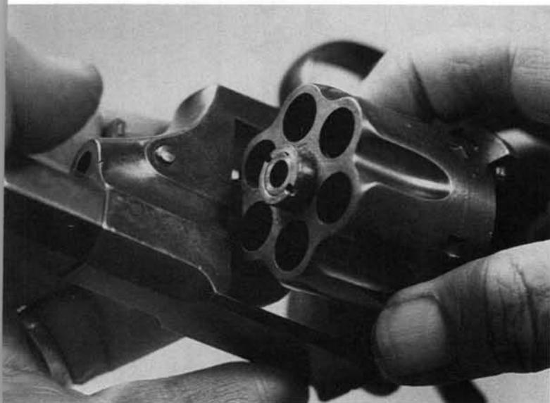
**4.** To remove the base pin latch, turn it upward, and unscrew it from the frame counterclockwise. To prevent marring of the frame on the first turn, use a piece of index card as a shield.
