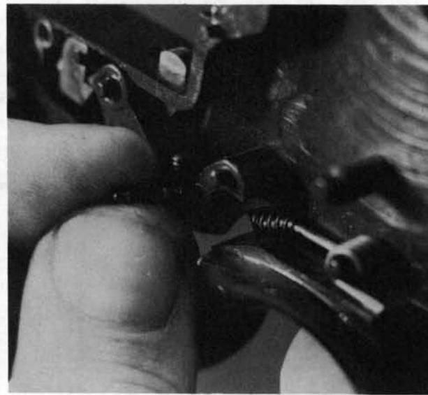
**18.** Remove the spring bearing pin from the trigger.
