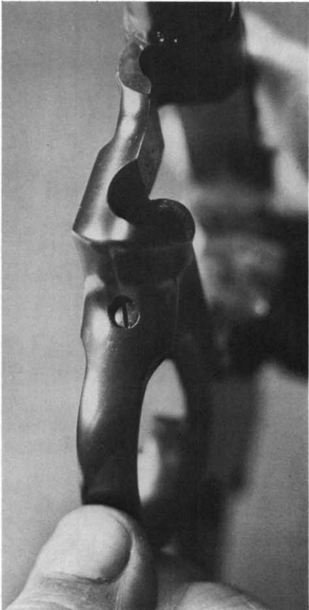
**18.** Tip the cylinder stop downward out of its slot in the frame, and move it out to the right for removal.
