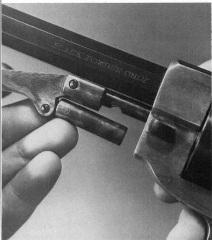
3. Remove the cylinder pin, and the attached loading lever assembly, toward the front.
