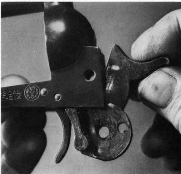
**9.** Drifting out the cross-pin at the middle front of the hammer will release the cylinder stop trip plunger and spring for removal downward.
