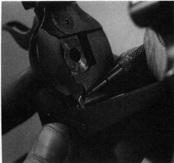
**3.** When replacing the trigger cross-pin, the gate spring must again be depressed. This time, put the end of a slim tool in the "hook" of the spring, and keep pressure rearward as well as downward, to ensure that the inside L-tip of the spring stays in its shelf on the gate.
