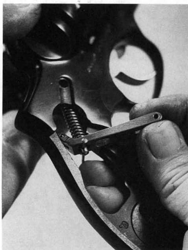
**9.** Move the lower end of the lever and spring assembly rearward, and turn it to the position shown for removal. The trigger must be forward during this operation. The mainspring unit can be disassembled if necessary. If this is done, control the powerful and compressed mainspring as the disassembly pin is removed.
