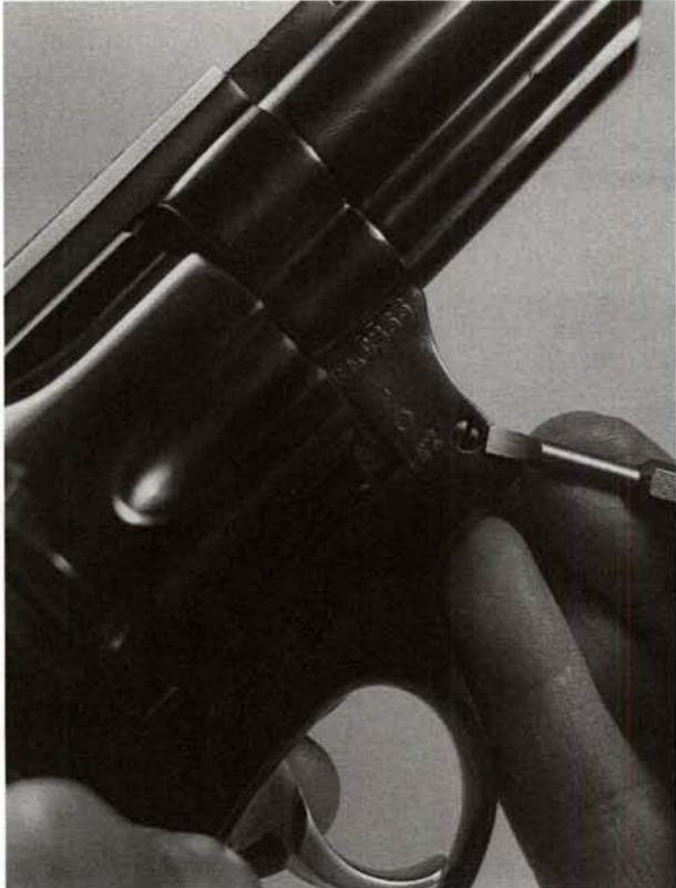
**2.** Operate the cylinder latch, move the crane and cylinder assembly forward out of the frame, and take it off toward the left.
