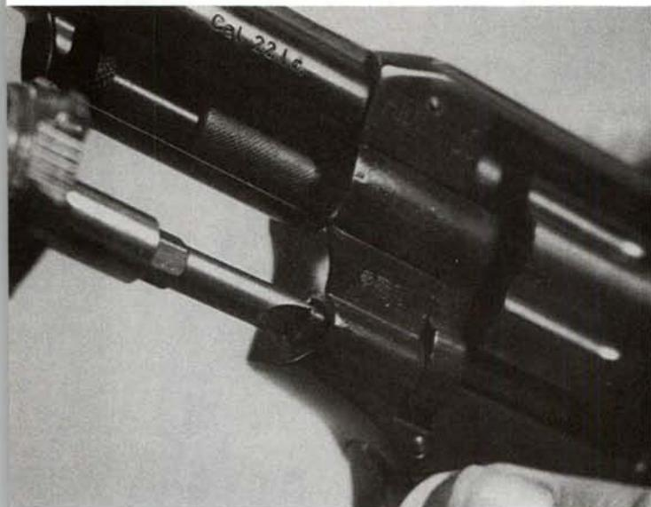
2. Operate the cylinder latch, and remove the crane and cylinder assembly toward the left.
