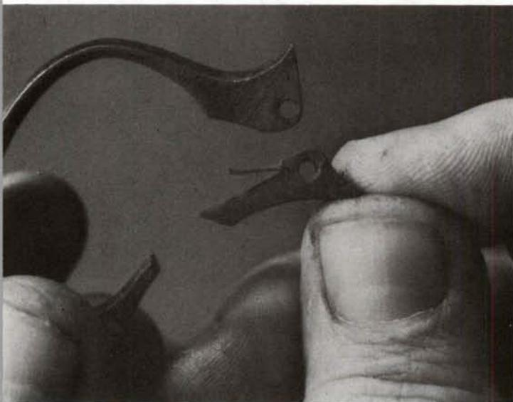
**14.** Remove the trigger spring from the front of the guard recess in the frame.
