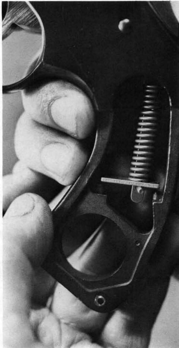
**5.** Remove the strut, spring, and base unit toward the left and downward. If these parts are to be separated, place the baseplate against the side of a slightly opened bench vise, and exert pressure to compress the spring while taking out the pin. Keep a firm grip on the top of the strut, and release the spring tension slowly.
