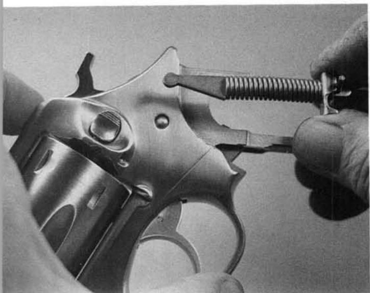
**4.** The hammer spring assembly is shown here in the proper orientation for installation.
