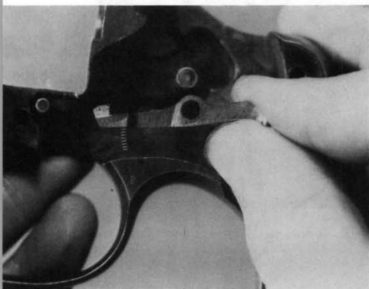
**19.** After removal of the screw, pry the cylinder stop spring outward from its recess in the frame with a small screwdriver. Move the cylinder stop down, then toward the rear for removal. Take care that the small spring is not detached and lost.
