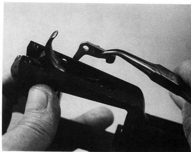
**19.** Move the trigger out until it can be detached from the transfer bar and removed.
