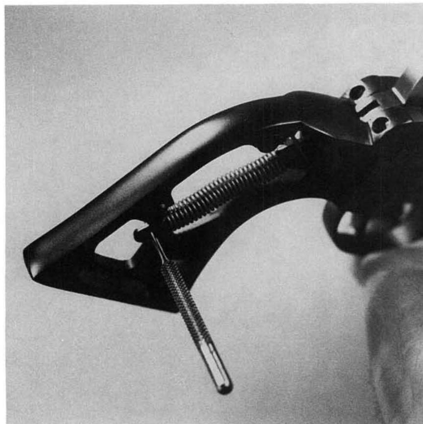
**4.** Pull the trigger and ease the hammer down. The spring will be trapped on the guide. It is not removed at this time.
