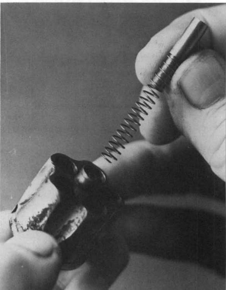
**4.** Remove the ejector/ratchet from the rear of the cylinder.
