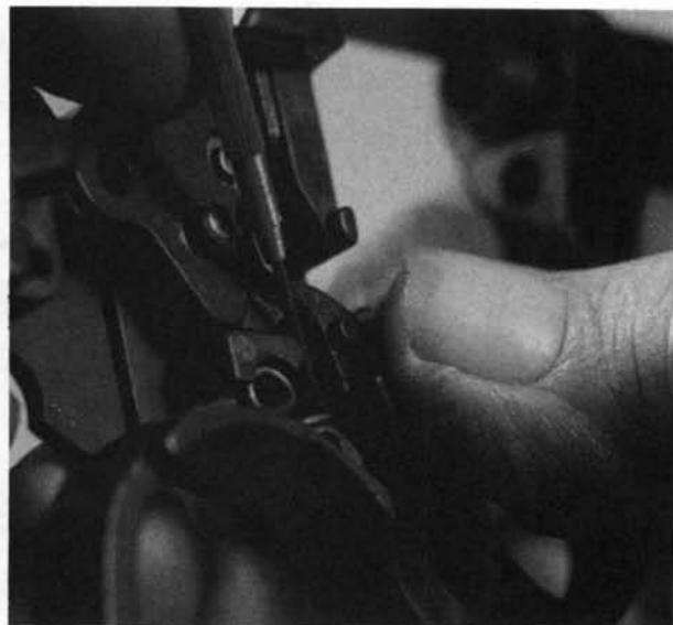
**3.** As the trigger is reinstalled, be sure the stud at left rear engages the hole in the transfer bar. Also, as shown here, be sure the front arm of the trigger spring bears on the cross-pin in the trigger.
