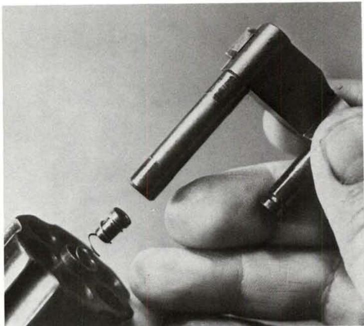
**12.** Remove the ejector spring and its bushing from the front of the cylinder.
