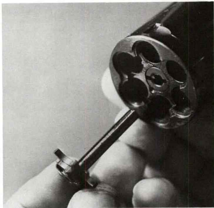
**13.** Remove the ejector/ratchet from the rear of the cylinder.
