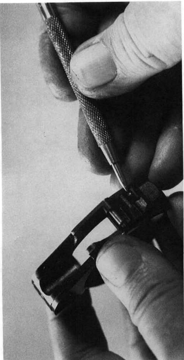
**19.** The crane pivot lock plunger and spring are staked in place at the factory, and they are not routinely removable.
