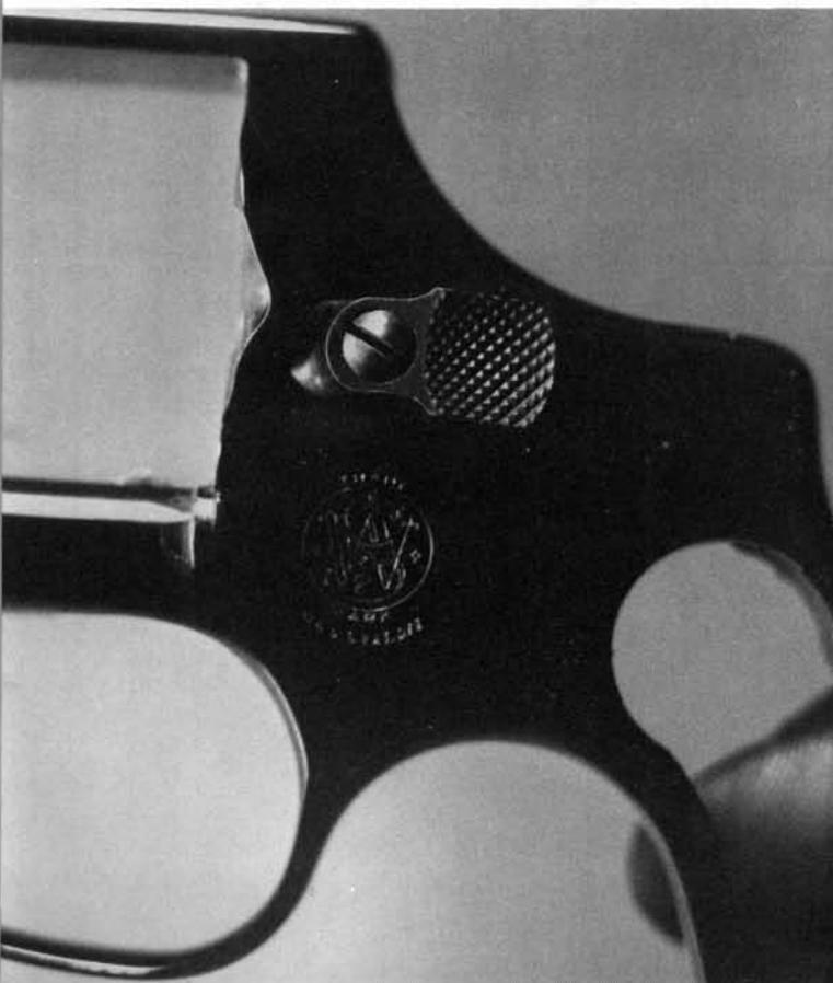
**18.** Remove the large cap nut from the cylinder latch, and remove the latch piece toward the left.
