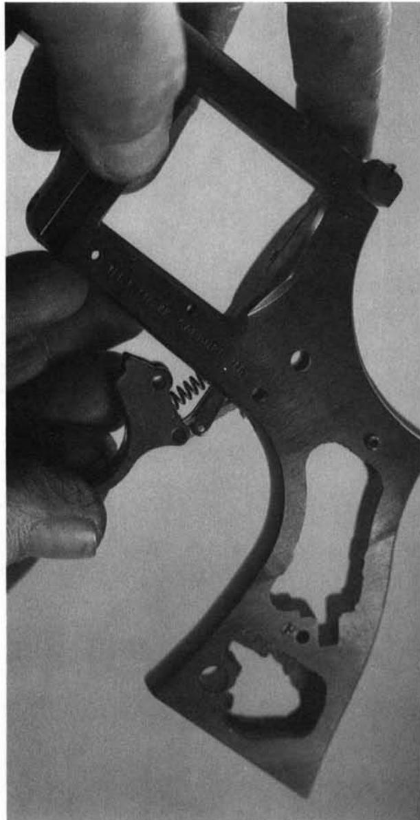
**17.** Drift out the trigger cross-pin toward the right.
