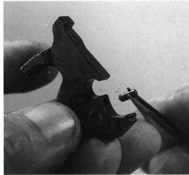
**21.** Remove the lever plunger from the front of the hammer.
