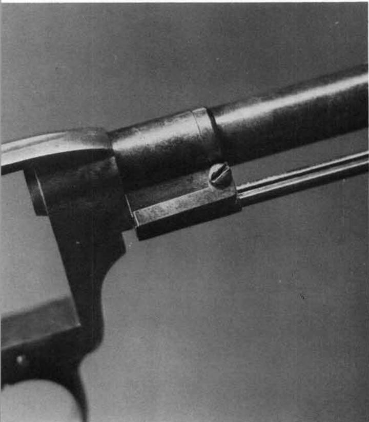
**22.** Removal of the spring will release the ejector rod, allowing it to be pulled out toward the front. The ejector housing can be taken off only after barrel removal, and this is not advisable in normal takedown.
