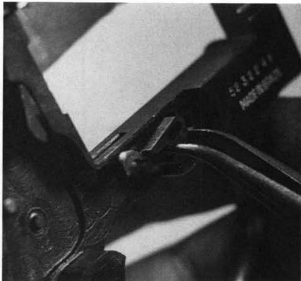
**23.** Remove the screw from the cylinder latch piece, and take off the latch piece toward the left.
