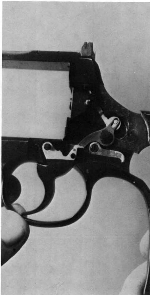
**16.** Remove the cylinder latch bolt toward the rear.
