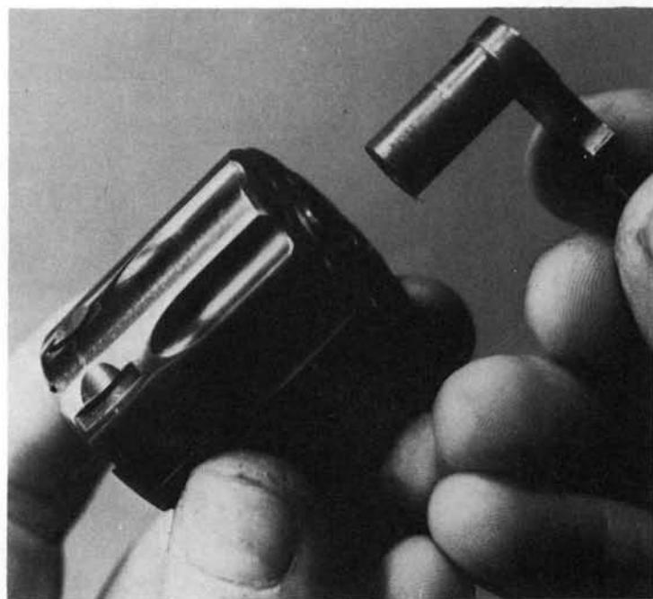
**11.** Drift out the cross-pins at the front of the trigger guard and at the rear center of the frame. Remove the sub-frame downward.
