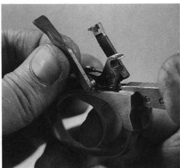
**13.** Depress the trigger slightly, and remove the transfer bar from the left side.
