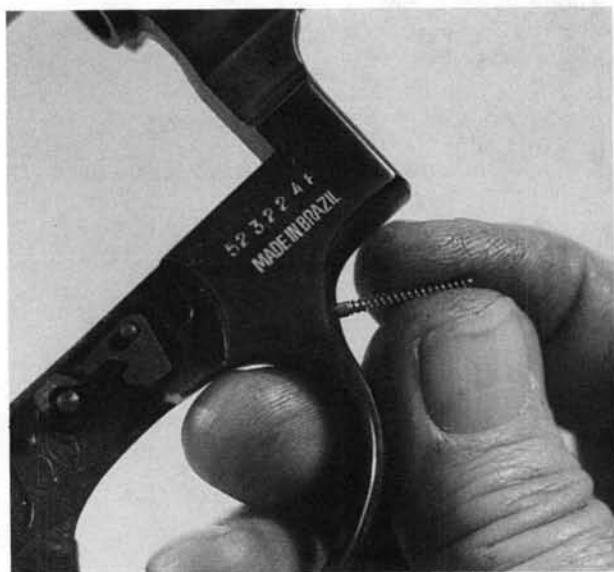
**21.** Remove the cylinder stop spring and plunger.
