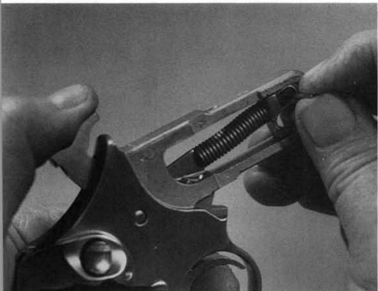
**5.** Cock the hammer, and insert the disassembly pin through the hole in the hammer strut.
