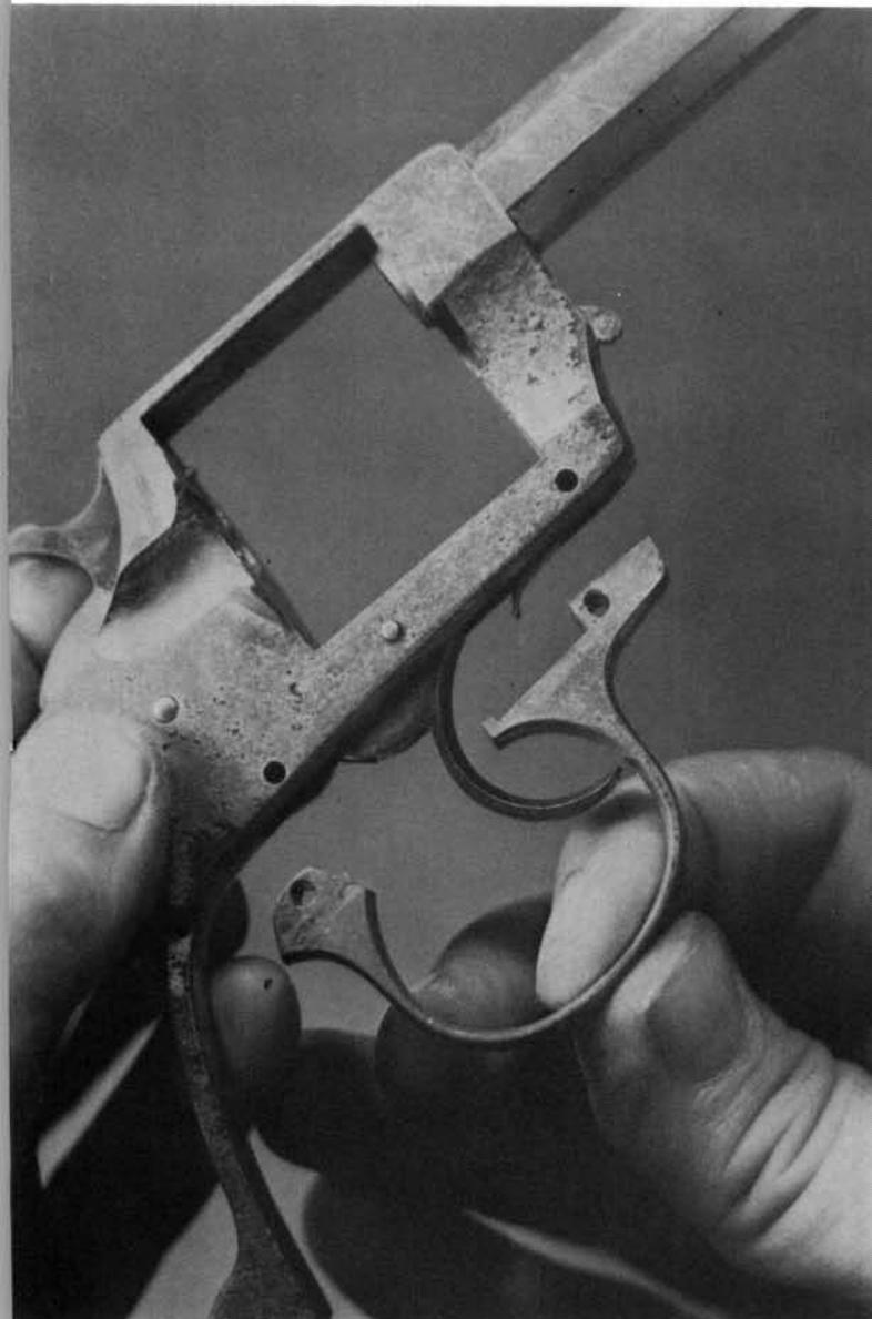
**4.** Remove the trigger spring from the lower front of the frame.
