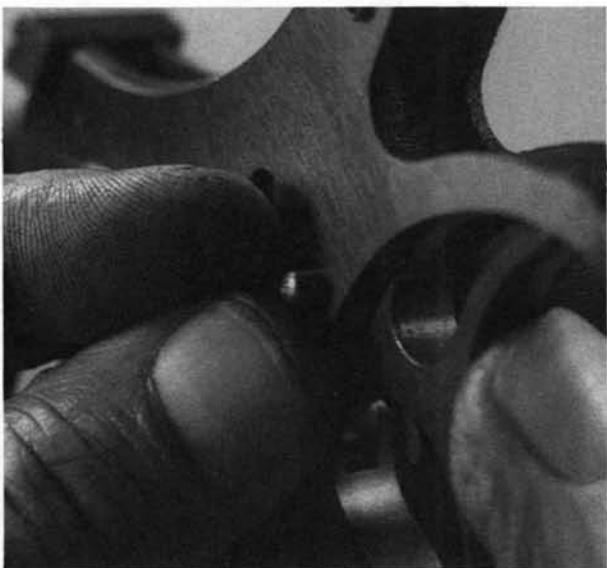
**5.** Before replacing the hammer in the frame, be sure the sear is turned down to the position shown, and keep the trigger pulled as the hammer is put in. Also, be sure the transfer bar is forward.
