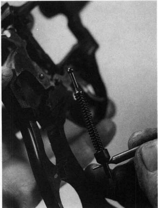
**14.** Push the cylinder latch to the rear, pull the trigger, and remove the hammer toward the right. The cross-pin at the front of the hammer can be drifted out to release the double-action lever and its spring for removal, but in normal takedown they are best left in place.
