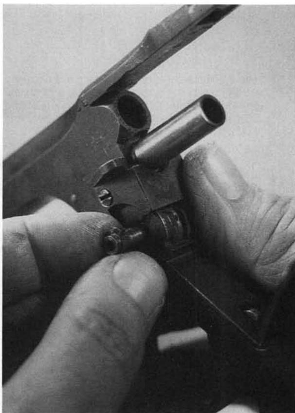
**8.** Remove the barrel hinge cap screw on the right side, and push out the barrel hinge toward the left. If the hinge is tight, first loosen the screw two turns, and tap it with a nylon mallet before removal, to start the hinge leftward.
