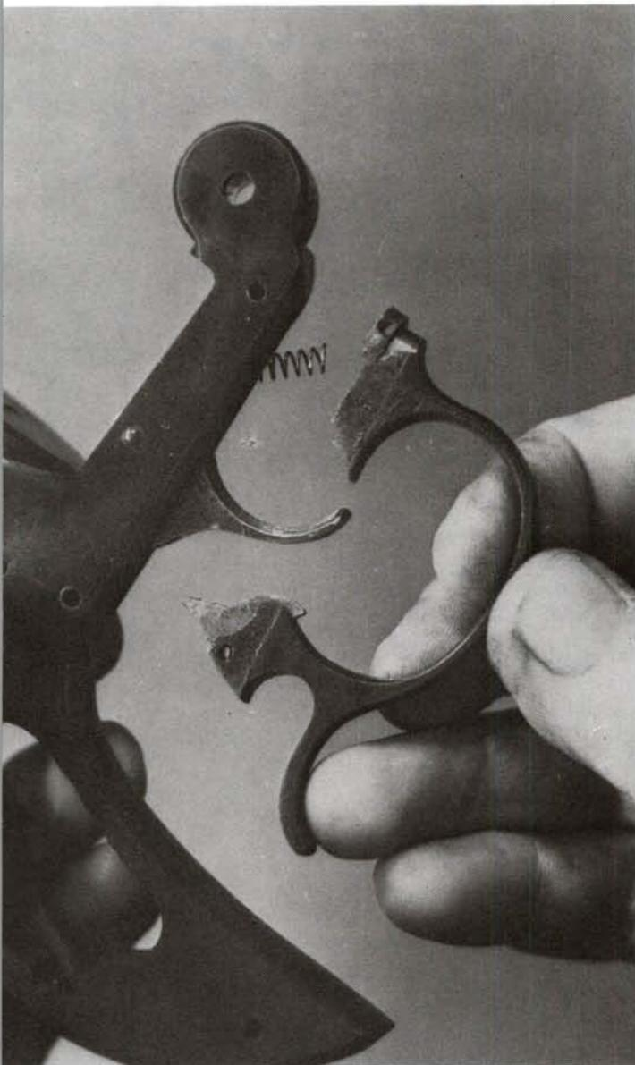
**13.** Remove the sear and its spring from the top rear of the guard.
