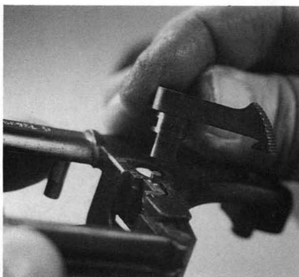
**15.** Swing the cylinder latch lock-piece out of its recess toward the front, and remove it toward the right.
