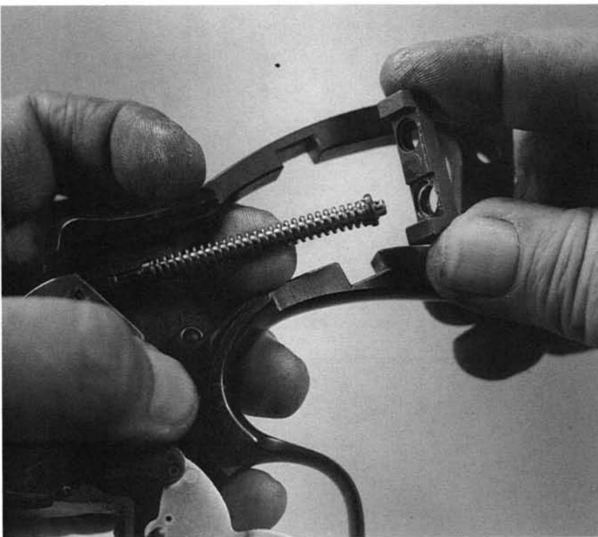
**4.** When installing the cylinder latch bar, it can't be just laid inside, as shown, because the small plunger and spring at the rear will not enter the sideplate recess, and they will be damaged.
