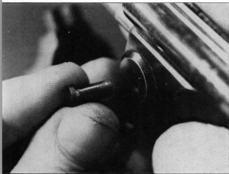
**7.** Remove the ejector cam downward from the barrel.
