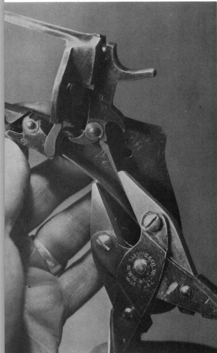
**11.** The hammer and trigger systems are shown here in the proper arrangement.
