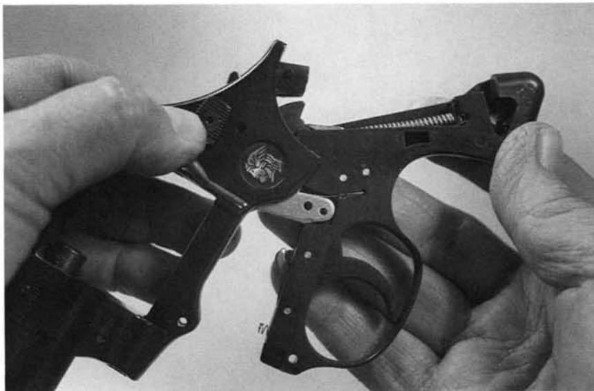
**15.** Push the cylinder latch button rearward, to clear the hammer block cross-piece, and remove the sub-frame downward
