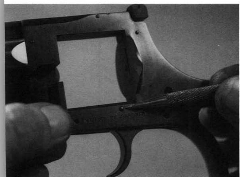
**19.** Remove the transfer bar from its post on the right side of the hammer lever.
