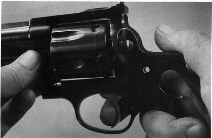
**7.** As the mainspring unit is put back in the gun, be sure the trigger strut engages the recess in the end of the spring guide rod, shown here. The engagement is visible through the hammer slot.
