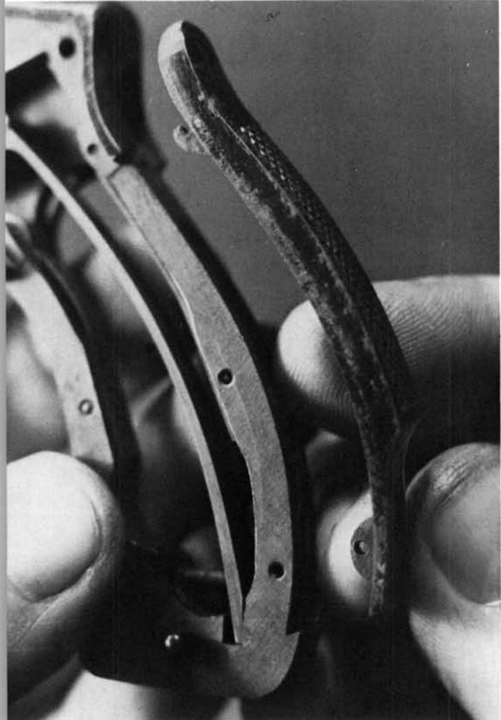
**16.** Back out the hammer spring screw, located at the lower front of the grip frame. Move the lower end of the hammer spring out toward the left, detach the spring hooks from the hammer stirrup, and remove the spring downward.
