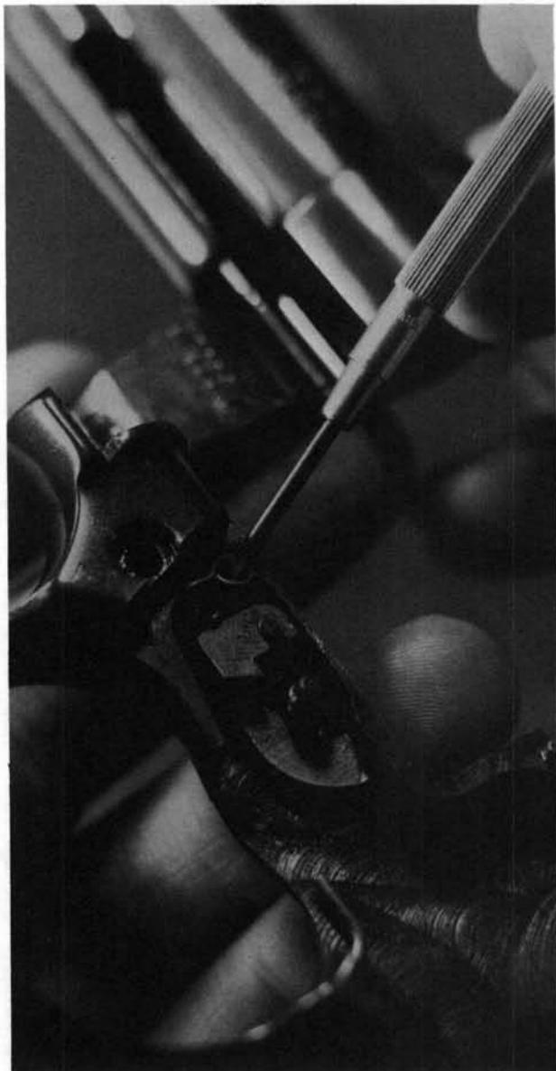
**22.** Use a small tool to lift the cylinder stop out toward the left. Note that it must be tipped downward, out of its slot in the floor of the cylinder recess. The firing pin and its spring and bushing are retained by a cross-pin, and after removal of the pin all three parts are removed forward. A cross-pin also retains the rear sight. After removal of the pin, the elevation screw must be turned counterclockwise to free the sight for removal.
