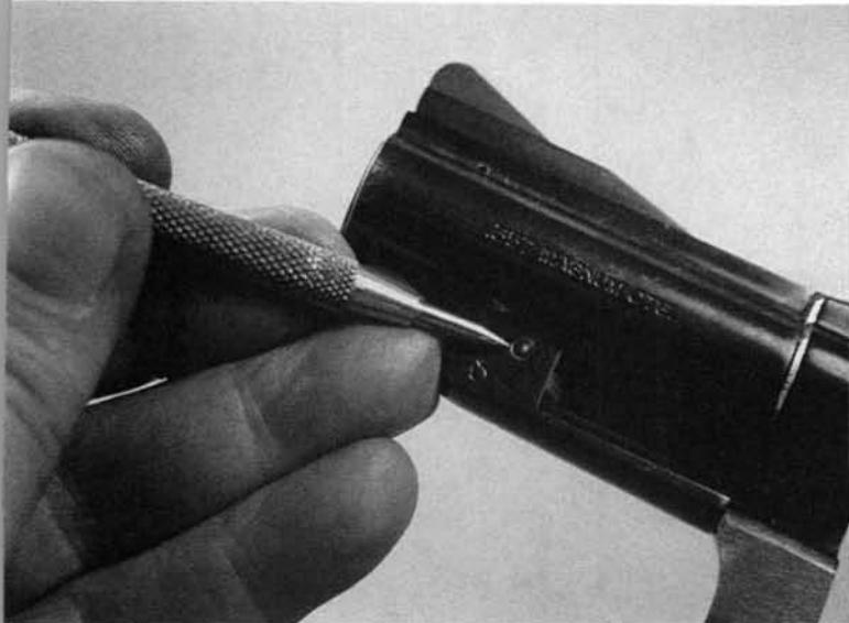
**26.** The firing pin and its spring are retained by a small cross-pin in the frame.
