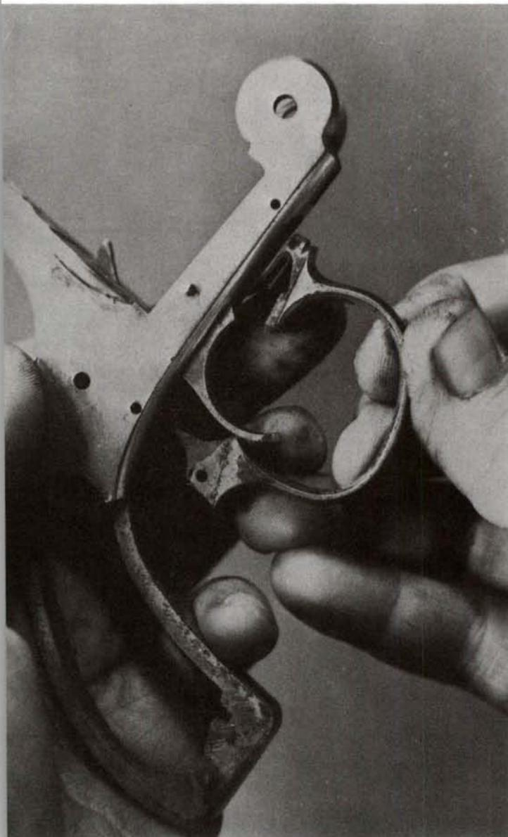
**16.** Remove the trigger spring from the underside of the frame.
