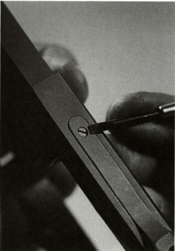
**30.** Remove the small screw in the forward extension of the rear sight.
