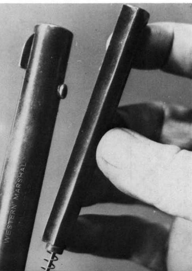
**17.** Remove the screw at the forward end of the ejector rod housing. Tip the housing away from the barrel at the front, then remove it forward, along with the ejector and spring.
