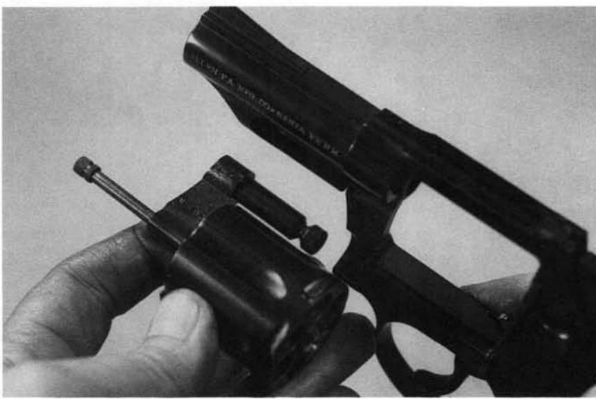
3. Operate the cylinder latch, open the cylinder, and move the cylinder and crane forward out of the frame.
