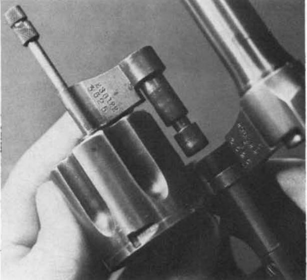
3. The existing commercial wrenches are not large enough for the ejector/ratchet of the Model 1917. To avoid marring the ejector star, use round-nosed wire bending pliers to unscrew the ejector toward the left (counterclockwise, viewed from the rear). Remove the ejector/ratchet from the end of the ejector rod.
