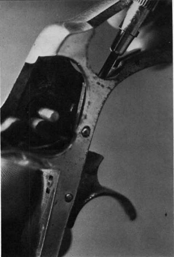
2. When installing the sear, be sure its forward beak is correctly positioned above the lower rear projection of the cylinder stop. To check proper engagement, use a small screwdriver to slightly lift the rear of the sear. The cylinder stop should then move downward into its slot in the frame.
