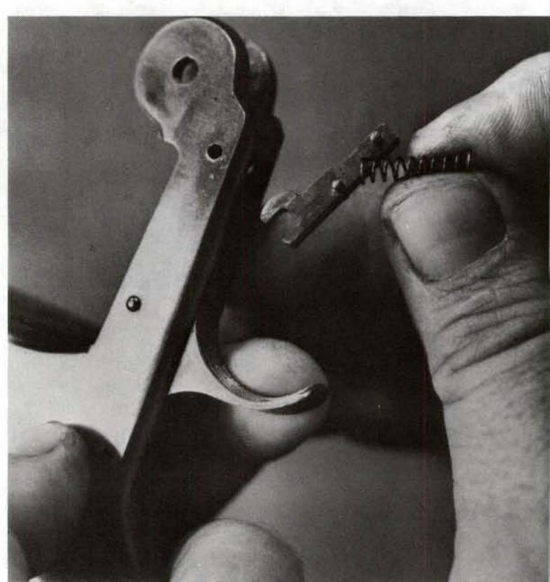
**15.** Drift out the trigger pin toward the right and remove the trigger assembly from the bottom of the frame.
