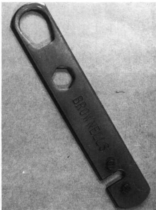
**8.** This universal Colt tool from Brownells will also work on some other autos of similar design, and even has features for some revolver work. Its main function, of course, is for the removal of a tight barrel bushing on Colt autos.
