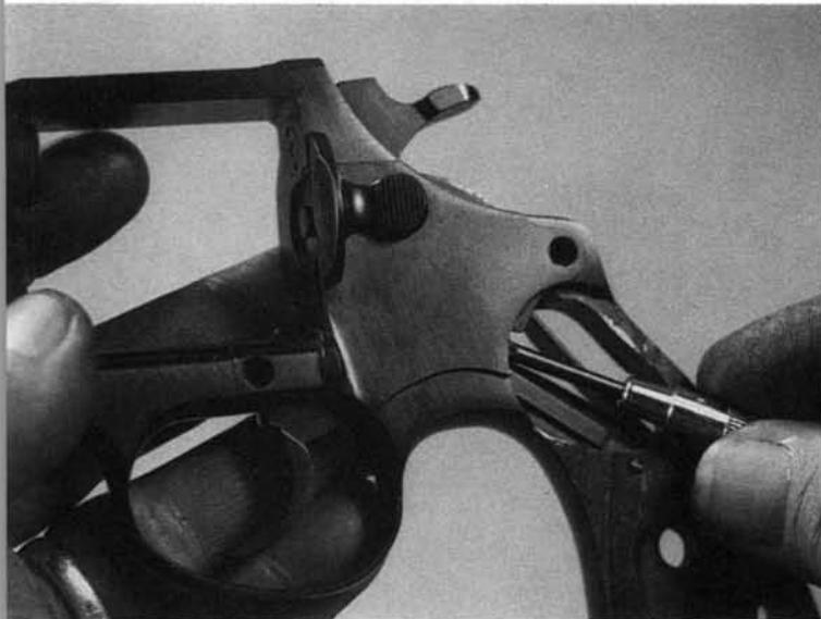
8. Remove the sideplate, and take out the cylinder latch piece toward the front. The latch piece plunger and spring are easily removed from their recess in the sideplate.
