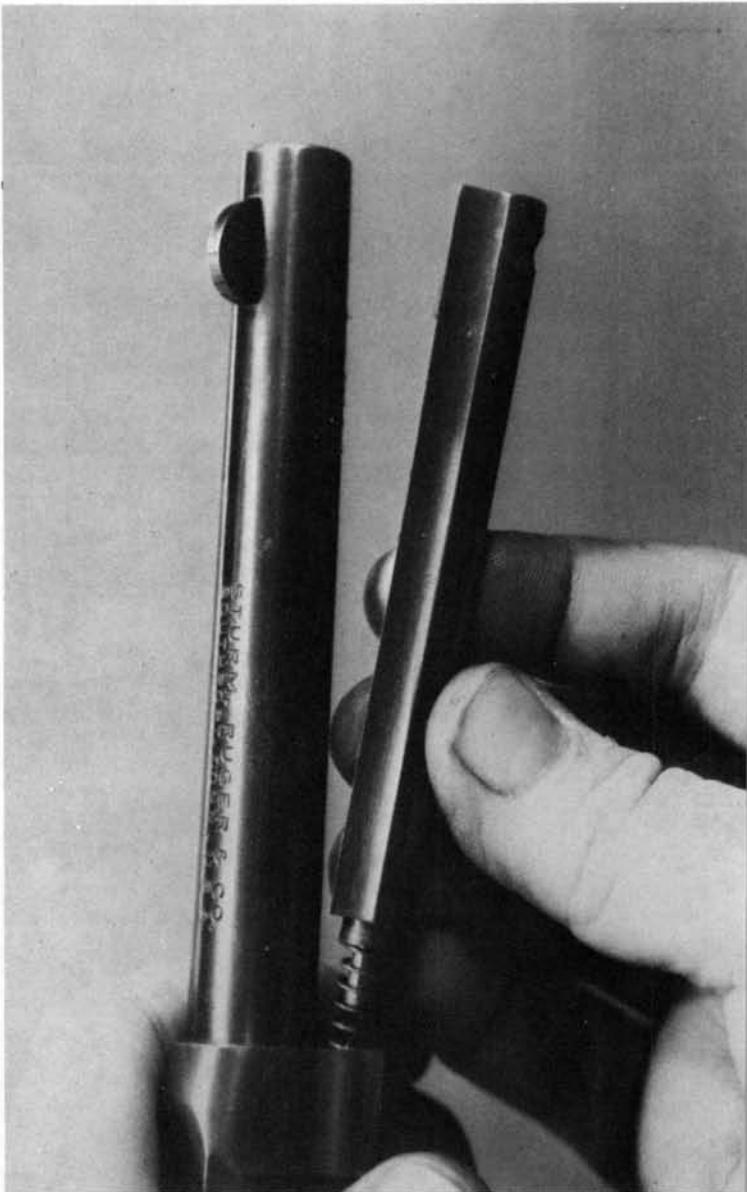
**19.** A twin-pointed tool is necessary to remove the cylinder base pin latch. The one shown was made by grinding the tip of an old Phillips screwdriver.
