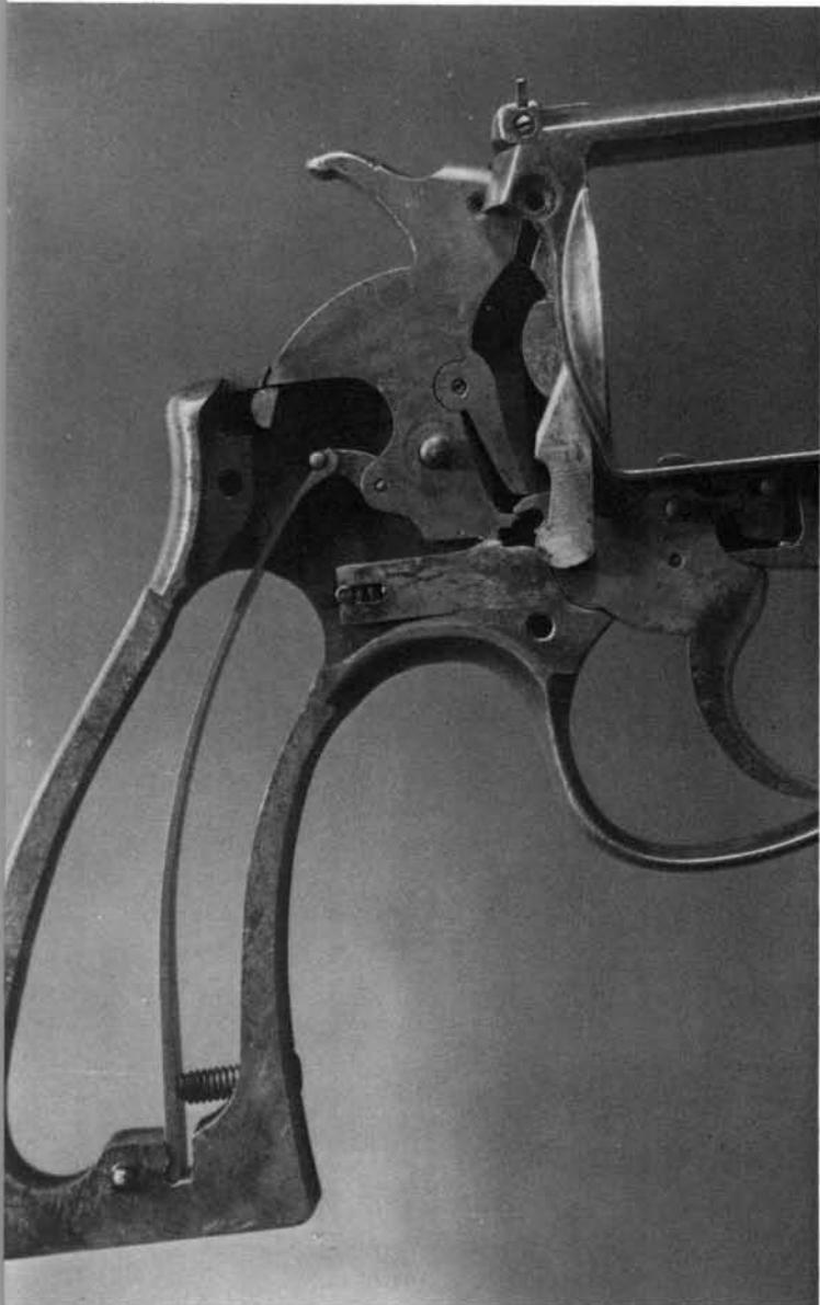
**10.** Pivot the cylinder hand toward the rear, and remove it toward the right.
