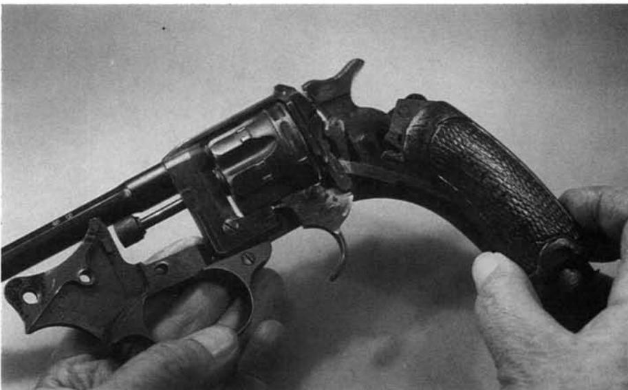
3. Slightly compress the mainspring, lift its lower end out of its recess in the grip frame, and remove it. The roller at the top of the spring is removable by drifting out the cross-pin, but in normal takedown, it is best left in place.
