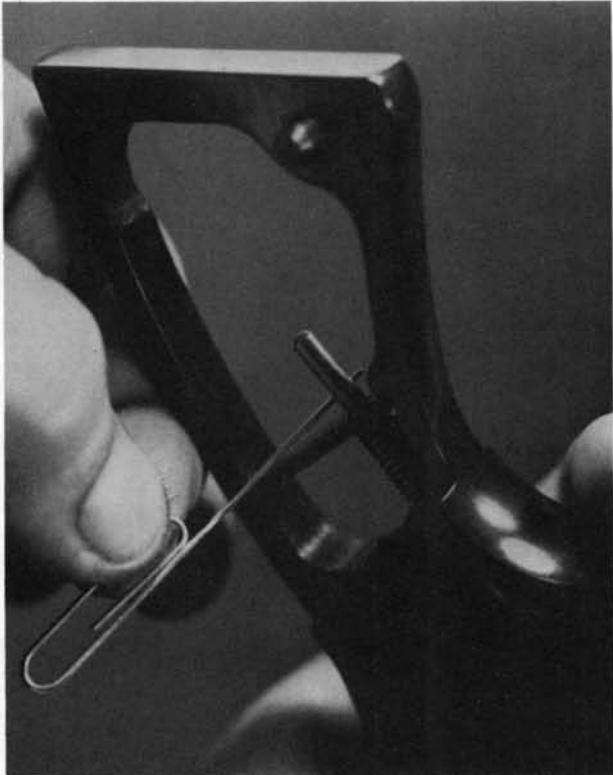
**13.** The trapped hammer spring, guide, and compression plate can now be removed from the frame. If they are to be separated, clamp the plate in a vise, push on the guide to compress the spring, and remove the paper clip from the hole. Be careful to release the spring tension slowly.
