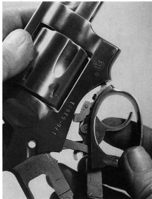
**12.** When the latch has cleared the frame, move the guard unit slightly rearward, to disengage its front projection, and take it off downward.
