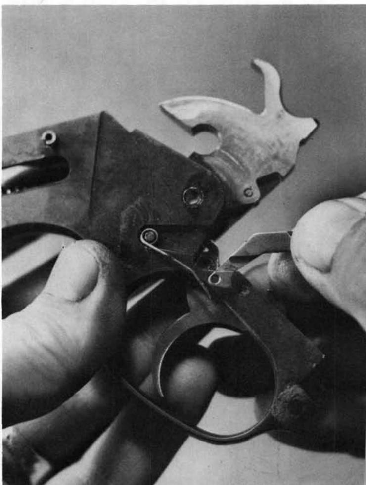
**14.** Remove the cylinder stop from the top of the sub-frame.
