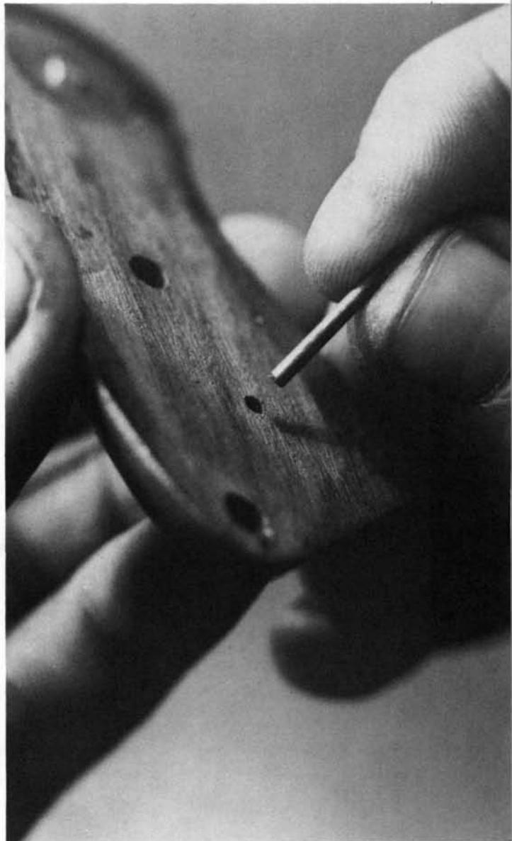
**3.** Cock the hammer and insert the disassembly pin through the hole in the lower end of the hammer strut, as shown.
