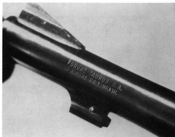
**19.** Drifting out the cross-pin in the barrel underlug will free the front lock and its plunger spring for removal toward the rear.
