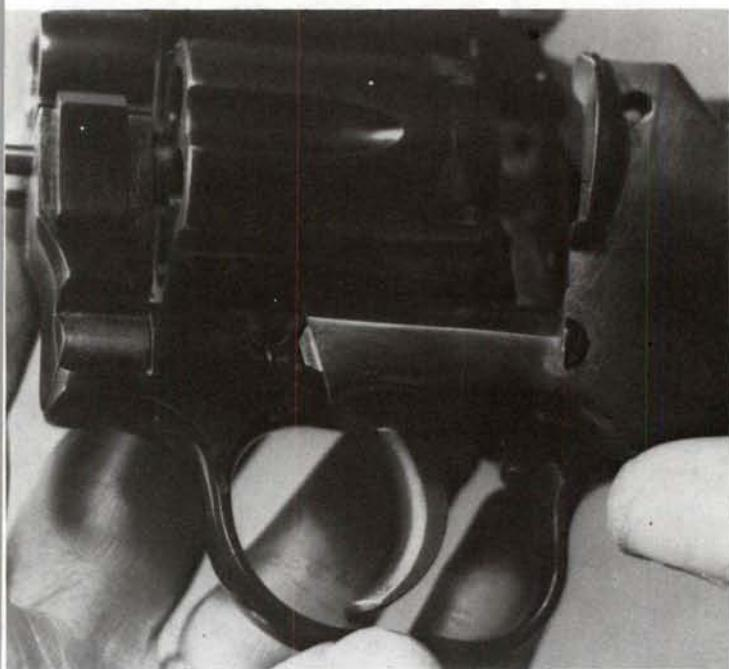
3. When replacing the sideplate, remember that the lip at its front edge must be put in first, then the rear of the plate moved inward.
