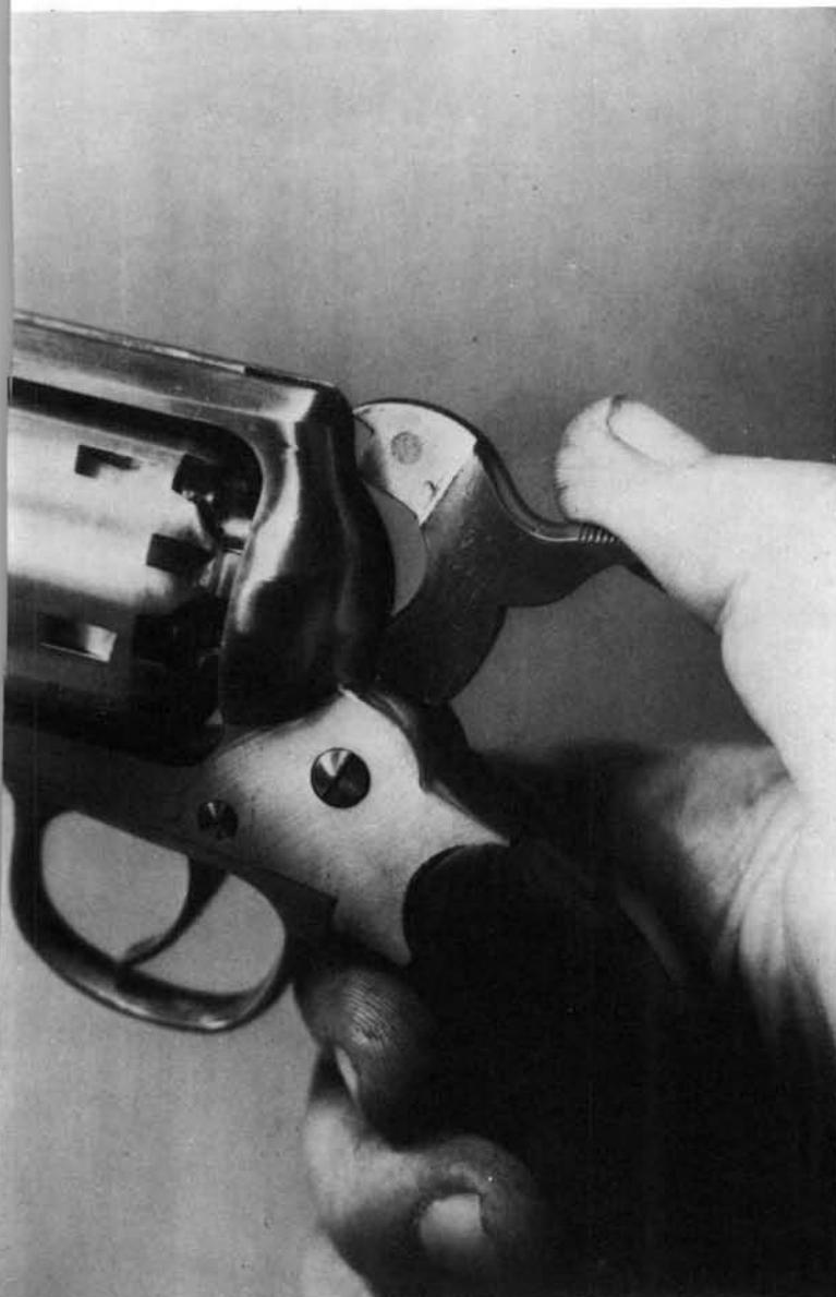
2. Swing the loading lever down and pull the cylinder base pin forward until it stops.
