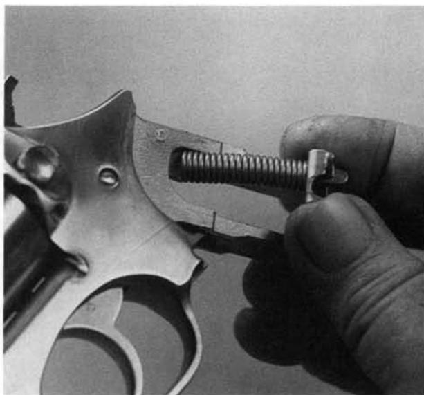
**6.** Ease the hammer down, and remove the hammer spring assembly toward either side. If these parts are to be separated, place the baseplate against the side of a slightly opened bench vise, and exert pressure to compress the spring while taking out the pin. Keep a firm grip on the top of the strut, and release the spring tension slowly.
