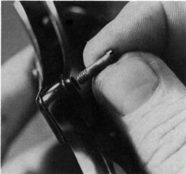
**13.** In addition to the cross-screw, the sub-frame is also retained by two pins at its lower edge, located forward and behind the trigger. Remove the forward cross-pin, then remove the rear cross-pin.
