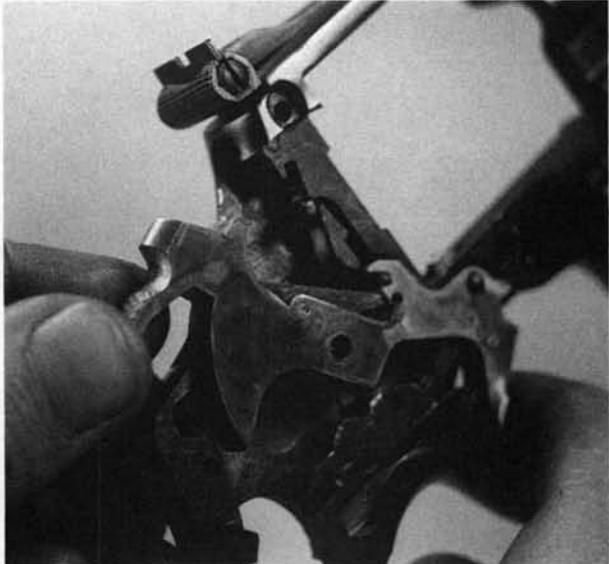
**15.** Use a small screwdriver at the rear of the rebound slide to slightly compress the spring and tip the rear of the unit outward, off its post. **Caution:** This is a strong spring, under compression, so keep it under control.
