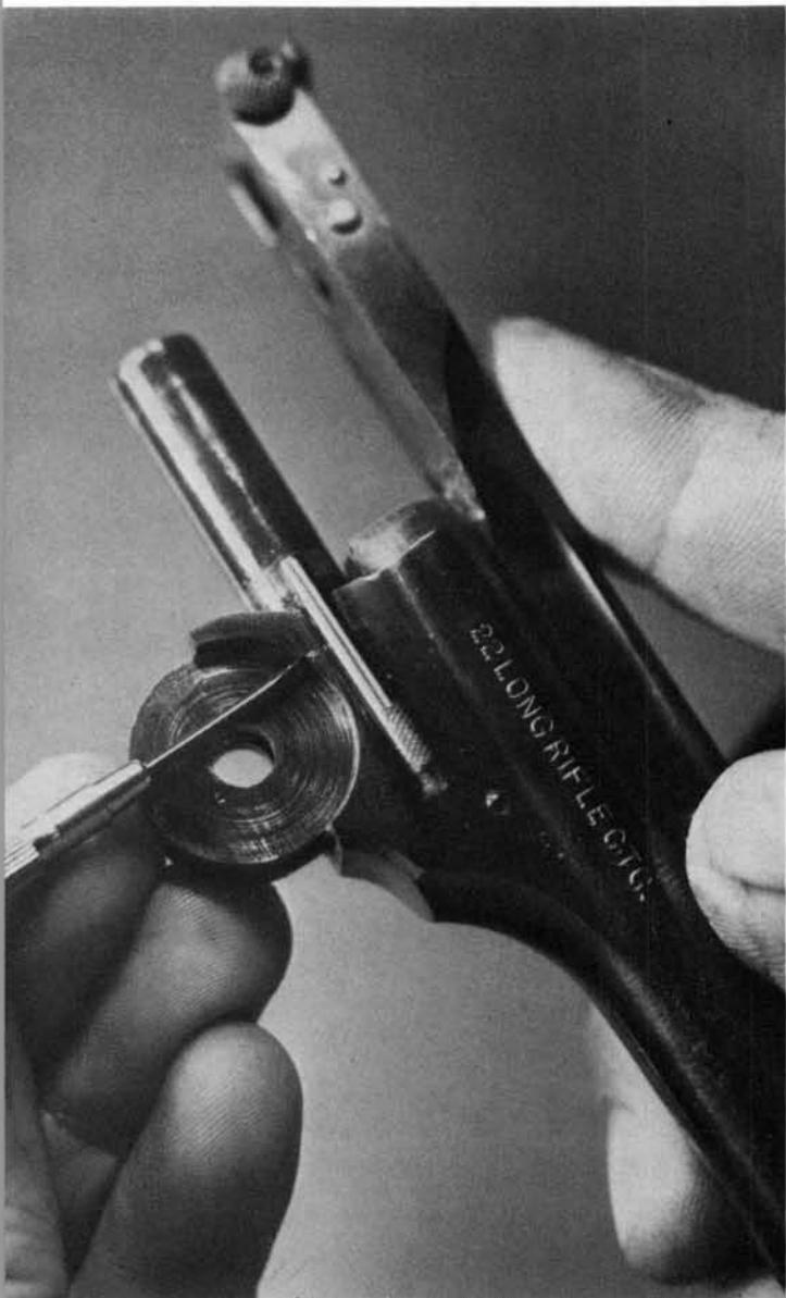
**8.** Remove the large screw at the lower rear of the grips and pull them off toward the rear.
