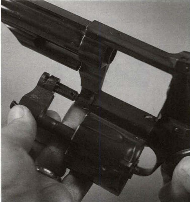
**3.** With leather-padded pliers, grip the ejector rod and the rod knob, and loosen the knob by turning it counterclockwise (front view).
