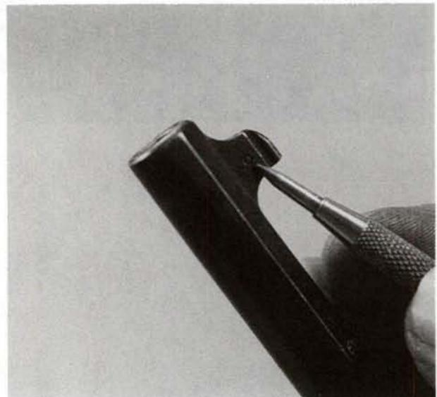
**19.** The front sight blade is retained by a small cross-pin, and the blade comes off upward. In normal takedown, it is left in place.
