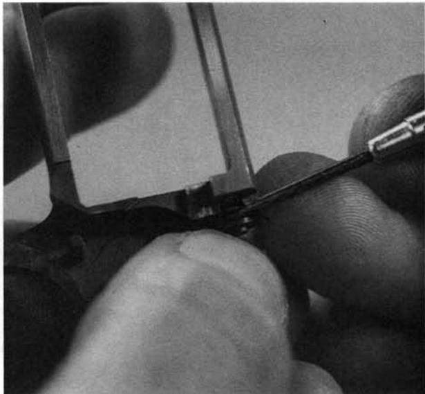
**13.** If necessary for repair, a small screwdriver or drift can be inserted at the rear to nudge the base pin spring out the front of the cylinder.
