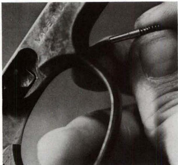
**19.** Tip the cylinder stop down out of its slot in the frame, and lift it out toward the right.
