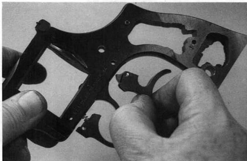
3. Installation of the trigger guard, along with the sear and sear spring, will require a short slave pin to hold the sear until insertion of the rear cross-pin. Also, be sure that the cylinder stop spring properly enters its recess in the front of the guard.
