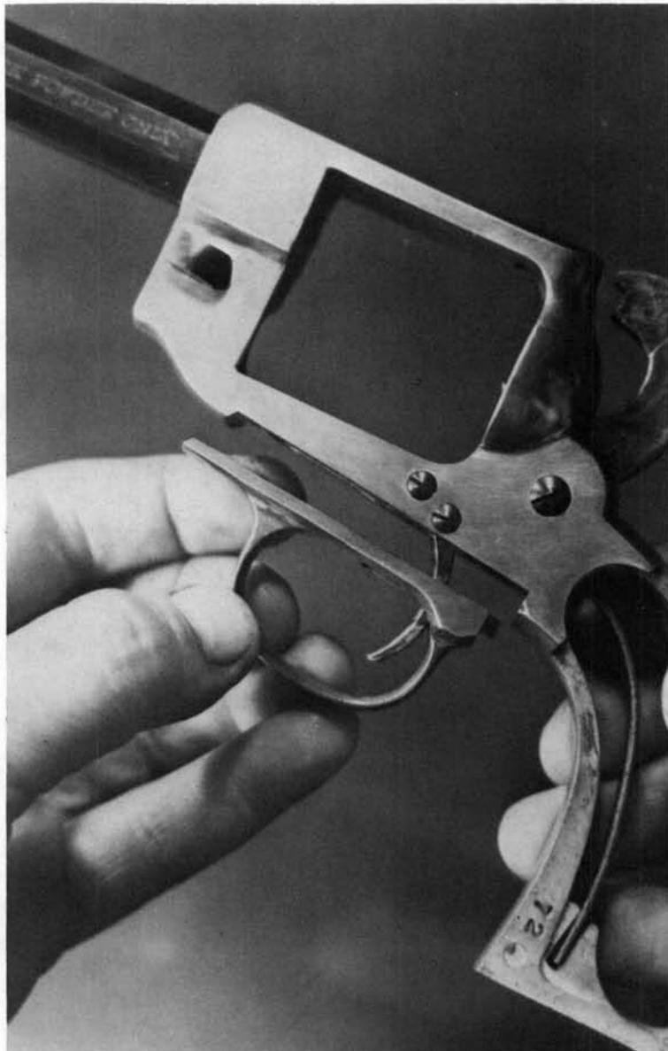
**9.** Remove the large screw at the front of the frame recess, and take out the combination trigger and cylinder stop spring.
