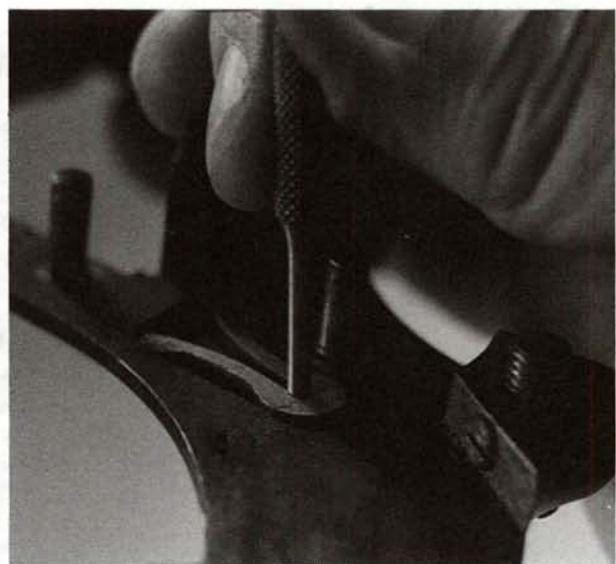
**12.** Use a drift of the proper size to tip the rear end of the cylinder latch spring slightly outward.
