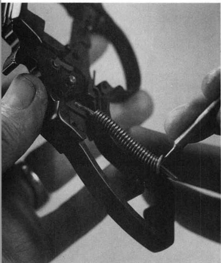
**17.** Remove the hammer spring assembly toward the right. If separation of the parts is necessary, wrap the unit in a heavy shop cloth and withdraw the drift.
