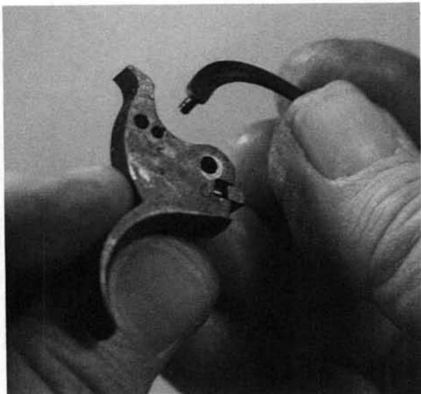
2. Be sure the forward extension of the rebound lever properly engages its shelf on the inside of the cylinder hand.
