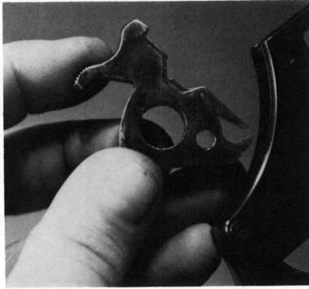
**11.** Pull the trigger to the rear and lift the hammer straight up out of the frame. Removal of the cross-pin at the front of the hammer will release the double-action lever and its plunger and spring.
