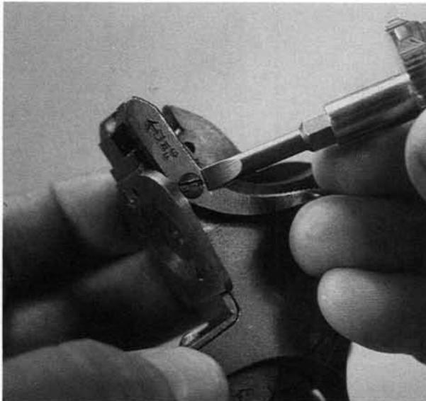
**15.** Move the latch to the rear, and take it off upward.
