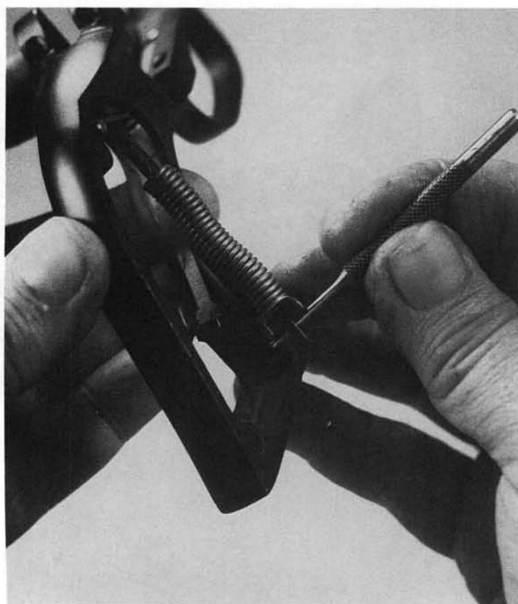
**11.** Remove the cylinder stop plunger and spring from the top of the grip frame.
