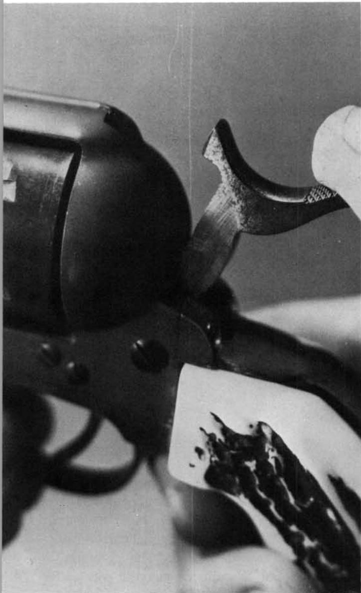
2. Depress the cylinder base pin latch and remove the base pin toward the front.
