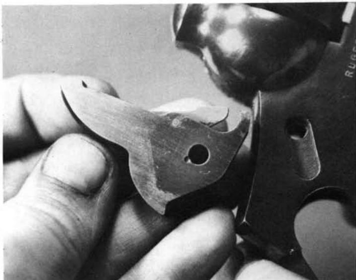
**7.** Pull the trigger to the rear, and remove the hammer from the top of the frame. Pushing out the cross-pin at the front of the hammer will release the double-action lever and its plunger and spring for removal.
