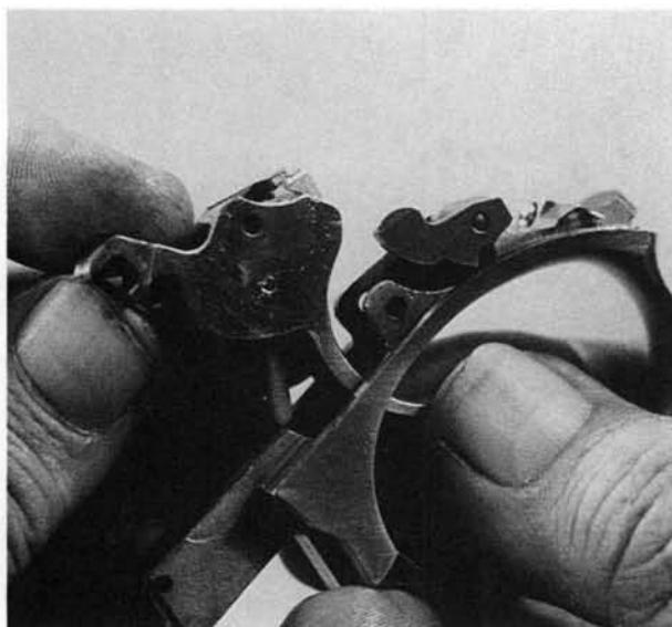
**19.** Remove the trigger upward and toward the rear.
