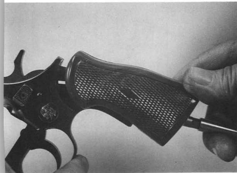
**11.** Drift out the cross-pin at the front of the guard.
