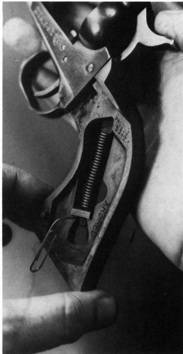
**5.** Remove the two screws at the upper rear of the grip frame, then the three screws in the underside of the grip frame, taking the forward screw out first. Move the grip frame slightly toward the rear, then remove it downward.
