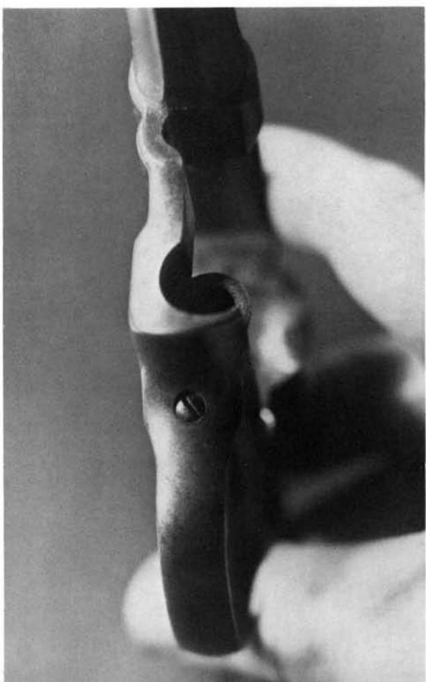
**18.** Remove the cylinder stop spring and its plunger.
