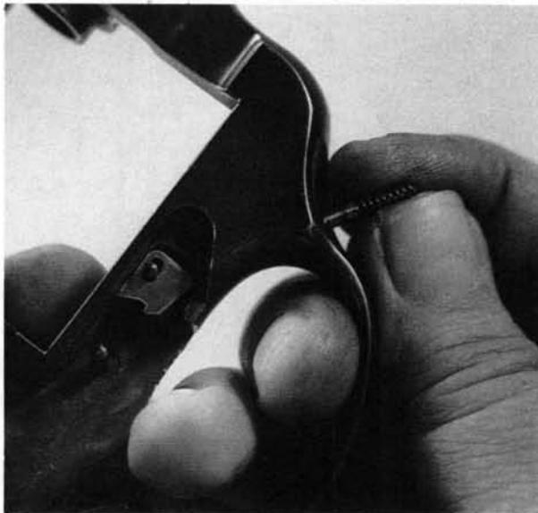
**20.** Move the cylinder stop to its rearmost position on the post, tilt it downward, and remove it toward the right.
