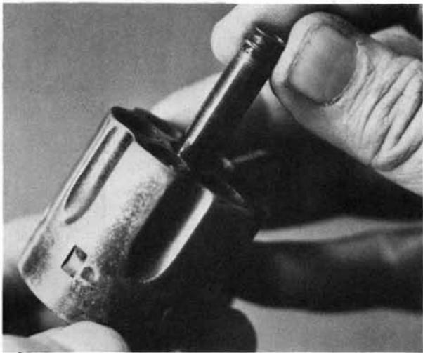
3. Remove the bushing from the front of the cylinder.
