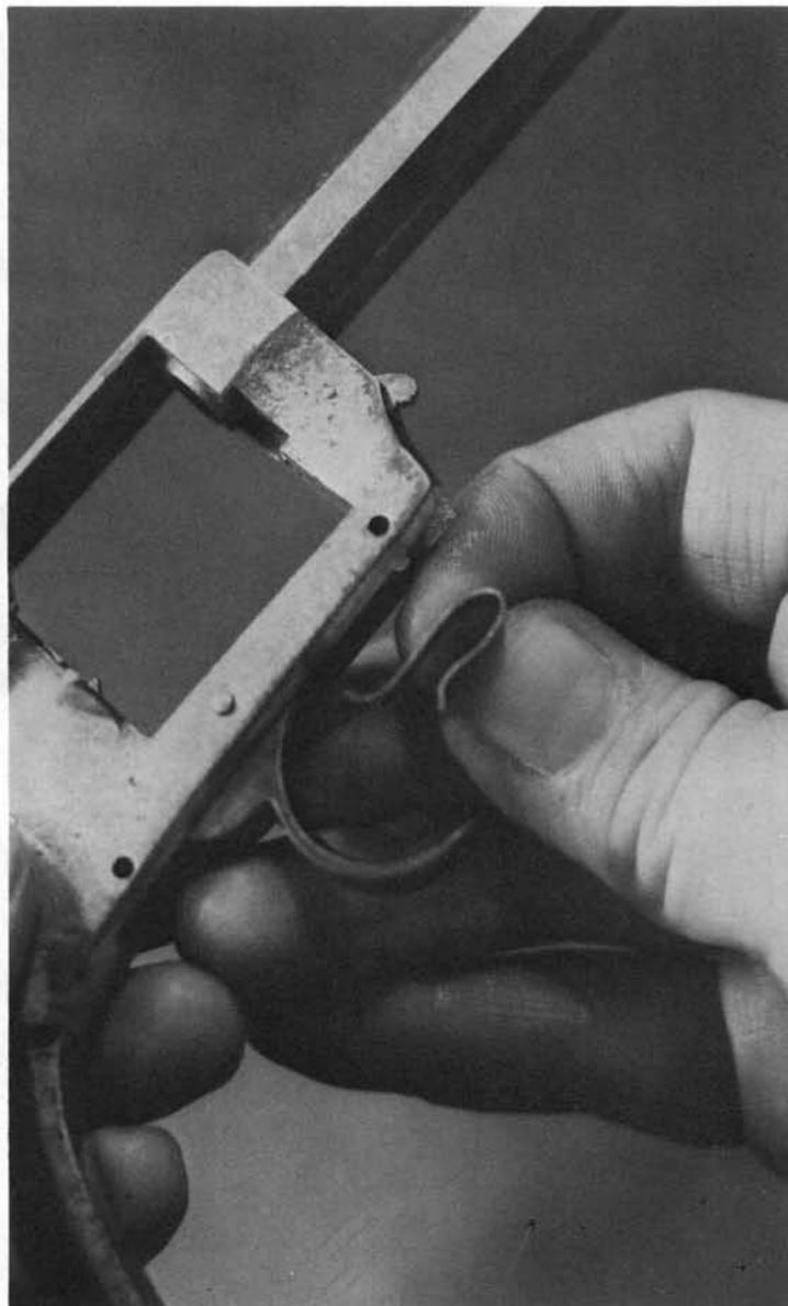
5. Drift out the cross-pin holding the trigger, and remove the trigger downward, along with the cylinder hand.
