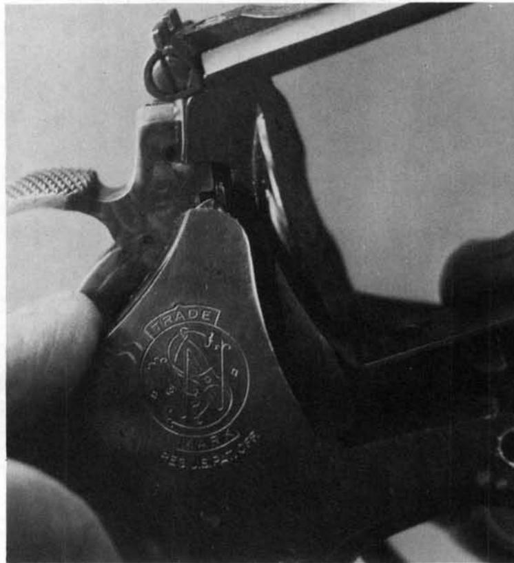
**2.** When replacing the sideplate, place the hammer block on its stud on the rebound slide, and move it to its upper position (see photo #10). Align the upper edge of the sideplate so the track on the inside of the plate encloses the top of the hammer block, then insert the upper lip of the plate and move the lower portion into place.
