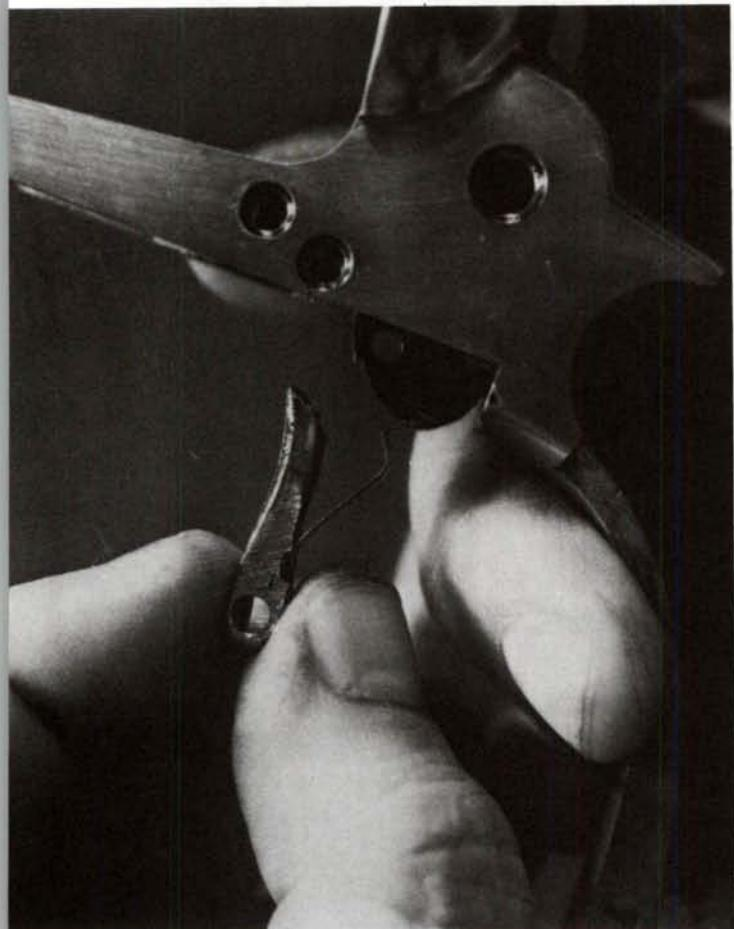
**15.** Remove the hammer from the top of the frame.
