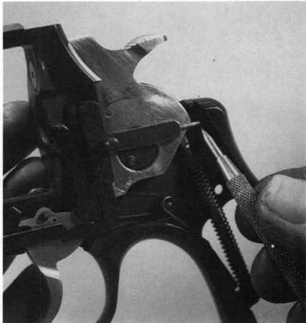
**5.** Place the latch bar in the sideplate recess, without its button installed, and push it fully to the rear, compressing the plunger and spring. Hold it in this position while the sideplate is moved very carefully back into place.
