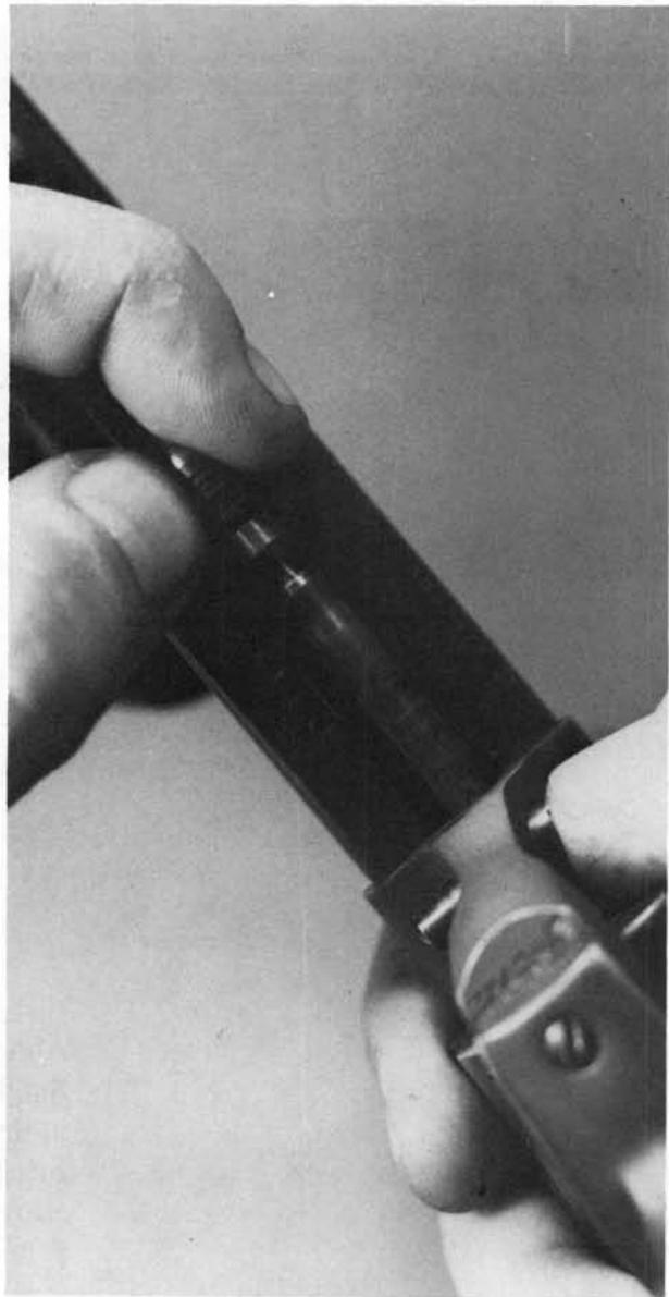
**3.** Open the loading gate and remove the cylinder toward the right.
