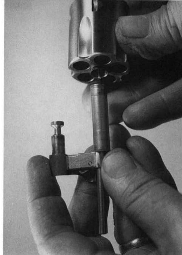
**23.** Remove the crane from the cylinder
