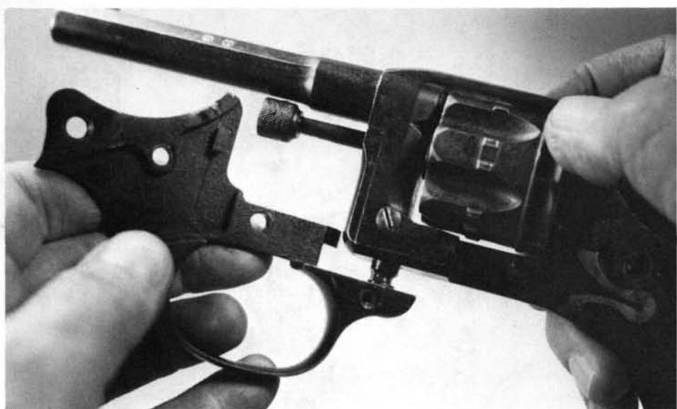
9. Remove the cross-screw at the front of the frame.
