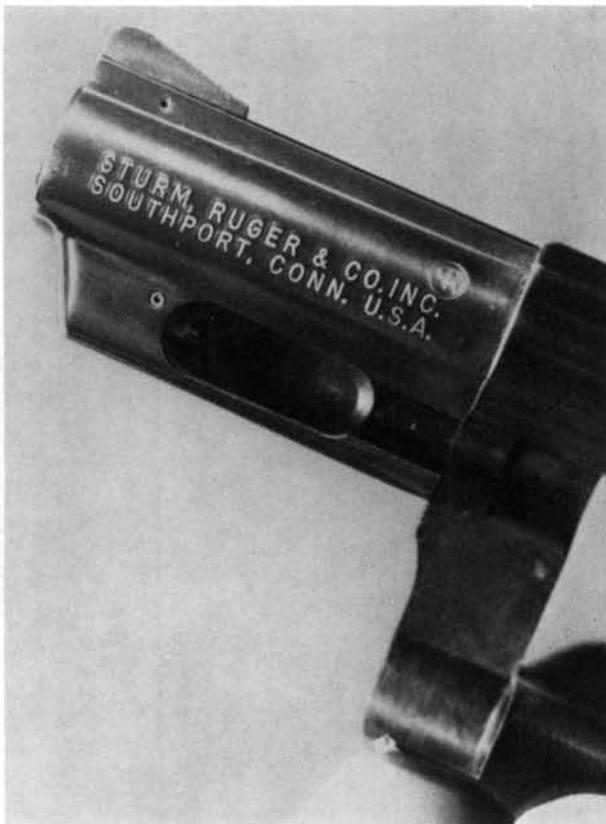
**30.** The firing pin housing, firing pin, and spring are removed toward the front after the cross-pin is drifted out. This cross-pin, near the top of the frame, has ends that are contoured with the sides of the frame, and removal and replacement will usually cause some damage to the ends. In normal disassembly, this system is best left in place.
