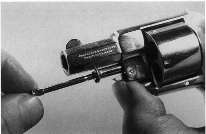
2. Depress the latch farther, and remove the cylinder base pin.
