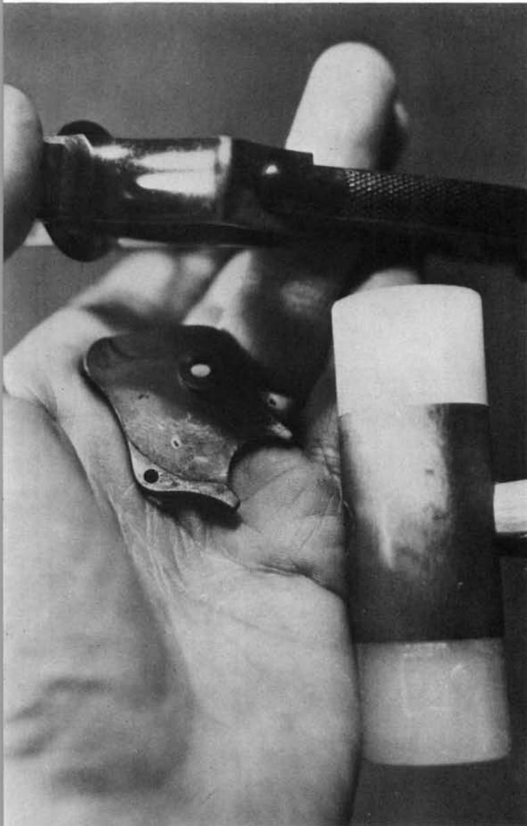
**13.** Remove the cross-pin at the top of the frame, just below the barrel latch posts, and cover the breech face with a shop cloth to arrest the firing pin in case it comes out freely. Pull the trigger several times to drop the hammer, and the firing pin impact will move the firing pin housing out of its well in the breech face. If it doesn't come all the way out, it will be extruded enough for easy removal.
