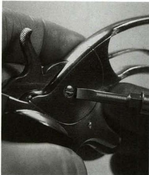
**5.** Hold the gun as shown, and tap the grip frame lightly with a non-marring mallet until the sideplate falls into the hand.
