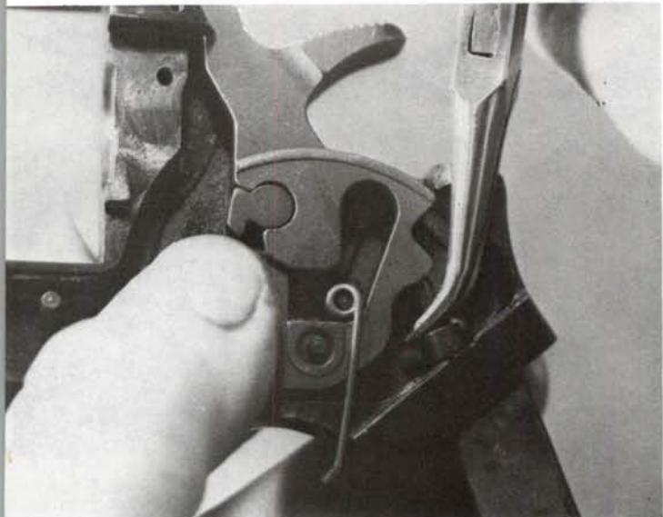
2. When replacing the cylinder hand, be sure the angled tip of the hand spring is engaged in the groove at the back of the hand, then move the hand downward and toward the right, onto its post on the trigger.
