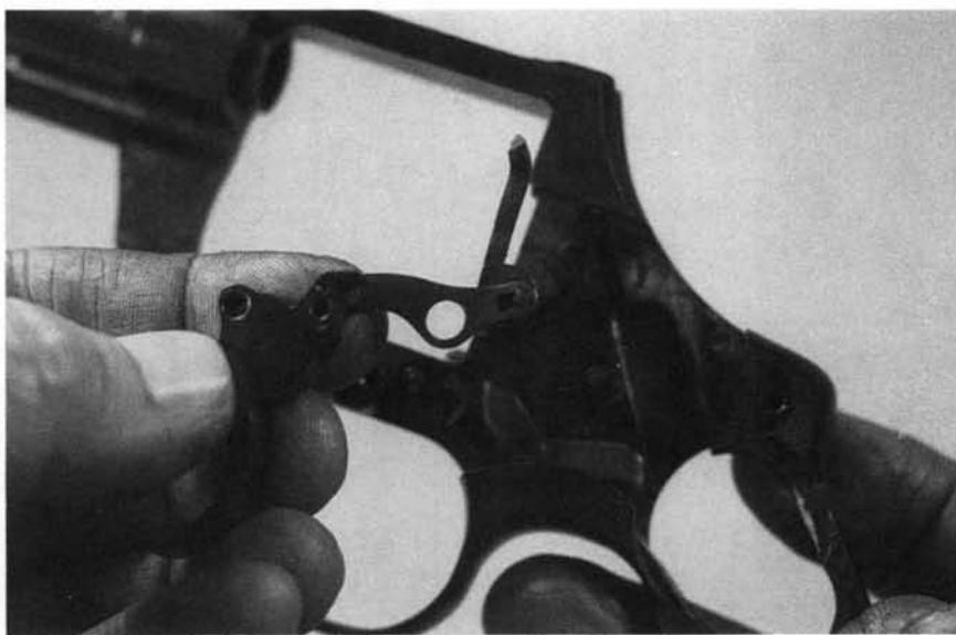
**15.** Remove the trigger and its attached hammer block safety system toward the left. The parts of the safety system may detach as the trigger is taken out.
