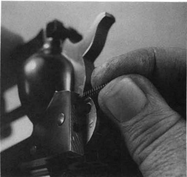
6. Remember to put the hammer spring unit in the grip frame before it is reinstalled. Note that the unit must be oriented as shown.
