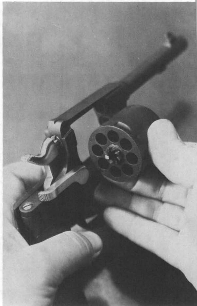
5. Exert forward pressure on the rear of the trigger guard and pull it downward. Pivot it forward until it stops against the frame.
