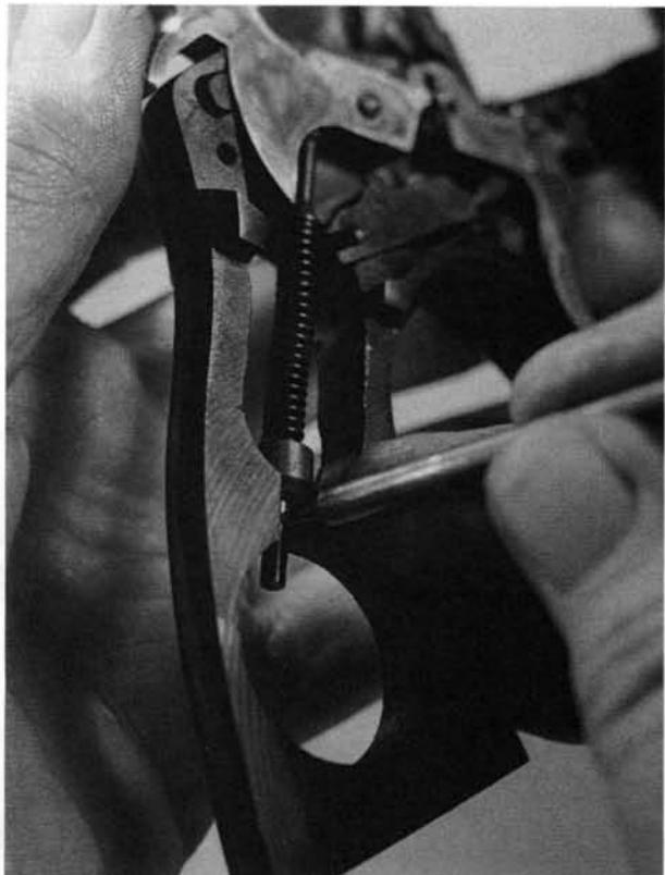
**13.** Pull the trigger and ease the hammer down. Take out the hammer spring assembly. If this is to be disassembled, use caution and control the compressed spring.
