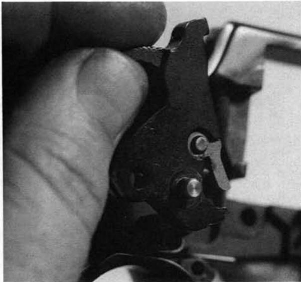
**19.** The pivot is easily removed from the hammer, toward either side.
