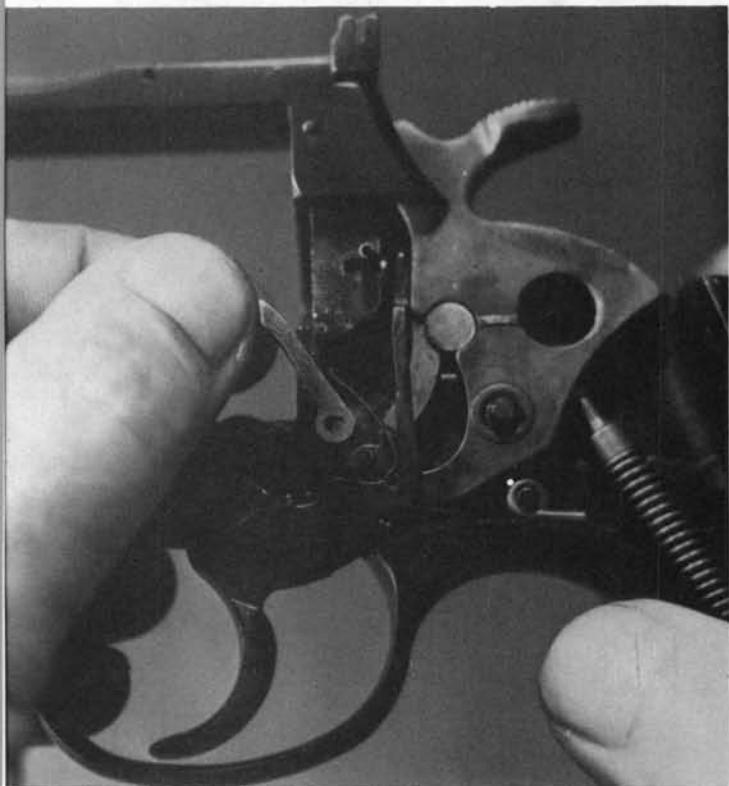
**10.** Remove the cylinder hand from its stud on the trigger.
