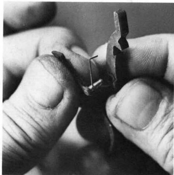
**17.** Remove the safety lifter upward.
