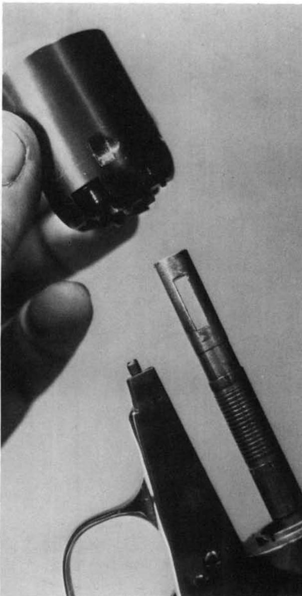
6. Taking out the screw above the barrel wedge will allow removal of the wedge toward the left. Backing out the cross-screw below the barrel will release the loading lever assembly for removal. Removal of the screw in the lever allows separation of the lever and rammer.
