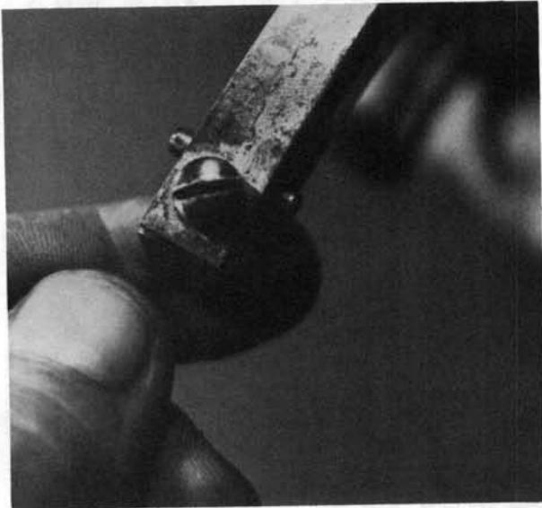
7. Remove the screw retaining the combination trigger and cylinder stop spring, and take out the spring.
