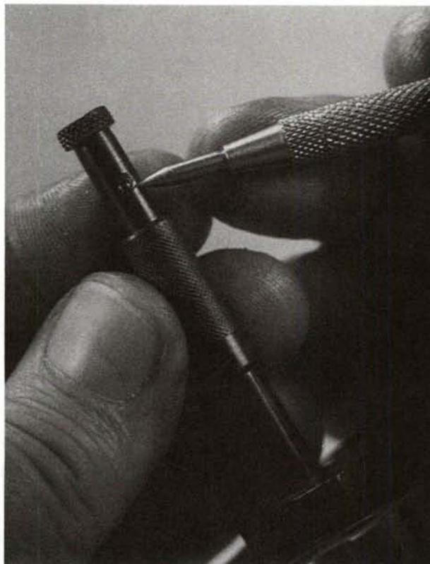
3. Support the ejector rod knob on a non-marring surface, and drift out the knob cross-pin.
