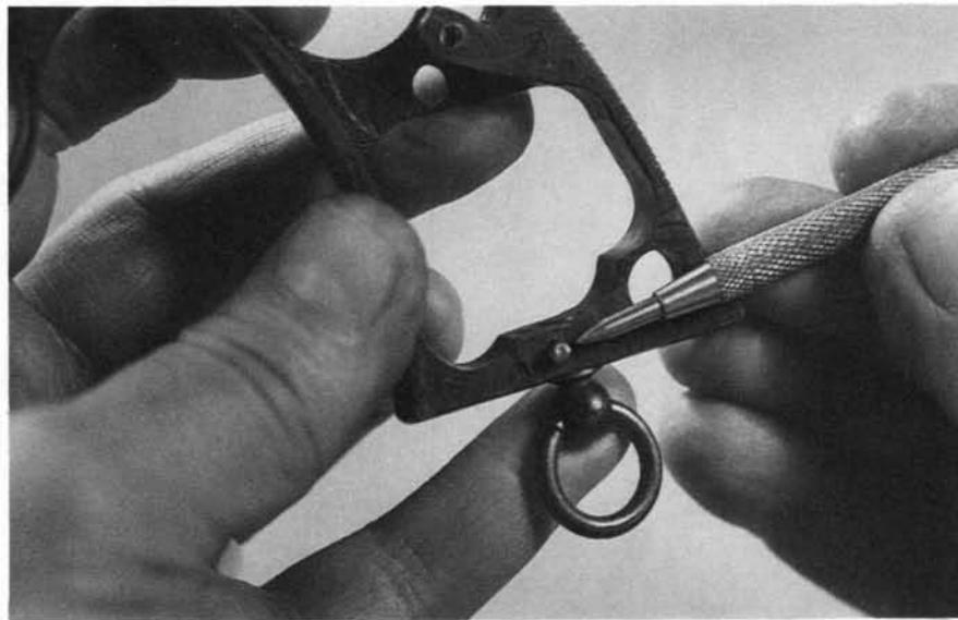
**28.** The lanyard ring is retained on the frame by a cross-pin which also stabilizes the grip panels. Drifting out the cross-pin will release the post and ring for removal downward.
