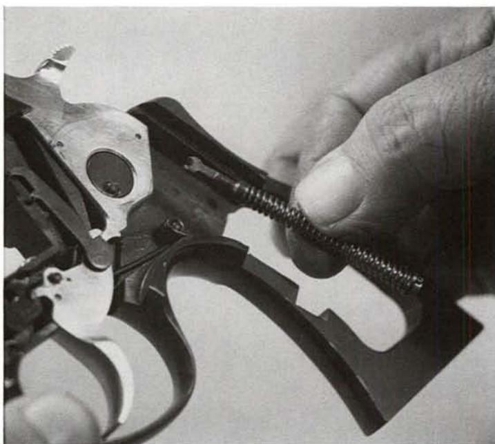
**21.** Remove the hammer spring assembly downward. This unit can be disassembled by drifting out the small roll pin at its lower end, but in normal takedown it is best left intact.
