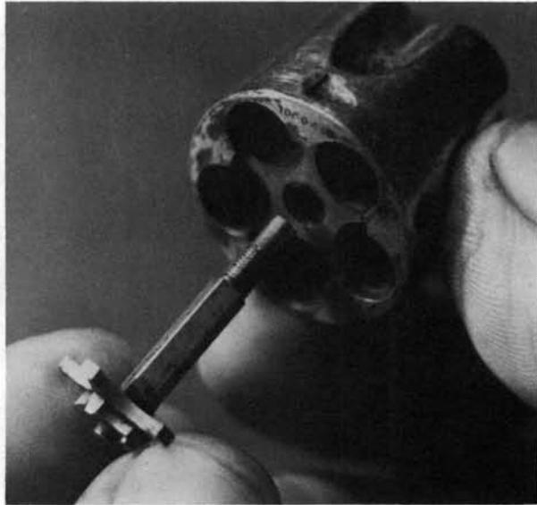
**5.** Remove the barrel hinge cap screw from the left side of the frame.
