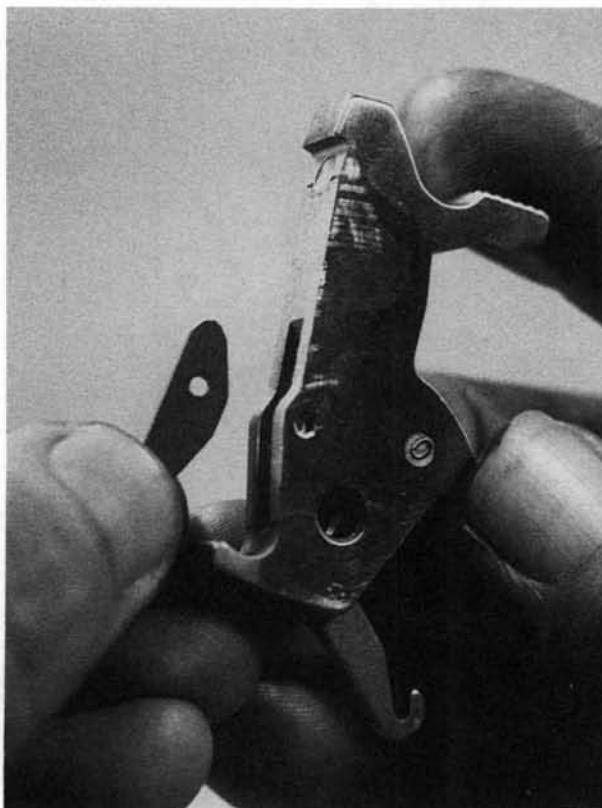
**8.** Push out the mainspring lever pivot pin toward either side.
