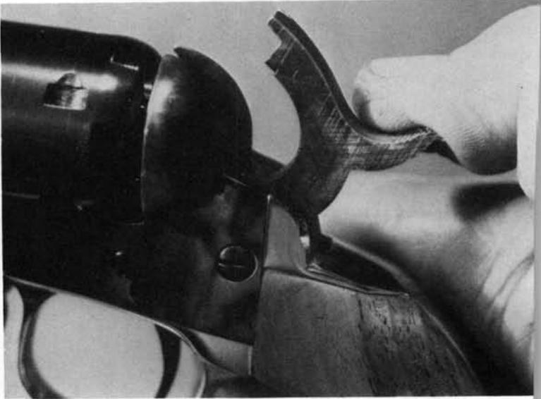
4. Set the hammer on the loading step, the middle notch, to free the cylinder.
