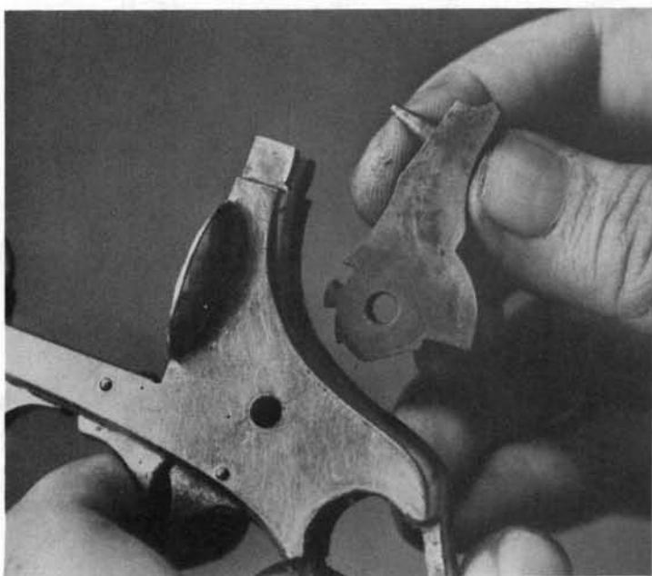
**13.** The hammer is retained by a cross-screw, and the trigger and guard are held in place by cross-pins. Take out the hammer screw, pull the trigger to the rear, and remove the hammer from the top of the frame. It may be necessary to insert a small tool downward, in front of the hammer, to disengage the lifter from its recess.
