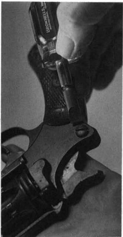
2. Open the sideplate, and move the left grip upward and outward for removal.
