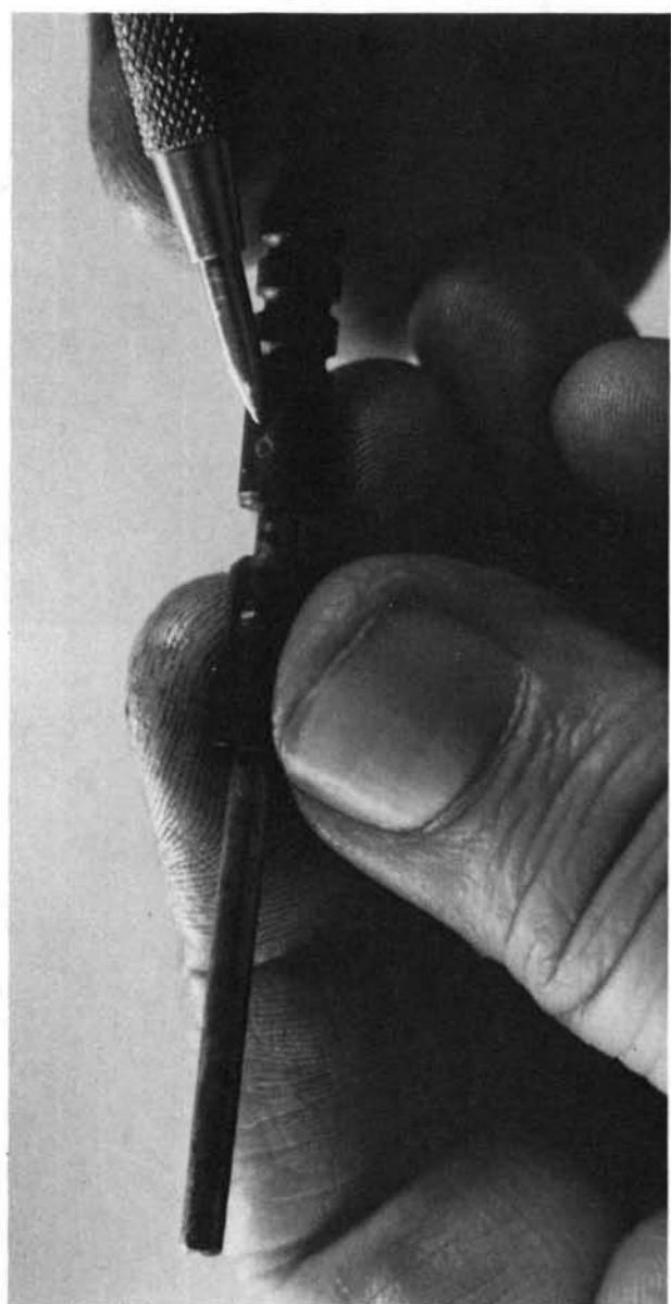
**6.** The knob is mounted on the rod with a blind pin, and the only way to remove it would be to drill it out. Because of this, the sleeve and its spring are not routinely removable from the rod.
