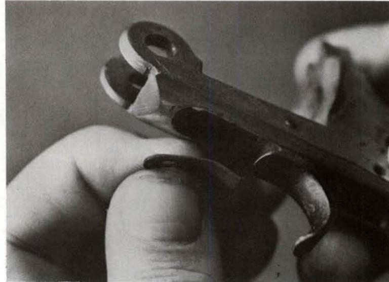
**15.** Drift out the trigger pivot pin and remove the trigger assembly downward.
