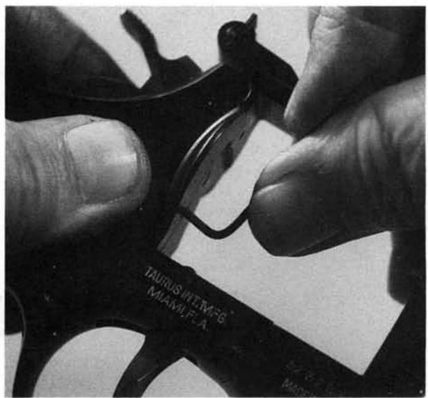
**4.** A small Allen wrench is perfect for keeping the cylinder hand plunger and spring depressed as the sideplate is moved back into place. With the short arm of the wrench, fully depress the plunger and hold it in that position while the sideplate is pushed in as far as possible. The wrench is then withdrawn, as shown here, allowing the plunger to engage the back of the cylinder hand. It is a fairly tricky operation.
