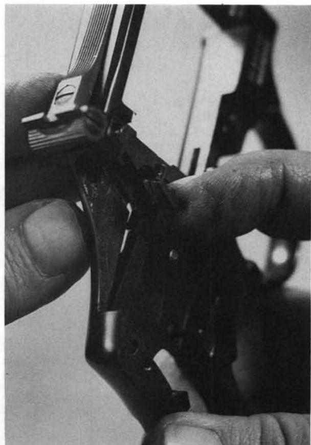
**24.** Move the cylinder latch assembly all the way to the rear, tip it outward at the front, and remove it. Take care that the small plunger and spring at its rear are not lost.
