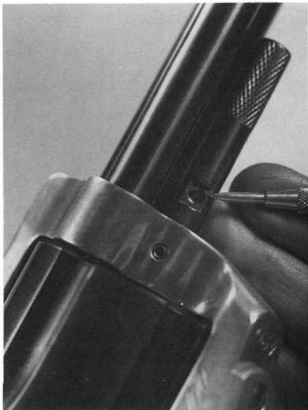
When replacing the grip frame, remember to first insert the hammer spring assembly, and be sure that all of the springs bear on their respective parts.
