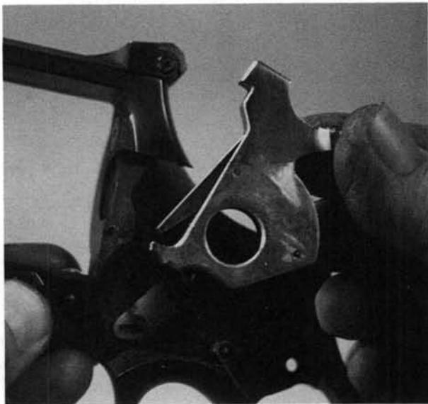
**26.** Remove the hammer pivot cam toward the left.
