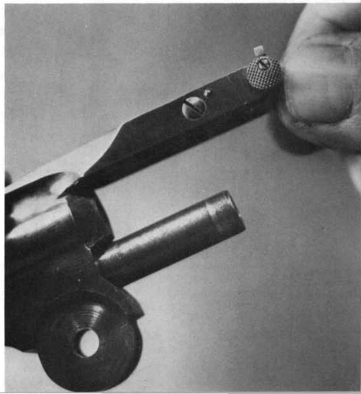
**7.** The cylinder latch is retained by a small vertical screw in the inner ledge of the right barrel hinge recess. When the latch is removed, take care not to lose the tiny spring and screw.
