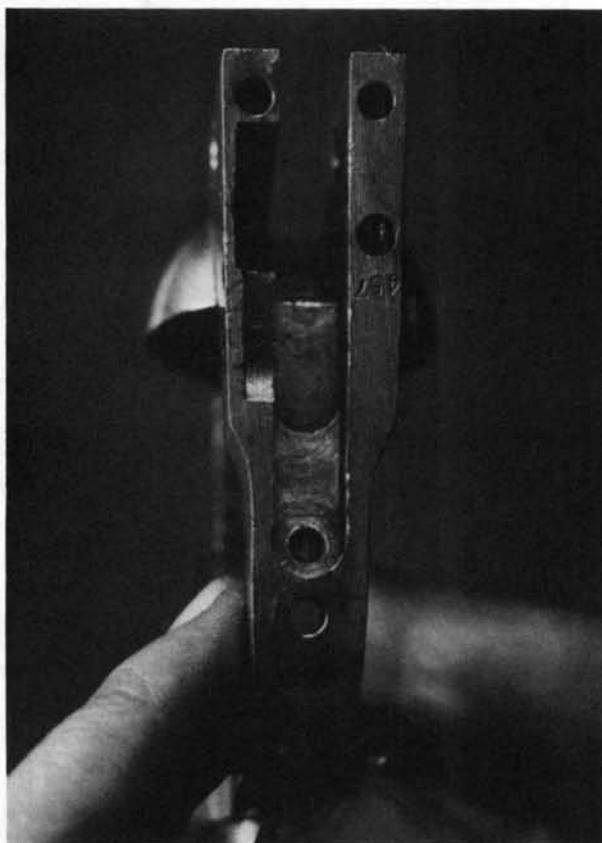
**17.** After the screw is taken out, remove the spring and plunger.
