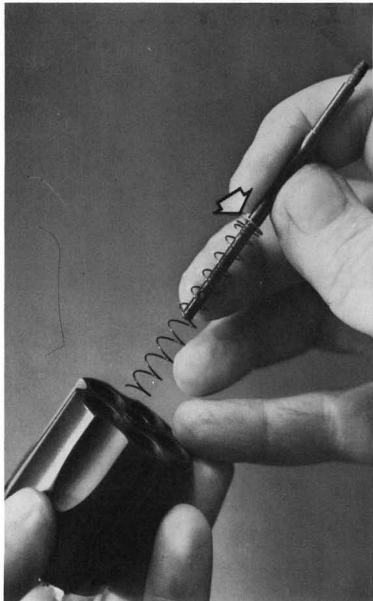
**7.** Remove the ejector/ratchet piece from the rear of the cylinder.
