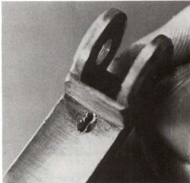
**12.** Drift out the cross-pin at the rear of the trigger guard and remove the trigger guard downward.
