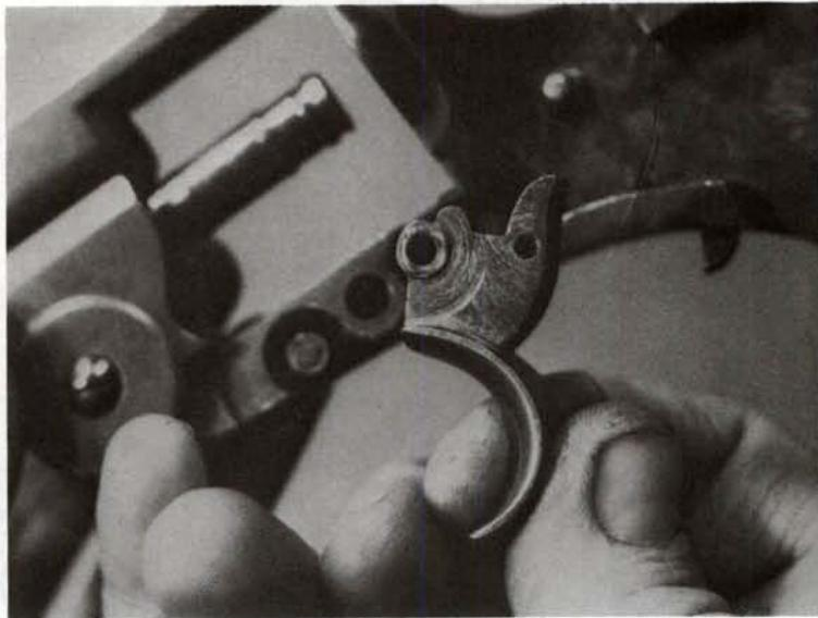
**16.** Backing out the vertical screw at the upper rear of the frame will allow removal of the sideplate.
