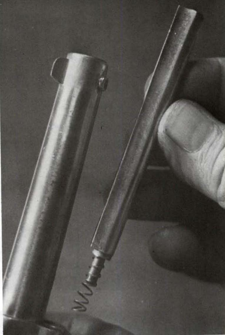
**20.** A screw near its muzzle end retains the ejector rod housing. After taking out the screw, tip the front end of the housing away from the barrel to clear the screw stud. Remove the housing toward the front. The rod and spring are easily removed by sliding them out the rear of the housing.
