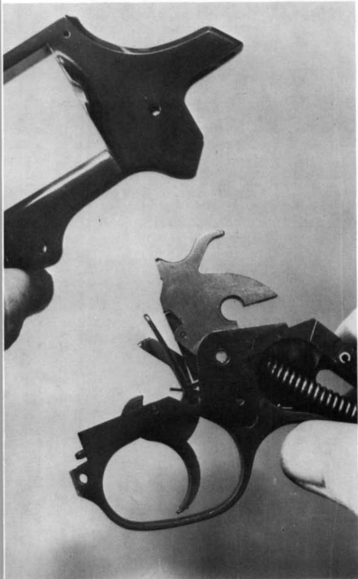
**12.** Remove the hammer block bar from the left side of the trigger.
