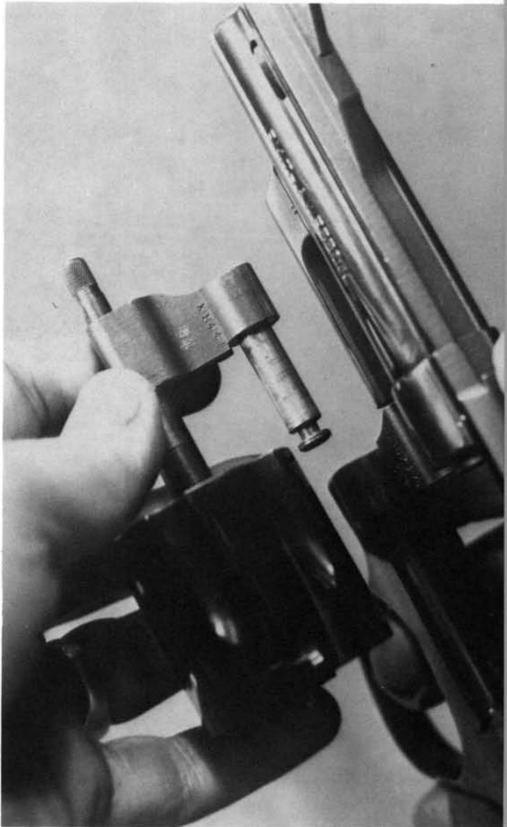
3. Remove the crane from the front of the cylinder. Grip the head of the ejector rod with leather-padded smooth-jawed pliers, and unscrew it *clockwise* (front view). Note that this is a reverse thread. If the rod is very tight, clamp the head of the rod in a padded vise, insert empty cartridge cases in two opposed chambers, and turn the cylinder to free the rod.
