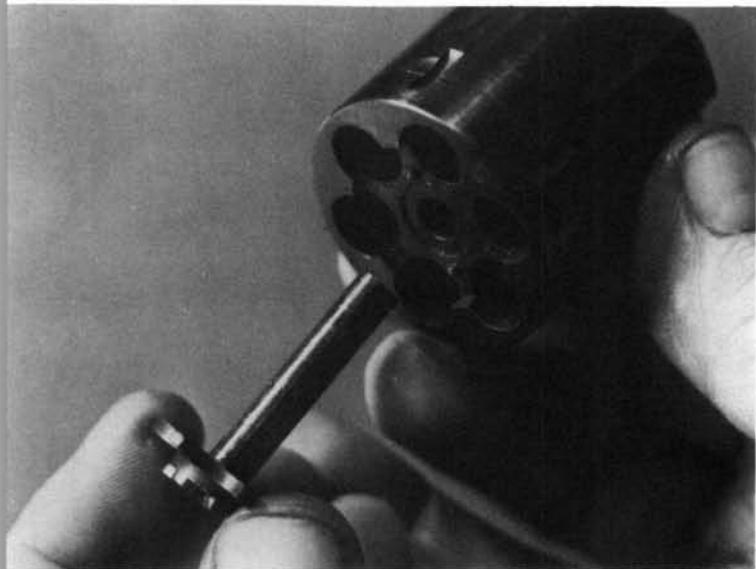
**24.** Use the front tip of the center pin to push the cylinder lock pin out of the front of the ejector.
