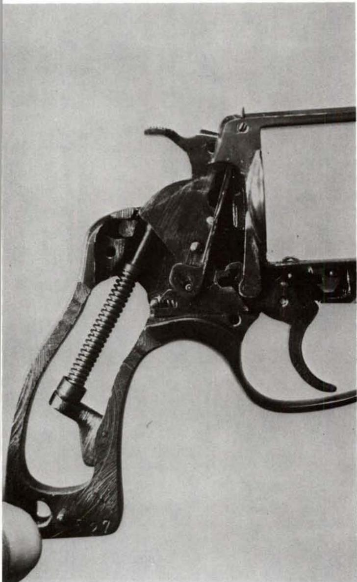
**10.** Grip the upper neck of the hammer strut with smooth-jawed sharp-nosed pliers, and move it slightly downward against the tension of the hammer spring, then ease it out toward the right and upward for removal.
