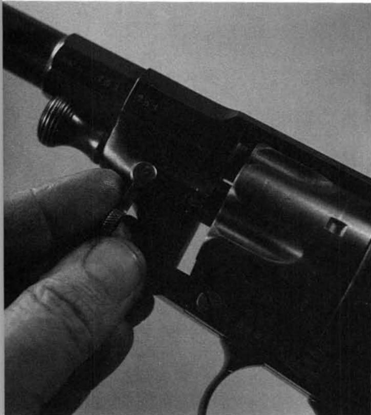
2. Remove the cylinder base pin toward the front.
