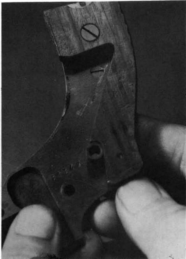
**17.** The larger screw on the frame sideplate retains a wood filler block, the smaller screw holds the left grip.
