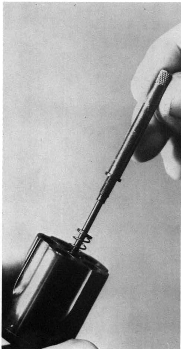
**5.** Remove the cylinder lock pin from the front of the cylinder, along with its spring.
