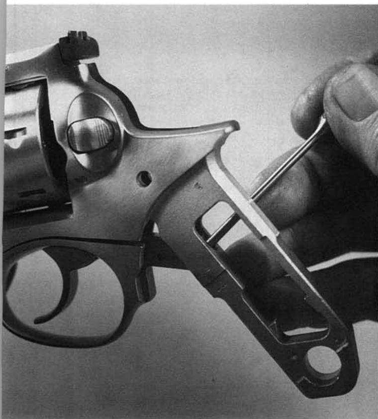
**11.** Use a tool to depress the trigger guard latch, and move the rear of the guard downward.
