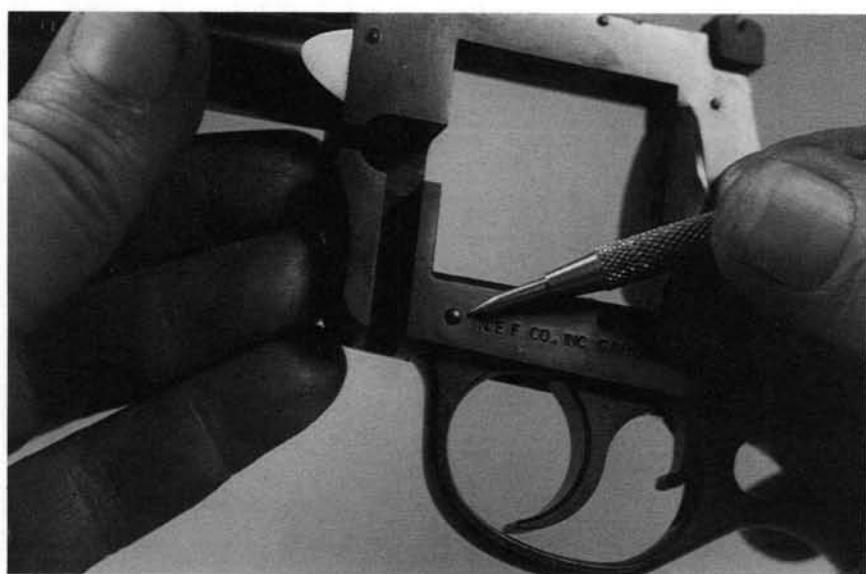
**12.** Drift out the forward trigger guard cross-pin.
