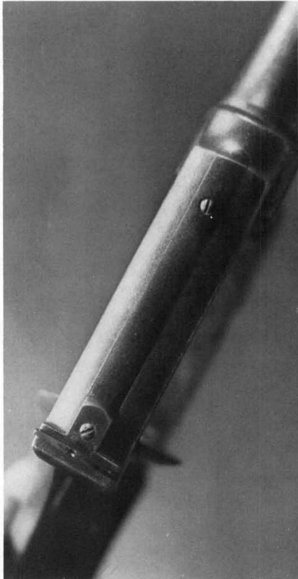
**27.** The front sight blade is retained by a cross-pin.
