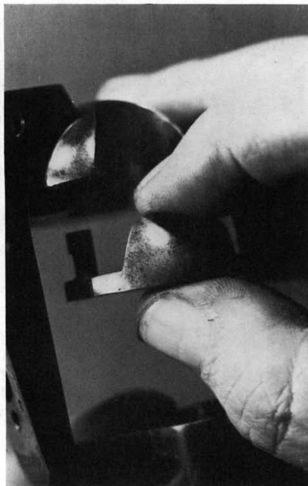
**16.** The loading gate can now be moved forward out of the frame.
