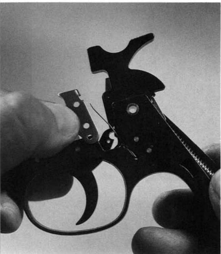
**20.** Cock the hammer, and insert a small drift punch or the end of an opened paper clip through the hole in the hammer spring strut.
