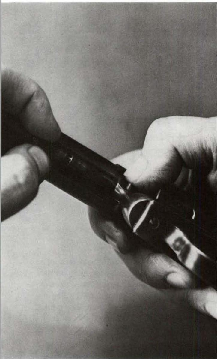
2. Open the loading gate and remove the cylinder toward the right.
