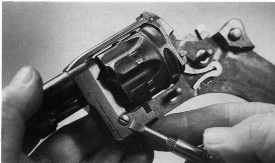
**10.** Operate the cylinder release, and move the crane to the half-open position. Move the crane and cylinder forward out of the frame, turning the crane to the fully-opened position after its detents have cleared the positioning spring.
