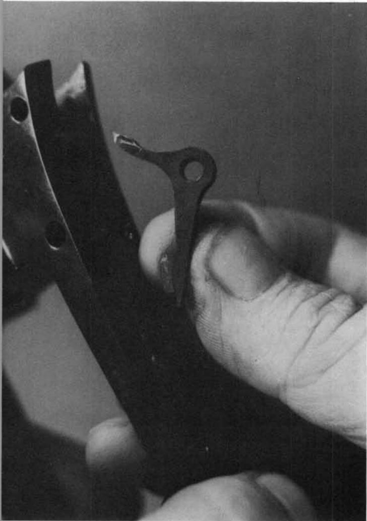
**14.** Remove the cylinder hand from the left side of the hammer.
