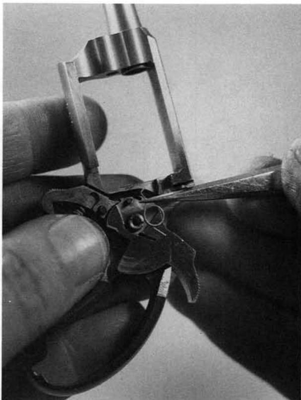
**10.** Depress the trigger, and remove the hammer toward the left.
