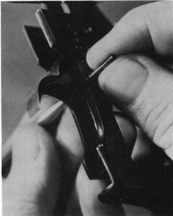
**16.** Remove the trigger assembly from the bottom of the frame. The cylinder hand and the transfer bar are easily removed from each side of the trigger.
