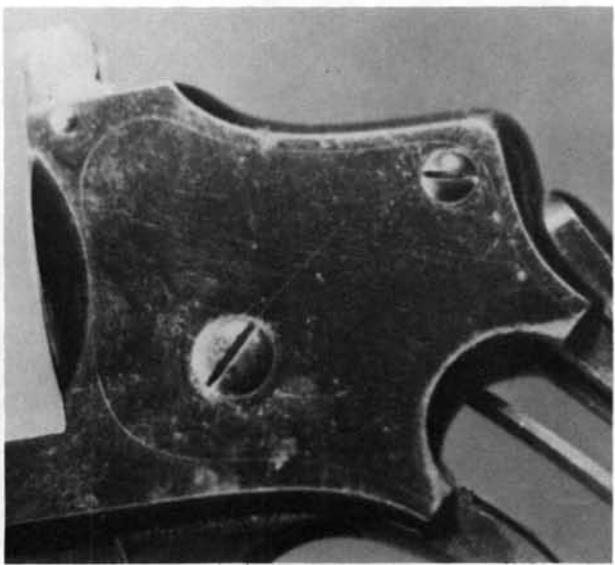
**11.** Remove the large and small screws that retain the sideplate. The large screw is actually an internally threaded cap nut.
