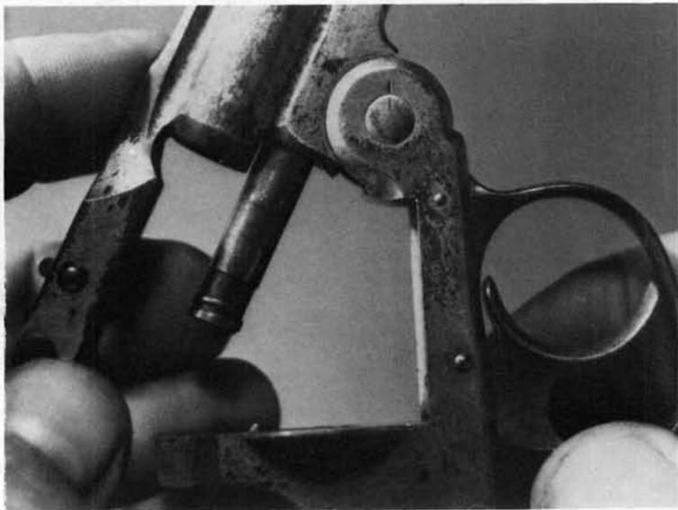
4. When installing the barrel hinge, note that the head of the hinge has a mark which must be aligned with a corresponding mark on the frame loop. This insures that the side lug on the hinge will enter its recess in the frame.
