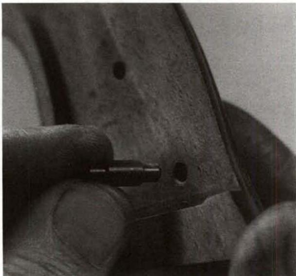
**14.** Remove the rear sideplate screw. It may be necessary to grip the smooth nut on the opposite side as the screw is removed. Take off the nut toward the right.
