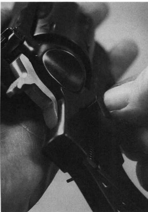
3. Pull the trigger and ease the hammer down. Push out the hammer pivot, and remove it toward the right.
