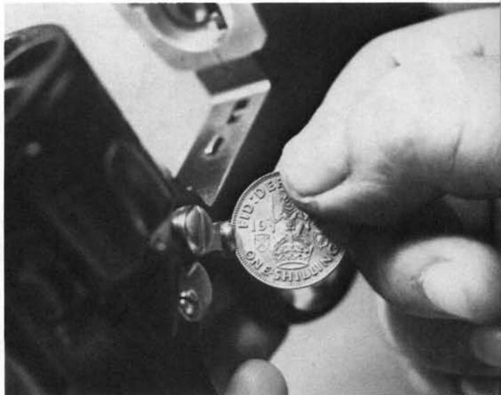
**3.** After removal of the screw, turn the lever upward until its short arm bears on the cylinder retainer and tips it downward. The cylinder can then be taken out toward the rear.
