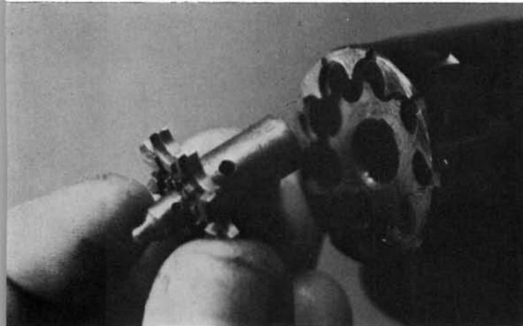
**8.** Remove the cylinder lock plunger and its spring from the center of the ejector/ratchet.
