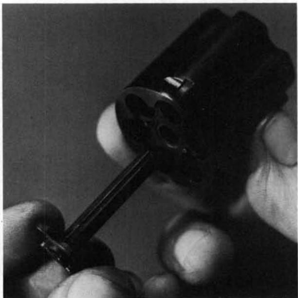
**9.** Remove the two remaining sideplate screws, hold the gun as shown, and tap the grip frame with a nylon mallet until the sideplate falls into the palm of the hand.
