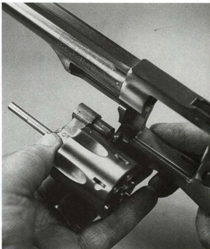
**25.** Operate the cylinder latch, open the cylinder, and remove the cylinder and crane assembly toward the front.
