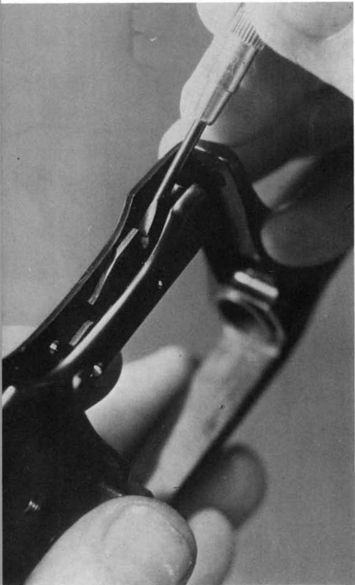
**23.** Move the cylinder stop inward, off its post, and remove it from the frame. Take care to release the plunger and compressed spring slowly. If it escapes, it can travel quite a distance.
