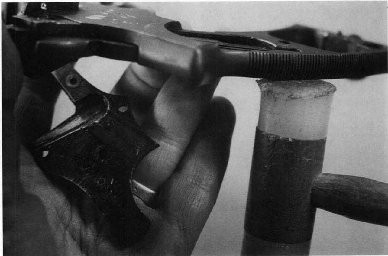
**19.** Slightly compress the main-spring, unhook it from the stirrup, and remove it. **Caution:** Control the spring.
