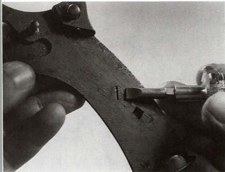
**17.** If removal of the lanyard ring is necessary, the grip stabilizer is pushed or driven toward the right until its internal opening aligns with the lanyard ring post. The post and ring are then taken off downward.
