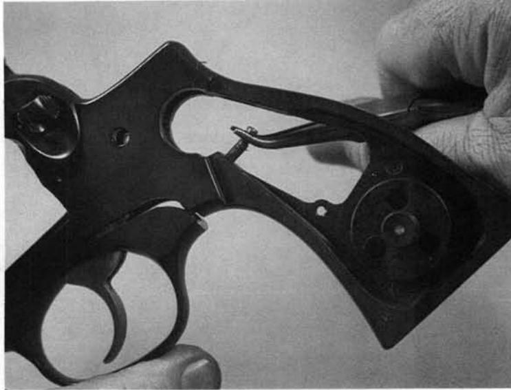
**6.** When the guard unit is in place, pull the trigger a few times (it must be returned manually) to be sure the cylinder is rotating and locking properly.
