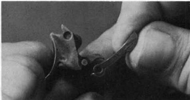
7. Remove the cylinder base pin latch spring from its hole in the forward underside of the frame. Drifting out the cross-pin that retains the latch will allow its removal toward the front.
