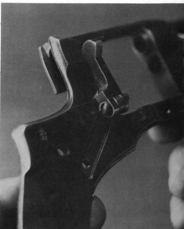
**20.** Remove the loading gate pivot screw, then remove the loading gate from its loop on the frame.
