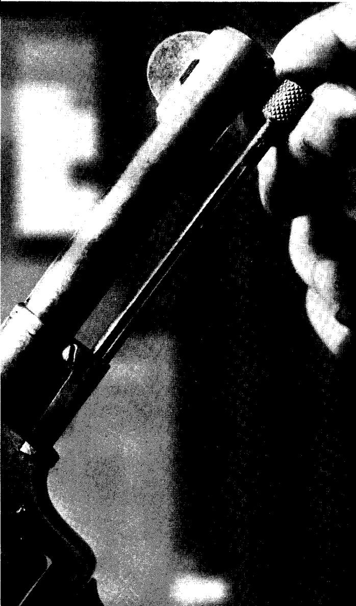
2. Turn the ejector housing from beneath the barrel toward the right side of the gun until the small groove on its right side aligns with a similar groove in the top of the barrel.
