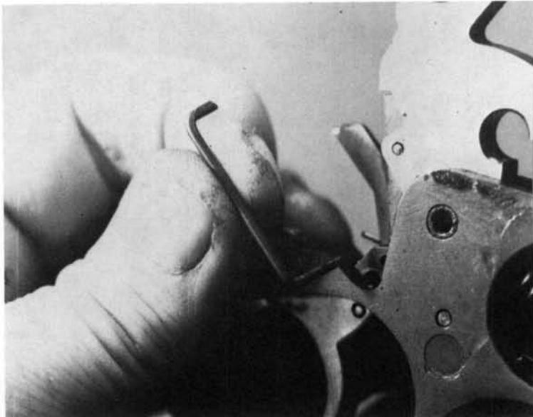
**13.** The lower right end of the hammer block bar also serves as the cylinder hand pivot. Disengage the arm of the hand spring from its shelf on the hand, and remove the cylinder hand toward the right.
