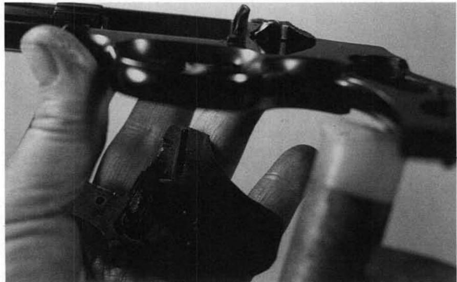
**9.** Hold the gun as shown, and tap the grip frame with a nylon hammer until the sideplate falls off into the hand.
