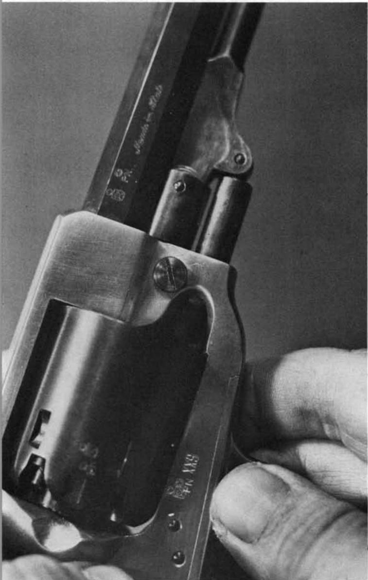
**5.** Remove the cylinder pin retainer toward the left.
