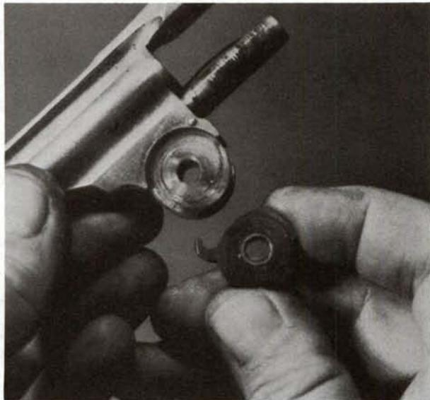
**8.** Remove the ejector cam trip from the front of the frame, and extract its small coil spring from the hole behind it.
