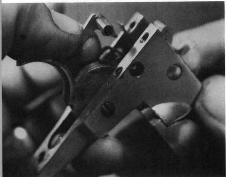
**11.** Remove the combination sear and cylinder stop spring from its recess in the frame.
