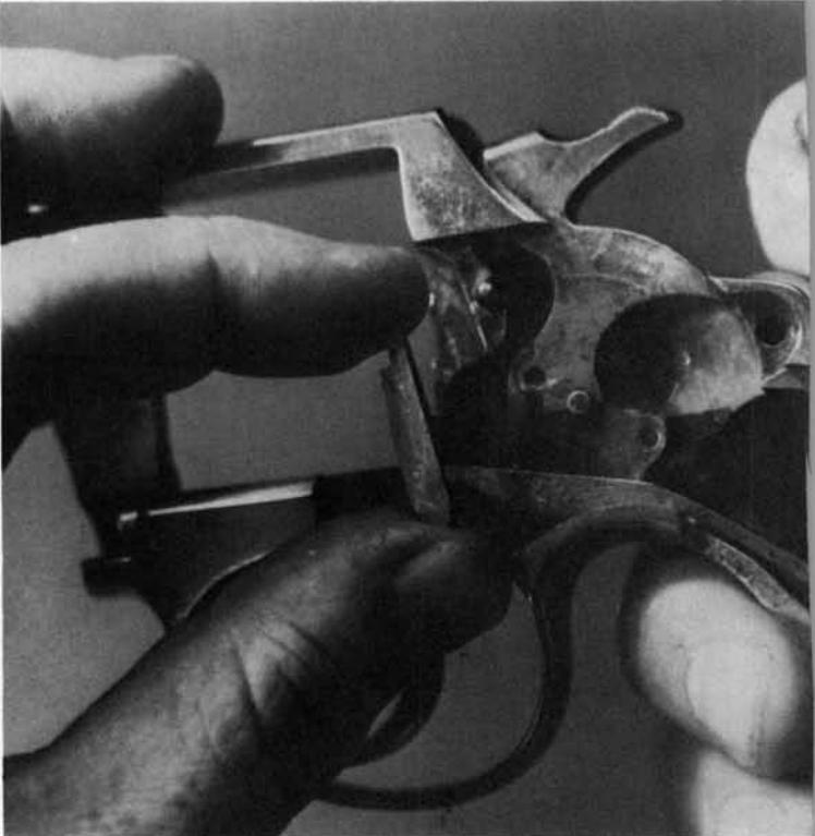
**15.** Drift out the rebound lever pin, located at the center of the grip frame. Move the rear loop of the rebound lever out of its recess in the grip frame, and remove the lever toward the left.
