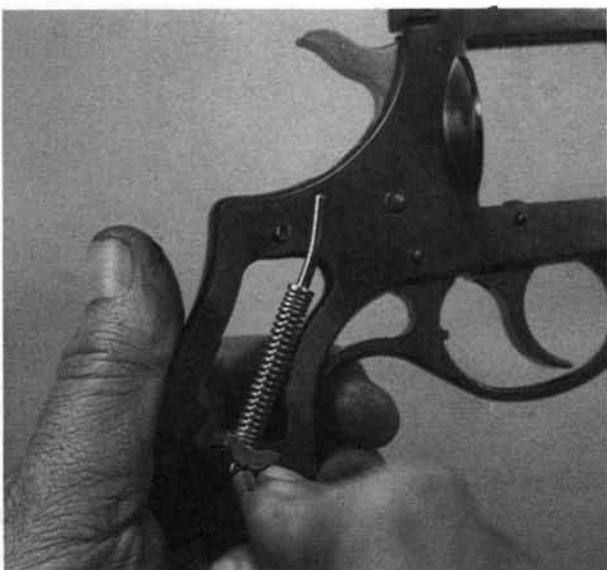
**6.** When installing the hammer spring unit, note that it is oriented with the bend at the top as shown.
