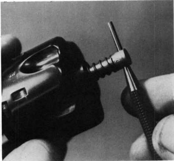
**5.** Remove the ejector rod head and the ejector spring toward the front. Then, remove the ejector/ratchet toward the rear.
