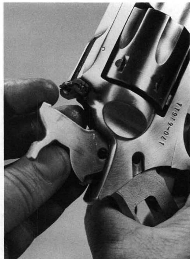
**9.** Pull the trigger, and remove the hammer upward.
