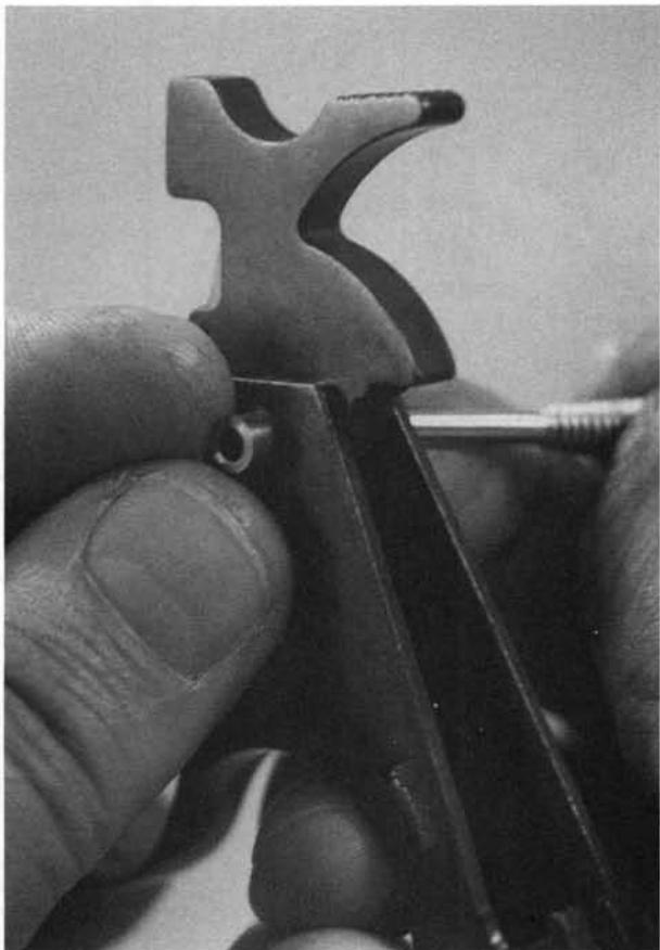
**23.** Pull the trigger, and remove the hammer from the sub-frame. Drifting out the cross-pin will free the double-action lever and its spring for removal. In normal takedown, they are best left in place.
