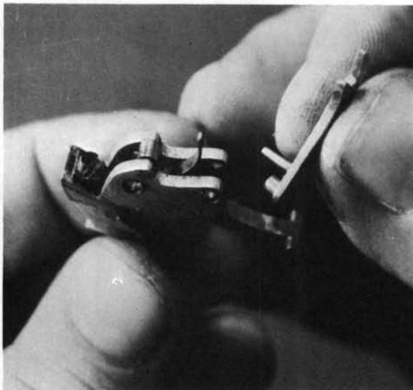
**15.** After the trigger is removed, the cylinder stop can be moved inward and out of its pivot-hole in the frame, then removed downward.
