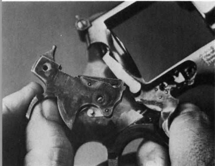
**14.** Use a small screwdriver to lift the rear of the rebound slide off its post, and ease out the spring. Remove the rebound slide assembly rearward and toward the right.
