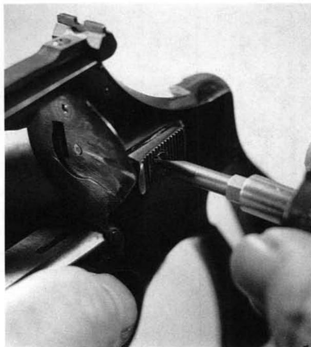
**21.** Remove the screw that retains the cylinder latch button. During removal of the screw, keep a fingertip on the latch bar inside, to prevent it from being forced outward. Remove the latch button toward the left.
