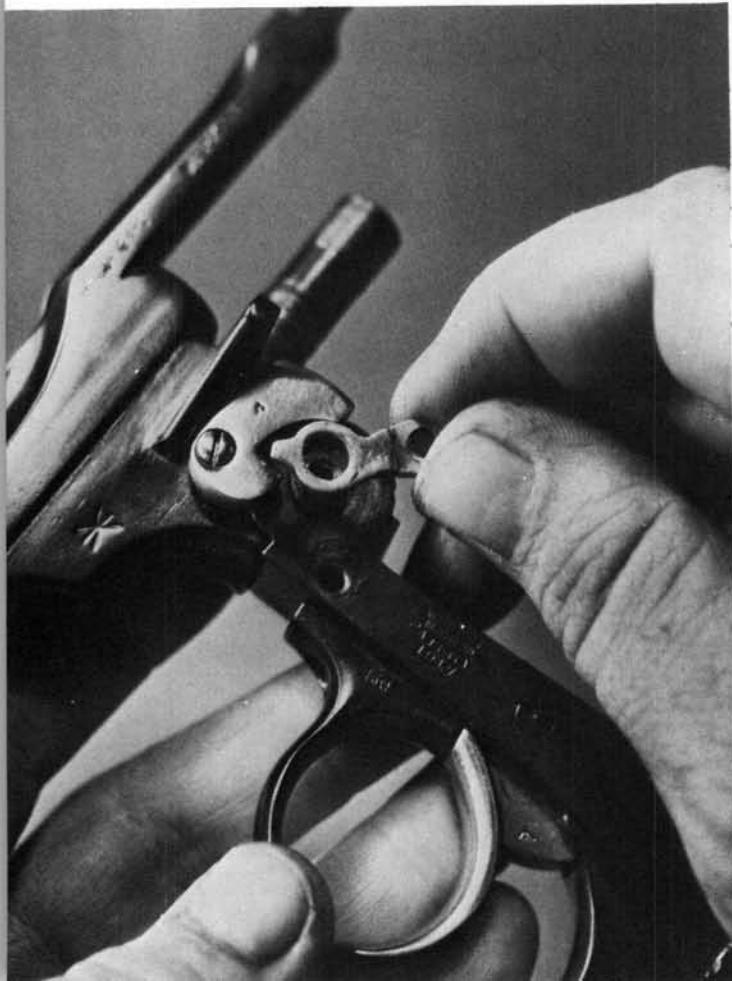
**6.** Remove the left cap screw and take off the cylinder release lever.
