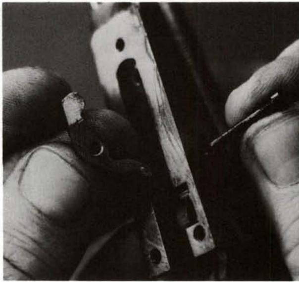
**16.** Take out the cylinder stop screw and remove the cylinder stop from the bottom of the frame.
