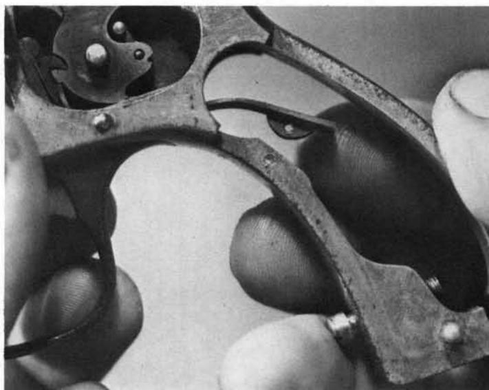
**14.** Pull the trigger to tip the hammer to the rear, and remove the hammer toward the left. Drifting out the small pin at the lower rear of the hammer will release the stirrup for removal.
