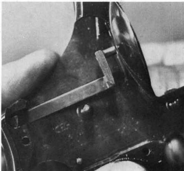
**22.** Remove the plunger and spring from the rear of the cylinder latch.
