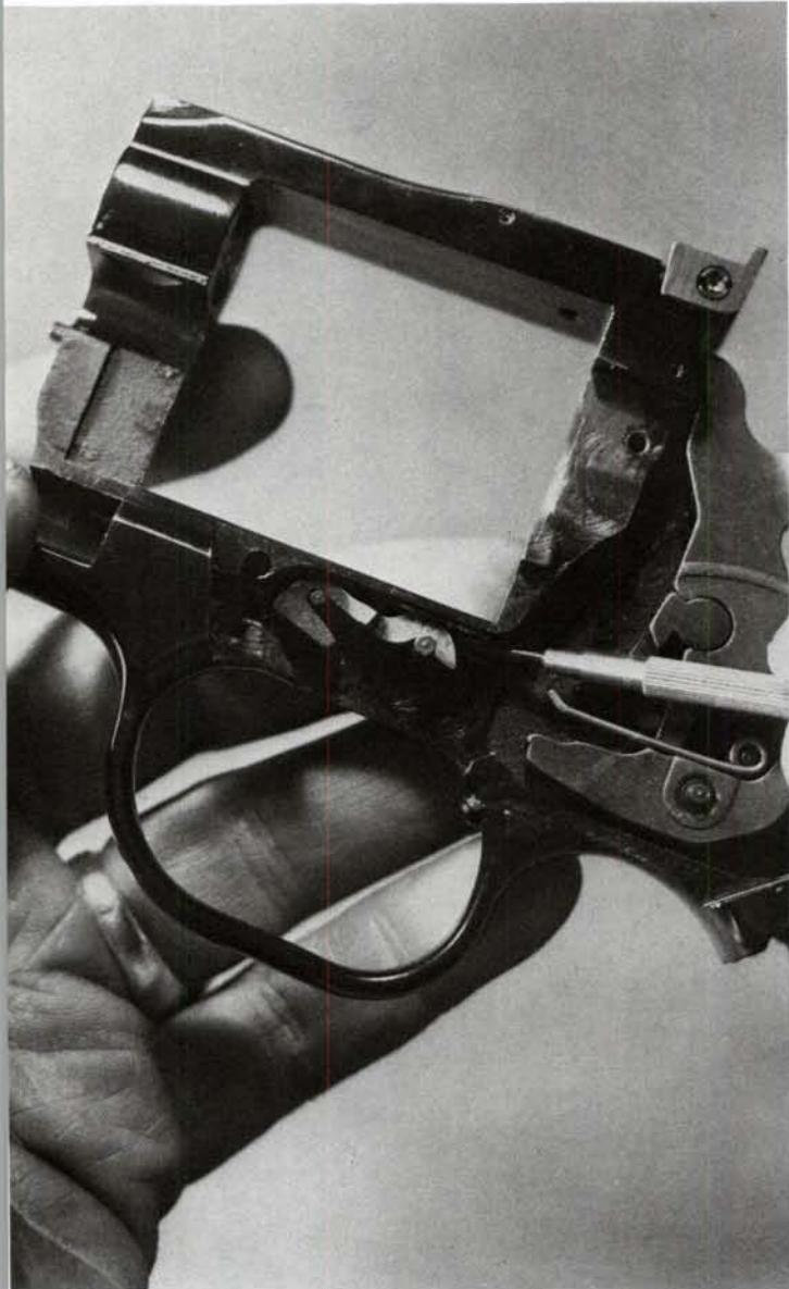
**20.** Lift the forward arm of the trigger spring off its shelf on the hammer and allow it to turn downward, relieving its tension.
