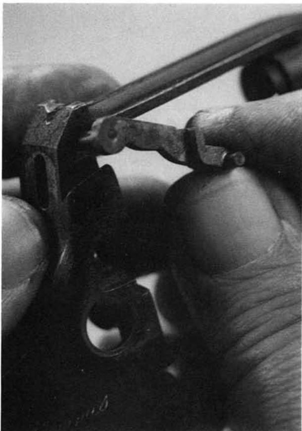
**16.** The right grip is retained by a screw on the inside of the grip frame.
