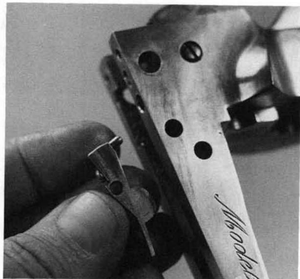
**18.** Remove the cylinder stop cross-screw, and take out the cylinder stop downward.
