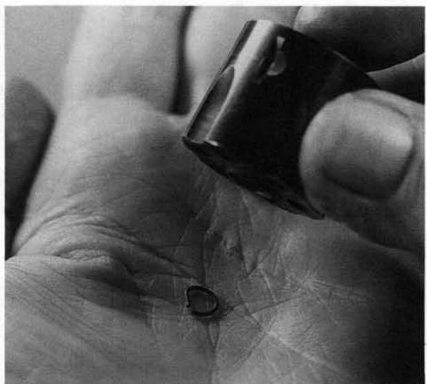
**5.** Take out or shake out the spring ring from inside the cylinder.
