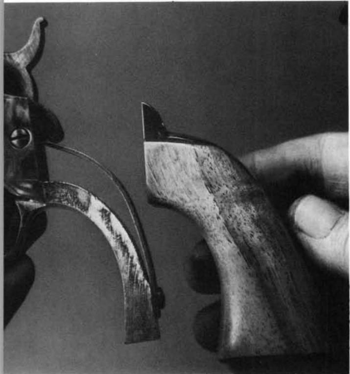
**9.** Tip the upper portion of the backstrap toward the rear, and remove it from the grip piece.
