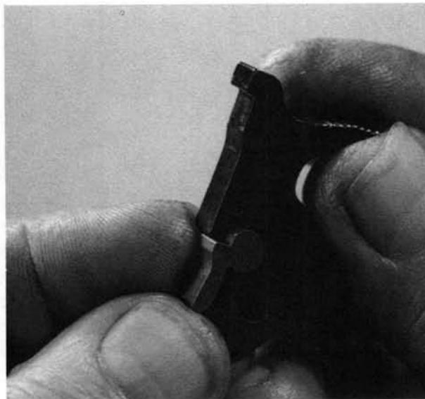
**20.** Push the double-action lever out of the hammer toward the left. **Caution:** Let the fingertip follow the part across, to arrest the plunger and spring as they are released.
