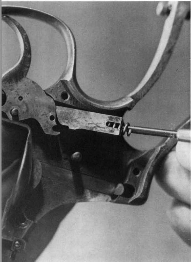
**16.** Drifting out the small cross-pin in the trigger will free the rebound strut for removal toward the rear.
