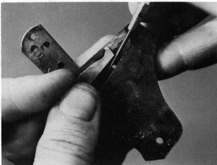
**2.** When replacing the sideplate, place the cylinder hand in position in its recess and release its spring plunger to hold it there. Be sure the pivot stud of the hand enters its hole in the trigger as the sideplate is pushed into place.
