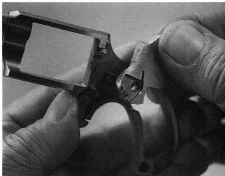
**11.** Remove the trigger toward the left. The coil spring is easily removed from the back of the trigger.
