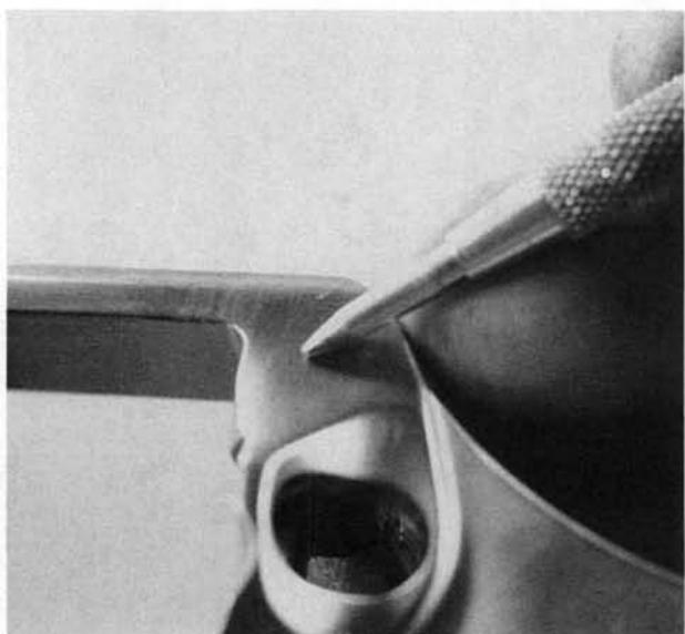
**33.** The firing pin housing ("recoil plate"), firing pin, and spring are retained in the frame by a cross-pin which is finished over at the factory. Even if it can be located and driven out, the finish will be badly marred. It's best to consider this a return-to-factory item.
