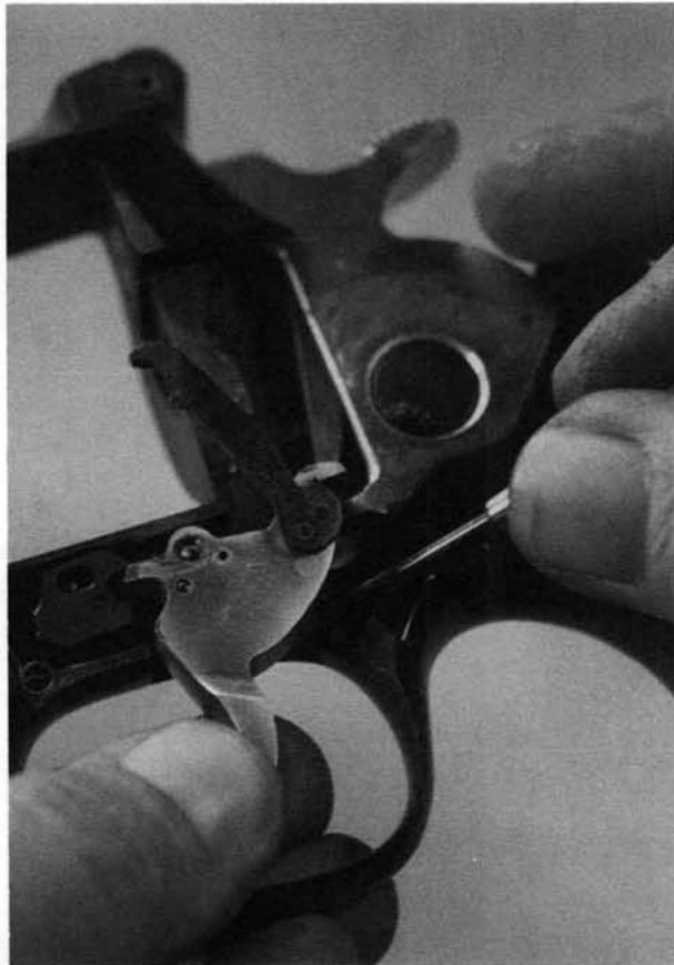
**23.** Insert a small tool to lift the rear arm of the cylinder hand spring, and remove the cylinder hand from the trigger.
