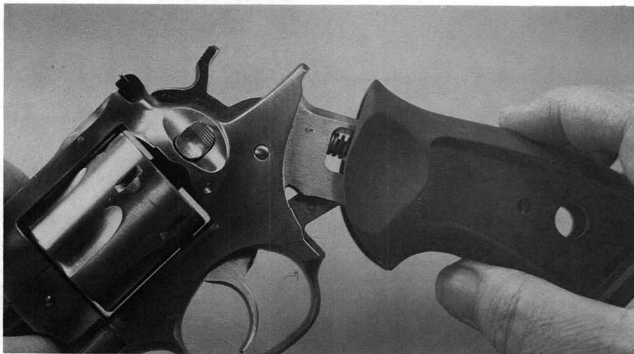
**6.** Cock the hammer, and insert the disassembly pin in the hole in the hammer strut.
