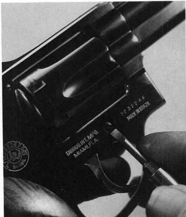
2. Operate the cylinder latch, open the cylinder, and remove the crane and cylinder assembly toward the front.
