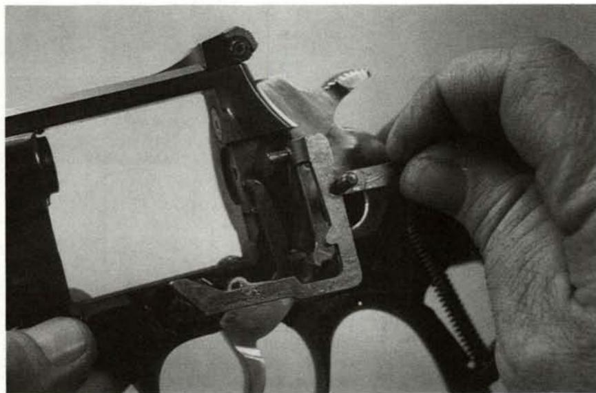
**18.** Remove the cylinder latch by moving it rearward to clear its center nose from the frame, then take it off toward the left.
