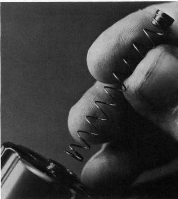
5. Remove the ejector/ratchet from the cylinder.
