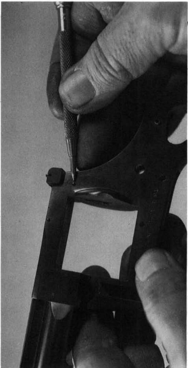
**24.** The rear sight is retained by a cross-pin. After the pin is driven out, unscrewing the elevation screw will release the sight. If the sight is removed, note that there is a spring under it.
