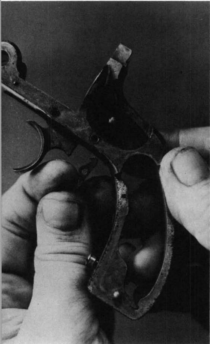
**20.** Move the trigger toward the rear until the hand and lever are against the hammer post, and use sharp-nosed smooth-jawed pliers to grip the cylinder hand, compressing the hand spring. Remove the cylinder hand toward the left.
