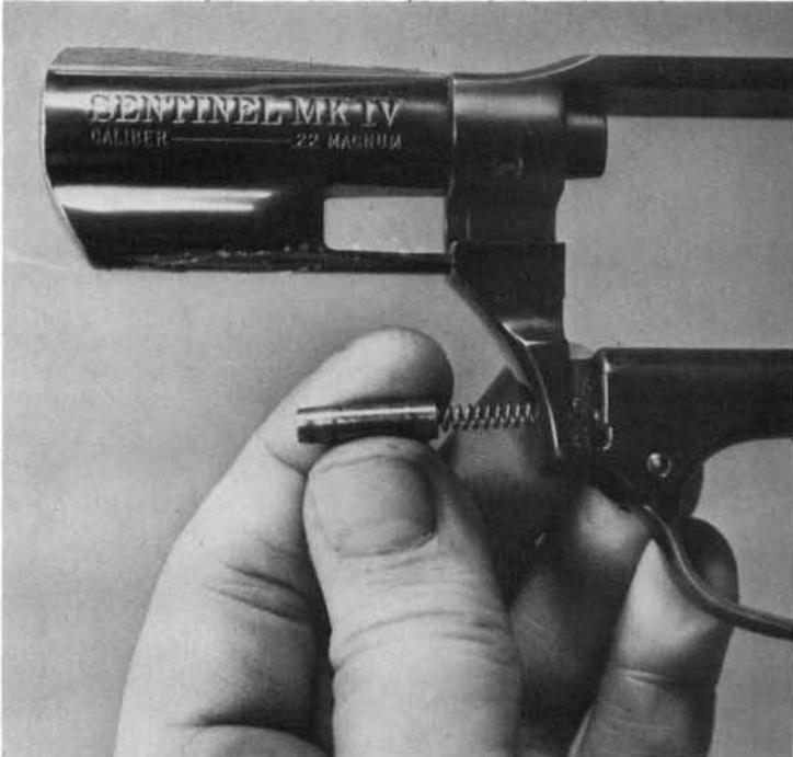
**4.** Pull the ejector/ratchet to the rear until its side lug emerges from the cylinder, and turn it to lock it in position. Note the retaining pin hole, just to the rear of the lug.
