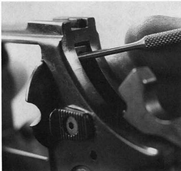
**14.** Ease the hammer down to fired position, and move the sub-frame downward to the level shown.
