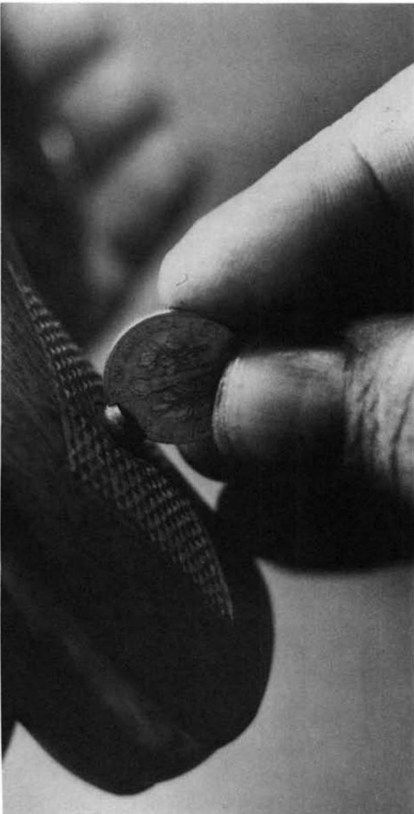
**2.** On the inside of the left grip is a hole which contains a small disassembly pin. When removing the grips, take care that this pin isn't lost.
