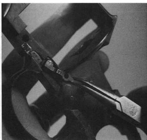
**23.** Tip the cylinder stop to its lowest position, and remove it toward the left.
