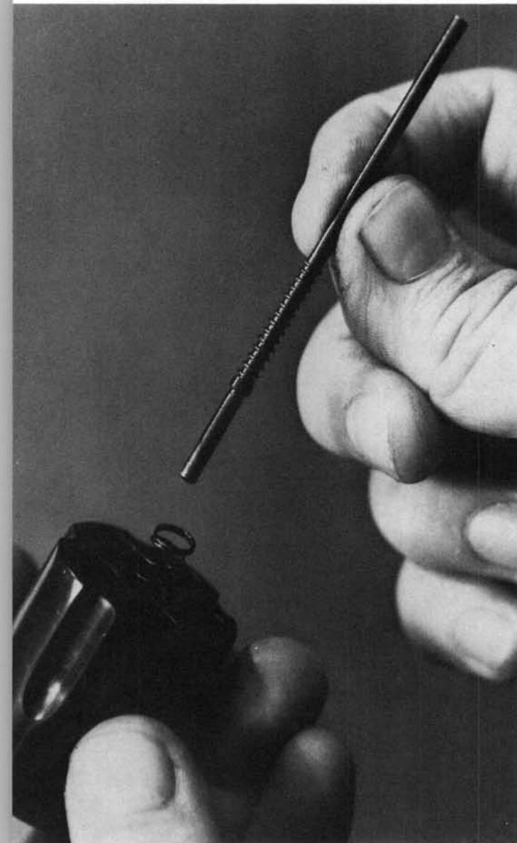
**6.** Remove the ejector spring from the front of the cylinder.
