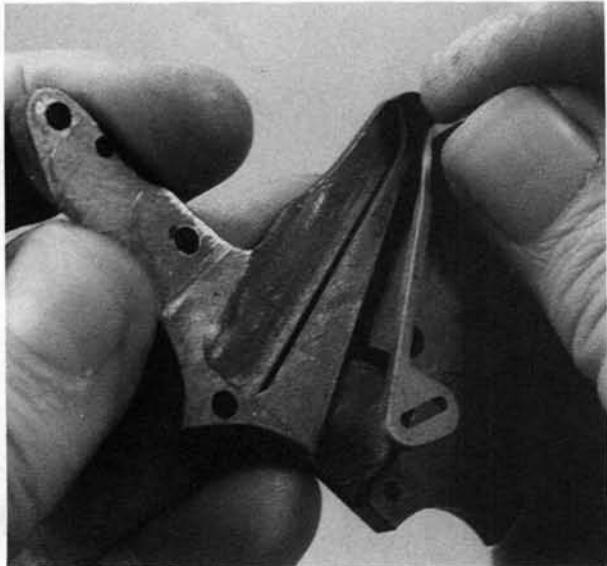
**11.** Push the hammer spring base ring out of the frame toward the left, controlling the spring as it comes out. When the hammer strut and spring are separated from the base ring, note which of the recesses is being used. There are four, of varying depths, for spring power adjustment.
