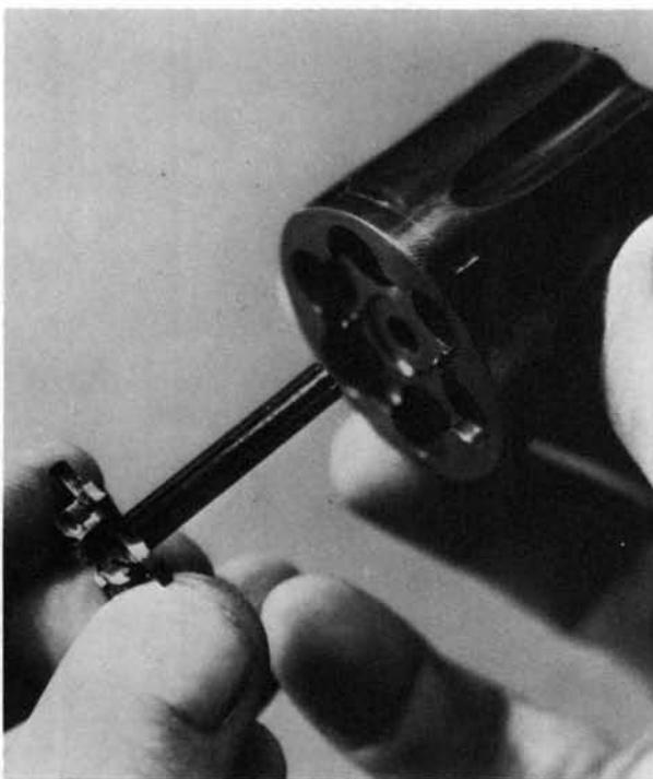
**7.** Use the Colt wrench to unscrew the retainer at the rear of the cylinder arbor on the crane, and remove the ejector spring toward the rear.
