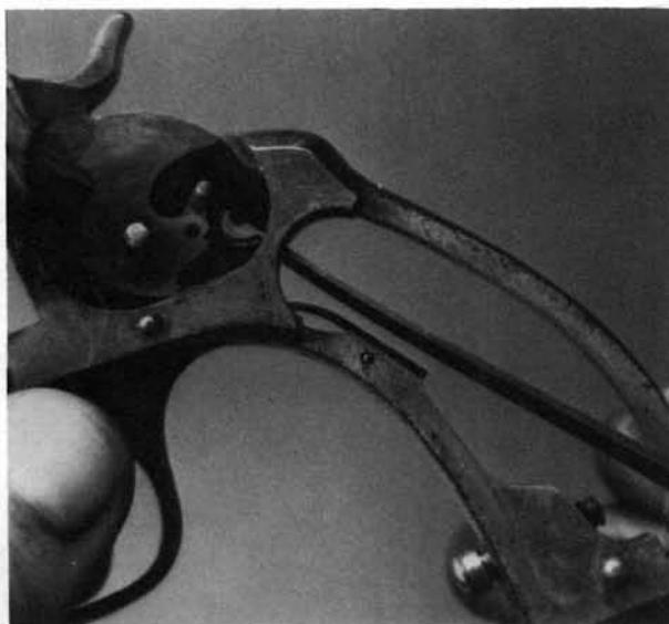
**13.** Drift out the small pin at the upper front of the grip frame and remove the sear spring toward the rear.
