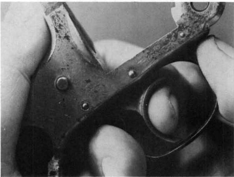
**16.** If the guard is very tight, it may be necessary to tap it forward, as shown, to jump it out of the frame recess.
