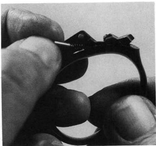
**18.** Remove the cylinder stop plunger and spring.
