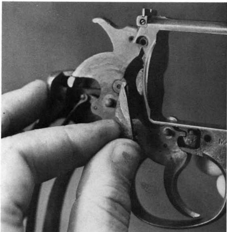
**11.** Back out or remove the hammer spring screw, located at the lower front of the grip frame.
