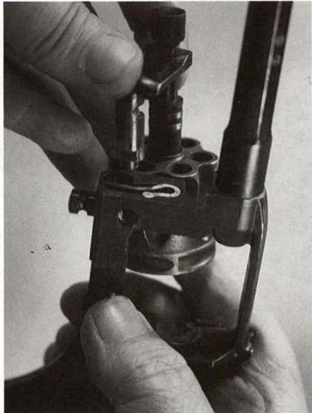
**11.** If removal of the crane positioning spring is ever necessary, its mounting post can be driven out toward the front from inside the cylinder space.
