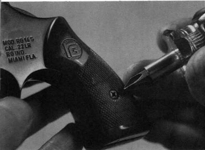
**7.** Use the same Phillips screwdriver to remove the three sideplate screws on the right side, two as shown, and one at upper rear.
