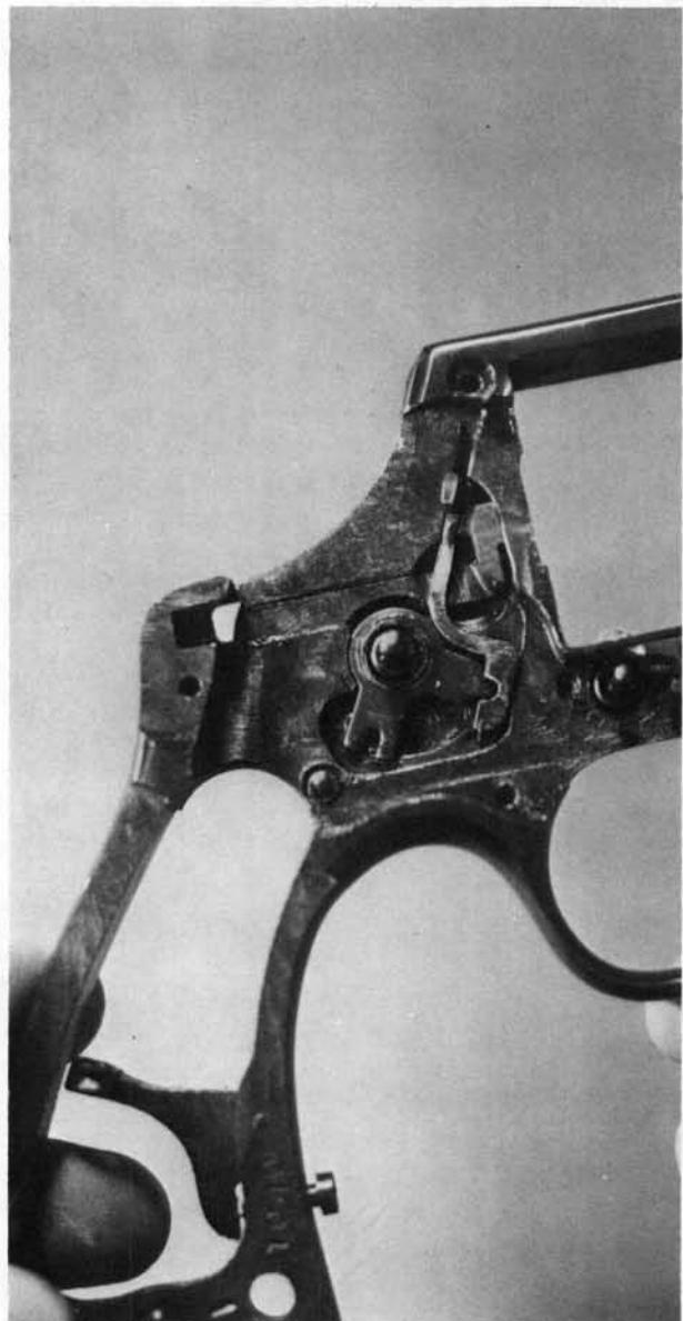
**17.** Remove the cylinder stop spring cover screw, located at the upper front of the trigger guard. Then remove the cylinder stop spring and plunger.
