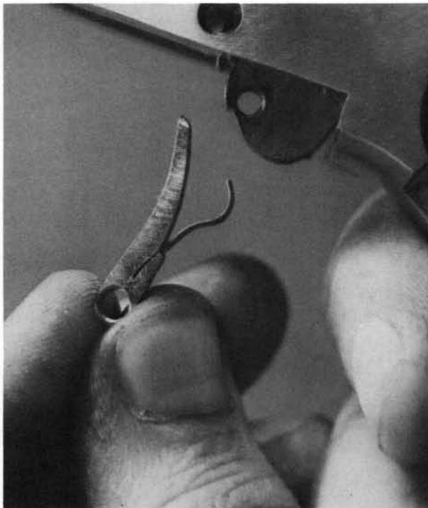
**15.** Remove the hammer from the top of the frame.
