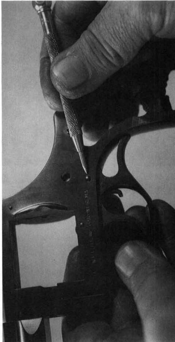
**14.** Remove the trigger guard downward and forward.
