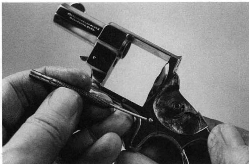
**12.** Drift out the trigger cross-pin.
