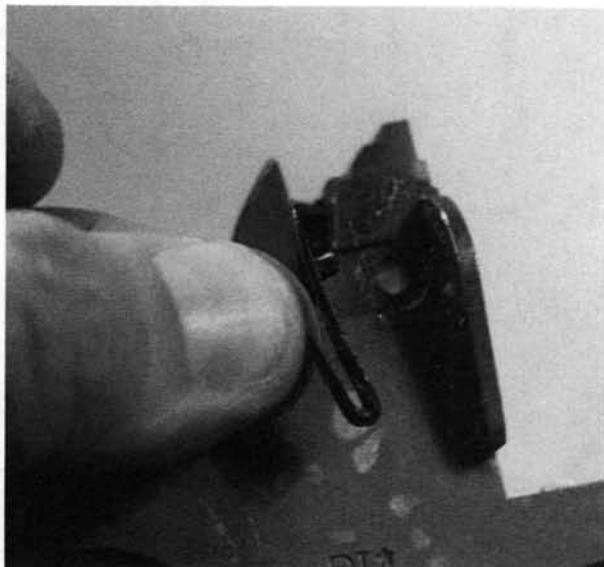
**16.** Remove the barrel latch spring from the right side of the frame.
