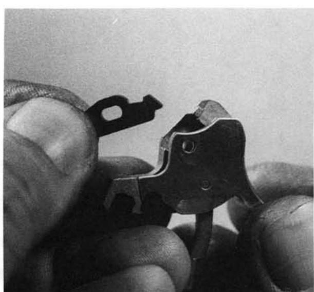
**16.** Remove the cylinder stop trip from its recess in the top of the trigger. The trigger spring strut is cross-pinned in the trigger. In normal takedown this is left in place.
