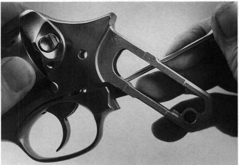
**9.** Insert a tool through the hole in the back of the grip frame to depress the trigger guard latch, and move the rear of the guard downward.
