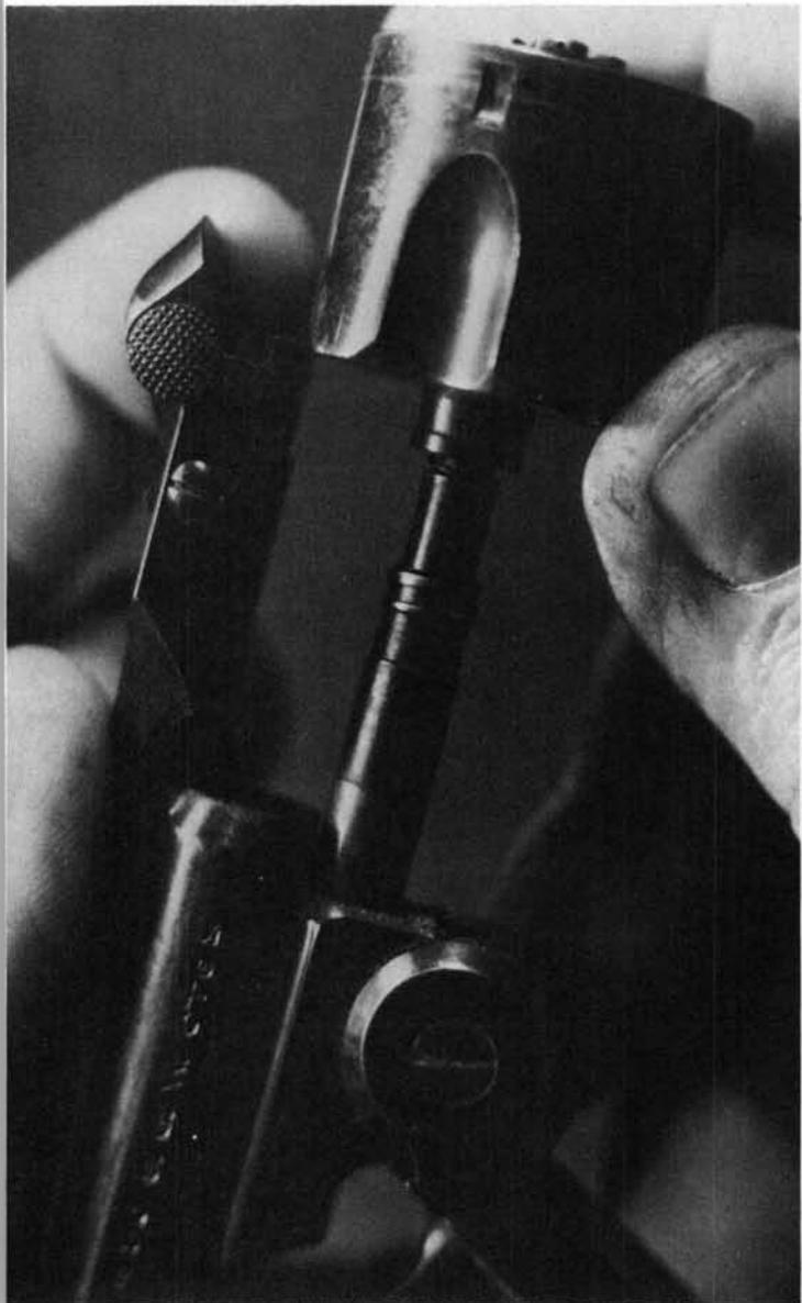
2. Using smooth-jawed pliers, grip the ejector post and turn it toward the left (front view). Unscrew the post from the ejector shaft.
