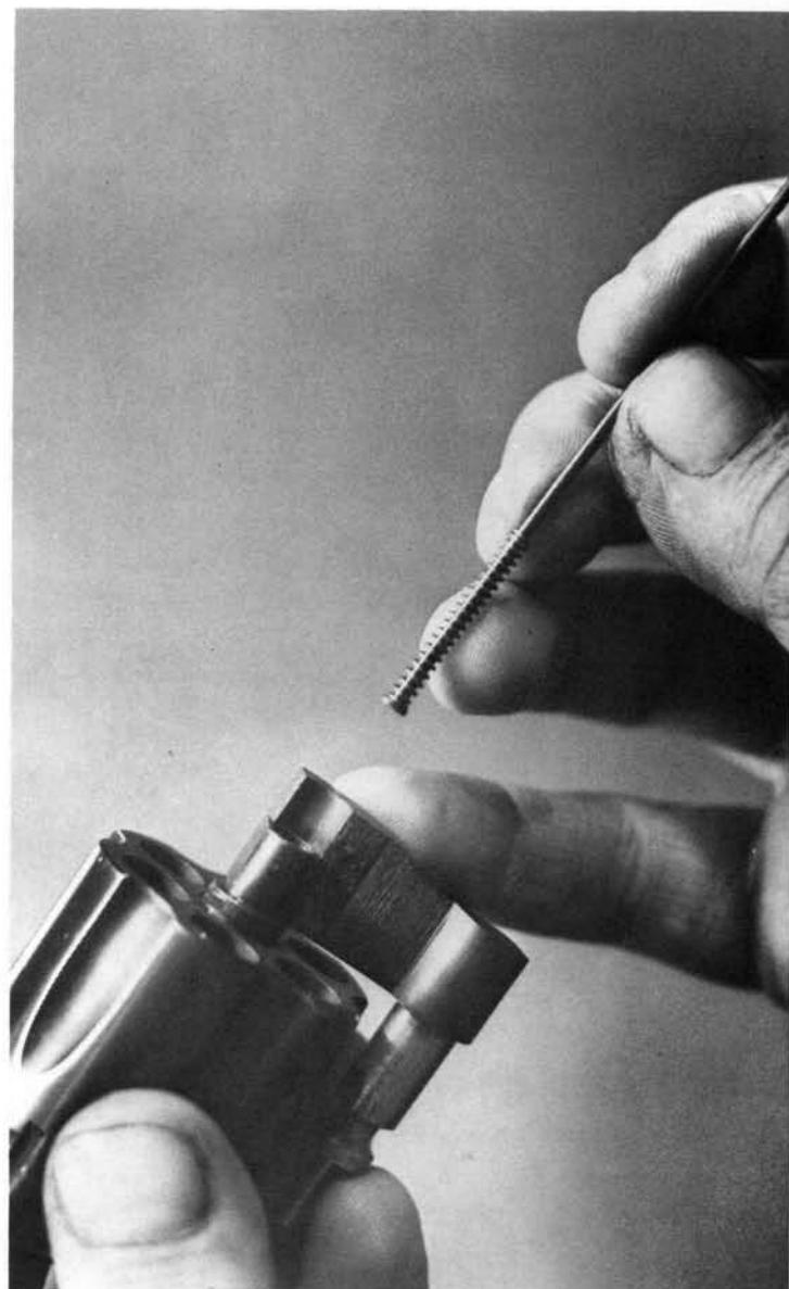
**20.** Remove the crane toward the front. The small ball bearing in the side of the cylinder arbor on the crane is staked in place, and removal is not advisable.
