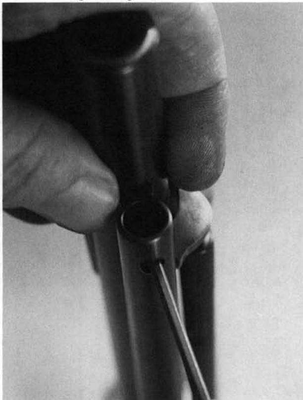
**23.** The ejector housing is often tightly fitted, and it may be necessary to use a drift and hammer, as shown, to nudge it forward out of the frame.
