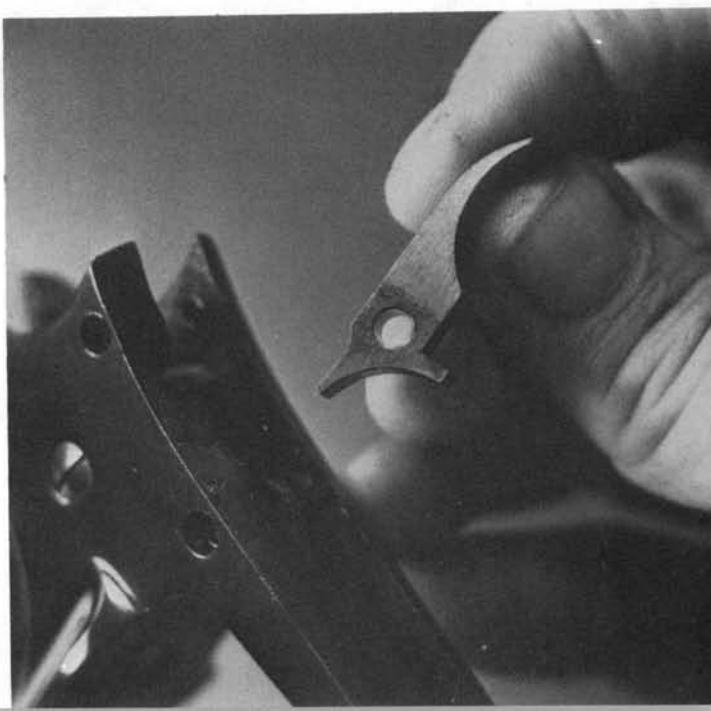
**12.** Retained by the same screw, the cylinder stop is also freed for removal from the bottom of the frame.
