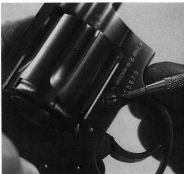
2. After the screw is removed, take out the crane retaining plunger and spring.
