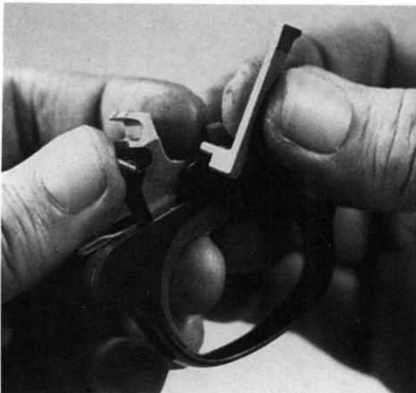
**14.** Push out the trigger cross-pin.
