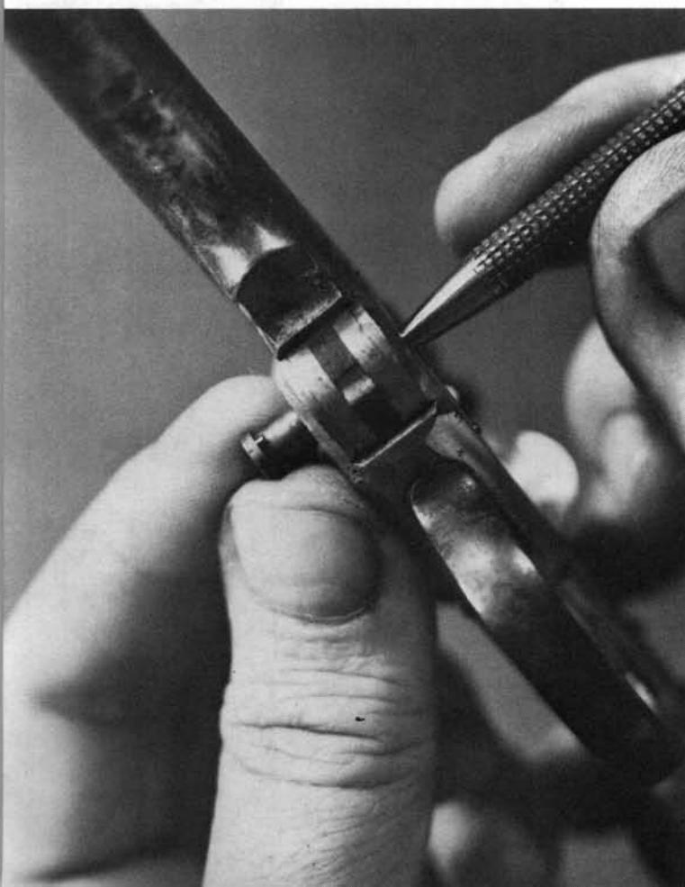
**6.** Select a drift punch that will easily enter the hole in the barrel hinge, and push the hinge out toward the right side.
