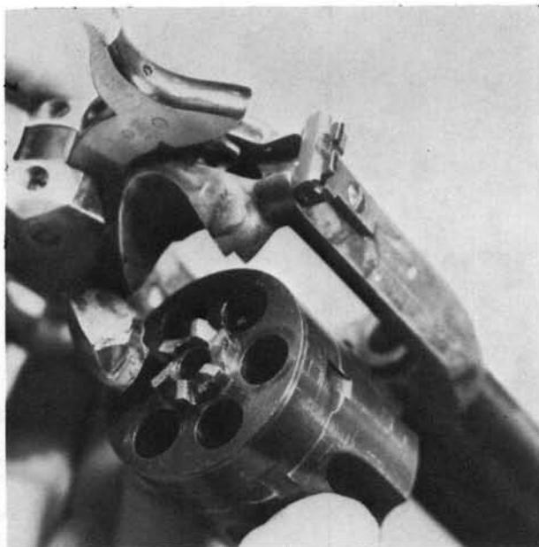
**3.** Open the loading gate and remove the cylinder toward the right.
