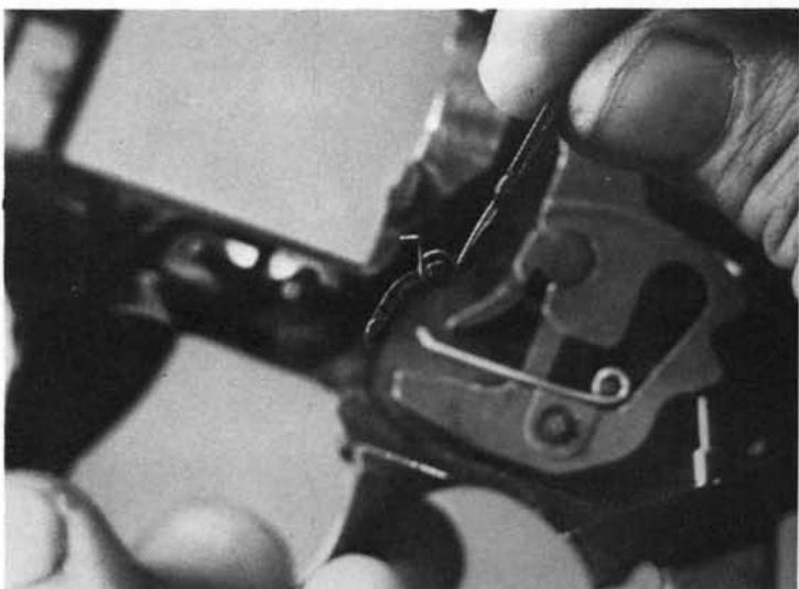
**19.** Tip the cylinder stop down out of its slot in the frame, and remove it toward the left.
