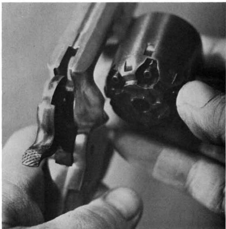
**7.** Drifting out the small pin at the end of the loading lever will release the lever latch and its spring for removal. Removal of the two cross-screws in the lever assembly will allow separation of the lever, rammer, and the cylinder base pin.
