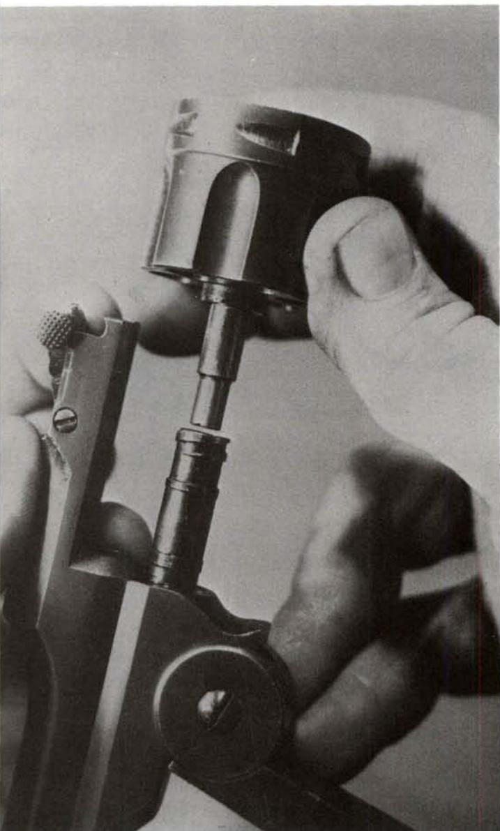
2. The ejector rod head is cross-pinned to the shaft of the ejector, and the pin is often difficult to locate on the polished surface. The tip of the drift punch is pointing to the pin here. The pin must be drifted out before the ejector head can be unscrewed.
