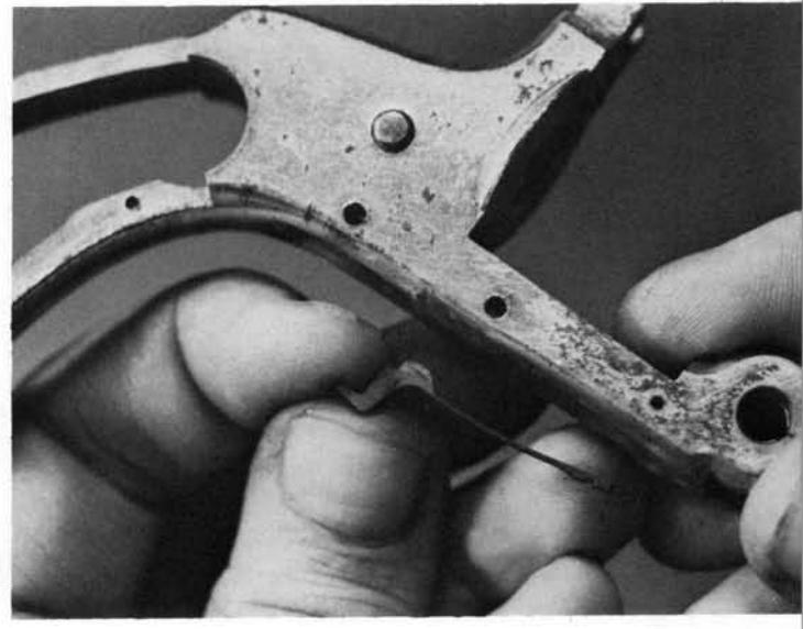
**24.** Remove the cylinder stop from the frame recess.
