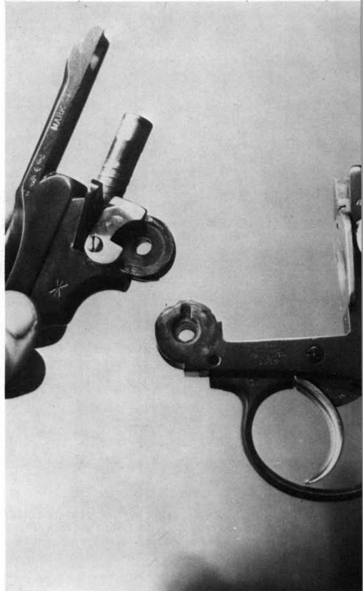
**9.** Remove the ejector cam from between the hinge loops at the bottom of the barrel unit. Drifting out a cross-pin in the cam will release the cam leaf and its spring, but this is not advisable in normal disassembly.
