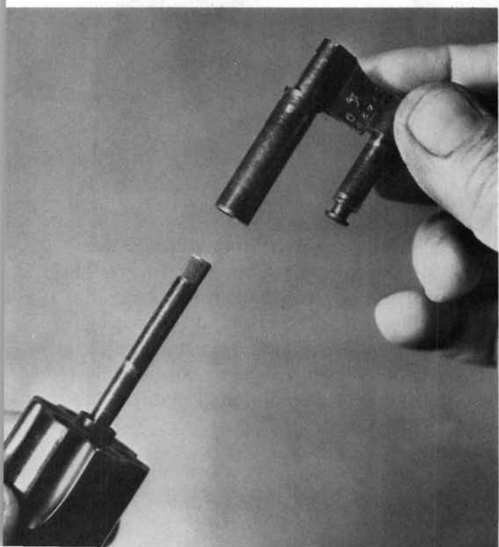
**4.** Grip the ejector rod head with leather-padded smooth-jawed pliers, and unscrew the ejector rod clockwise (front view).
