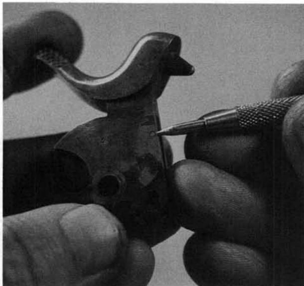
**19.** With a wrench of the proper size, unscrew the trigger spring retainer.
