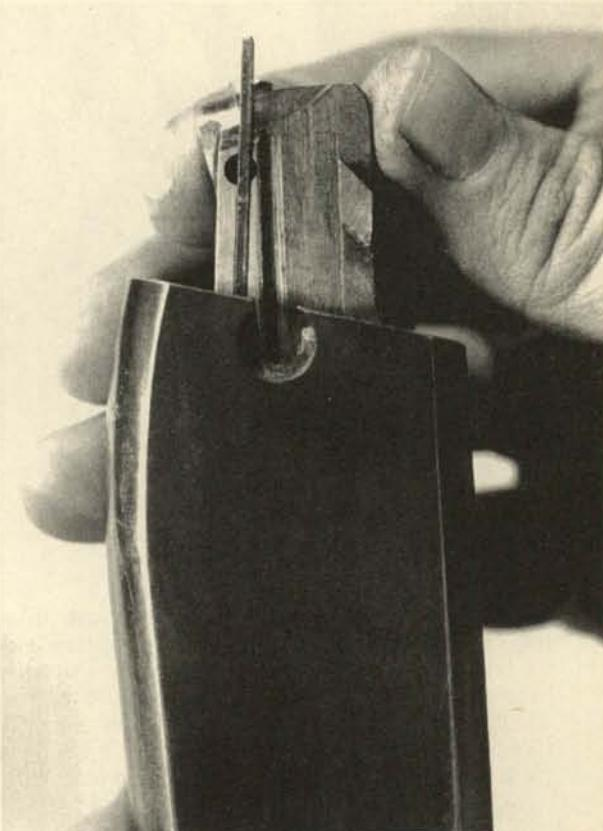
5. To begin disassembly of the bolt, drift out the vertical pin in the left lower front that retains the feed extractor and its transverse coil spring. The pin should be driven out downward using a very small diameter drift punch to start it. Its upper end is within a recess on the bolt, so it can't be drifted straight out. After starting, it usually comes out easily.
