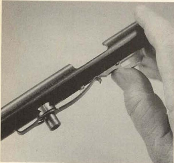
**10.** Pull the rear of the sear/ejector downward, just far enough to clear its rear upper projection, and remove it toward the rear.
