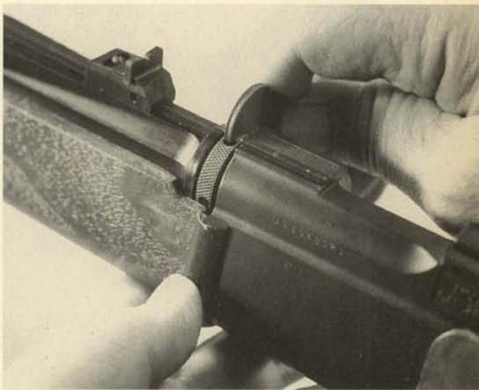
**2.** When tightening the barrel nut, be sure the forend is kept in alignment to properly enter the flange at the front of the receiver.
