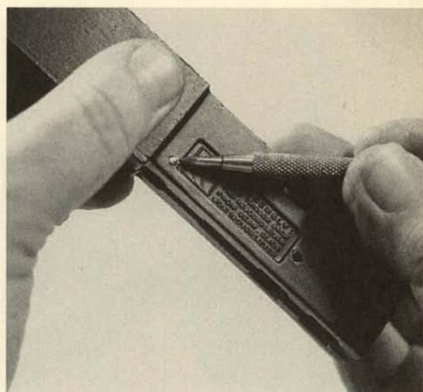
**28.** Drift out the sear spring retaining pin, and remove the sear spring downward.
