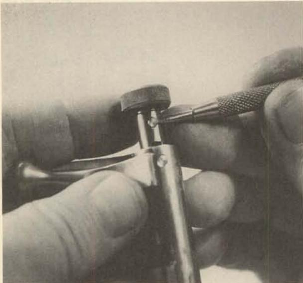
**14.** Remove the cocking knob and rebound spring toward the rear. The spring is easily removed from inside the knob shaft.
