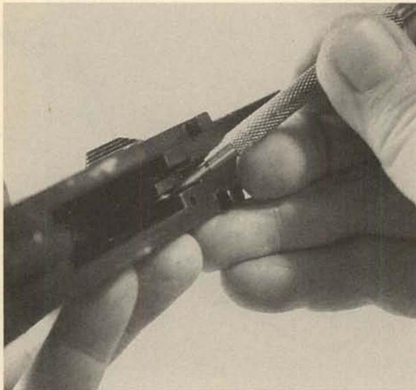
**28.** Drifting out this cross pin will release the bolt hold-open and its coil spring for removal.
