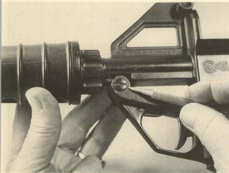
**18.** For easier access to the parts in the lower receiver, you may wish to separate it from the upper receiver. To remove the pivot shaft, use a properly-fitted screwdriver to take off the cap screw. It will be necessary to hold the head of the shaft on the other side. Grip it with non-marring pliers, or, as I did, just press it against the wooden edge of a workbench. The finish is easily marred, so work with care.
