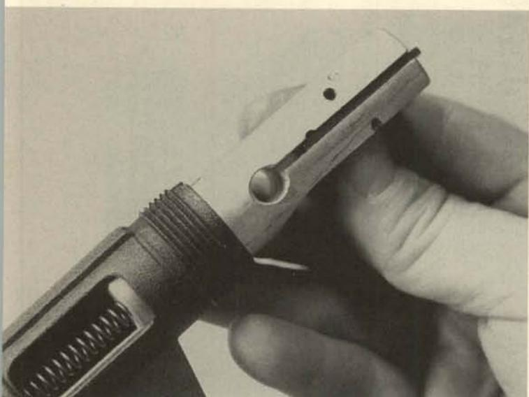
**13.** Remove the bolt, along with its twin springs and spring guide unit, toward the front.
