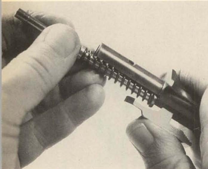
2. When replacing the Allen screw, be sure the screw hole is precisely aligned before turning the screw into place.
