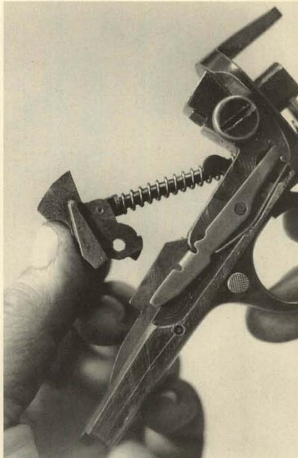
**19.** Remove the carrier upward and toward the rear, disengaging the tip of its frame-mounted torsion spring from the slot and cross pin in the lower lobe of the carrier. Do not lift the carrier straight up or move it forward during removal, or the spring will be deformed. The spring is retained in the frame by a cross pin, located just forward of the guard. Note its position inside the frame before removal.
