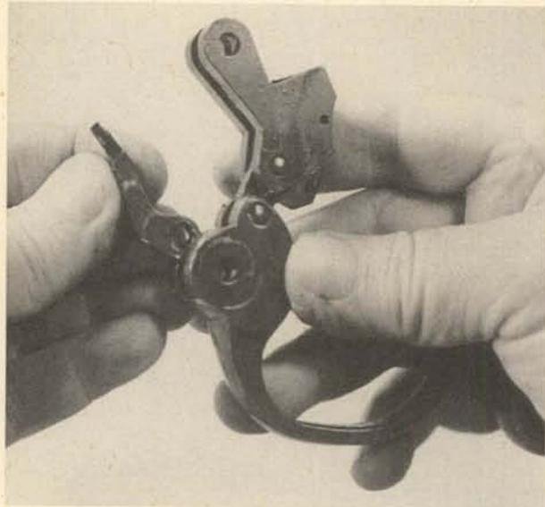
**12.** Remove the ejector from the front of the lever.
