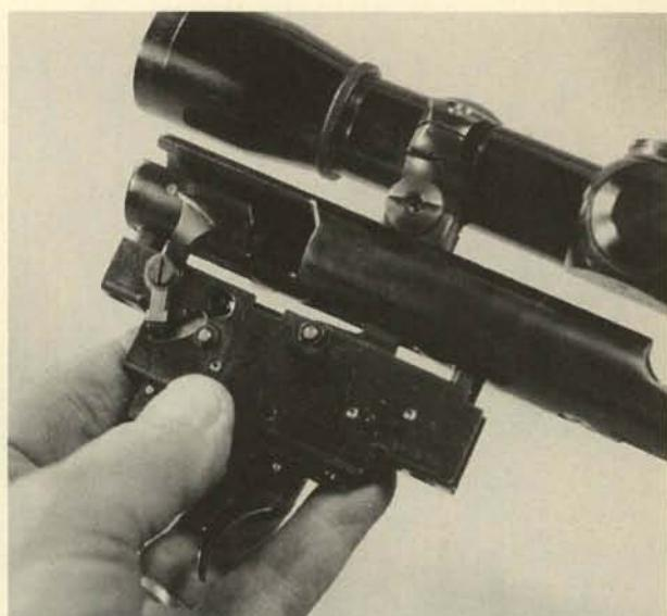
**25.** The principal spring-bearing cross pins in the trigger group are riveted in place, and routine removal is not possible. The set-trigger system is in the same category. If necessary for repair, some of the main parts can be removed, and we will show the sequence here, without removal of the parts. The safety-lever and its detent ball and spring can be taken off by removing this screw. Take care that the detent ball isn't lost.
