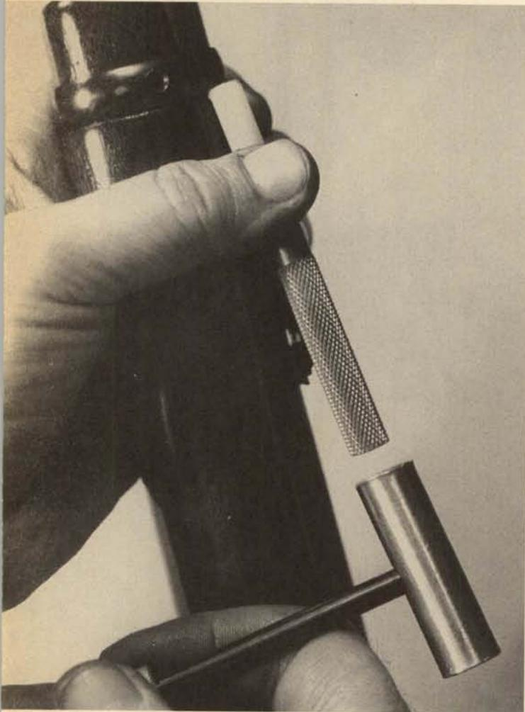
**18.** Remove the cross screw from the front barrel band, and slide the outer magazine tube out toward the front. Remove the forend forward and downward.
