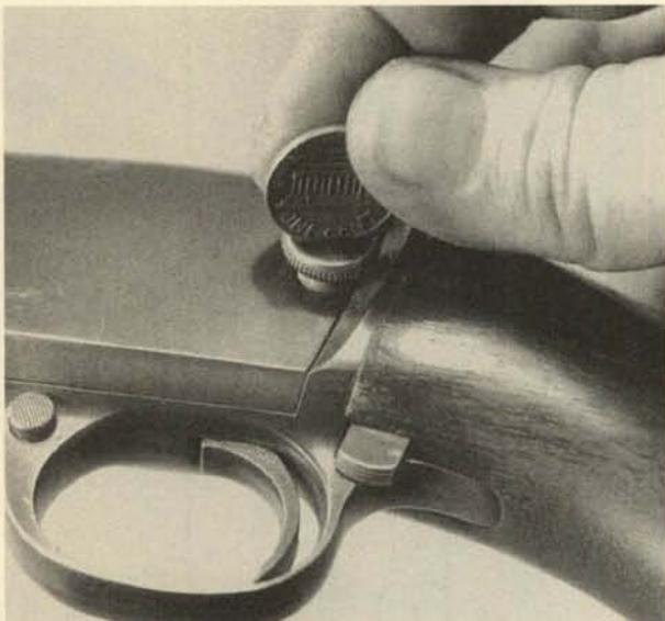
2. When the takedown screw has moved a short distance to the left, clearing its seat in the receiver wall, separate the front and rear sections of the gun, moving the rear section toward the rear and downward.
