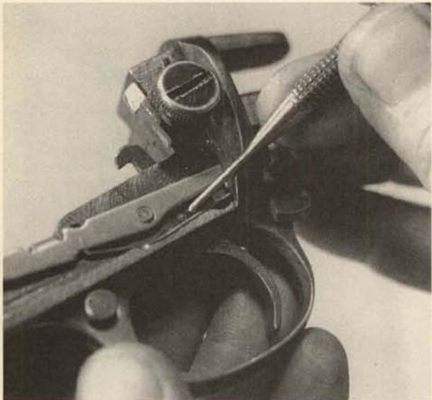
**21.** Removal of the trigger pin will also free the hammer catch/slide latch lever, and it can be tipped down at the front, moved toward the rear, and taken out the rear opening of the frame. The clearances here are close, and some maneuvering of the part will be required.
