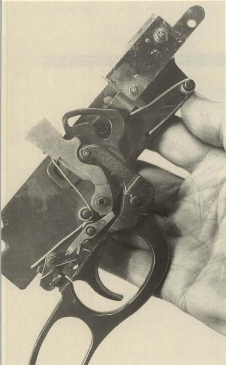
**2.** This photo shows the safety catch in place and in the on-safe position. Note that the spring arm at its lower edge goes *below* the stop pin.
