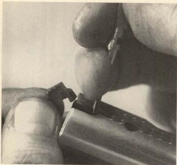
**13.** Invert the gun and move the bolt slowly toward the rear. Lift the front of the bolt enough to clear the receiver, and ease the bolt out forward, slowly relieving the tension of the bolt spring. **Caution:** *Control the compressed spring. Remove the spring and its guide from the rear of the bolt.*
