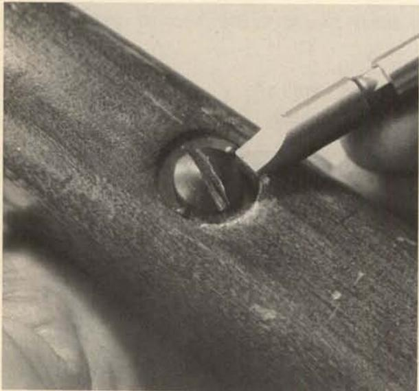
**2.** Pull the trigger to drop the hammer to the fired position and unscrew the receiver end piece, taking it off toward the rear.
