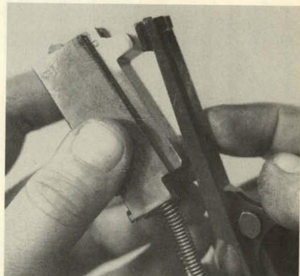
**8.** Remove the striker from the rear of the bolt.
