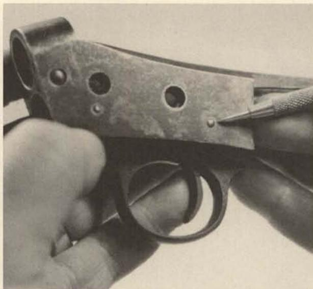
**8.** Drift out the trigger cross pin and remove the trigger upward.
