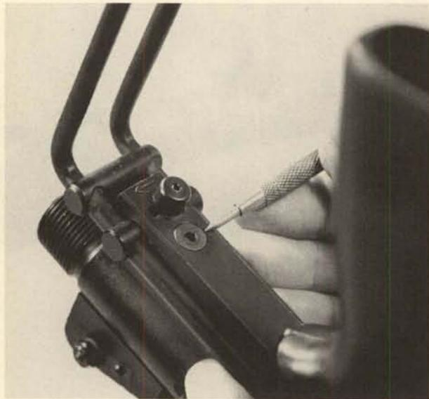
**15.** Remove the large Allen screw at the rear of the lower receiver.
