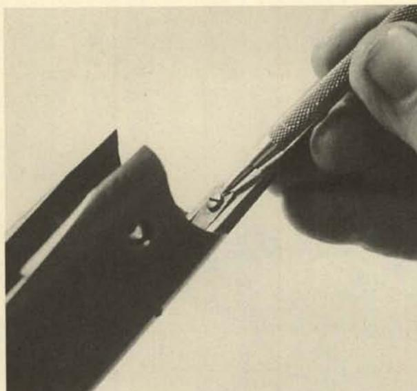
**19.** In our subject gun, the sear spring screw is located inside the upper tang. Remove the screw and take out the sear spring.
