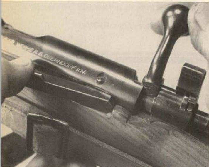
2. Taking care not to trip the safety-lever, unscrew the bolt sleeve, turning it counterclockwise (rear view). Remove the bolt sleeve and striker assembly toward the rear.
