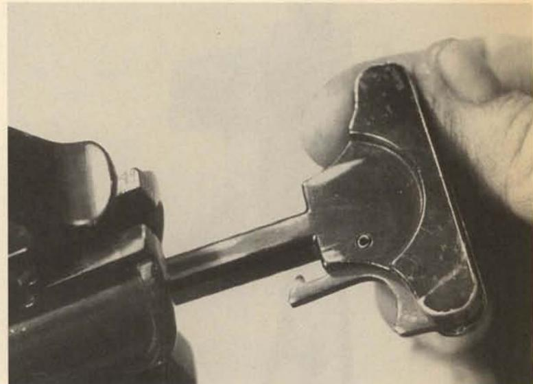
3. Move the charging handle downward, out of its track in the top of the receiver, and remove it toward the rear. Drifting out the vertical roll pin in the left lobe of the handle will allow removal of the lock lever and its spring.
