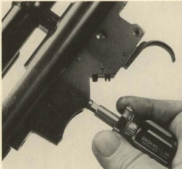
**22.** Remove the trigger and magazine housing downward.
