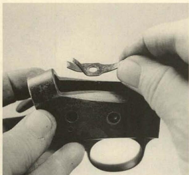
**11.** Remove the screw inside, in the floor of the receiver, and take out the combination spring.
