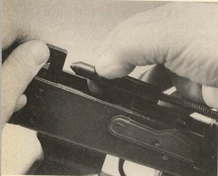
4. If removal of the spring from the guide is necessary, pull the spring away from the C-clip and remove the C-clip from the rod. **Caution:** Control the spring.
