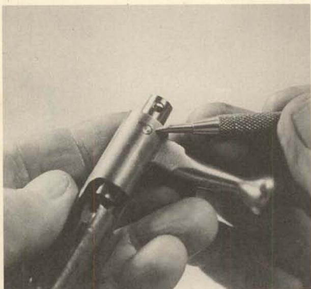
**15.** Drift out the striker retaining pin upward. Avoid canting the pin after it clears one wall of the bolt.
