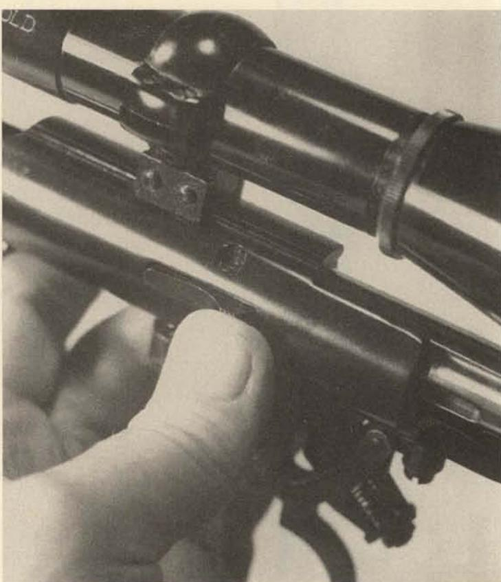
**4.** Grip the front section of the bolt and turn the safety-lever counterclockwise (rear view) until the striker drops to the fired position. Continue turning the safety until it stops; it can then be taken off toward the rear.
