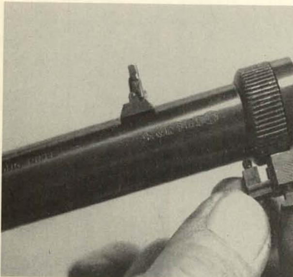
**5.** Remove the takedown latch base ring toward the rear. Unscrew the knurled barrel adjustment nut and remove it toward the rear.
