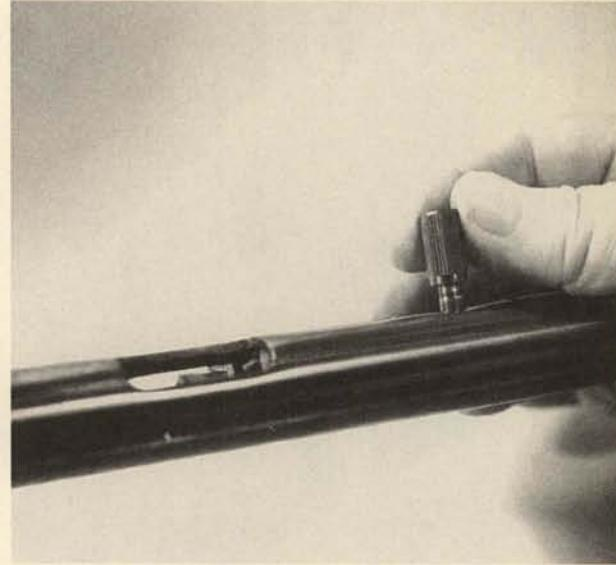
8. Point the barrel upward and retract the bolt handle fully to the rear. While exerting slight outward pressure on the bolt handle, push the striker (firing pin) forward until its exit cut aligns with the bolt handle. The bolt handle can then be removed toward the right.
