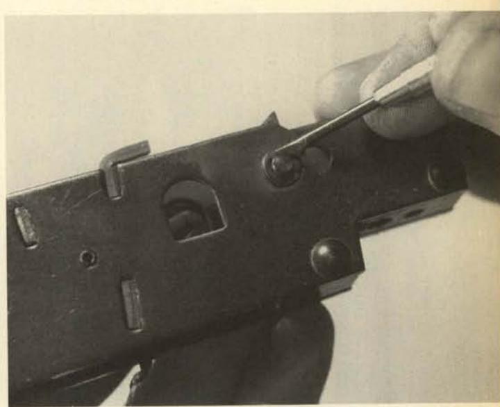
**11.** The bolt hold open device is retained by a C-clip on the right side of the group, the clip gripping the end of its cross-shaft. Note that there is also a small washer under the C-clip, and take care that it isn't lost. The hold open is removed toward the left.
