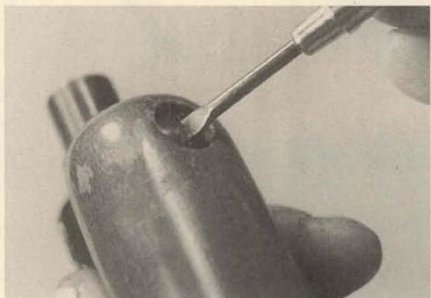
**3.** When replacing the action in the stock, note that the front sight must be slid onto the muzzle before the action is seated, so the protrusion on its underside will enter its well in the stock. The sight screw and nut may be turned into place together; then the small center screw may be turned separately for any adjustment necessary to snug the unit in place.
