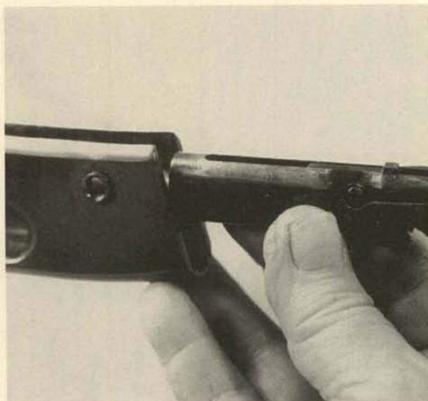
**10.** Remove the magazine housing toward the rear. The forend will be freed as the magazine housing clears it.
