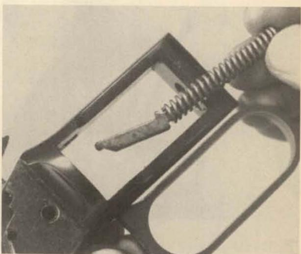
**12.** Restrain the hammer against its spring tension, pull the trigger to release it, and ease the hammer forward, past its normal down position. This will relieve the tension of the hammer spring, and the spring and its guide strut can then be removed from the rear, toward either side.
