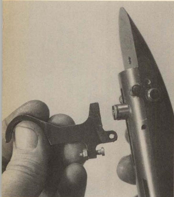
**21.** Remove the sear and disconnector assembly downward.
