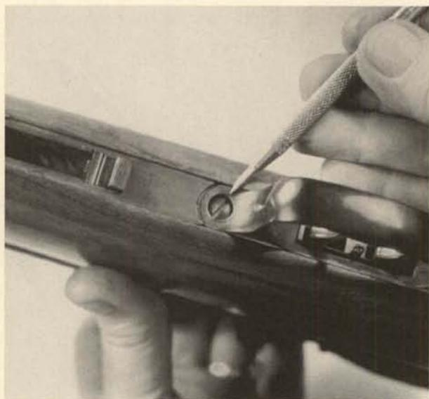
**11.** Remove the screw in front of the trigger guard.
