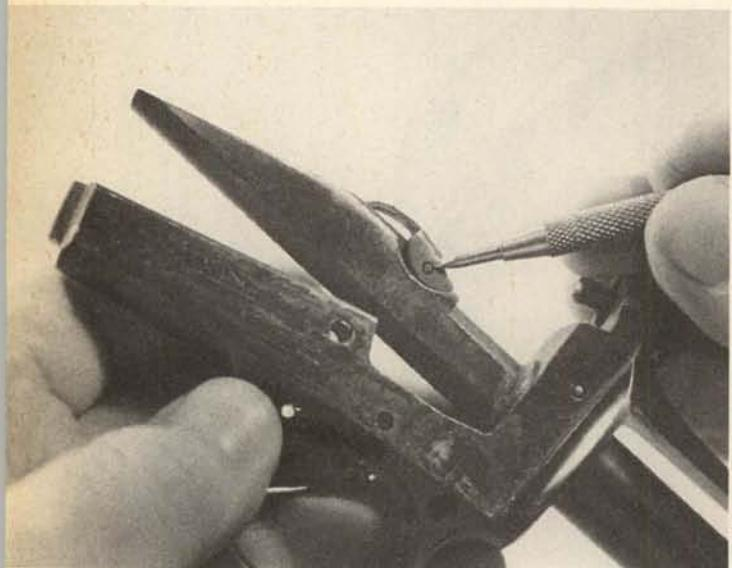
**32.** In normal takedown, the magazine housing is best left in place. However, if removal is necessary, this cross pin retains it in the lower receiver. After the pin is drifted out, the housing is moved forward out of the lower receiver. In removal of the magazine housing, there is always the possibility of damage.
