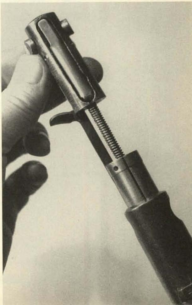
**4.** Bring the bolt and sear housing (end piece) together until they meet to cock the striker. With a firm grip on the bolt and end piece, push out the cocking handle retaining pin, located at the right rear of the bolt. **Caution:** Control the compressed bolt spring, and let the tension off slowly as you move the bolt and end piece apart. Removal of the cocking handle will instantly release the two parts, so be prepared for it.
