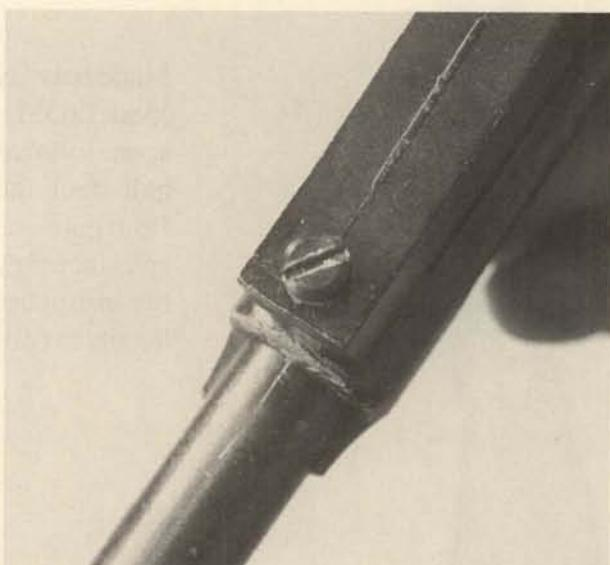
4. Cycle the bolt to cock the internal hammer and remove the vertical screw at the front of the trigger group.
