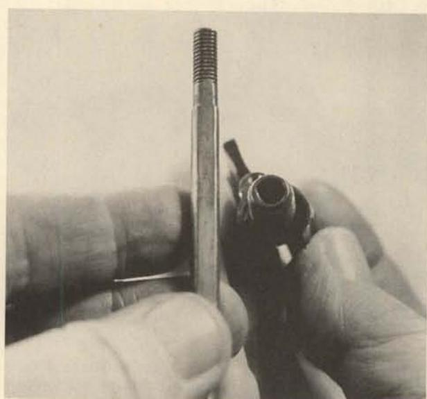
**2.** When reassembling the striker assembly, note that one side of the striker shaft is flat, and it must mate with a like surface inside the end piece.
