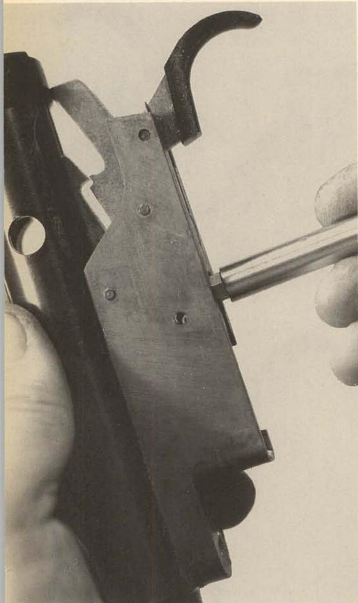
**12.** Remove the magazine housing downward.
