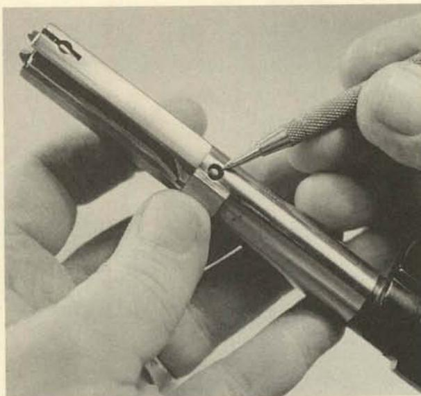
**3.** After the headpiece is turned, the head of the breechblock pin will be visible in this opening. Use a drift in the aperture on the other side, and push the breechblock pin out. Remove the breechblock toward the front.
