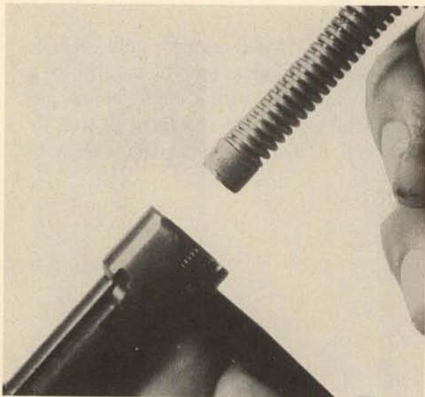
3. Remove the striker and its captive spring assembly from the rear of the bolt. The striker head may be separated from the front portion of the striker by drifting out the roll cross pin. This will release the striker spring with force, so proceed with caution. In normal disassembly, this unit is best left intact. If it is taken apart, take care not to lose the compression washer, located between the spring and the striker head.
