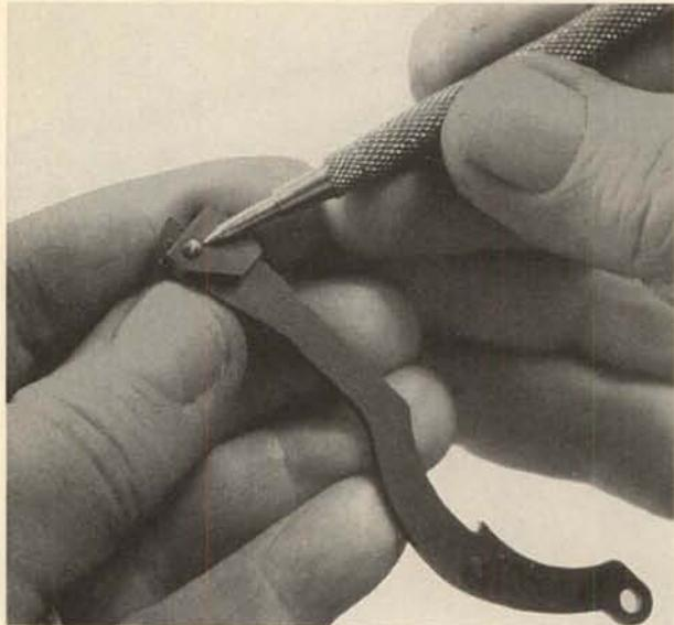
**22.** Restrain the sear and push out the sear cross pin. **Caution:** The spring is under tension.
