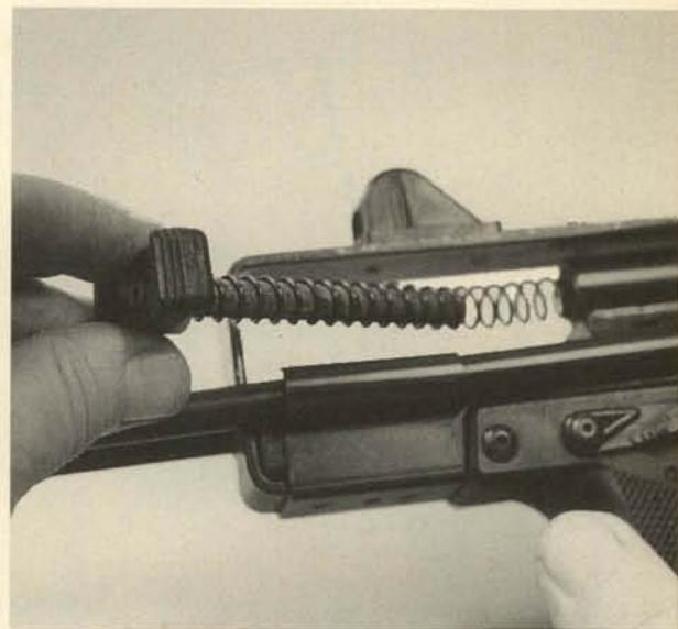
**7.** Move the bolt assembly all the way to the rear, and tip the bolt handle downward. Remove the bolt assembly toward the right.
