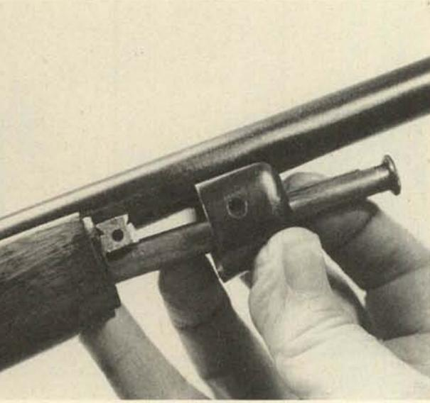
**3.** Remove the two screws, one on each side, that retain the forend cap. Remove the forend cap and cocking plunger assembly toward the front. The plunger spring is easily removed from inside the plunger. The knob is retained on the plunger by a cross pin.
