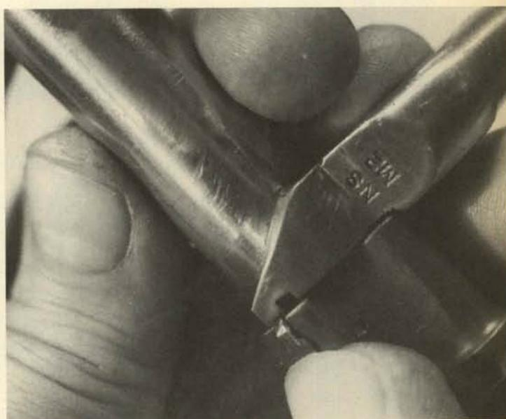
**12.** Grip the bolt firmly and pull back the striker knob until the safety can be turned up to vertical position, halfway between the on-safe and off-safe positions. This is more easily done before taking the bolt out of the receiver. Press the bolt sleeve lock inward, hold it in, and turn the rear section of the bolt counterclockwise (rear view), unscrewing the rear portion from the bolt body.
