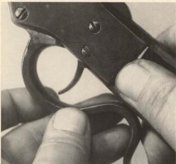
**6.** Taking out the hammer and trigger pivot screws will release the hammer for removal upward and the trigger for removal downward.
