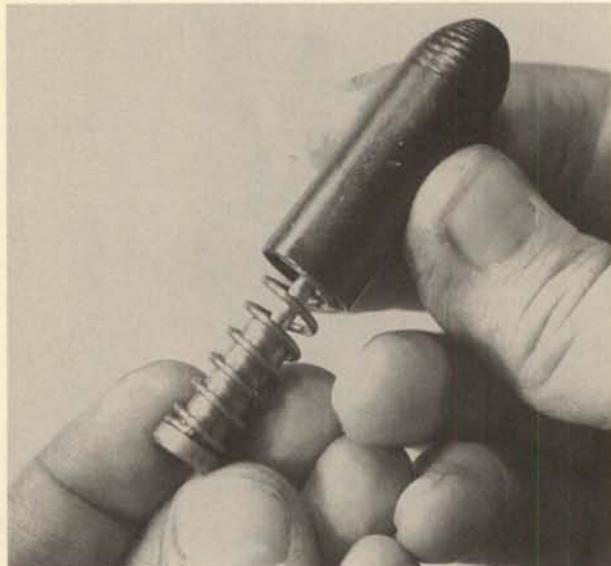
6. Move the bolt handle sleeve off toward the rear, taking with it the striker/firing pin unit.
