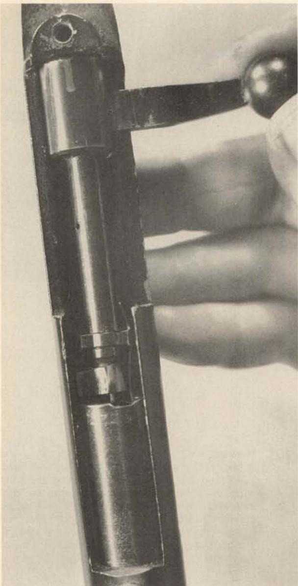
**2.** When replacing the trigger group on the underside of the receiver, be sure the front screw, the one with the extended tip, is put back in front, and see that the barrel is oriented so the screw tip will enter the recess in the underside of the barrel, locking it in place.
