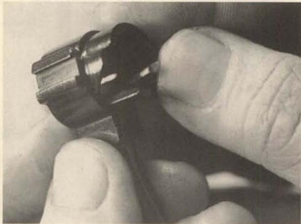
10. To remove the bolt handle positioning plunger and its spring, push the plunger toward the rear and tip its flat rear end inward; then move the part out toward the front of the handle sleeve. Take care not to lose the small coil spring.
