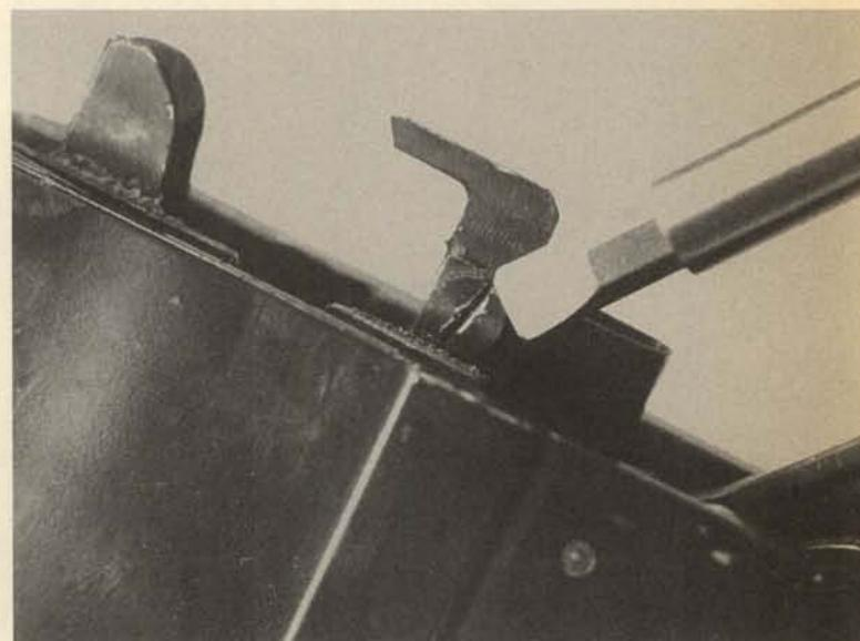
**12.** Turn the safety to the off-safe position, restrain the hammer, and pull the trigger. Ease the hammer down. Removal of the ejector/hammer stop will allow the hammer to go further forward than its normal position, partially relieving the tension of the hammer spring. Drift out the hammer pivot pin toward the right, and remove the hammer and hammer spring upward.
