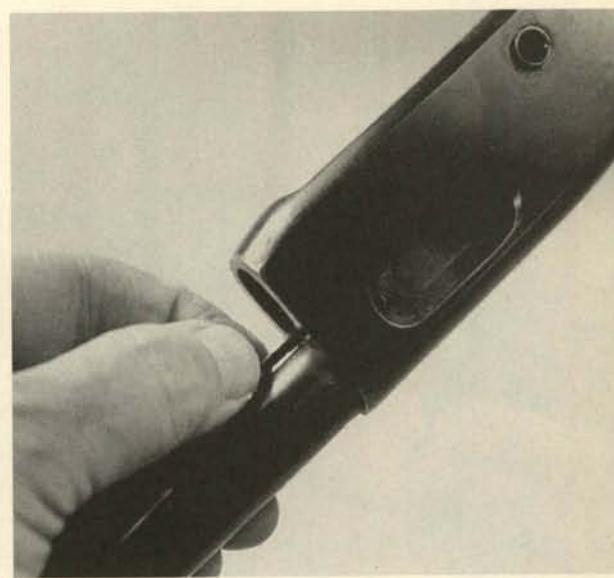
**11.** Lift the front portion of the cartridge guide and remove it toward the rear. **Caution:** Lift it only enough to clear its retaining recess.
