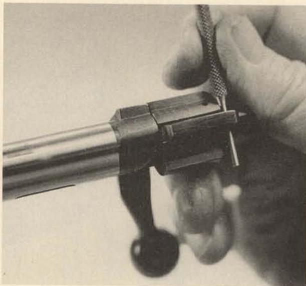
**3.** Remember to turn the bolt head back to cocked position, as shown, before the bolt is reinserted in the receiver.
