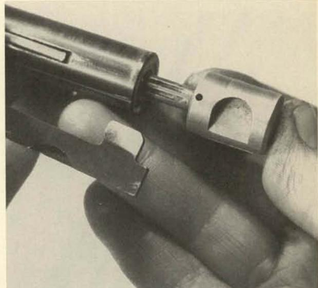
**14.** Remove the small screw on the underside of the front magazine tube hanger and slide the outer magazine tube out toward the front.
