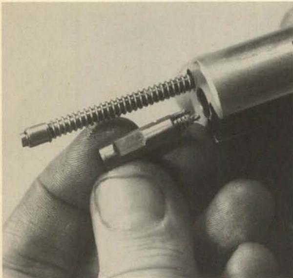
**17.** The ejector is mounted inside the firing pin, along with its spring, and they are retained by a cross pin at the rear of the firing pin. Push out the pin, while restraining the spring, and remove the ejector and spring toward the rear.
