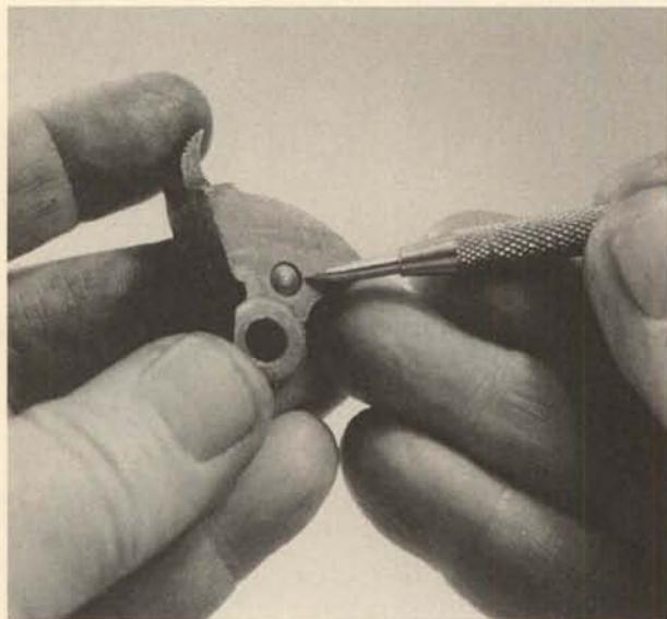
**7.** Drift out the firing pin cross pin. Remove the firing pin toward the rear.
