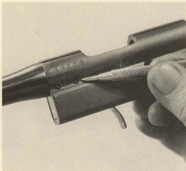
**31.** Two cross pins retain the barrel and the front insert block in the receiver. In normal takedown, these are best left in place. The rear sight is retained by two Phillips-type screws, and the dovetail-mounted front sight is drifted out toward the right.
