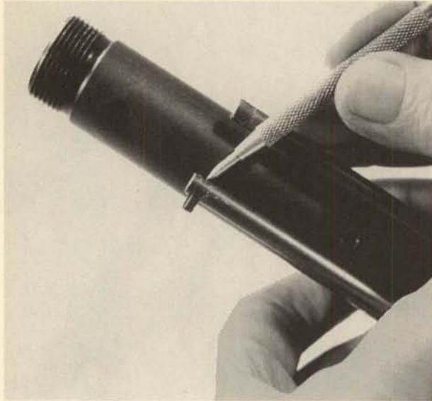
**14.** Remove the large Allen screw at the front of the lower receiver.
