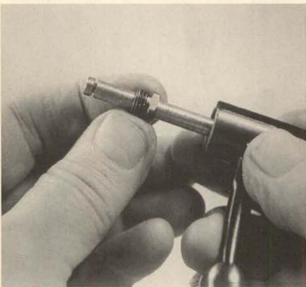
**7.** Remove the retaining nut toward the front.
