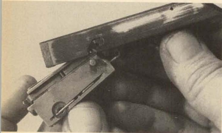
**3.** Separate the bolt from the bolt slide and take out the bolt cam pin which crosses the bolt at the rear. The cam pin does not fit tightly and can fall out, so take care that it isn't lost during disassembly.
