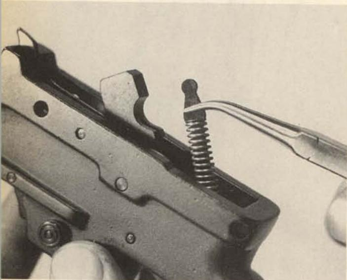
**10.** Restrain the hammer against the tension of its spring, pull the trigger, and ease the hammer forward beyond its normal fired position. The hammer spring assembly can now be moved forward and upward, out of the trigger group. The hammer spring assembly can be taken apart by compressing the spring and sliding the slotted washer off the lower end of the guide. Proceed with caution, as the spring is under tension.
