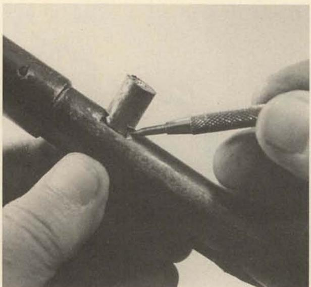
**12.** The stock mounting post and the front and rear sights are dovetail-mounted on the barrel. If removal is necessary, they are driven out toward the right.
