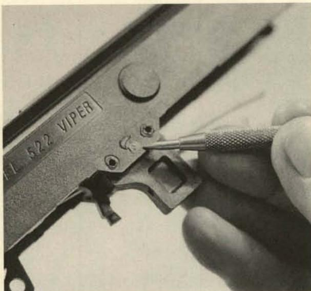
**11.** On the left side of the receiver, the sear pin is heat-sealed. For removal, the polymer must be softened with a small soldering iron. In normal takedown, this system should not be disturbed.
