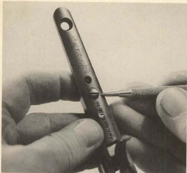
**15.** Remove the sear knock-off spring retaining screw and take out the spring.
