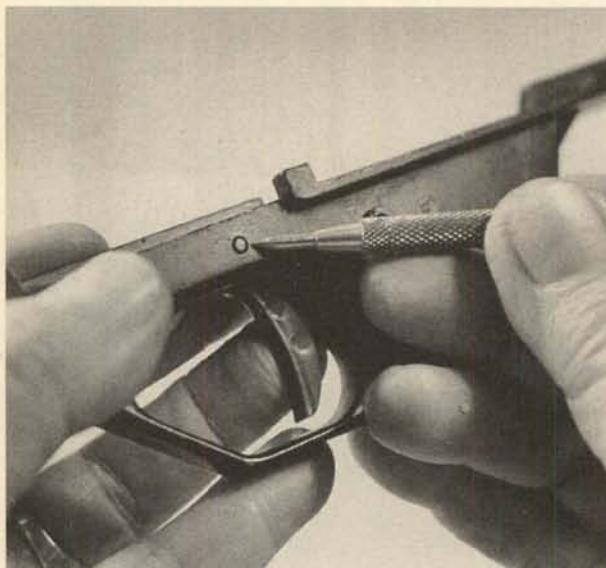
**29.** Drifting out the trigger cross pin will allow the trigger to be moved forward and turned down into the guard opening for removal.
