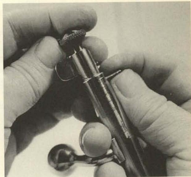
**4.** Viewed through the hole in the bolt body, use the slave pin as a guide to position the striker assembly for insertion of the bolt cross pin. The parts are shown here at the proper depth, but the slave pin head is a more precise guide.
