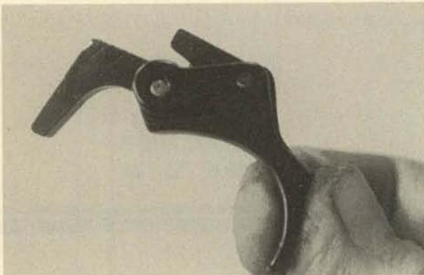
**2.** When replacing the hammer, its pivot bushings and the bolt latch spring, note that the spring must be on the right side of the hammer, as shown. Be sure the lower arm of the spring engages its notch in the cross-piece of the bolt latch. The upper arm of the spring goes below the cross pin that retains the ejector.
