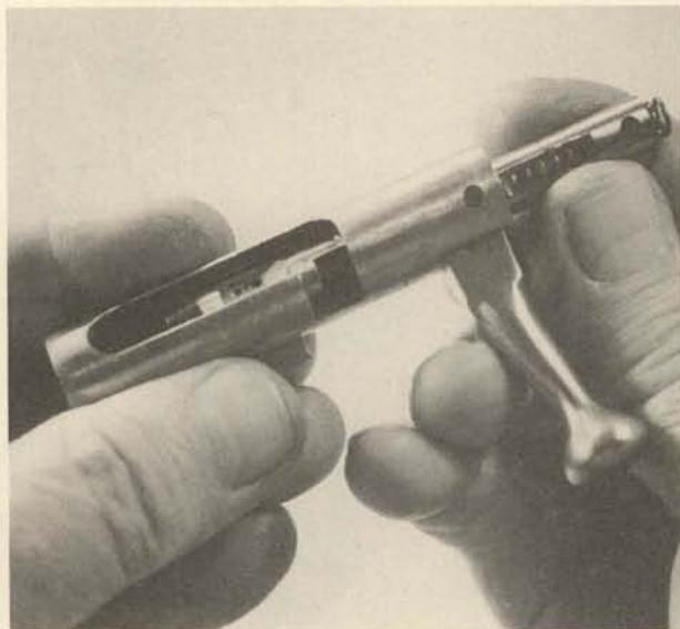
**16.** Remove the striker and spring toward the rear. The spring is easily removed from inside the striker.
