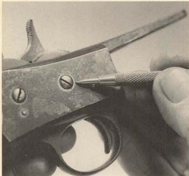
**6.** Tip the hammer to the rear and remove the breechblock upward. Remove the hammer upward.
