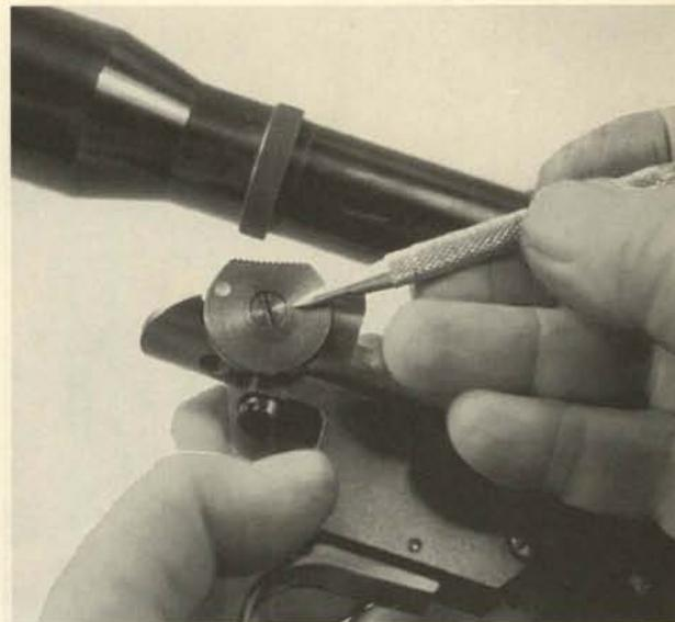
**16.** The safety disc need not be removed for further disassembly. However, if it is to be taken off, its pivot screw is the retainer.
