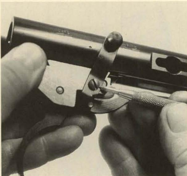
**18.** Restrain the trigger and push out the trigger pivot pin. **Caution:** Two small plunger-and-spring systems are mounted in the trigger, so control them.
