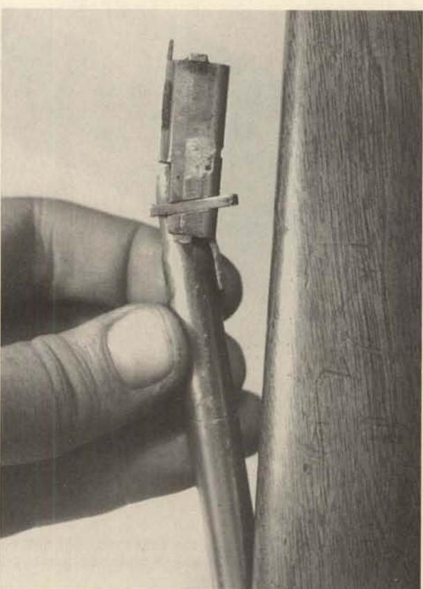
**15.** The outer magazine tube assembly can now be moved up and forward, out of the stock, and the trigger taken out upward.
