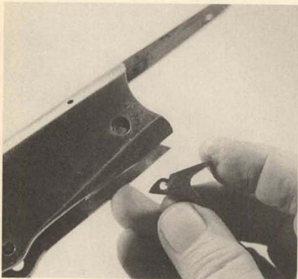
**22.** The barrel is threaded into the receiver and is also secured by a large cross pin. In normal takedown, this is left in place.
