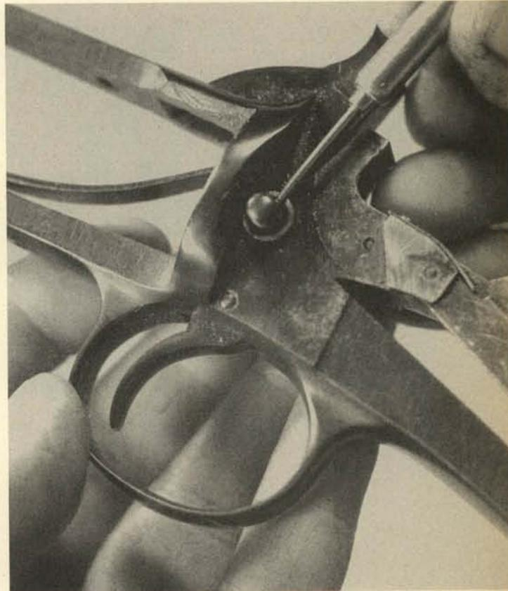
**4.** To remove the takedown cross screw, use a very small diameter drift punch to drive out the transverse pin near its left tip. To make the pin accessible, the takedown screw must be moved as far toward the right as it will go. After removal of the pin, the screw is removed toward the left.
