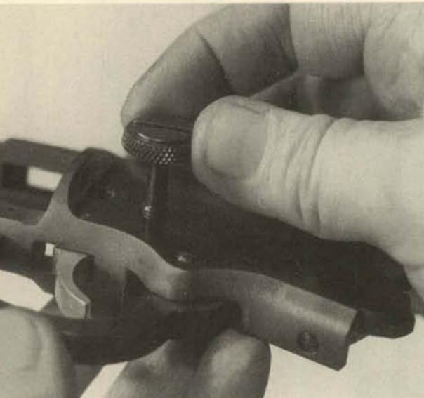
**14.** Move the takedown screw over until its threads engage the threads in the right side of the receiver, and unscrew it toward the right side for removal.
