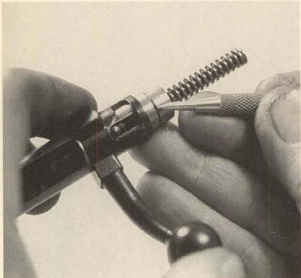
**6.** After the retainer tip is in place, turn the end piece counterclockwise (rear view) to feed the retainer back into its internal groove.
