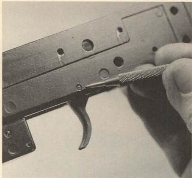
**34.** Remove the trigger assembly upward, moving it slightly rearward to clear it from the sear. The cross pin can be removed to separate the trigger bar from the trigger, and the spring is easily detached from the rear tip of the bar.
