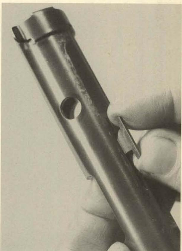
**16.** The ejector is easily pushed from its slot in the underside of the receiver for removal.
