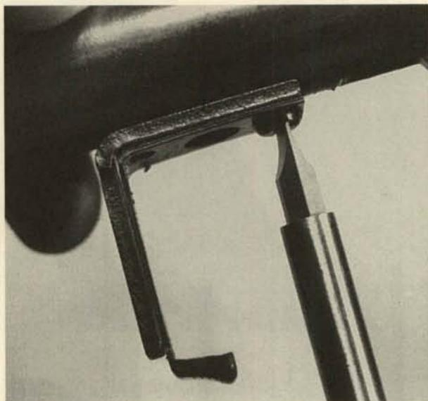
**14.** Remove the trigger and its spring downward.
