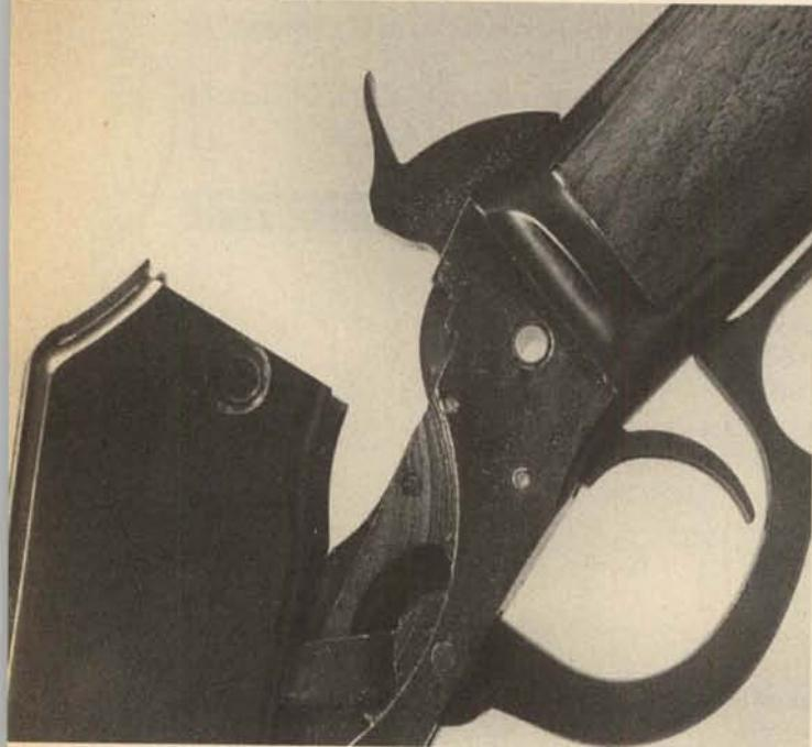
**2.** Remove the bolt assembly from the receiver toward the rear.
