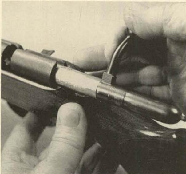
**2.** Remove the screw at the front of the trigger and magazine plate.
