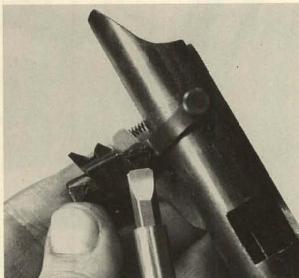
**15.** Restrain the sear and remove the screw on the right side of the receiver. Remove the safety-lever toward the right.
