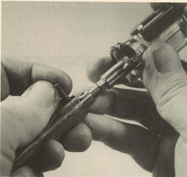
2. When installing the bolt detent plunger, note that its smaller tip goes toward the rear.
