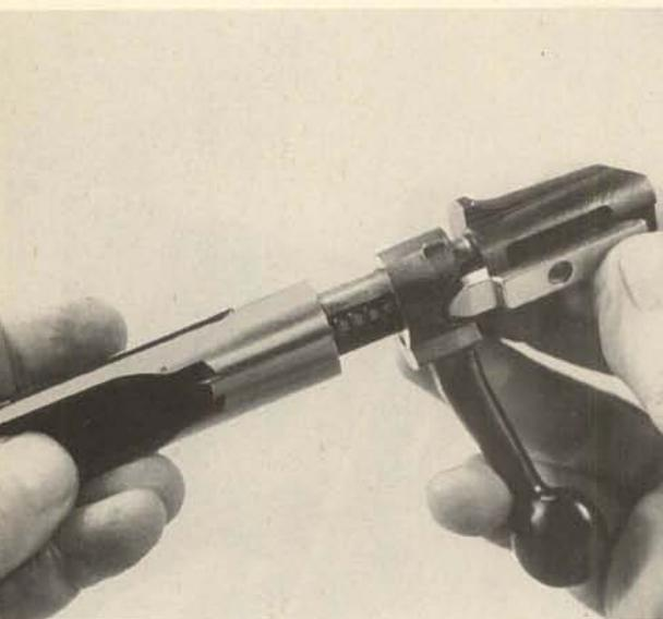
**26.** Remove the end piece and striker assembly toward the rear.
