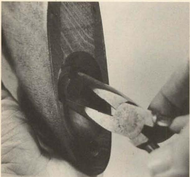
**15.** Once the nut is freed, an opened sharp-nosed plier can be used to unscrew it.
