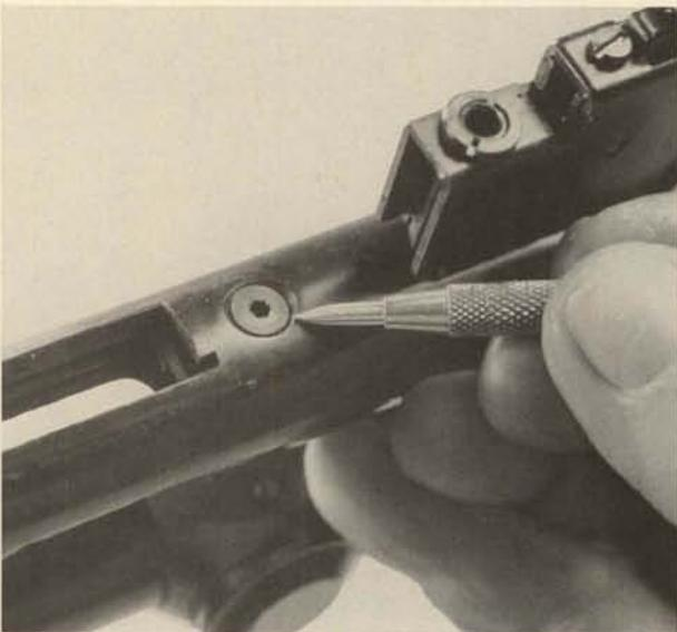
**21.** Removal of the trigger housing will require a twin-point tool, made to fit the recesses in the cap nuts at front and rear.
