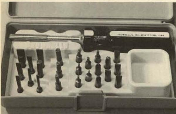
**2.** When a larger screwdriver is needed, this set from Brownells covers a wide range of blade sizes and also has Phillips- and Allen-type inserts. The tips are held in place by a strong magnet, yet are easily changed. These tips are very hard. With enough force you might manage to break one, but they'll never bend.
