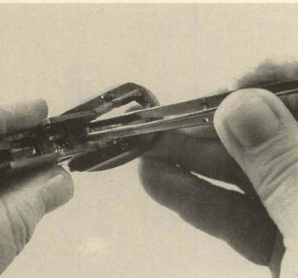
**18.** Remove the combination trigger and carrier spring and plunger from their well in the top of the trigger.
