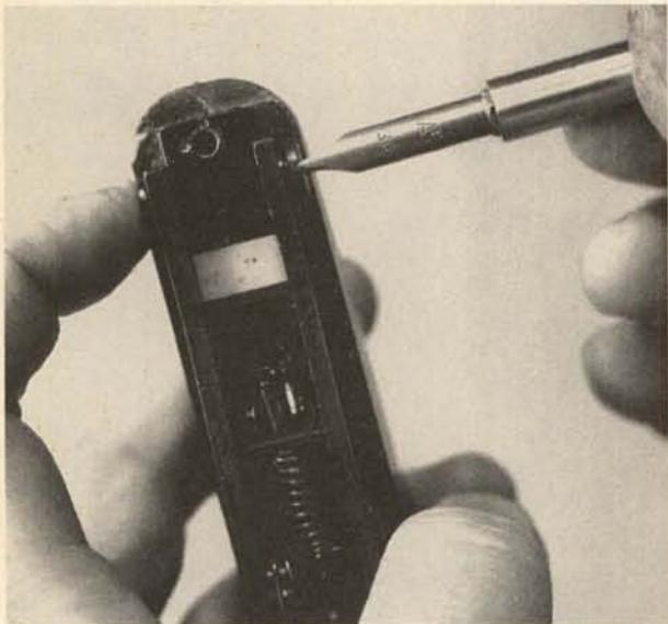
**6.** Remove the two opposed screws at the front of the sub-frame below the receiver.
