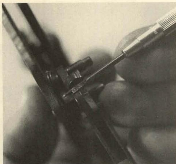
**17.** Disengage the lever latch spring from the back of the lever latch and allow the spring arm to swing forward, releasing its tension.
