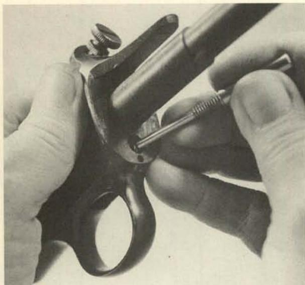
**27.** Use a tool to push the trigger spring out toward the front, into the receiver, for removal. **Caution:** Lay a shop cloth over the lower receiver to arrest the spring as it is freed.
