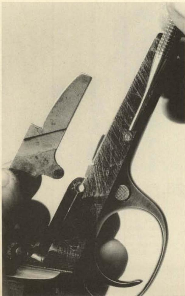
**18.** Restrain the hammer against the tension of its spring and carefully remove the pin or drift from the hole in the rear tip of the spring guide. Ease the hammer off forward and upward, along with its guide and spring. The spring is easily removable from the guide, but the cross pin that attaches the guide to the back of the hammer is usually riveted in place, and in normal takedown it is best left on the hammer.
