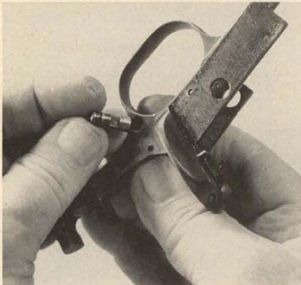
**2.** When installing the safety plunger and spring, insert a small tool to depress the spring as the cross pin is reinserted.
