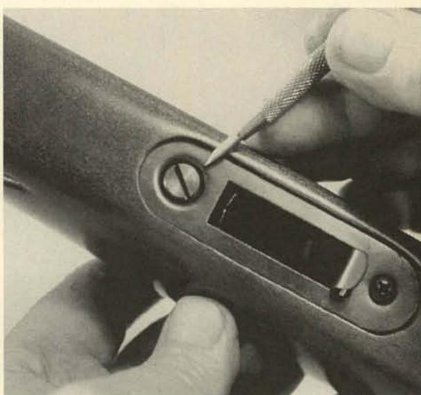
**13.** Remove the stock mounting screw and take the action out of the stock. The trigger guard, guard plate, magazine plate and the stock buttpiece are each retained on the stock by Phillips-type wood screws.
