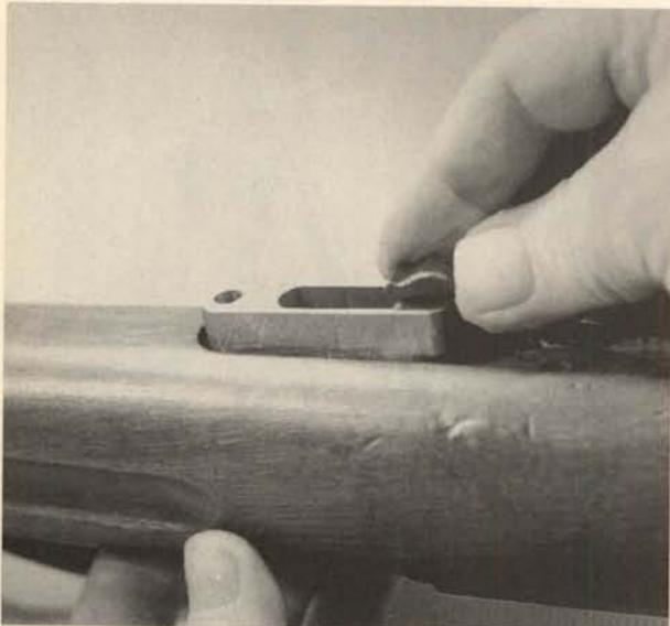
**10.** Drifting out this cross pin will allow removal of the magazine catch and its spring from the housing.
