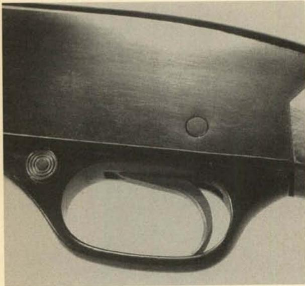
**2.** Tip the trigger housing down at the rear and move it slightly toward the rear to disengage its forward stud from its recess inside the receiver. Remove the trigger group downward.
