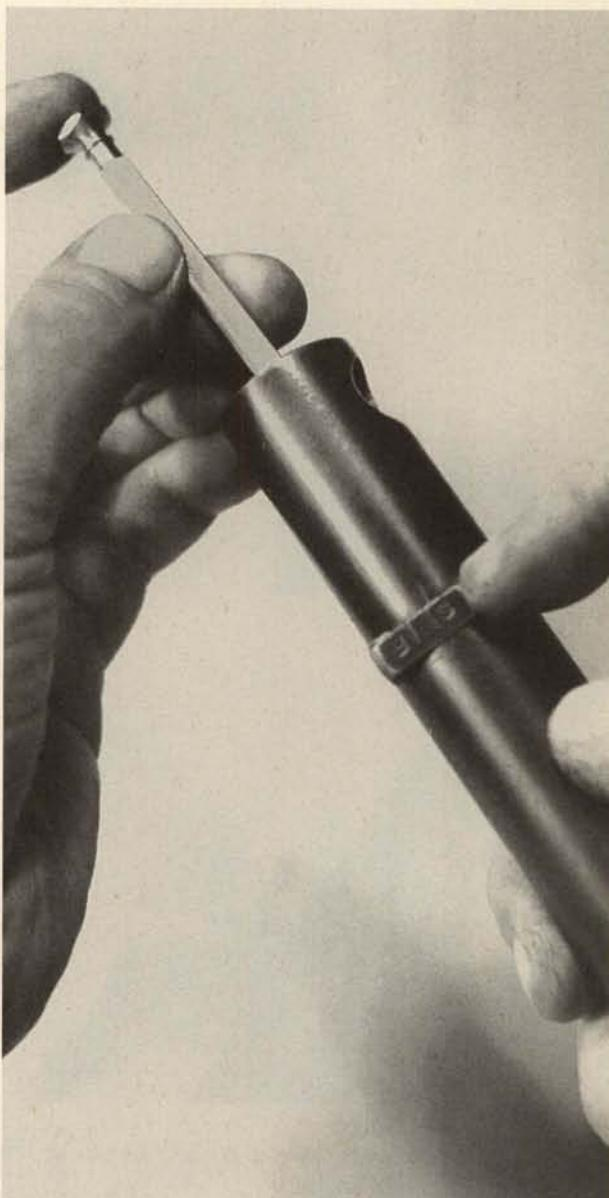
**13.** The cartridge feed guide is retained by a single cross pin on the underside of the receiver. After the feed guide is removed, the twin cartridge stops are easily detachable from it by swinging them outward on their fixed pins and removing them toward the rear.
