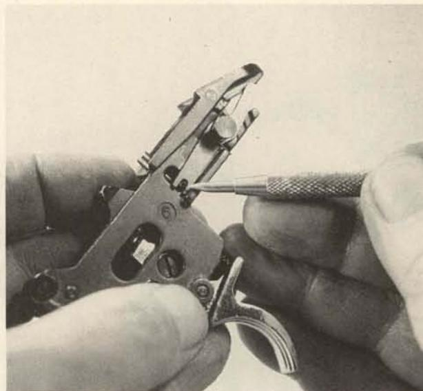
4. When installing the safety-lever, be sure its front fork engages the bolt lock side pin, as shown. After the post is drifted into place, remember to rehook the spring under the lever at the rear.
