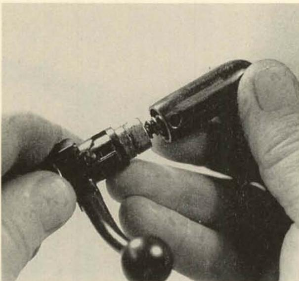
**10.** When the end of the retainer is cleared, remove it. Ease the spring tension and take off the end piece toward the rear.
