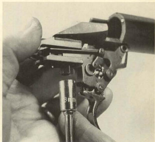
**8.** Remove the trigger housing downward.
