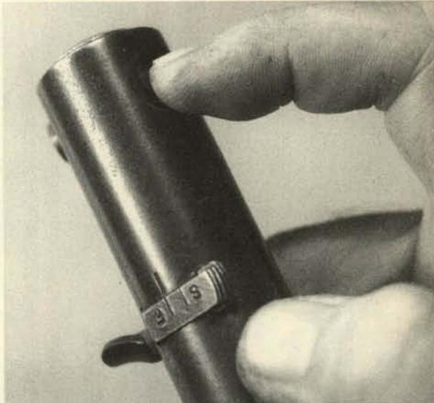
3. While holding the latch to the right, withdraw the bolt and firing mechanism assembly from the rear of the receiver.
