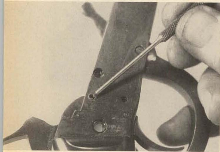
**11.** Use a roll pin punch to drift out the hammer stop pin, located just forward of the hammer. Set the hammer on its safety step while the stop pin is drifted out.
