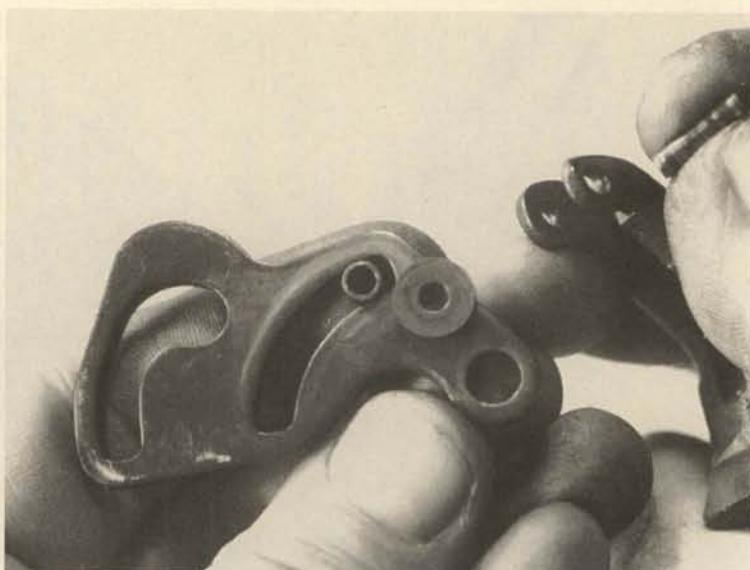
**23.** Remove the C-clip on the inside tip of the carrier pivot and take out the carrier pivot toward the left.
