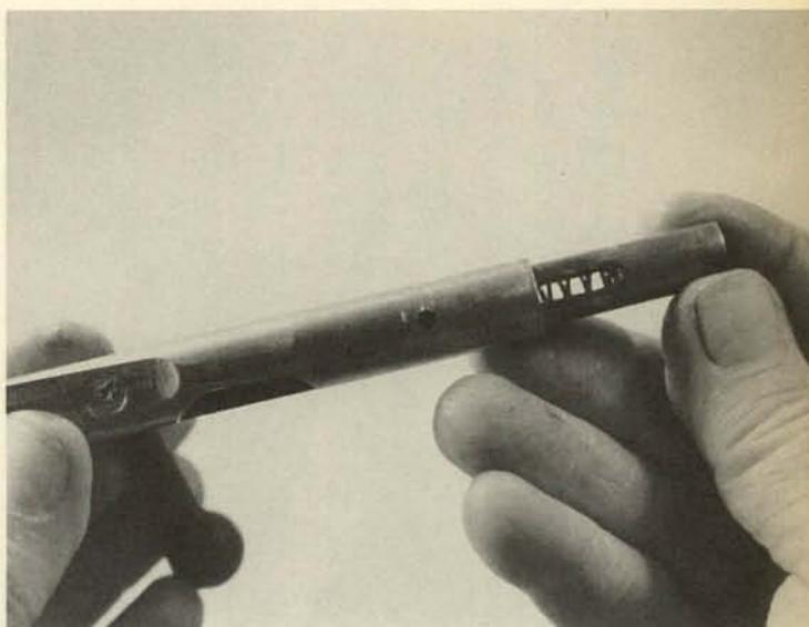
8. Remove the striker assembly toward the rear. The spring is easily removed from inside the striker.
