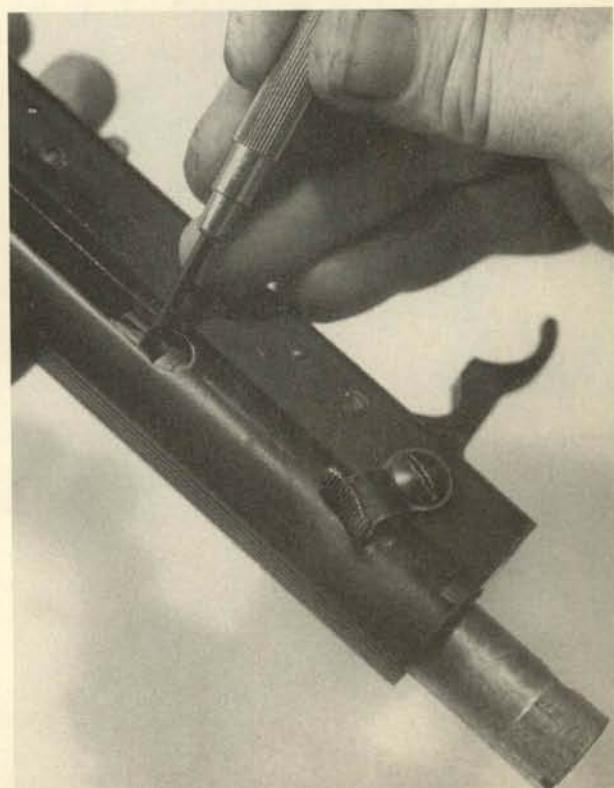
5. Remove the striker (firing pin) from the rear of the bolt.
