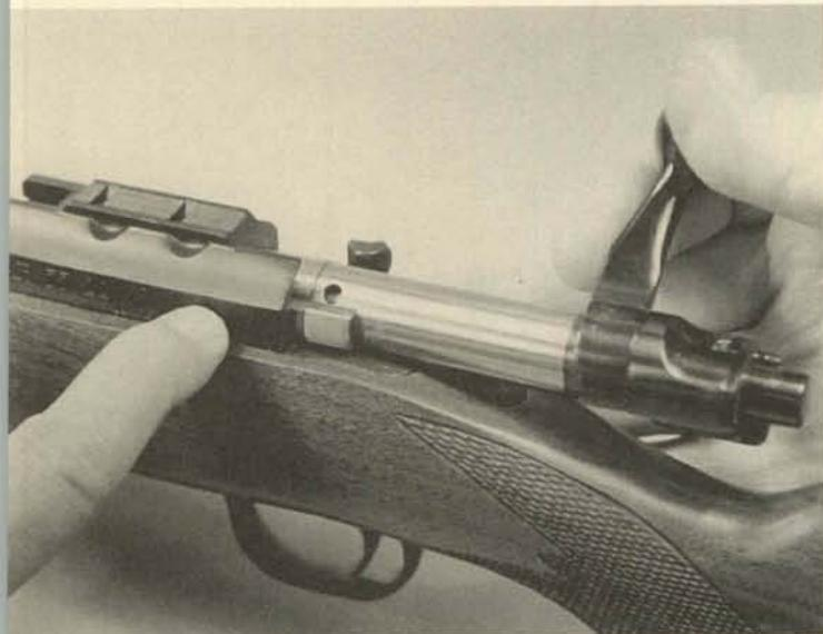
**2.** Insert a drift through the hole in the underlug of the striker end piece and turn the bolt headpiece to the position shown.
