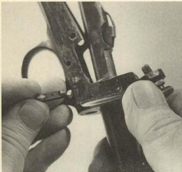
**2.** The trigger spring must be inserted through the trigger guard, and a tool is used to push it back into its tunnel. The proper orientation is shown. You will know it is properly in place when its rear bends are visible at the back of the lower receiver (see step 27).
