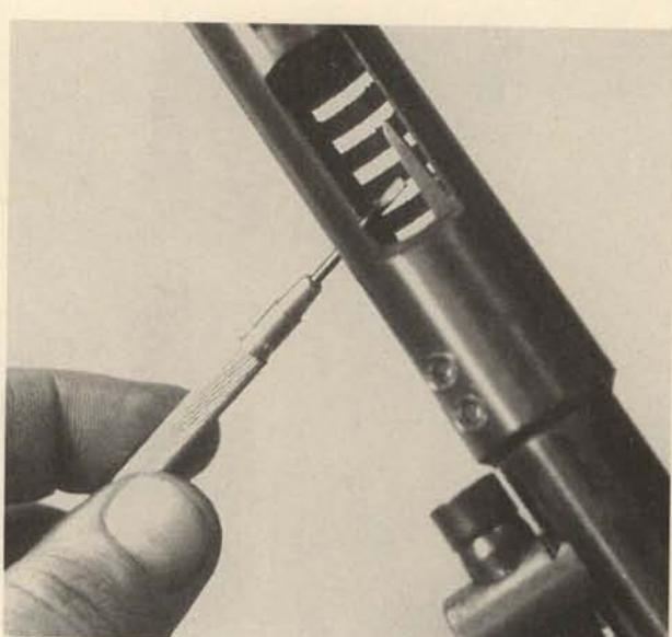
**19.** The cartridge guide, mounted inside and above the chamber, is removable only when the barrel is taken out. There is also a small coil spring mounted in a recess in the roof of the receiver, above the guide.
