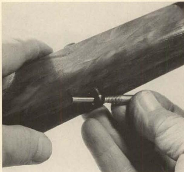
**7.** To remove the forend from the barrel, insert a drift through the hole in the sling stud and unscrew it, as shown.
