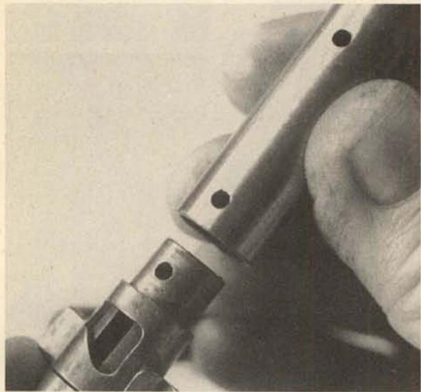
**10.** Restrain the extractor plunger and spring, and remove the extractor from its recess. Ease out the plunger and spring.
