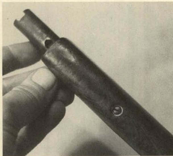
3. The forend is held on the underside of the barrel by a single screw.
