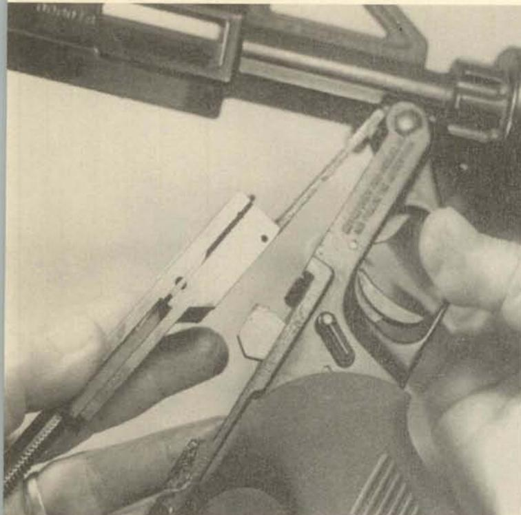
**9.** Remove the ejector from its recess in the top of the bolt.
