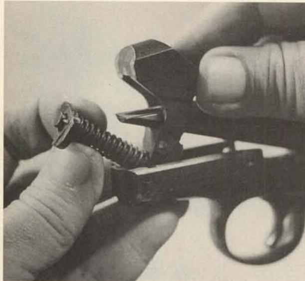
**23.** Remove the hammer and spring assembly toward the front. Pressing the spring base against a slightly opened vise and removing the keeper pin will allow the base and spring to be taken off the guide. **Caution:** The spring is under tension. The guide pivot pin can also be removed to take the guide off the hammer.
