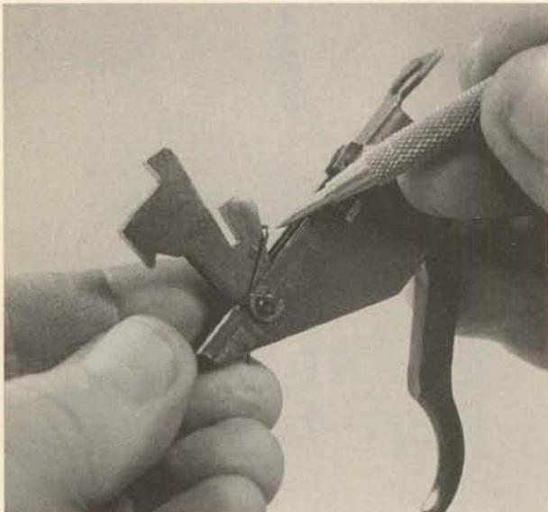
**2.** A large screwdriver bit and a small hammer will make replacement of the safety retainer easier, as shown.
