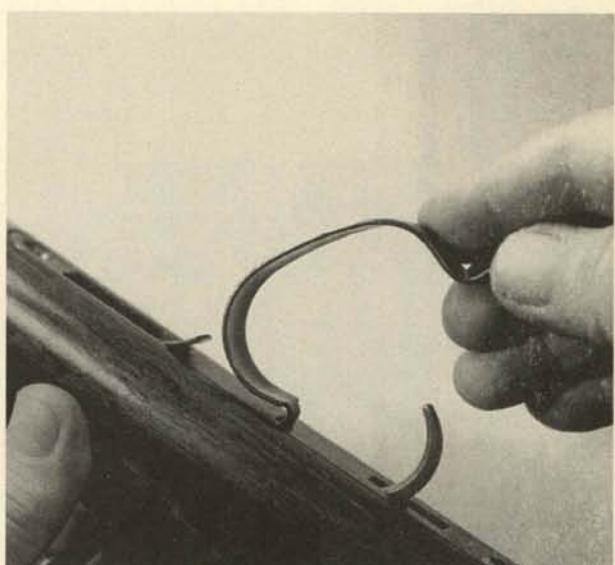
**4.** Tip the trigger guard forward and remove it.
