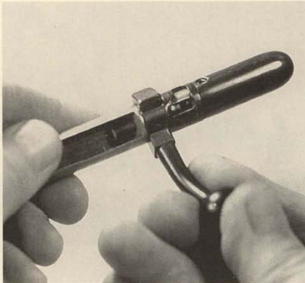
**7.** Grip the forward portion of the bolt firmly and turn the bolt to lower the striker to fired position, as shown.
