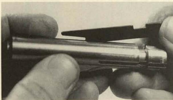
**12.** The extractor spring also retains the firing pin, and it can now be removed from its recess in the top of the bolt.
