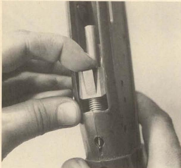
**10.** Push out the cross pin located in the receiver just above the forward end of the trigger guard (arrow). Tip the trigger guard downward at the front, disengage its rear hook from inside the receiver, and remove the guard downward.
