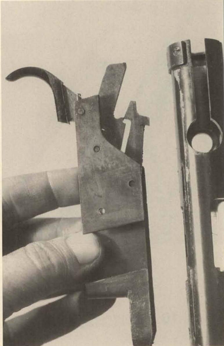
**13.** Push out the cross pin at the top of the magazine housing, and remove the sear upward and toward the front.
