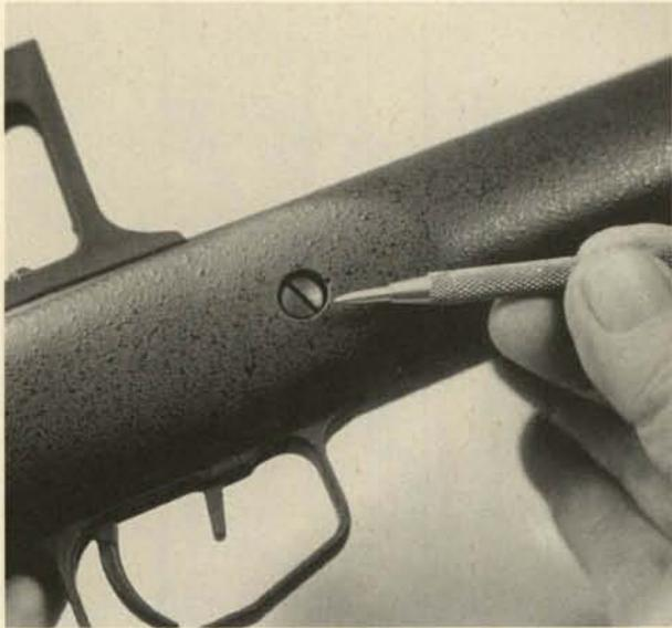
**2.** Remove the screw at the rear, between the port cover and the buttpiece.
