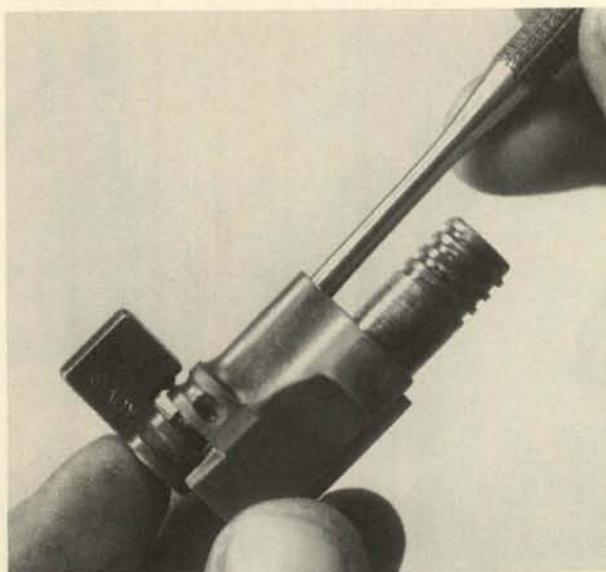
**19.** To remove the safety from the bolt sleeve, turn the lever up to central position and use a drift punch against the front tip of its pivot shaft, as shown, to nudge it out toward the rear. **Caution:** As the small plunger and spring inside the safety-lever clear the rear top of the sleeve, they will be released downward. Restraine them, and take care they aren't lost.
