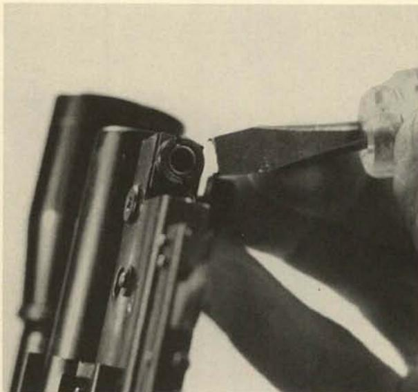
**22.** Remove the bolt stop by pushing its retaining clip off the post. Control the clip as it is freed from the post.
