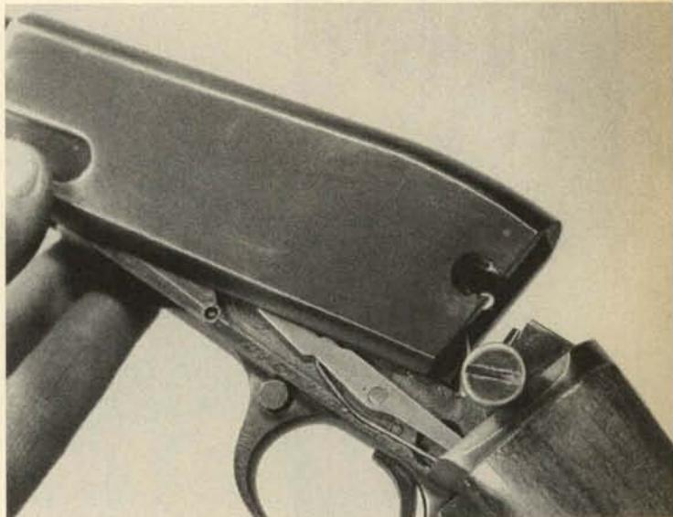
3. With the front section of the gun inverted, move the breechblock (bolt) all the way to the rear and depress the retaining spring, located in a slot inside the right wall of the receiver. Move the bolt forward and upward, disengaging its side lug from the action slide bar; then move the bolt toward the rear.
