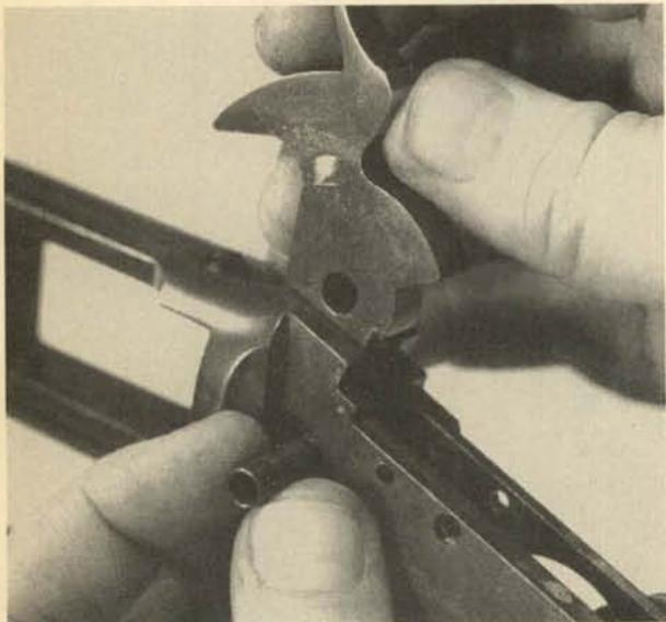
**14.** With an Allen wrench of the proper size, take out the screw that retains the lever tension spring and its plate, and remove the plate and spring upward.
