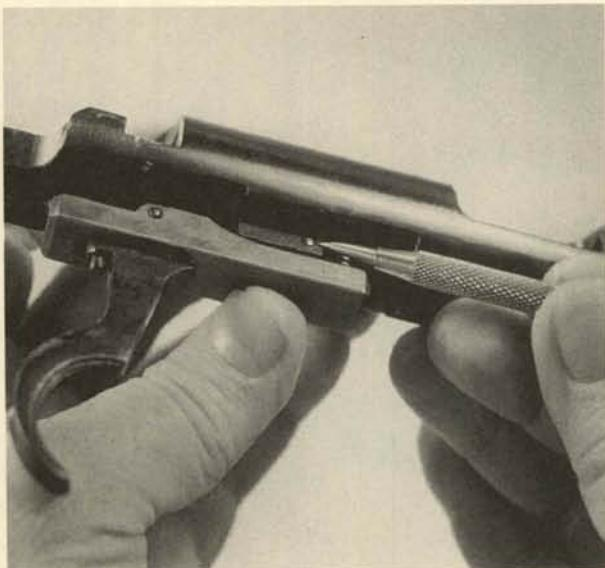
**14.** Ease the spring tension slowly, and remove the trigger and sear assembly downward.
