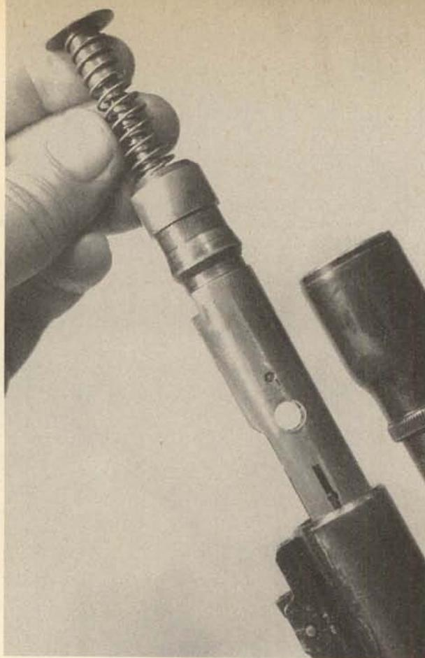
5. Remove the bolt assembly from the rear of the receiver.
