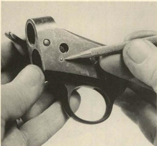
**10.** Remove the ejector upward.
