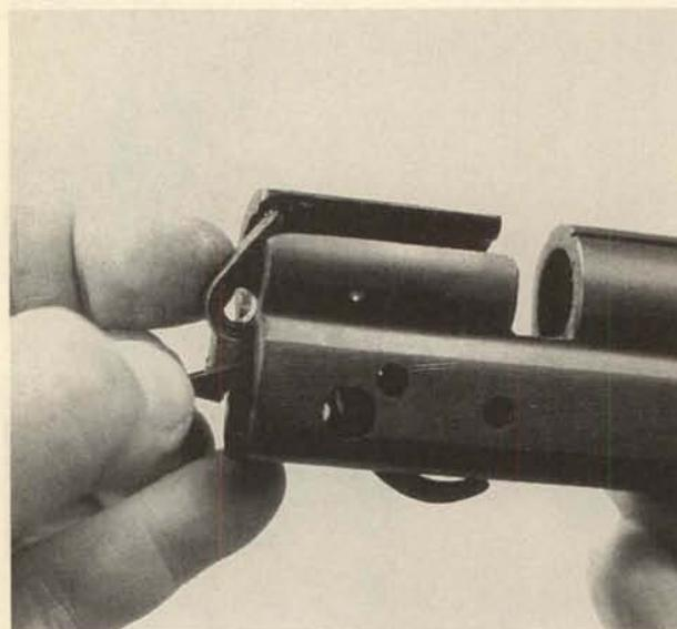
**22.** Move the trigger inward and toward the rear for removal, along with the disconnector slide.
