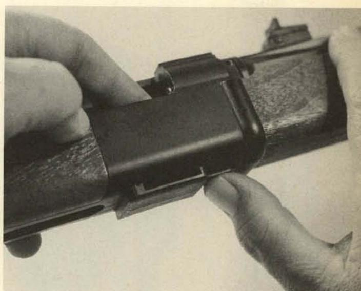
4. Operate the latch and push the magazine downward out of the receiver.
