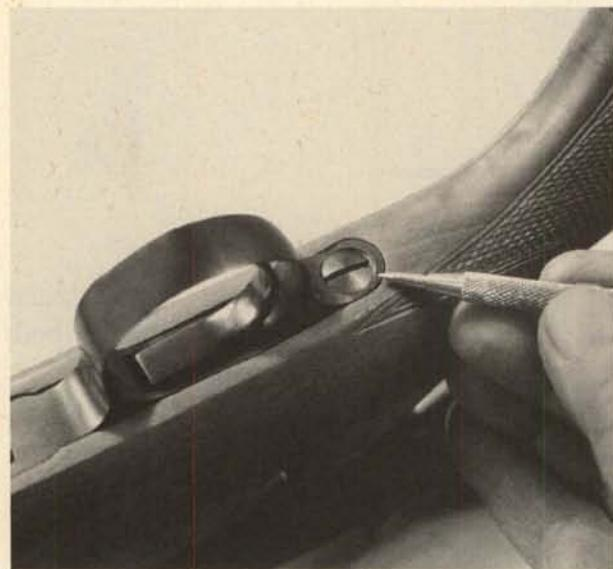
**3.** Remove the large screw behind the trigger guard. Keep the two screws in order, as they are not interchangeable.
