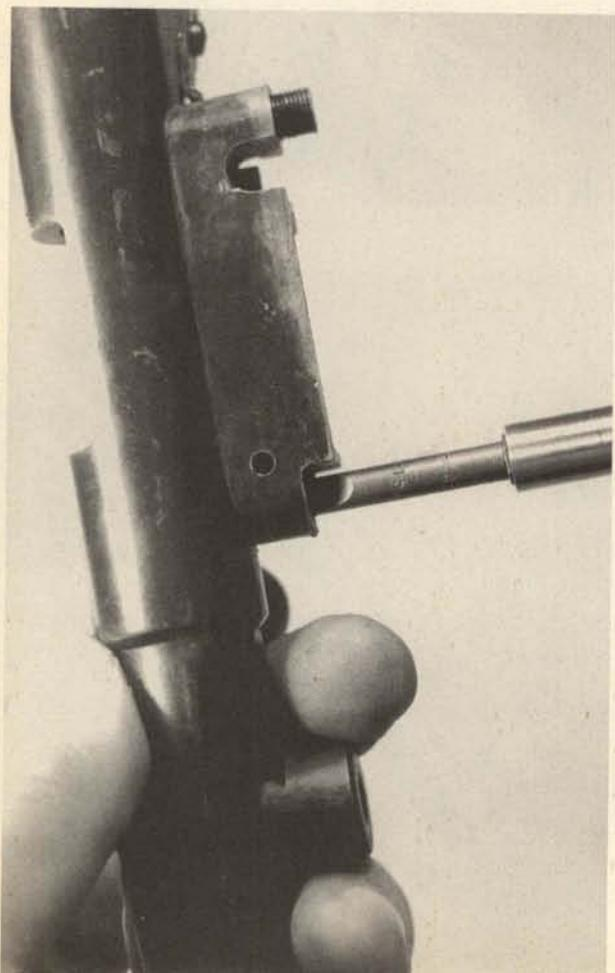
**12.** Remove the front magazine housing screw.
