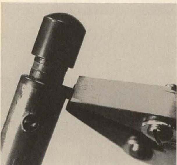
3. The striker must be cocked before the bolt is put back into the receiver. Grip the cam pin with non-marring pliers and turn the bolt clockwise (rear view) until the cam pin engages its notch at the rear of the bolt.
