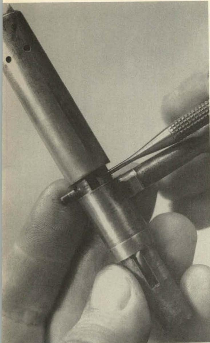
8. Move the bolt handle sleeve back forward, against its shoulder on the bolt, and turn it until the widest part of its internal opening is aligned with the firing pin on the underside of the bolt. Then, move the firing pin all the way to the rear, tip its rear end downward and remove it from the bolt. The clearances are very close here, so proceed with care.
