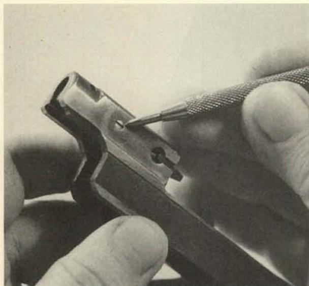
**11.** Remove the extractor plunger stop screw.
