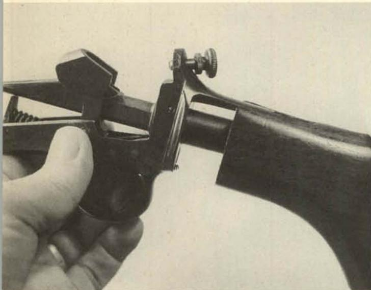
**18.** Remove the safety detent plunger and spring toward the rear.
