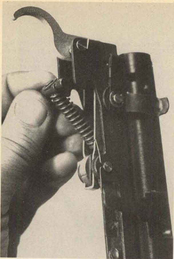
**8.** Insert a tool inside the receiver to restrain the hammer, depress the sear lock on the right side, and pull the trigger. Ease the hammer down to the fired position. Push the hammer spring base out of its recesses in the front of the trigger housing, and remove the base and hammer spring assembly downward. The hammer spring assembly can be taken apart by removing the C-clip behind the base. **Caution:** The spring is under compression. Control it, and ease it off.
