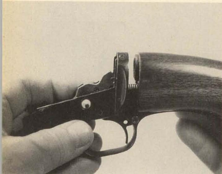
**15.** Move the safety to off-safe position. Insert a small tool or keeper pin in the cross hole in the hammer spring guide and pull the trigger, easing the hammer forward until the spring is trapped.
