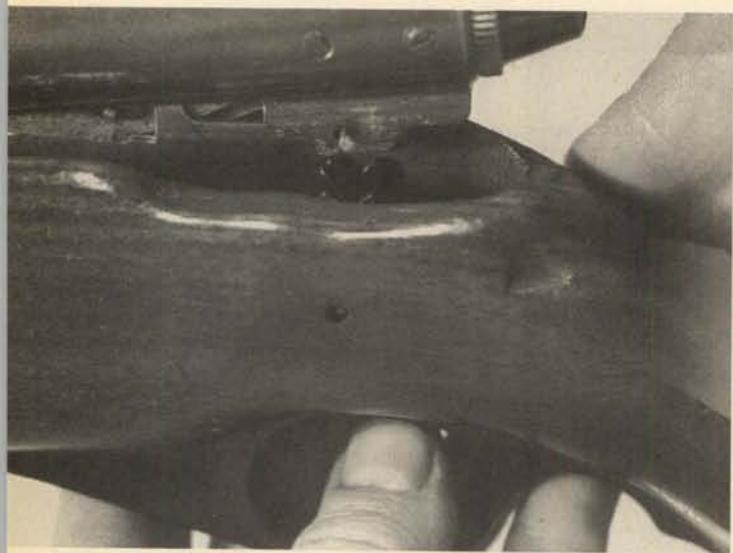
**4.** When replacing the action in the stock, pull the trigger very slightly to be sure its upper extensions properly engage the cross pin in the disconnector.
