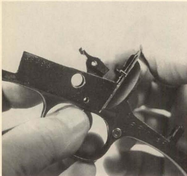
**21.** Drift out the cross pin that retains the safety detent plunger and spring. **Caution:** When the drift is withdrawn, the spring will be released, so control it.
