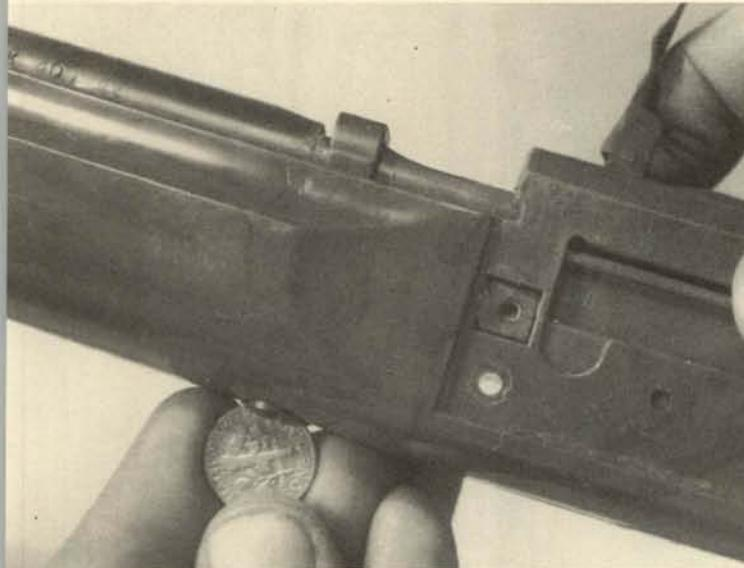
**6.** The front sight is retained on top of the barrel by two screws, one at each end.
