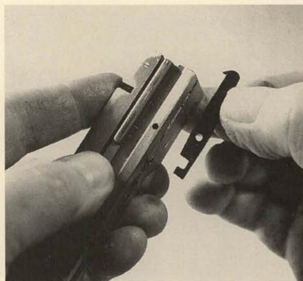
**15.** Remove the extractor from its recess.
