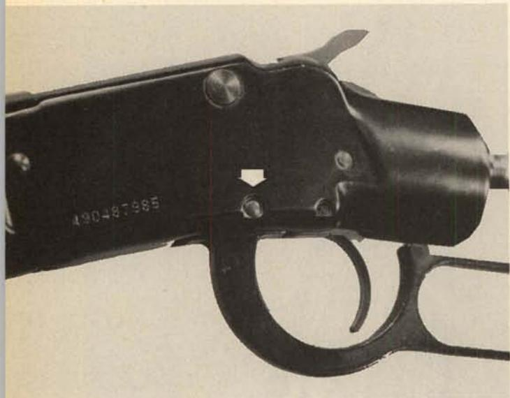
**5.** Remove the lever downward, and remove the trigger spring and plunger from the back of the lever base.
