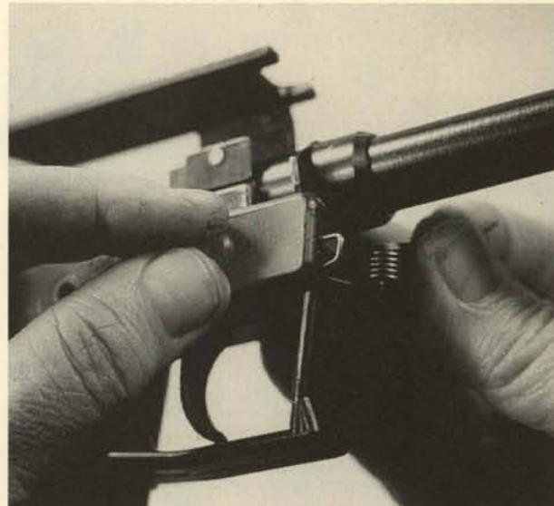
**2.** Fit the long loop of the stock latch spring onto the right front screw. Use a tool to hold it in place, and tighten the screw, with the nut retaining the spring.
