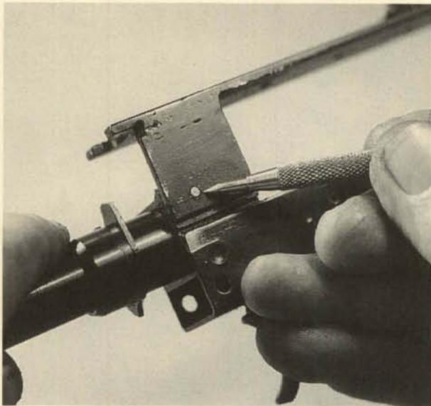
**36.** Drifting out this cross pin will allow the trigger to be taken out downward. **Caution:** The trigger spring will be released. The trigger bar is turned upward to follow the trigger out.
