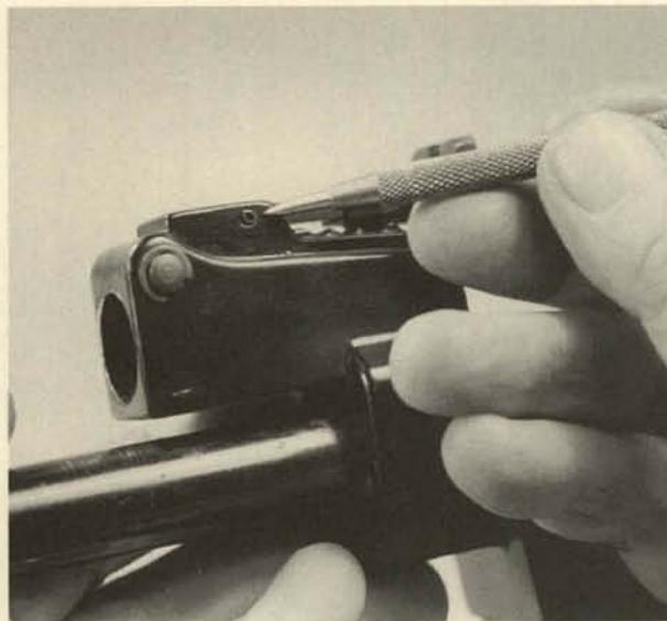
**39.** The rear sight is retained by a roll-type cross pin. The latch at the front of the sight base is a cosmetic part. If it needs to be removed, the C-clip on the left side is taken off, and the latch is removed toward the right.
