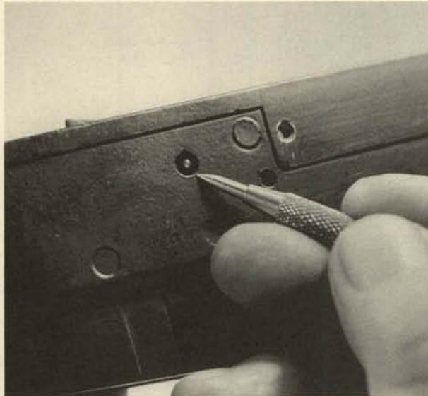
**38.** If all parts have been taken off the barrel, and all parts removed from the receiver, removal of this Allen screw will allow the barrel to be driven out of the receiver toward the rear. In normal takedown, it is best left in place. The cleaning rod spring, visible at the front of the receiver, can be taken out of its well if necessary.
