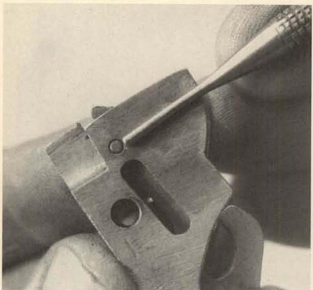
**19.** Drifting out the cross pin at the front of the carrier will free the cartridge stop for removal toward the front.
