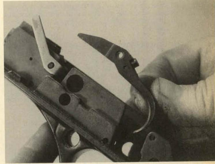
**18.** The right rear tail of the hammer spring retains the safety, and the safety can now be turned slightly and removed toward the left.
