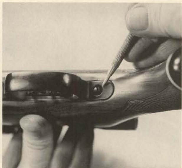
**12.** Remove the screw behind the trigger guard.
