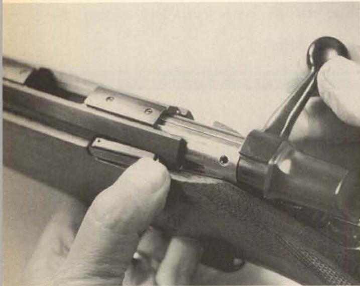
**2.** Remove the stock mounting bolt, located just forward of the magazine well.
