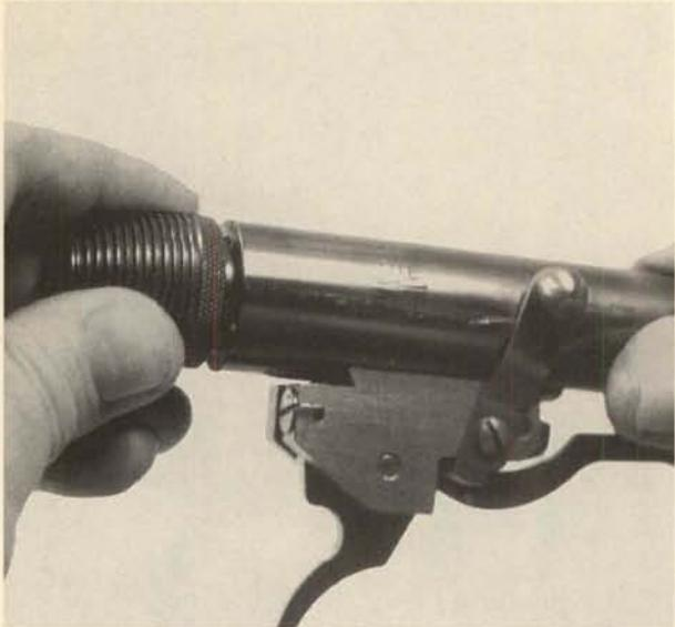
**6.** Remove the end piece toward the rear. In normal takedown, the nylon buffer is not removed from the end piece.
