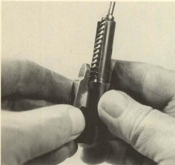
**29.** The striker, its spring, and the collar at the rear can be separated from the cocking piece by drifting out the roll cross pin. **Caution:** The captive spring is still under tension. Except for repair, this system should be left intact.
