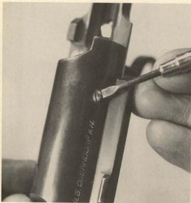
**10.** Remove the vertical screw at the left rear of the receiver, the pivot and retaining screw for the bolt stop. Slight inward pressure on the stop will ease removal of the screw.
