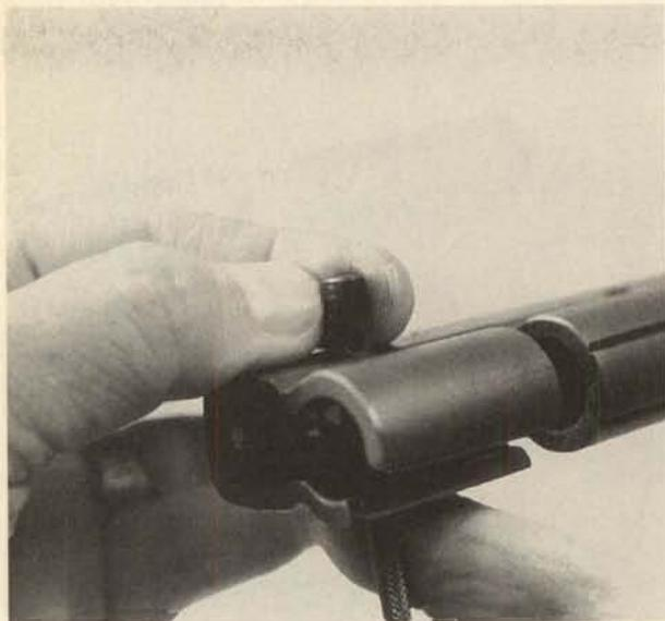
**21.** Push out the trigger cross pin.
