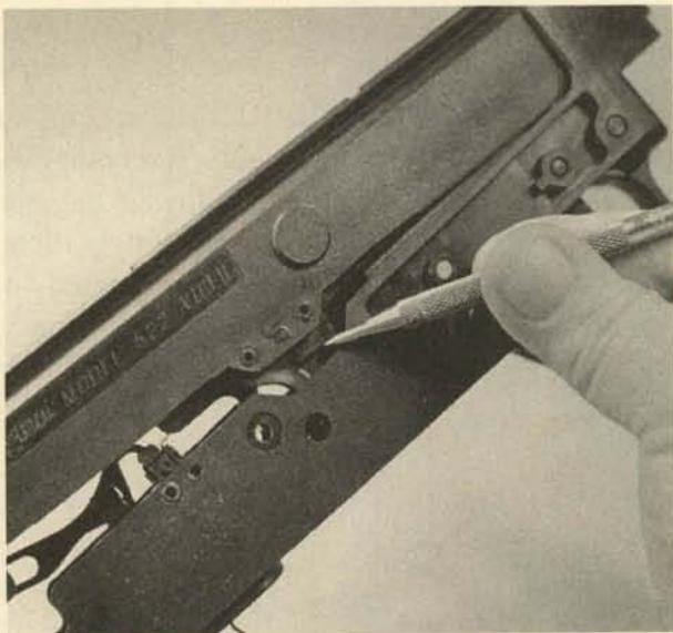
**2.** With the springs properly engaged, move the lower housing forward and upward until its latch at lower front engages. There is an assembly guide on the left side of the receiver that helps in proper placement.
