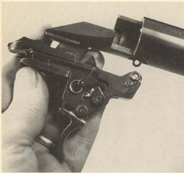
**9.** The bolt latch can be removed from the left side of the receiver by backing out its retaining and pivot screw. Restraine the latch as the screw is taken out, and ease it off. Remove the spring. In the front of the latch, a vertical roll pin retains the bolt stop/guide pin.
