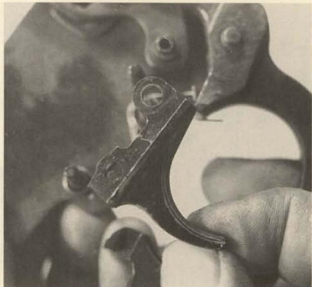
**21.** Move the lever and lever cam plate off their posts toward the right. The cam plate may be tight and will have to be worked and pried gently off.
