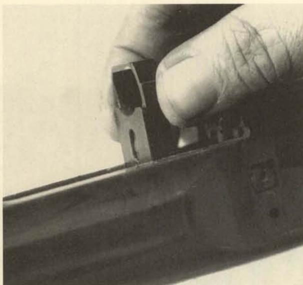
**7.** Take out the cross-slotted screw from the bottom of the stock, and lift the barrel retainer and its front plate out of their recess in the top of the stock.
