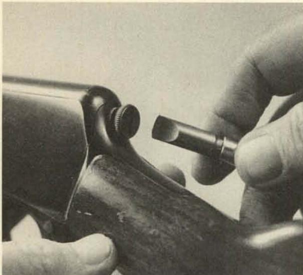
**2.** Separate the buttstock and trigger group assembly from the receiver, moving the assembly straight toward the rear. Tight fitting may require the use of a rubber mallet for initial separation.
