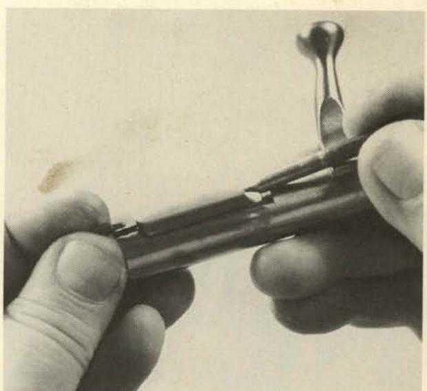
**13.** Drift out the cross pin that retains the cocking knob. When the drift is withdrawn, control the knob, as it is under tension of the rebound spring.
