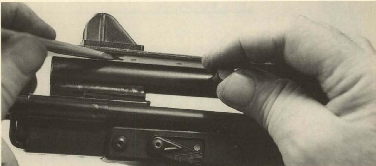
**9.** As the bolt assembly is reinstalled, it must be depressed downward to properly engage the rails, working against the tension of the hammer spring. This is easily done by using a large screwdriver at the top, as shown.
