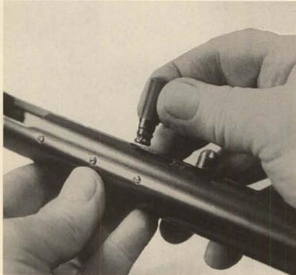
**14.** Pull the trigger and remove the bolt toward the rear.
