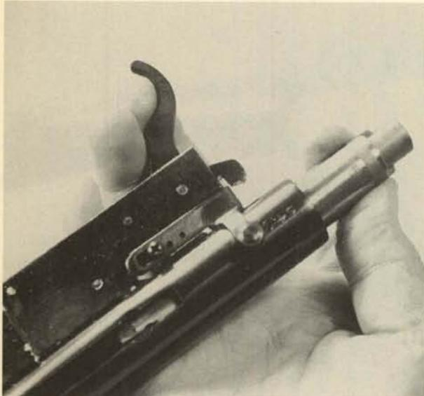
**10.** The striker (firing pin) is easily removed from the top of the bolt.
