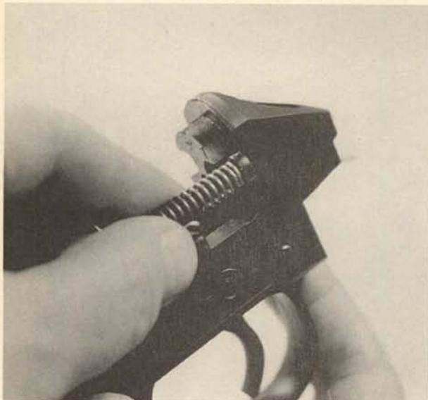
**6.** Move the bolt all the way to the rear and take out the striker assembly. The combination striker and firing pin unit is retained in the red polymer headpiece by a roll-type cross pin. Except for repair purposes, this system should be left in place.
