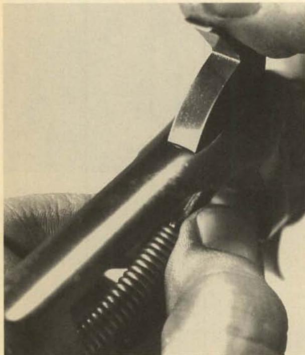
**3.** When replacing the hammer strut and spring, guide the spring at the rear to position the rear tip of the strut in alignment with its hole in the rear vertical bar of the trigger group. Be sure the front tip of the strut enters its recess on the rear of the hammer as the hammer is drawn back to the safety step.
