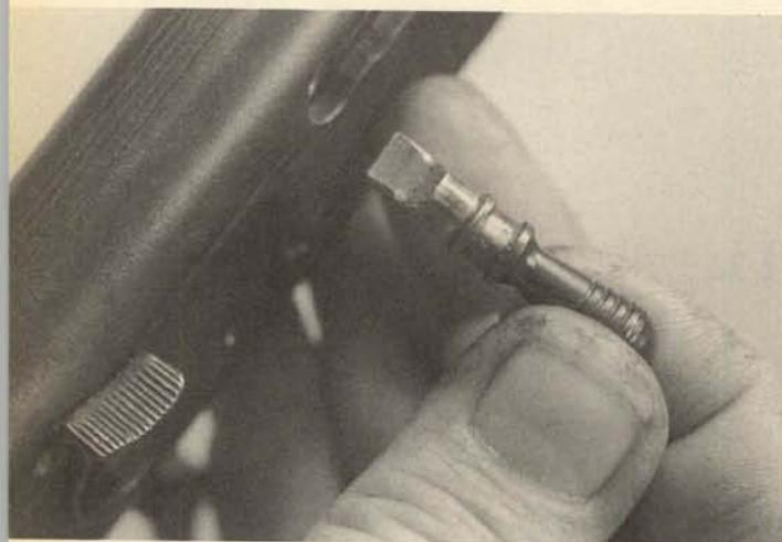
**2.** When replacing the bolt handle, be sure the flat inner tip of the handle is at the top, as shown. Also, be sure the carrier is in its raised position (up at the front) before inserting the bolt in the receiver.
