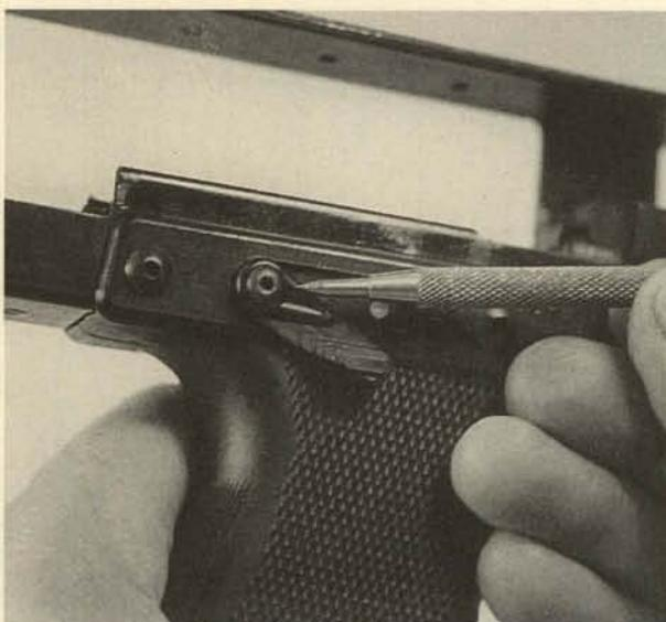
**22.** Restrain the hammer and push out the safety cross-piece, which is also the hammer pivot.
