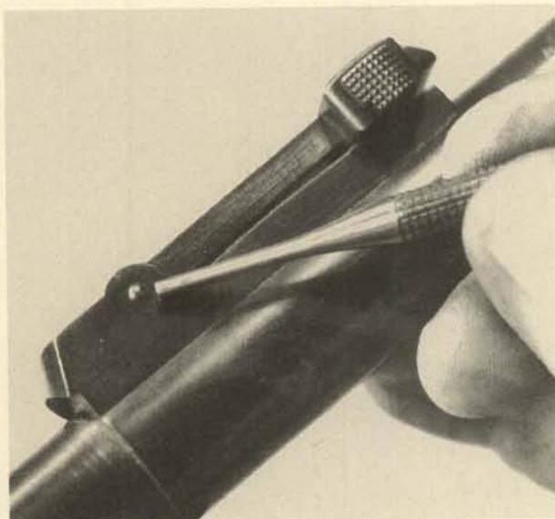
**14.** The rear sight is retained on its base by a cross pin. After the sight is removed, the elevation slide can be moved forward and off the sight.
