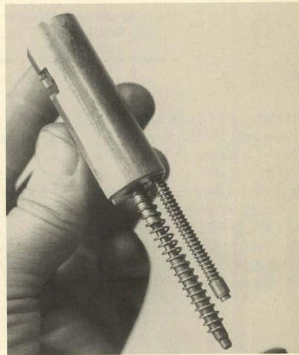
**3.** Replacement of the striker and its spring will be easier if they are placed in their hole in the rear of the bolt and inserted with the bolt.
