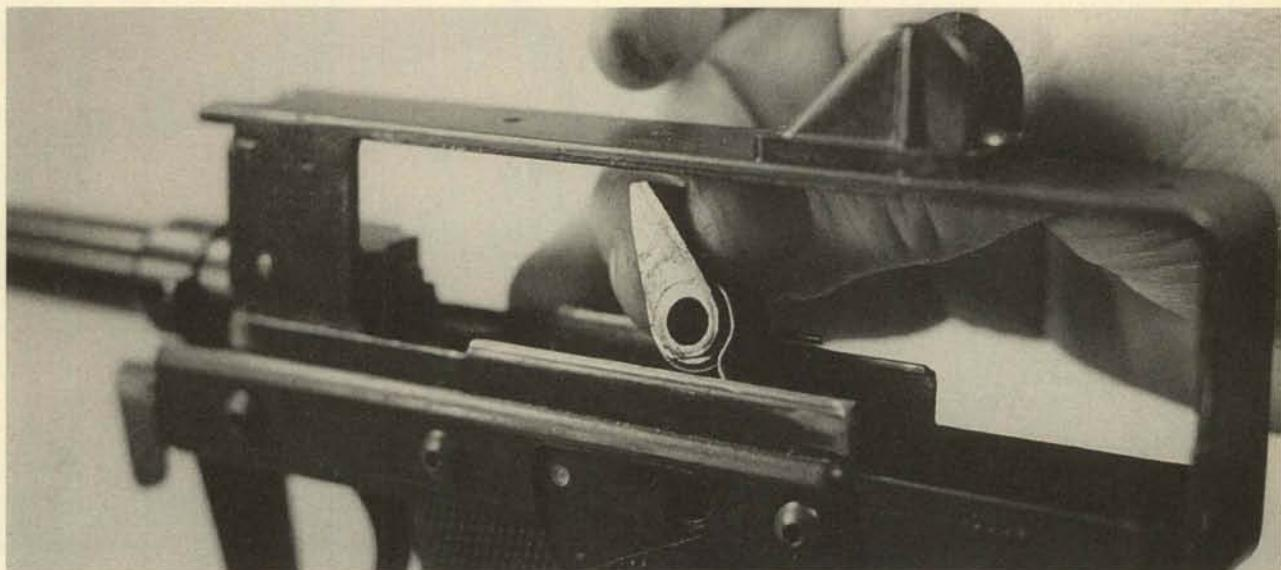
**23.** Remove the hammer and hammer spring assembly. The bushing and spring are easily removed from inside the hammer.
