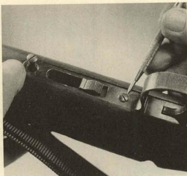
7. Remove the screw at the front of the magazine opening. Remove the wood screw behind the magazine catch. Remove the screw behind the trigger guard.
