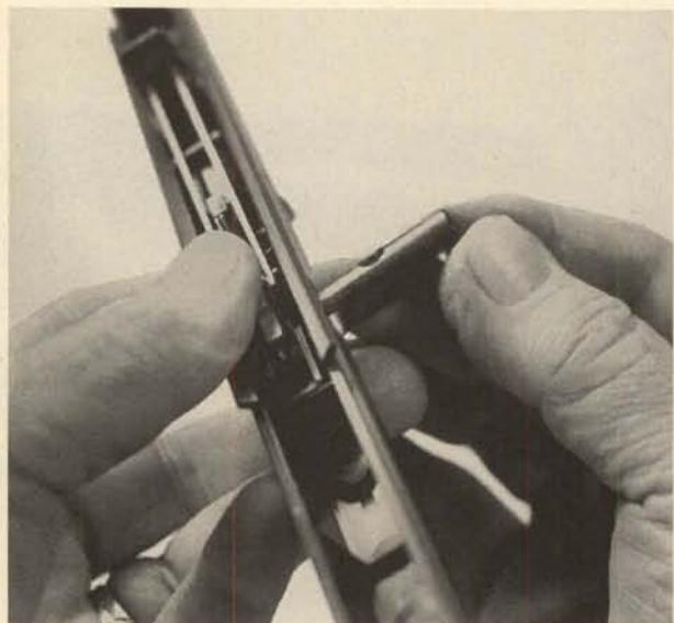
**23.** The lower receiver parts should not be removed unless necessary for repair. If the trigger system is to be removed, first drift out the stock retaining pin (see step 13), and remove the stock toward the rear. Push out the front stock cross pin.
