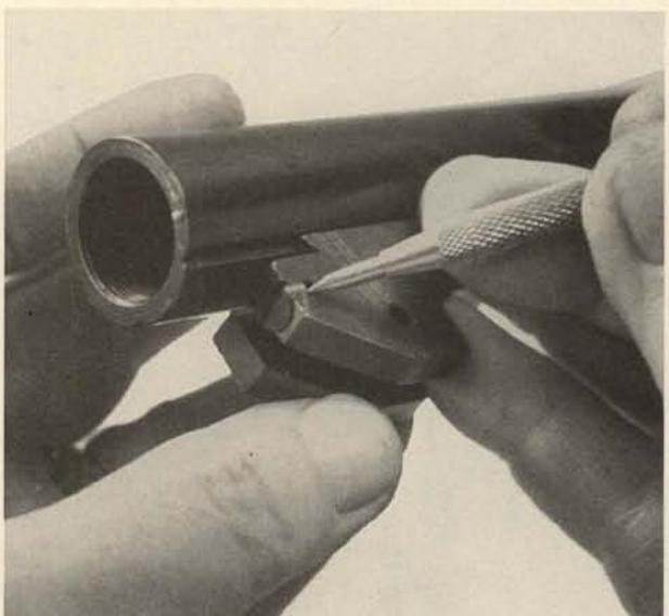
**24.** The screw at the rear of the trigger housing is the trigger adjustment screw. It is pre-set by the factory, and should not be disturbed.
