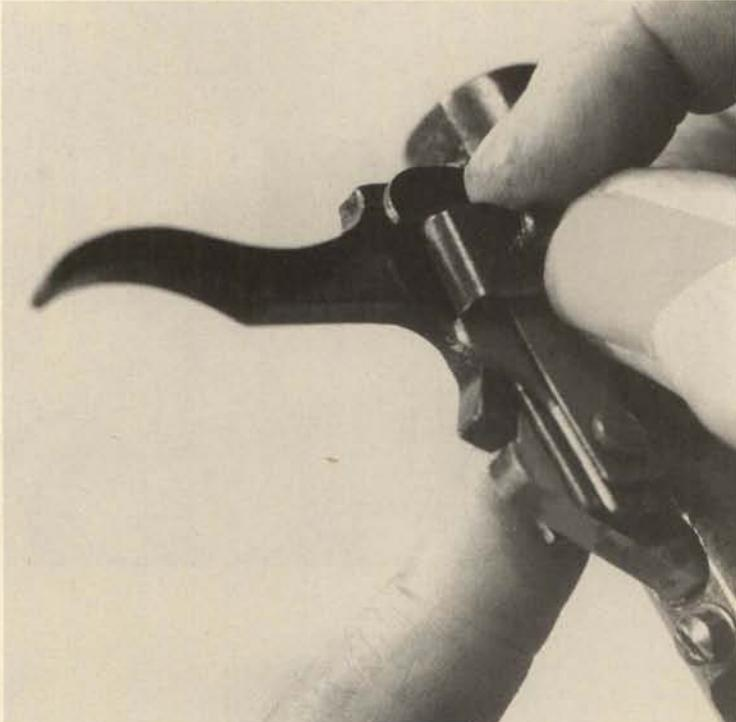
**3.** When replacing the spring clips on the sear and trigger pins, be sure the pins are turned fully toward the left, so the clips will engage their grooves in the heads of the pins.
