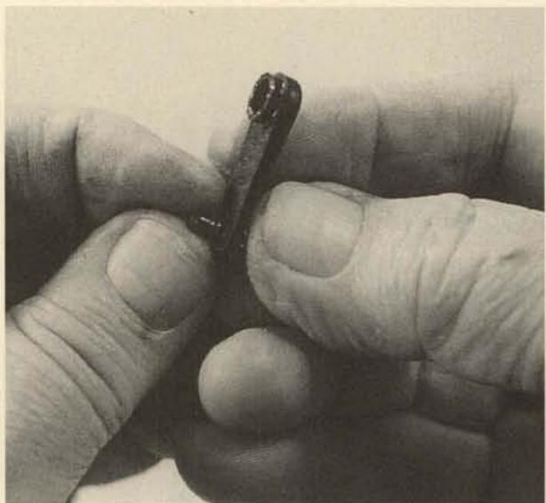
**20.** The plunger and spring are easily removed from inside the lever.
