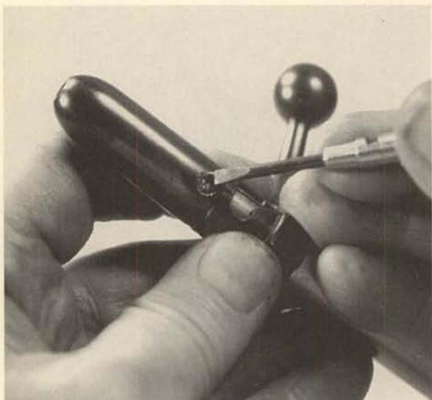
**7.** When the loop of the retainer is aligned with the lock hole, use a tool to push it down into place.
