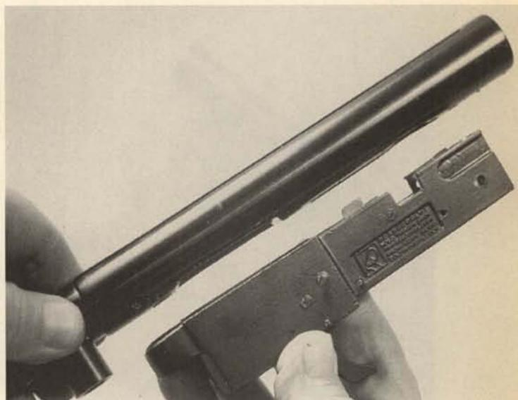
**24.** Remove the trigger group housing from the action.
