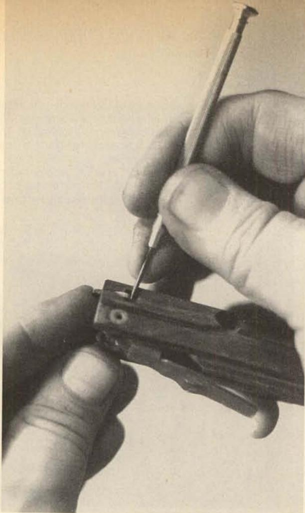
**25.** Insert a small screwdriver between the rear of the extractor and its plunger, and depress the plunger while lifting the extractor out of its recess. **Caution:** The spring is under compression, so take care it doesn't get away. Ease it out, and remove the plunger and spring.
