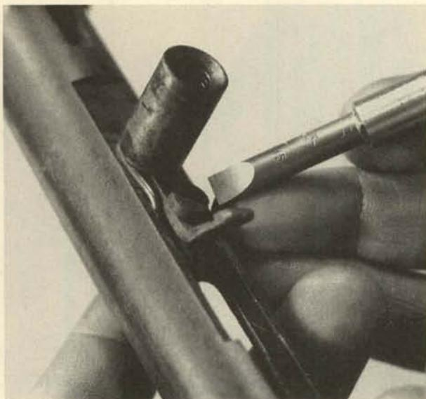
**11.** The magazine catch hook is retained on the underside of the receiver by a single screw, and is taken off downward.
