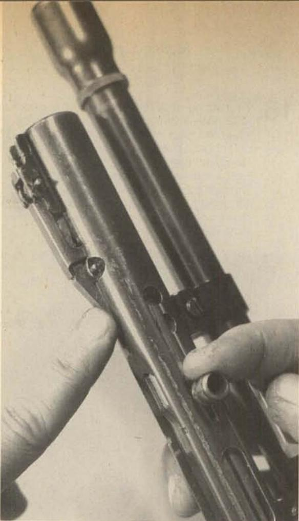
**2.** When moving the bolt forward, press in the front of the sear to allow the striker to pass, so there will be no tension on the spring.
