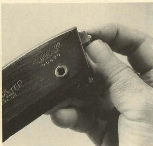
**3.** Move the action slide all the way to the rear, and tip the protruding rear of the bolt downward.
