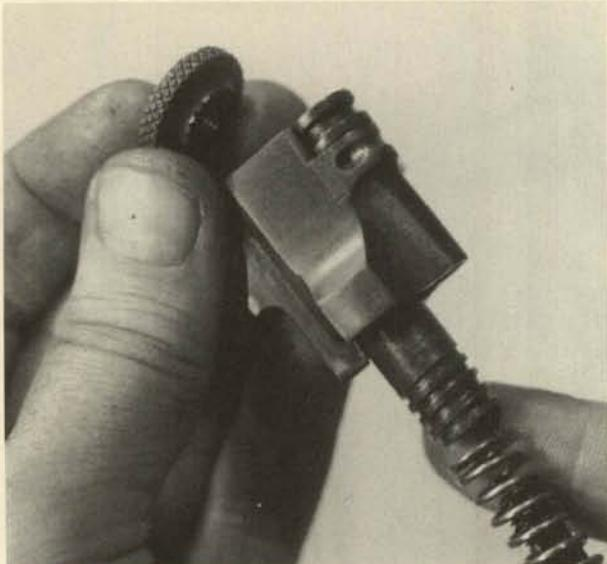
**18.** Remove the cocking piece from the rear of the bolt sleeve. The round-wire nut tension spring is mounted in the rear of the cocking piece and is easily taken out toward the rear.
