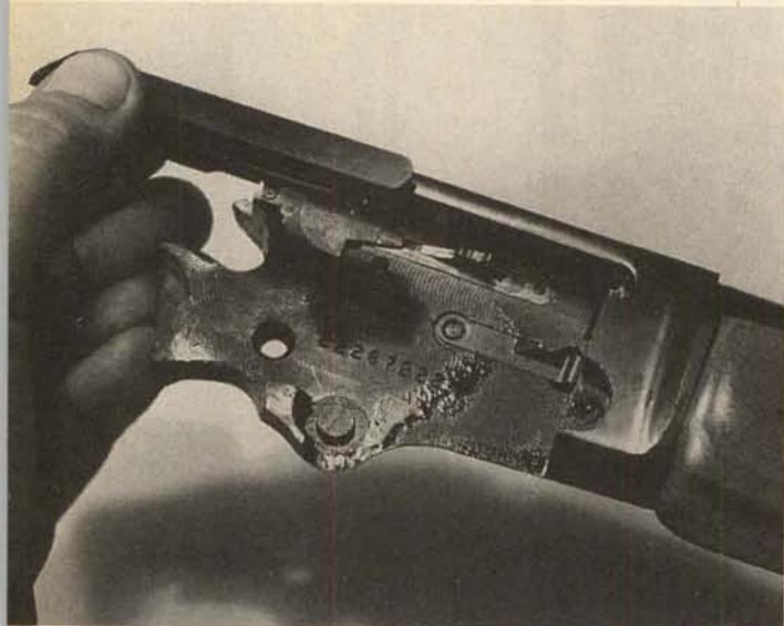
**4.** The firing pin is easily lifted from the top of the breech-block.
