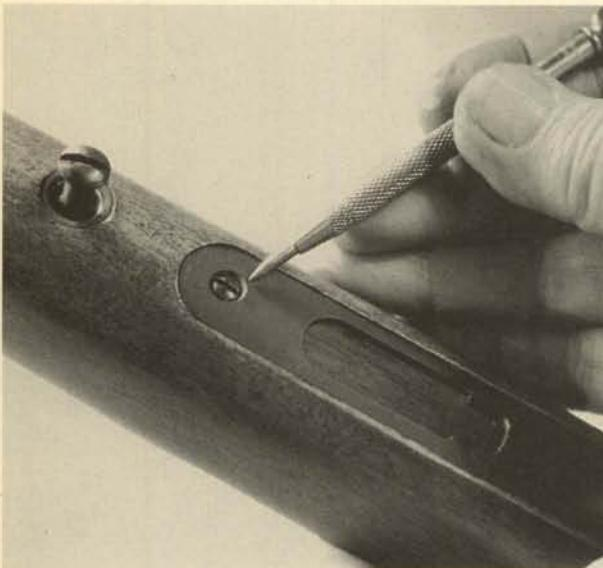
3. The trigger guard unit and the buttplate are each retained on the stock by two wood screws. The stock mounting bolt can be removed by continuing to turn it counterclockwise.
