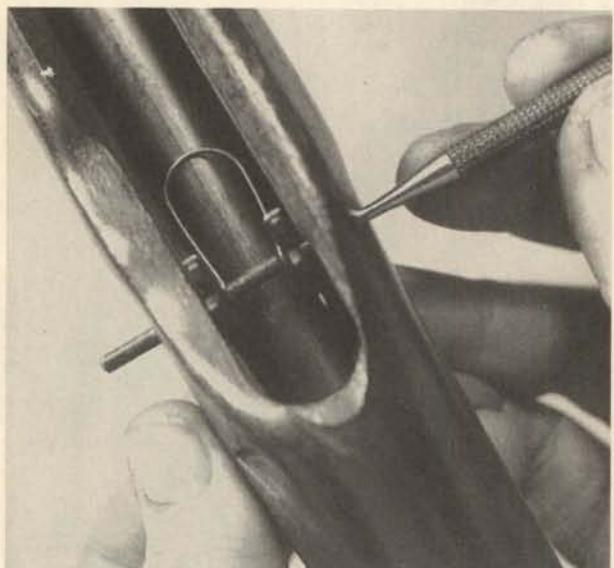
**14.** Push out the trigger pivot pin, which crosses the stock above the magazine tube, and remove the trigger spring upward.
