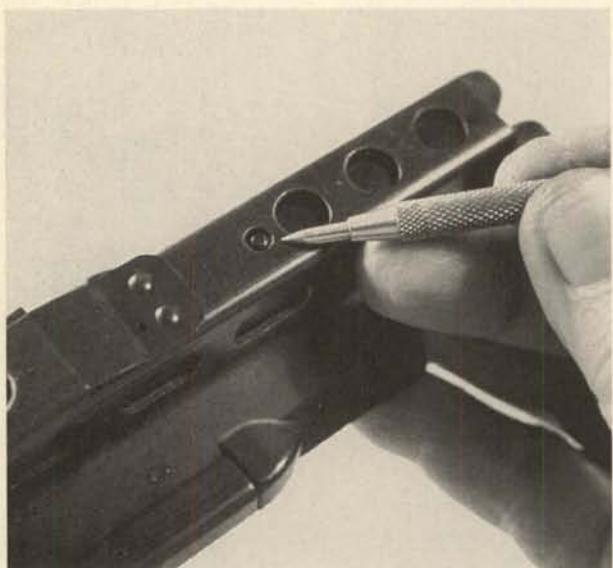
**5.** If the stock has been removed, drift the retaining pin down until its tip is level with the exterior of the stock piece, as shown.
