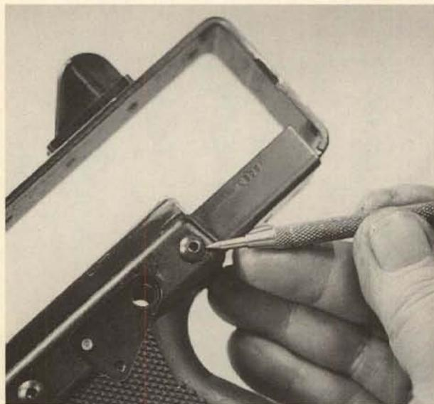
**26.** Remove the Allen screw on the left side at the rear of the grip frame.
