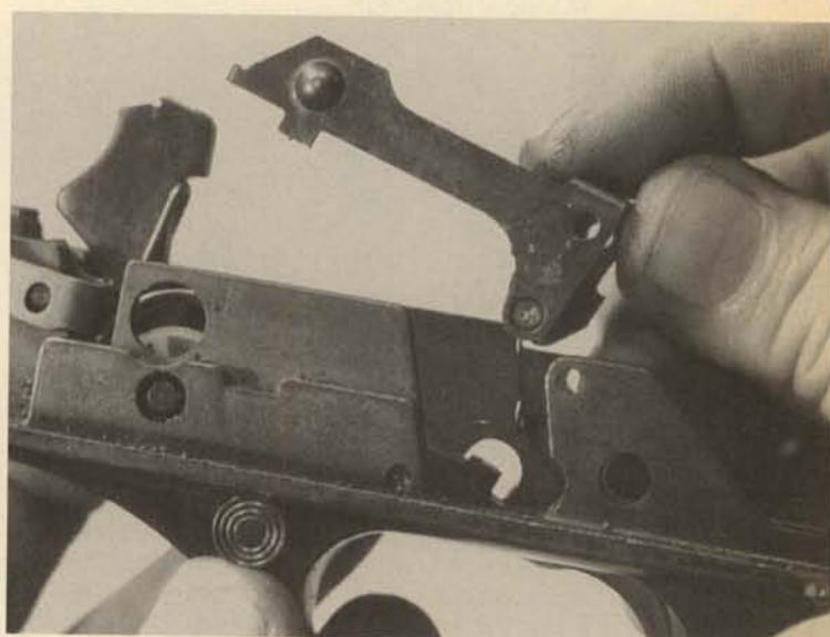
**16.** Remove the sear/disconnector assembly upward. The sear and its spring are a permanent assembly inside the disconnector, the pivot pin being riveted in place at the factory. Routine removal is unwise in normal disassembly.
