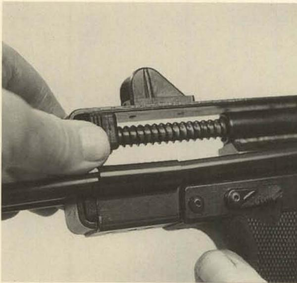
**6.** Tip the assembly out toward either side and remove it. Ease the spring tension slowly.
