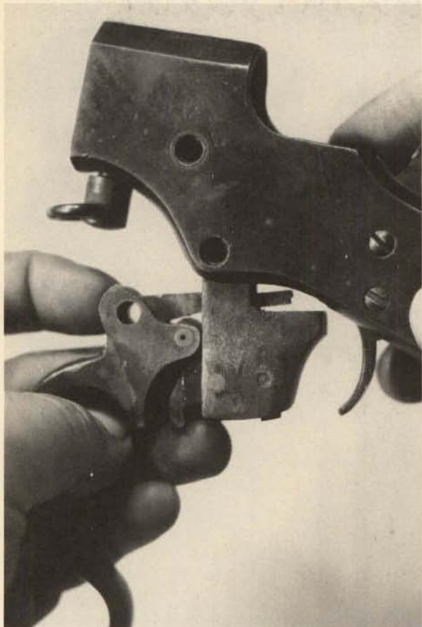
When replacing the lever and breechblock assembly in the receiver, the forward arms of the breechblock should be inserted into the bottom of the receiver first; then the breechblock is tipped into position.
