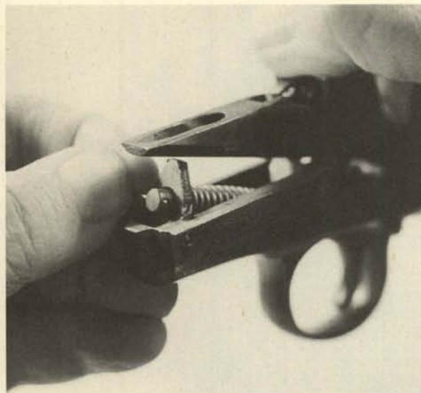
**19.** Retract the hammer slightly until the cross-hole near the tip of the spring guide is accessible, and insert a small pin to trap the hammer spring. Ease the hammer back forward.
