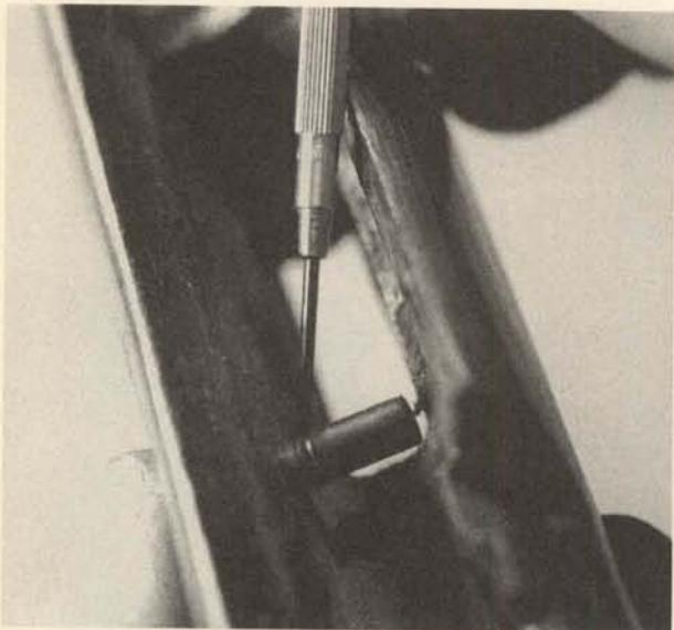
**18.** The magazine catch release button is retained in the left side of the stock by a circular spring clip which rests in a groove on the button shaft. Push the button in to give access to the clip, move it out of its groove and slide it off the shaft toward the right. The button and its coil spring can then be taken off toward the left.
