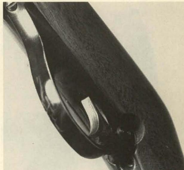
**5.** Remove the cap screw and screw-slotted post at the rear of the sub-frame below the receiver. If this assembly is very tight, it may require two opposed screwdrivers to immobilize the post while the screw is taken out.
