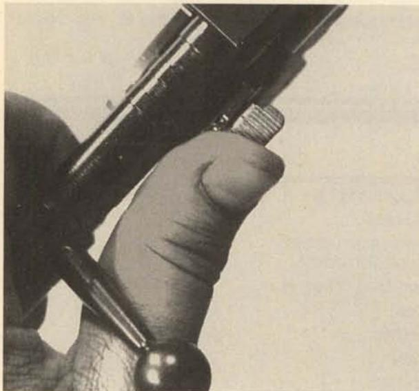
2. Grip the underlug of the striker head, at the rear of the bolt, in a sharp-edged bench vise, and be sure it is firmly held. Push forward on the bolt end piece, against the tension of the striker spring, and unscrew the forward portion of the bolt from the end piece. **Caution:** The powerful spring is under heavy tension, so control the bolt as the threaded section is cleared.
