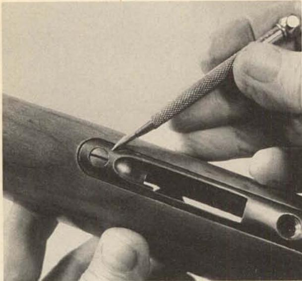
6. Push out the trigger pin toward either side. Restrain the trigger, as the spring is under tension.
