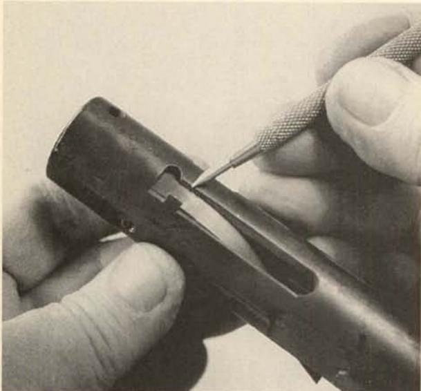
**2.** Re-hook the trigger rod and grip safety rod to their bars in the firing system before the system housing is swung back upward into place. The proper arrangement is shown.
