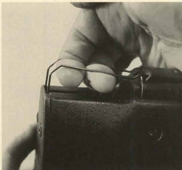
**3.** Pull the cocking piece guard upward slightly at the rear, just enough to snap it out of engagement with its detent.
