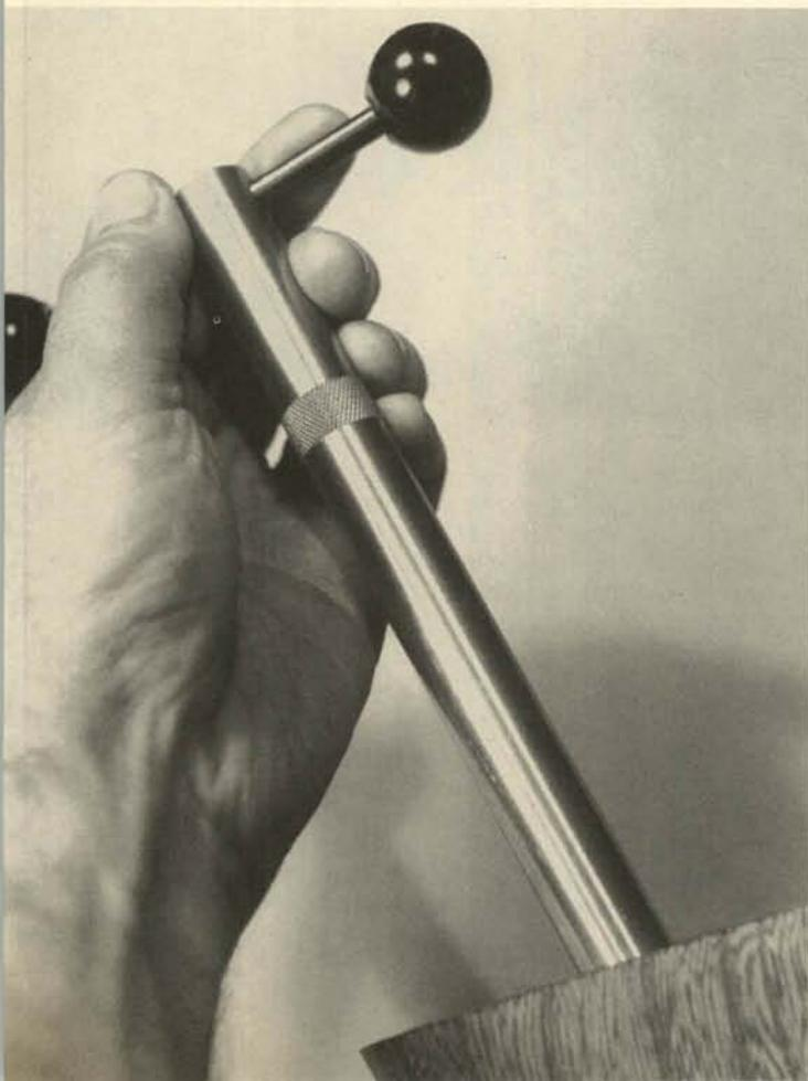
3. Take off the buttpiece and use a B-Square stock tool, a 3/8-inch socket wrench, or a long screwdriver to remove the stock mounting bolt. Take off the stock toward the rear. Grip the stock mounting stud firmly with leather-padded pliers and unscrew it from the rear of the receiver. Take out the hammer spring toward the rear, and take care not to lose the lock washer on the neck of the stud.
