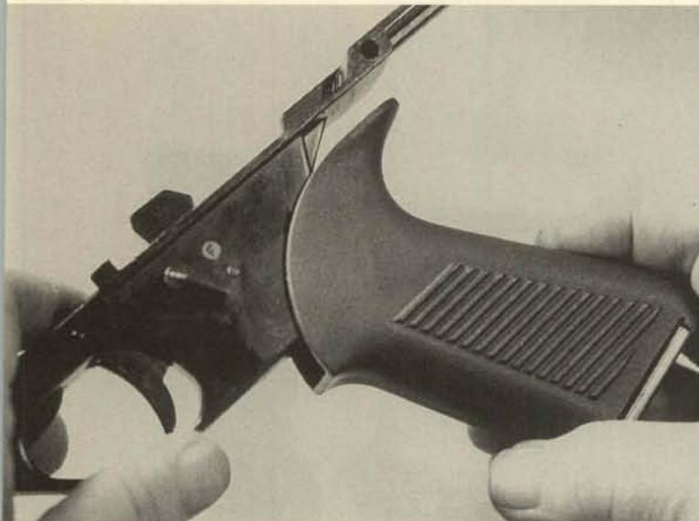
**24.** Move the safety to off-safe position, restrain the hammer, pull the trigger, and ease the hammer down to fired position. Restraine the hammer and drift out the hammer pivot pin.
