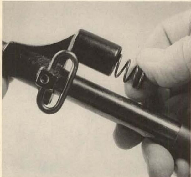
**18.** Restrain the hammer, pull the trigger, and ease the hammer down to fired position. Drift out the trigger guard cross pin toward the left, and take off the trigger guard downward.
