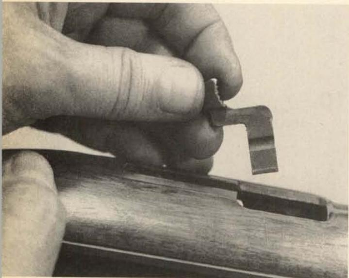
**13.** Continue tipping the front of the bolt outward until it clears the inner edge of the receiver; then ease it out, releasing the spring tension slowly. Take out the bolt spring and its guide.
