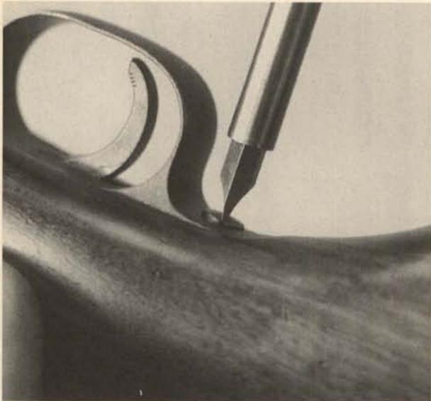
6. To remove the rear sight, first turn out the knurled knob on the right side at the front of the sight until it stops; then push it toward the rear and hold it there while sliding the sight upward out of its base. It can be taken completely off, or just moved until it exposes the screw covered by the sight slide, near the scale marker.
