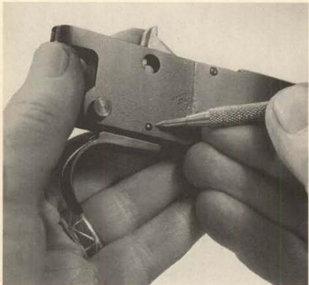
**27.** If the previous steps have been done, drift out the trigger cross pin and remove the trigger downward.
