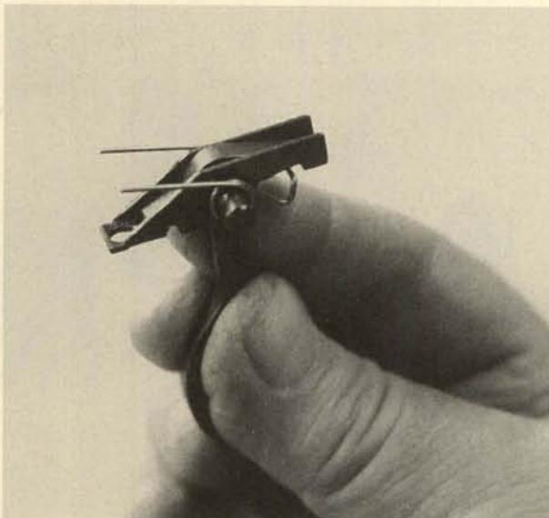
**2.** When installing the safety cross-piece, depress the rear arms of the trigger spring on each side, to bear under the cross-piece.
