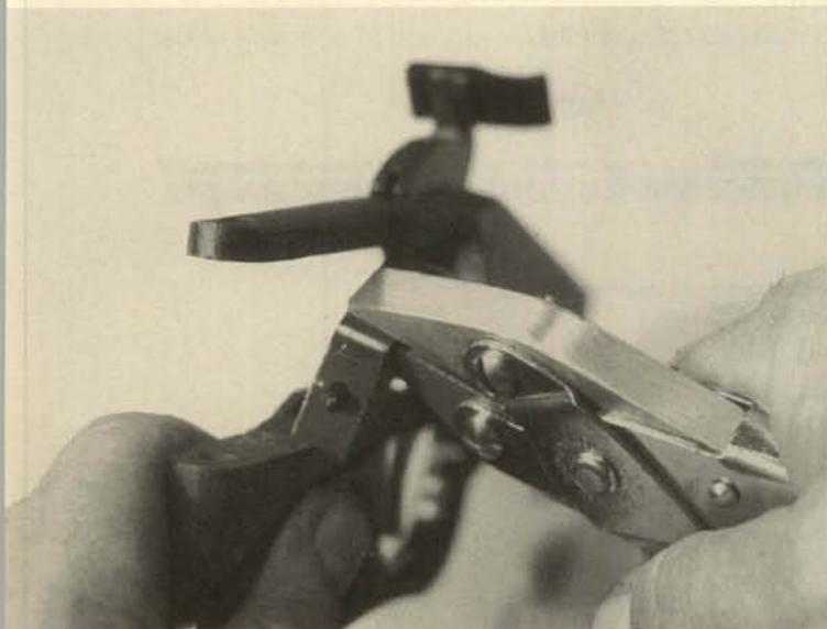
**2.** When rejoining the front and rear parts of the gun, be sure the breechblock is all the way forward, the hammer is at full cock or on the safety step, and take care that the front tongue of the sideplate (arrow) is properly engaged with its mating recess in the main frame.
