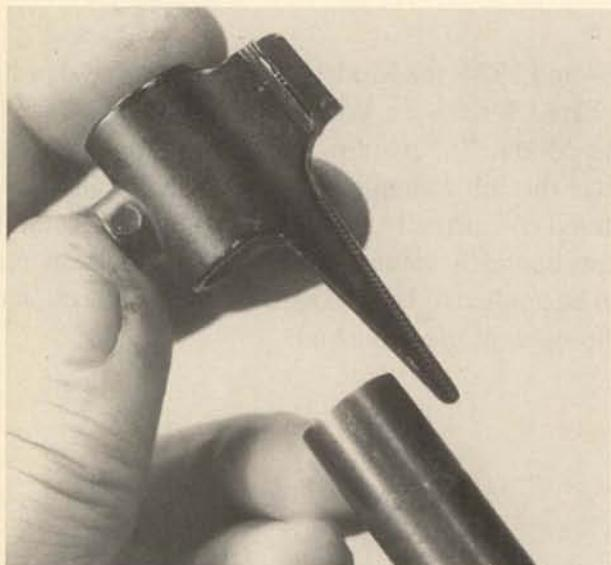
3. When the action is out of the stock, the front sight is easily slid off toward the front.
