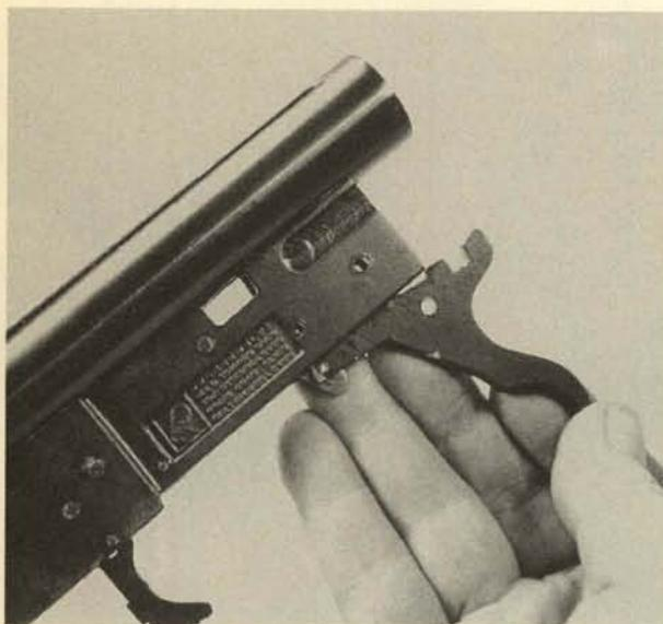
**19.** Move the trigger assembly downward and toward the rear for removal.
