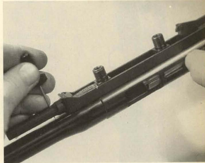
**4.** After the system is in place, with the rear lug engaging the bolt, draw the bolt back until the tip of the recoil spring guide enters its recess in the frame. The tool can then be taken out to release the spring.
