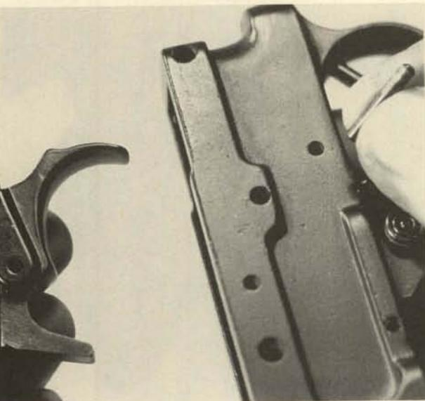
**14.** Note the position of the sear and disconnector in the top of the trigger before disassembly. Push out the trigger pivot cross pin, and remove the trigger/sear/disconnector assembly upward. As the trigger is moved upward, the trigger spring and plunger will be released at the rear of the trigger guard. Ease them out, and remove them downward and toward the front.
