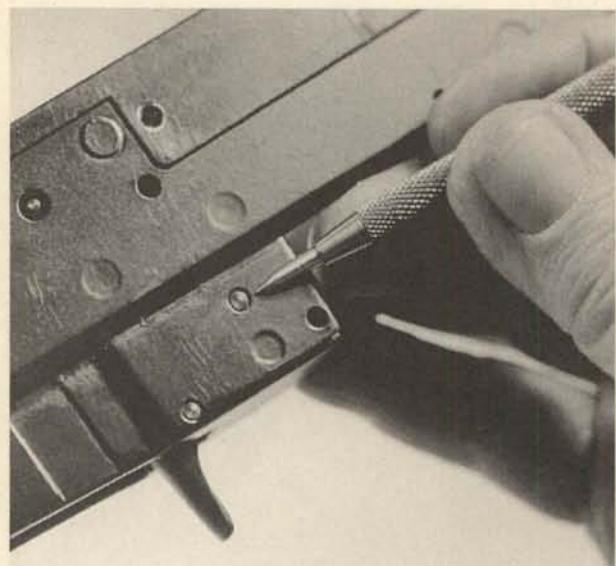
**35.** Drifting out this cross pin will allow removal of the sear and sear spring. Control the spring as the drift is taken out.
