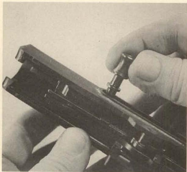
**7.** Align the bolt handle with its exit space in the track, and remove the handle toward the right.
