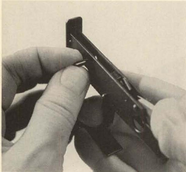
**30.** Push the trigger forward and push out the trigger cross pin toward either side.
