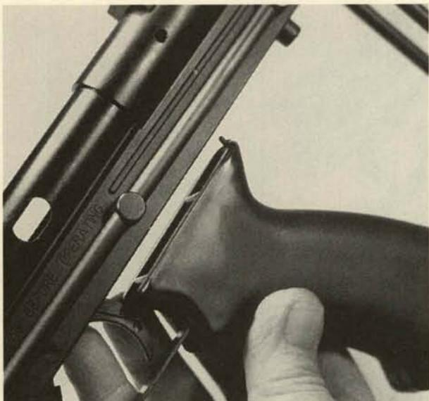
**18.** Remove the middle Allen screw in the lower receiver.
