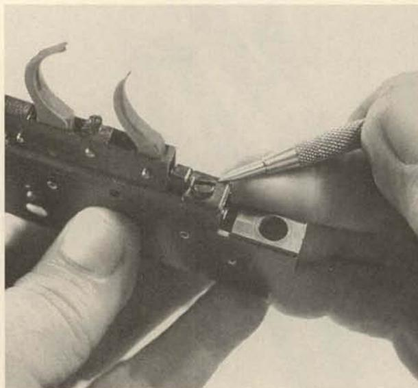
**28.** The spring for the main (firing) trigger is removable by taking out the screw that retains its housing.
