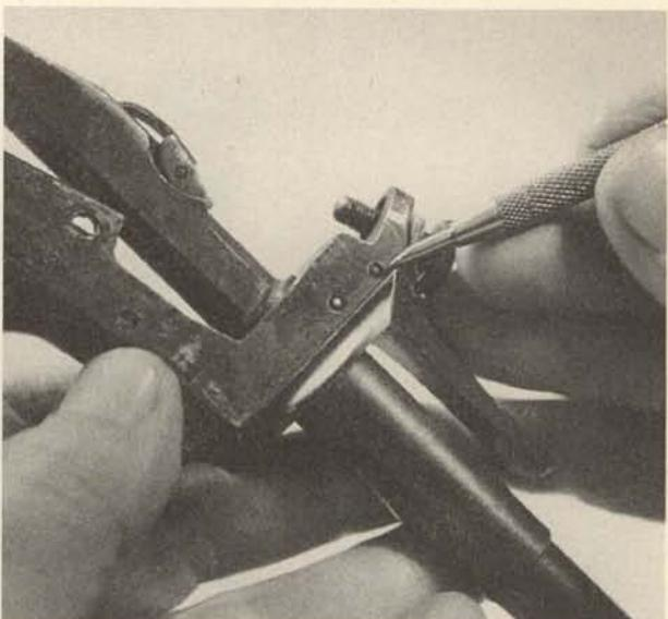
**31.** The cartridge stop and its spring can be removed from the magazine housing by pushing out this cross pin. Take care that the small coil spring is not lost.
