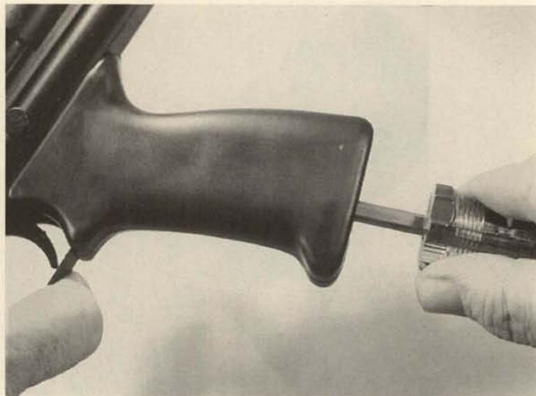
**16.** With a larger Allen bit, remove the screw inside the pistol grip. Note that there are two washers on this screw. Take care that they are kept in order and not lost.
