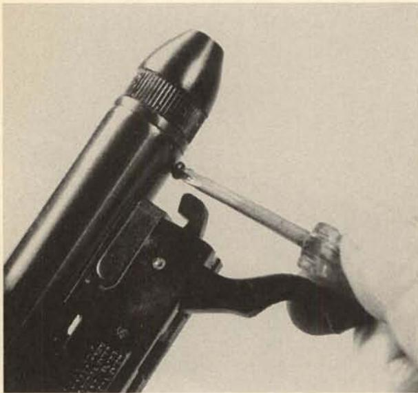
6. Unscrew and remove the receiver end cap. **Caution:** Springs are under tension, so control the cap.
