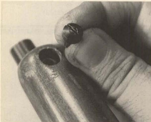
2. Back out the main stock mounting screw, located on the underside of the stock, just forward of the trigger guard, and remove the action from the stock.
