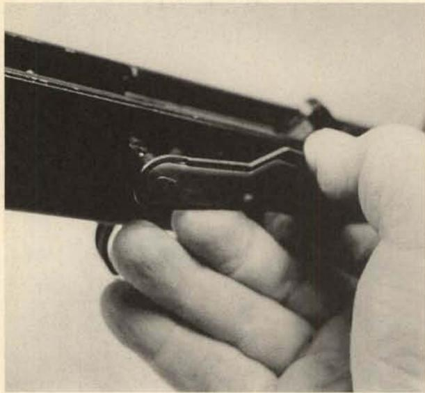
**26.** Remove the two screws on the right side at the rear of the receiver cover. Removal of the screws will release the sling loop on the left side.
