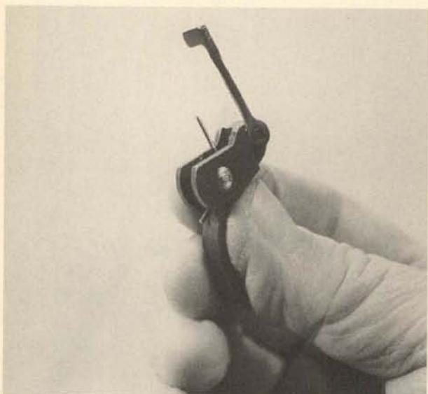
**5.** Use a slave pin to retain the trigger spring during reassembly and be sure the loop of the hammer block engages the post on the trigger.
