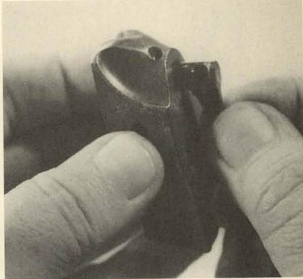
**13.** Remove the screws on each side of the receiver that retain the lower tang unit. **Note:** Keep these in order, right and left, and they will fit better on reassembly.
