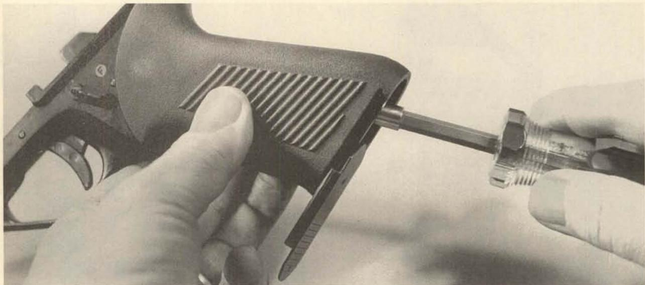
**22.** Slide open the pistol grip cap and use a screwdriver to remove the mounting screw.
