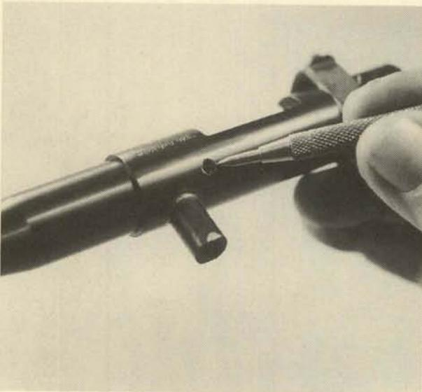
**10.** With a tool or a strong thumbnail, depress the extractor plunger and remove the extractor toward the side. **Caution:** Control the strong spring and plunger.
