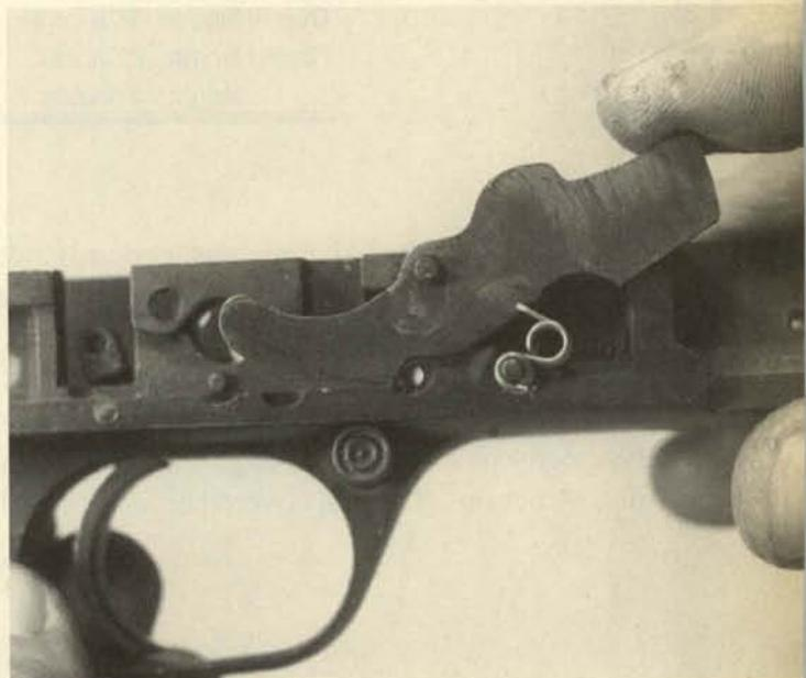
Install the sear, hammer and disconnector in that order, to ensure that the inner arm of the disconnector is in proper engagement with the side tab of the sear. When installing the sear, be sure the right-angled tip of the forward arm of the sear spring engages properly with its shelf on the inside right wall of the trigger group.
