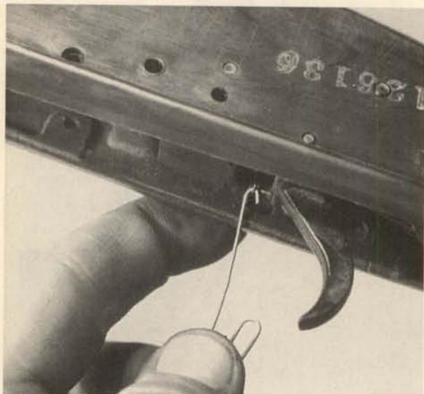
**5.** It is very difficult to reattach the trigger spring to the front of the trigger without a small hooked tool. The one shown was made from an opened paper clip.
