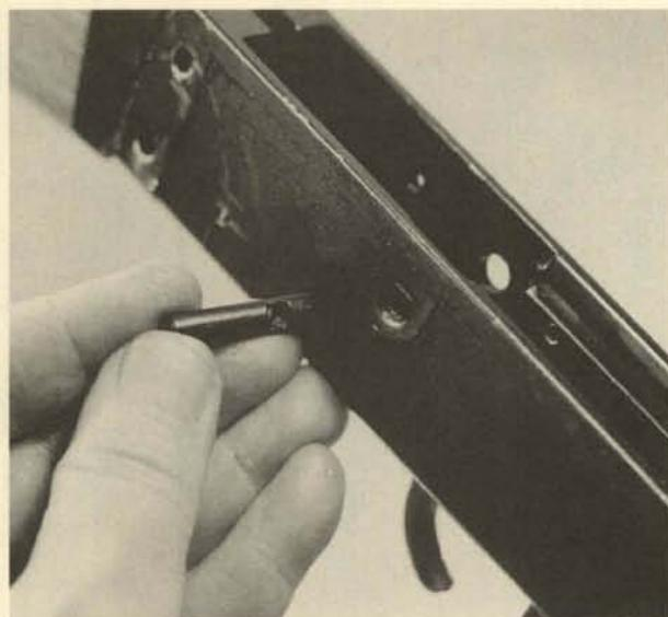
**31.** Remove the hammer spring base pin.
