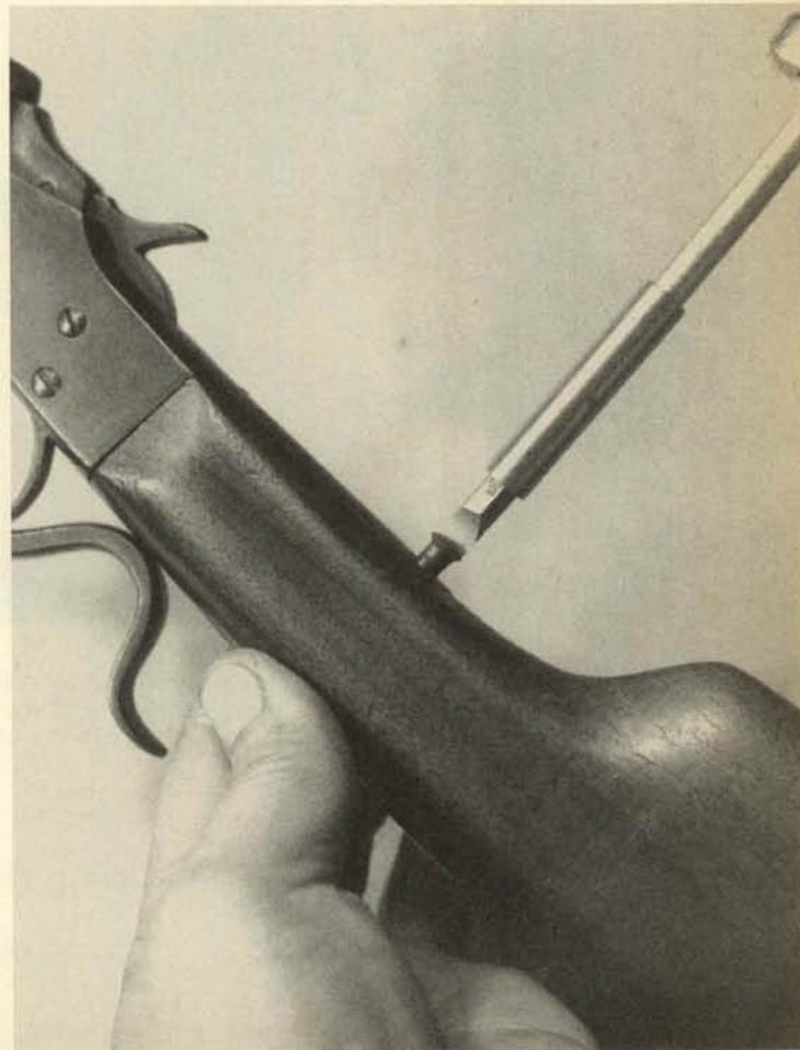
4. Remove the screws at the rear tip of the upper and lower receiver tangs to release the stock for removal. Remove the stock toward the rear. If the stock is very tightly fitted, it may be necessary to bump the front of the comb with the heel of the hand or with a soft rubber hammer.
