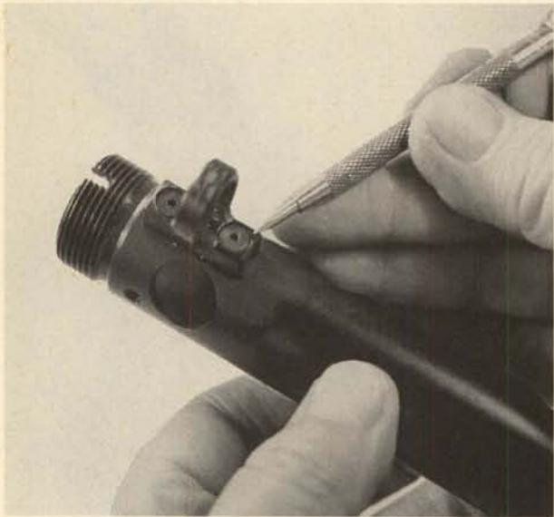
**22.** Inside the rear of the lower receiver are two polymer spacer blocks, through which the mounting screws pass. Remove these and keep them in the correct order and orientation as they are not interchangeable.
