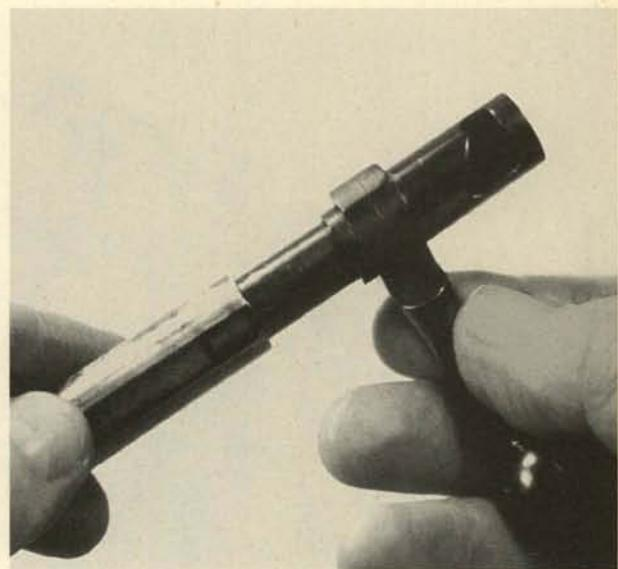
**9.** Insert a tool at the rear to arrest the striker spring and push out the retaining cross pin. **Caution:** *Control the spring.*
