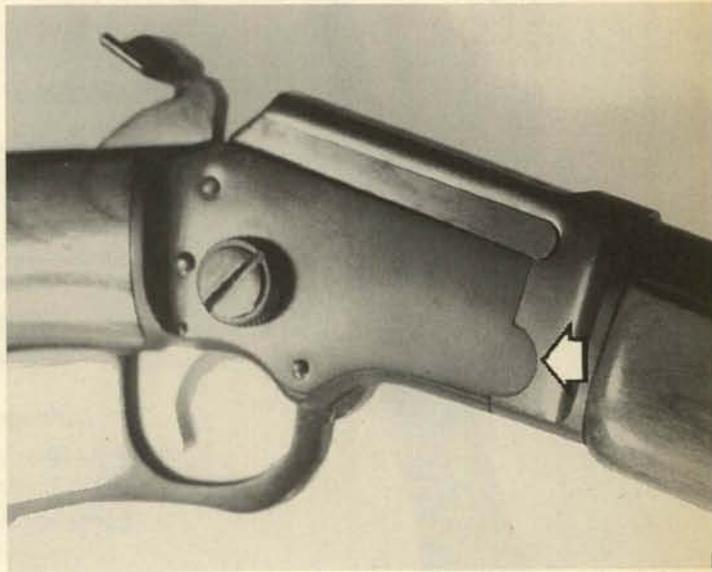
Avoid over-tightening the small screw which holds the cartridge guide spring above the chamber, or the spring may crack. This advice also applies to the cartridge stop screw. Both should be firm and snug, but use no excessive force.
