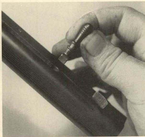
**3.** Move the bolt all the way to the rear, until the bolt handle aligns with the opening at the end of its track, and remove the bolt handle toward the right.
