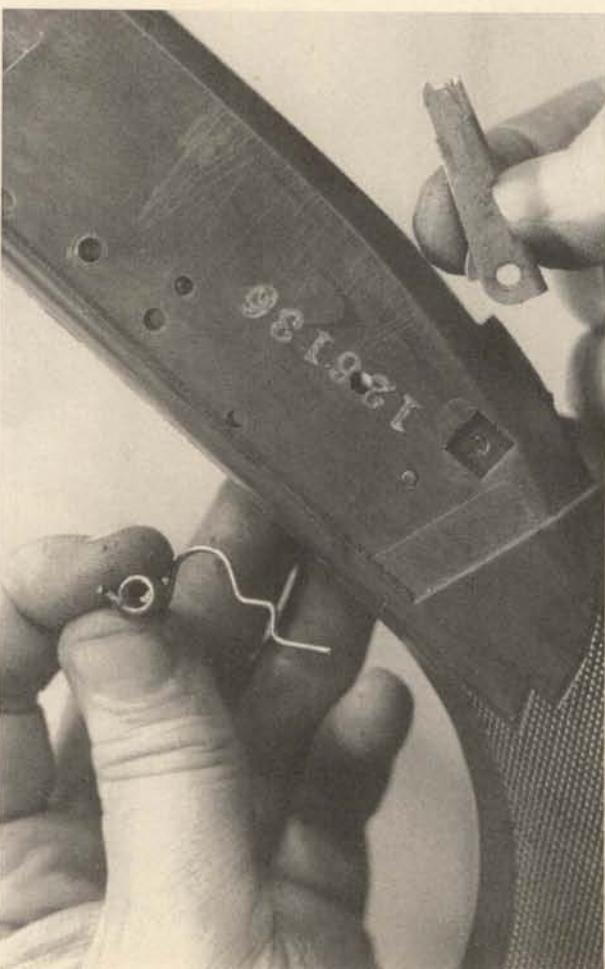
**20.** Push out the sear pivot pin, and remove the sear and its spring from the top of the receiver (actually, the spring will usually fall from the bottom as the pin is taken out).
