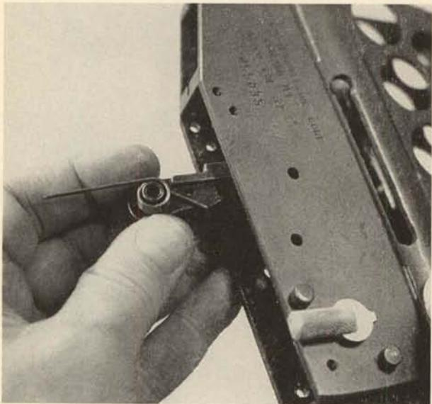
**18.** An Allen screw retains the safety spring and plunger at the rear of the receiver on the right side.
