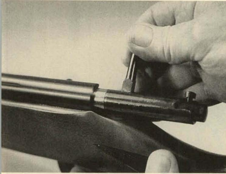
2. Push the cocking lug off its step to lower the striker to fired position.
