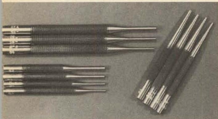
**9.** A good set of drift punches will prevent a lot of marred pins. These, from Brownells, are made by Mayhew. The tapered punches at the right are for starting pins, the others for pushing them through. Two sizes are available—4 inches or 6 inches.
