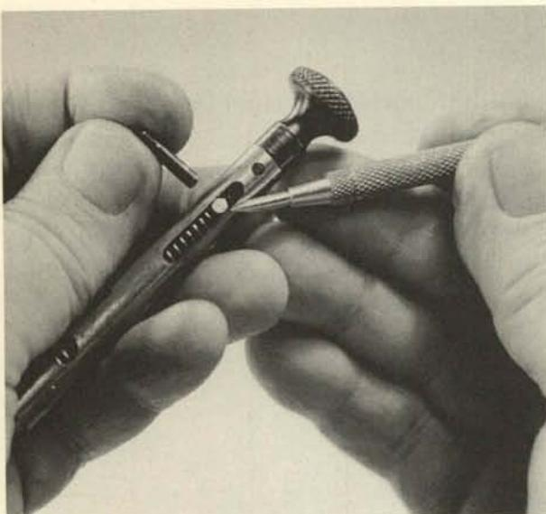
**3.** Use a slave pin to separate the rebound spring from the head of the striker spring plunger, as shown.
