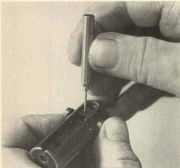
8. The extractor is retained by a vertical pin at the front of the bolt, accessible at the extreme rear of the open firing pin groove in the top of the bolt. The pin is driven out toward the bottom of the bolt. Here, again, use a very slim drift punch. When the pin is out, the extractor and its spring are removed toward the right.
