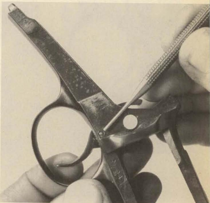
**14.** Drifting out the trigger cross pin will allow the trigger to be removed upward. The sear is an integral part of the upper projection of the trigger.
