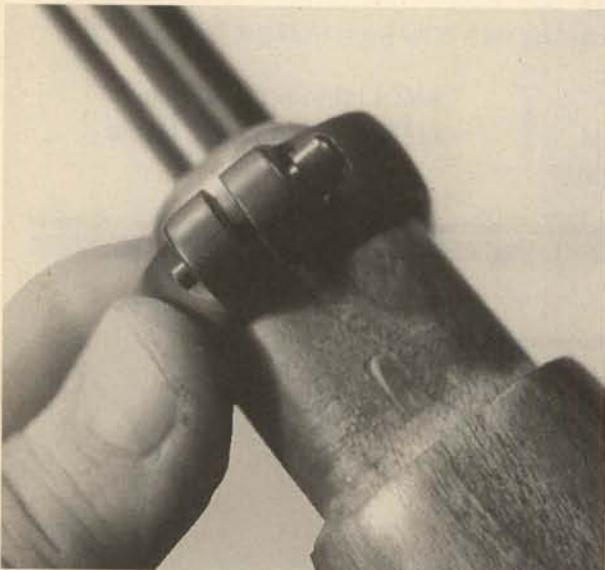
**2.** Remove the magazine, and cycle the action to cock the internal hammer. Back out the main stock screw, located on the underside just forward of the magazine well.
