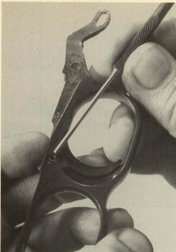
**18.** Drift out the roll cross pin at the rear of the trigger, restrain the sear link, and remove the link and its spring upward.
