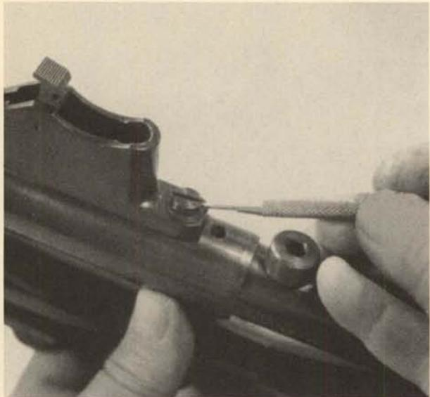
**18.** Remove the screw and lock washer at the rear of the housing.
