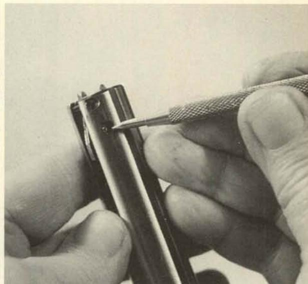
**23.** The combination ejector and firing pin can be removed by drifting out this roll pin, but the plunger and spring may be difficult to remove without further disassembly of the bolt. It can be done, though, if only this part needs to be replaced in repair. The forward roll pin is a guide only, and it does not have to be removed.
