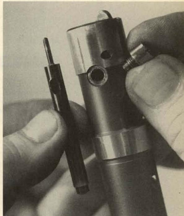
When replacing the trigger and disconnector assembly, push the small rear spring pin halfway across, and hook the rear loop of the expansion spring onto it. Then, drive the pin into place. Lift the sear and insert the front of the disconnector arm into the vertical slot in the sear. Allow the sear to hold the trigger and disconnector in place while the trigger is positioned for insertion of its cross pin.
