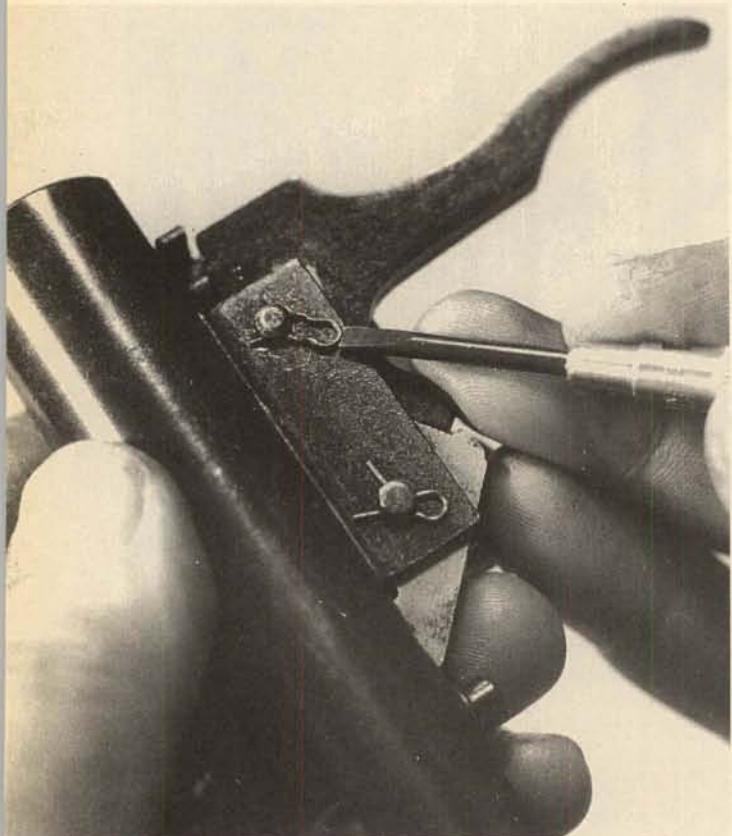
4. When replacing the striker/firing pin unit in the bolt, insert it only as far as shown, then install the bolt handle sleeve, and let it carry the striker into the bolt.
