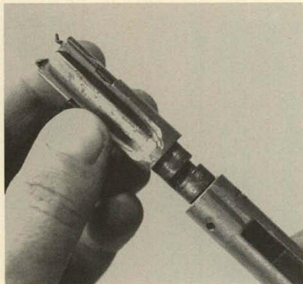
**3.** Remove the front section of the bolt toward the front.
