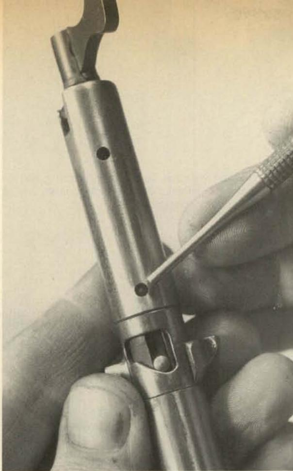
**5.** Drift out the cross pin just to the rear of the bolt handle sleeve.
