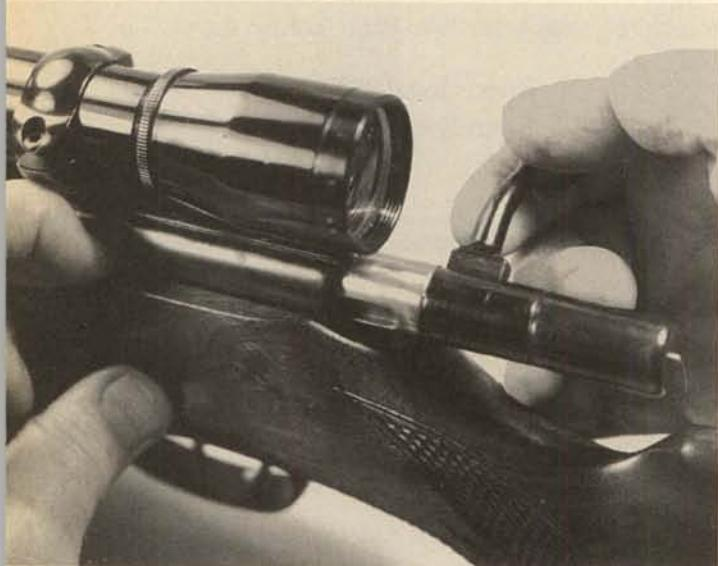
2. Grip the front portion of the bolt firmly and turn the handle to lower the striker to fired position.
