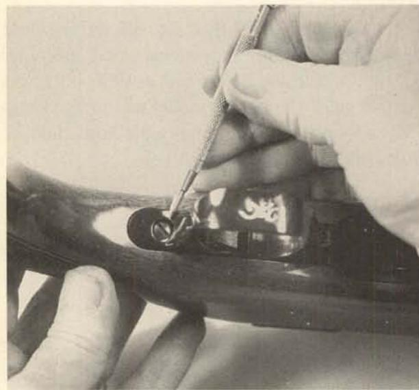
**3.** Remove the rear stock mounting bolt, located at the rear of the trigger guard unit.
