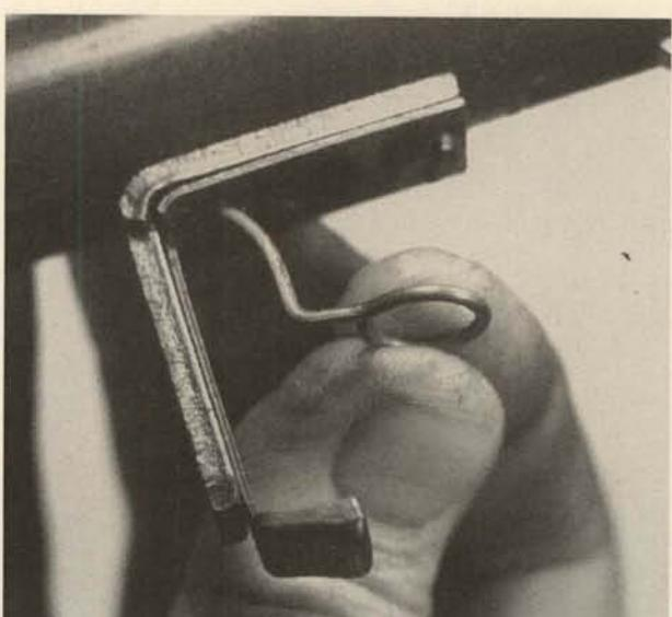
**13.** Remove the smaller screw, at the rear of the magazine guide bar and catch base. Remove the guide bar and magazine catch downward. Drift out the trigger cross pin, taking care that the trigger post is well supported.
