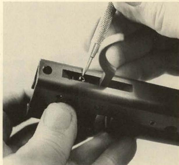
**19.** Before the safety cross-piece can be removed, the roll pin that engages the disconnector slide must be drifted out downward, from inside the receiver.
