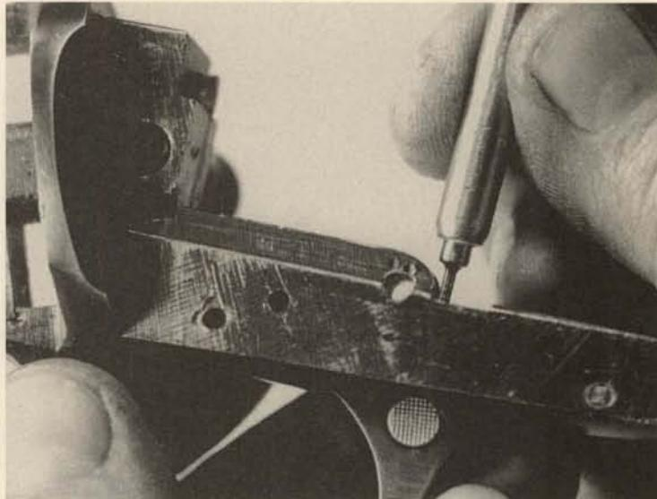
**23.** With the safety in off-safe position, insert a very small drift into the hole in its top, inside the frame, and tip the drift punch over toward the front of the unit, turning the safety to disengage its positioning plunger from the detent cuts on the underside of the safety. The safety can now be tapped out toward the left side. **Caution:** As the safety clears the plunger and spring mounted below it, they will be released. Restraine them, and ease them out.
