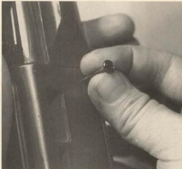
**3.** Remove the receiver cover assembly upward. The internal cartridge guide spring and the rear sight base are riveted on the cover, and removal is not advisable in normal disassembly.
