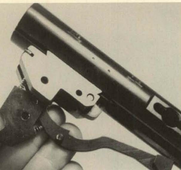
**19.** Remove the trigger and disconnector assembly downward.
