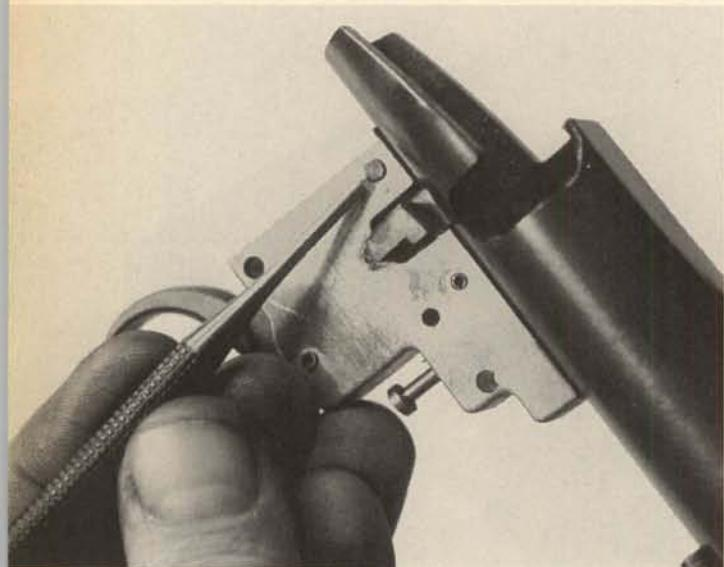
**10.** The trigger housing retaining pin is a roll pin at the upper center of the housing. Drifting out this cross pin will allow the trigger housing to be taken off downward. When the housing is removed, the bolt stop and its spring can be lifted from their well in the top of the housing, and the sear is easily removed by drifting out its cross pin.
