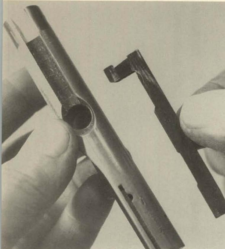
**9.** The twin extractors are retained by two vertical roll pins at the front of the bolt. Use a roll pin punch to drift out the pins, and remove the extractors from each side, along with the single transverse coil spring that powers both.
