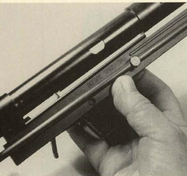
**19.** Remove the lower receiver downward.
