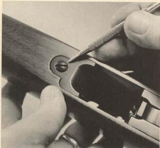
**7.** Remove the large screw in front of the magazine opening and take off the forward plate.
