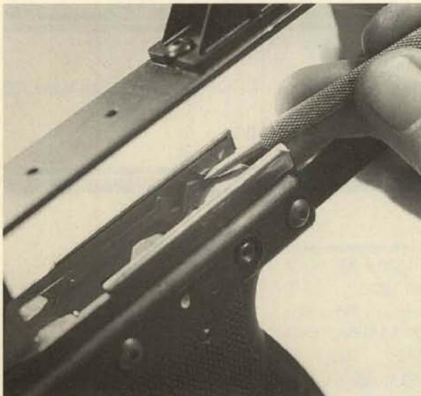
**8.** If the firing pin has been removed, check the free movement of the firing pin as the Allen screw is tightened. If it binds the firing pin, back it off until the pin moves freely.
