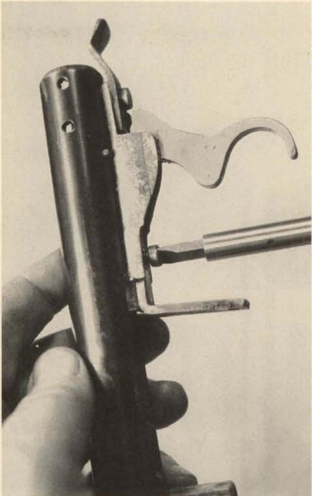
**10.** Remove the trigger bracket downward. The safety-lever is easily detached from the rear of the trigger bracket.
