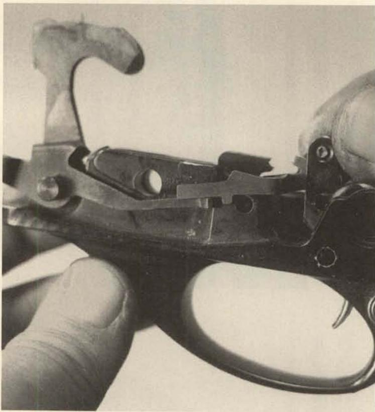
**4.** To replace the receiver coverplate on the underside, invert the gun and start the plate with its inner surface facing outward. Press it inward, compressing its rear side wings; then swing it over forward until it can be snapped into its retaining grooves.
