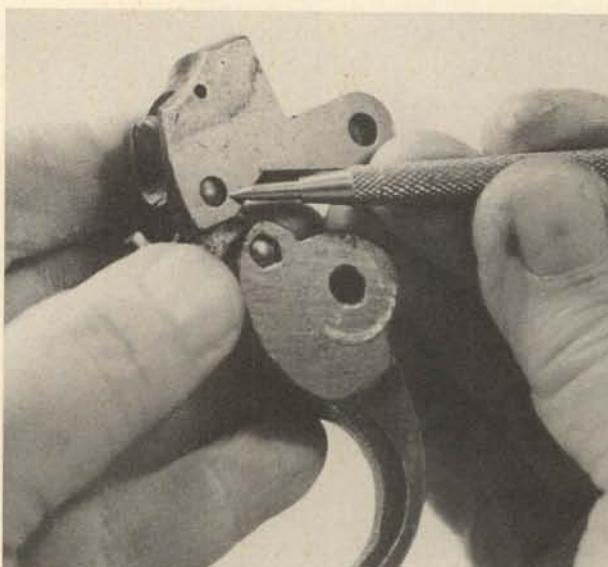
**13.** Drift out the breechblock link pin and separate the breechblock and link. If the firing pin has not been previously removed, drift out its roll-type pin and remove the firing pin and its spring toward the rear.
