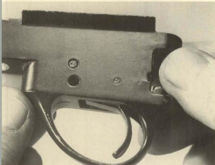
**14.** Restrain the hammer against the tension of its spring, pull the trigger, and ease the hammer down to the fired position. Drift out the hammer pivot, the larger of the two cross pins, and remove the hammer and the combination hammer and trigger spring upward. Drift out the trigger pivot, the smaller cross pin, and remove the trigger upward, along with the sear, which is mounted in the top of the trigger and pivots on the same pin.
