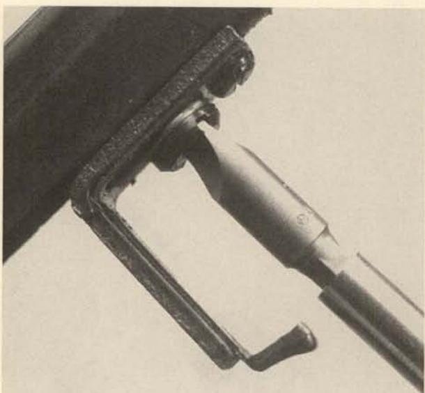
**11.** Remove the large vertical screw on the underside of the receiver, just to the rear of the magazine guide bar and catch.
