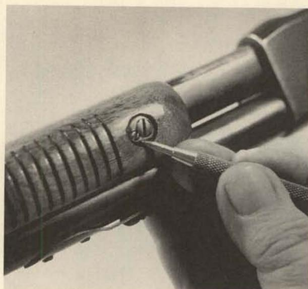
**9.** Move the forend forward until it is clear of the enlarged portion of the magazine housing.
