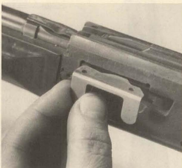
**5.** Loosen the large cross-slotted screw on the underside of the stock, just forward of the trigger guard; then push it upward to raise the barrel retaining piece until its upper cross bar clears its recess on top of the barrel. Slide the barrel out toward the front.
