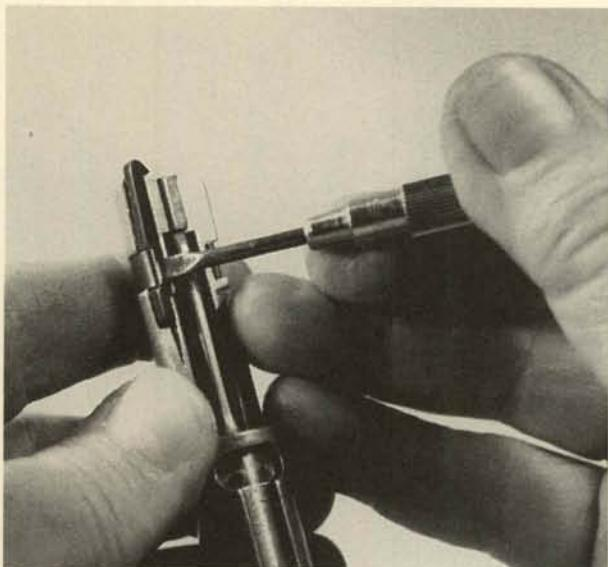
**11.** To remove the extractor, use a tool to pry the band-type spring until its hook clears the shelf. **Caution:** Control the spring band.
