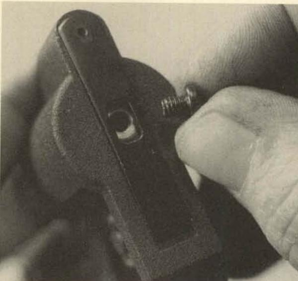
2. When replacing the sideplate, be sure the small tip of the hammer pivot is aligned with its hole in the sideplate.
