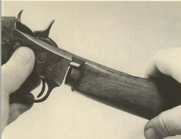
**3.** Remove the large screw at the end of the upper tang. Take off the buttstock toward the rear. The buttplate is retained by two wood screws.
