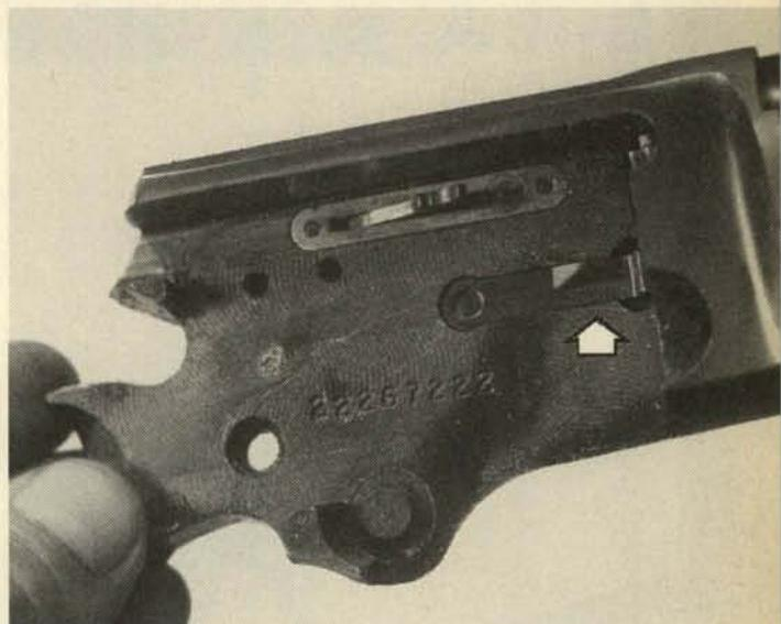
**7.** The cartridge guide spring, located just above the chamber, is retained by a screw which enters from the top of the receiver. This is the larger screw near the front scope mount screw. The cartridge guide spring is removed downward.
