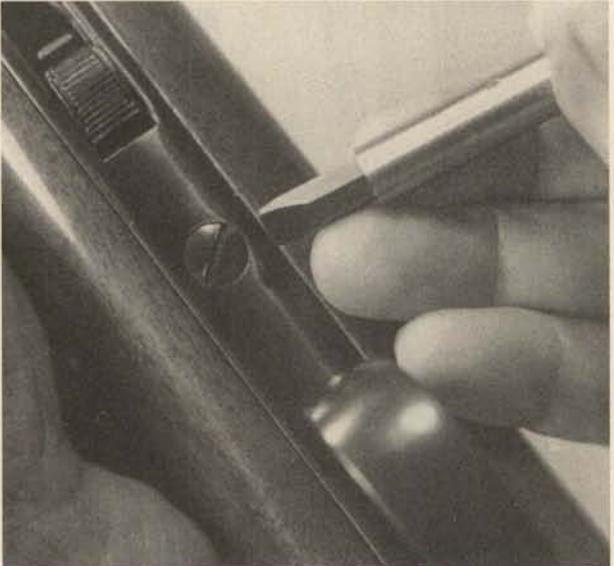
**3.** To remove the bolt, open it and move it toward the rear while depressing the bolt stop, located on the left side of the receiver, and withdraw the bolt toward the rear. Note that the safety must be in the horizontal off-safe position before the bolt can be opened.
