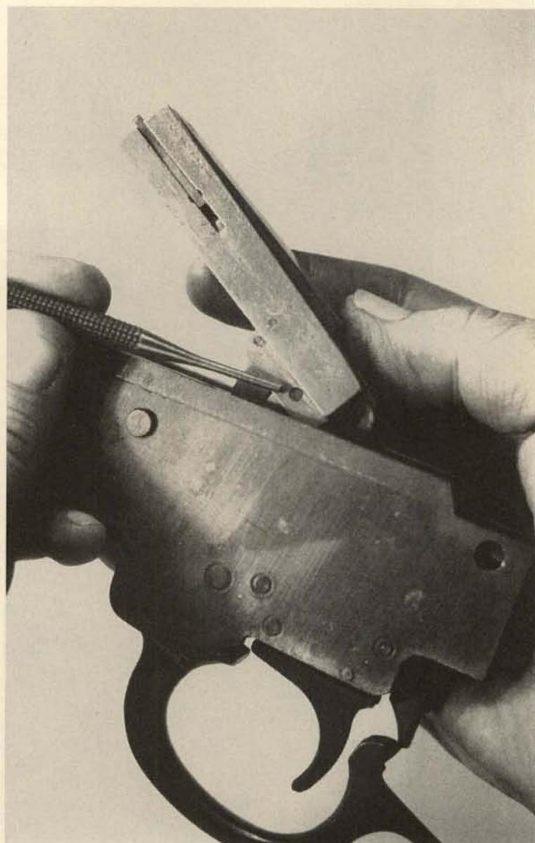
7. Restrain the hammer, pull the trigger and ease the hammer down to fired position. Remove the sideplate screw on the right side of the sub-frame.
