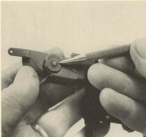
**25.** The cross pin that retains the grip safety bar at the rear must be drifted out toward the right. A spacer washer will be freed inside the unit as the pin is removed. The grip safety bar can then be moved forward and is taken out upward, along with its attached expansion-type spring.
