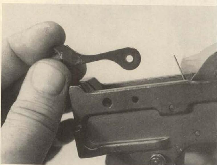
**11.** Before going any further with disassembly of the trigger group, carefully note the relationship of all parts and springs, to aid in reassembly. Tip the front of the ejector out of its slot in the front of the trigger group, push out the cross pin at the rear of the ejector, and remove the ejector upward. Note that removal of the cross pin will also release the upper arm of the bolt latch spring.
