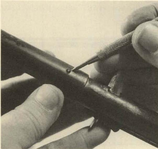
**1.** When replacing the striker in the bolt, be sure the sear contact notch is on the underside, as shown.
