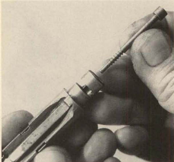
6. Insert a very small screwdriver from the front under the left extractor arm, and lever it outward and over toward the right to remove the twin extractor unit. Be sure to lift it only enough to clear, to avoid deformation or breakage.
