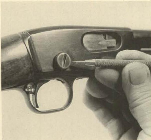
**2.** Separate the buttstock and trigger group from the main receiver, toward the rear and downward.
