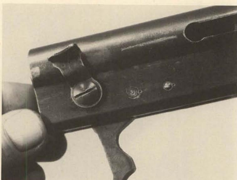
**9.** Drift out the cross pin in the forward section of the receiver, and remove the carrier assembly and its spring downward. The two leaves of the carrier, the spacer bushing, and the spring are easily separated. This pin also is the sear pivot, and the sear can now be moved forward and taken out downward.
