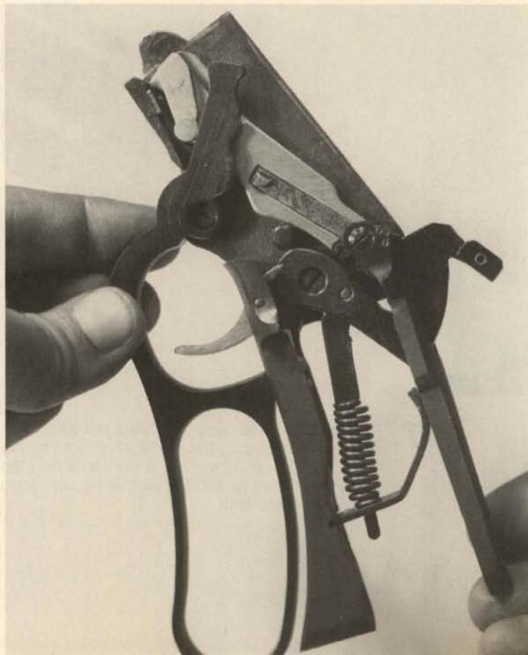
**12.** Grip the upper part of the hammer spring base with pliers and slide it out toward either side, moving its lower end out of its slot in the lower tang. The hammer, of course, must be at rest (in fired position). Remove the base and the spring toward the rear.
