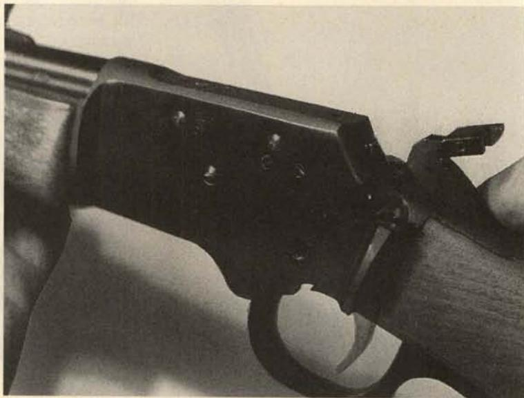
**3.** Slide the breechblock (bolt) toward the rear until its lower projection stops against the shoulder of the receiver, and then remove the bolt toward the right side of the frame.
