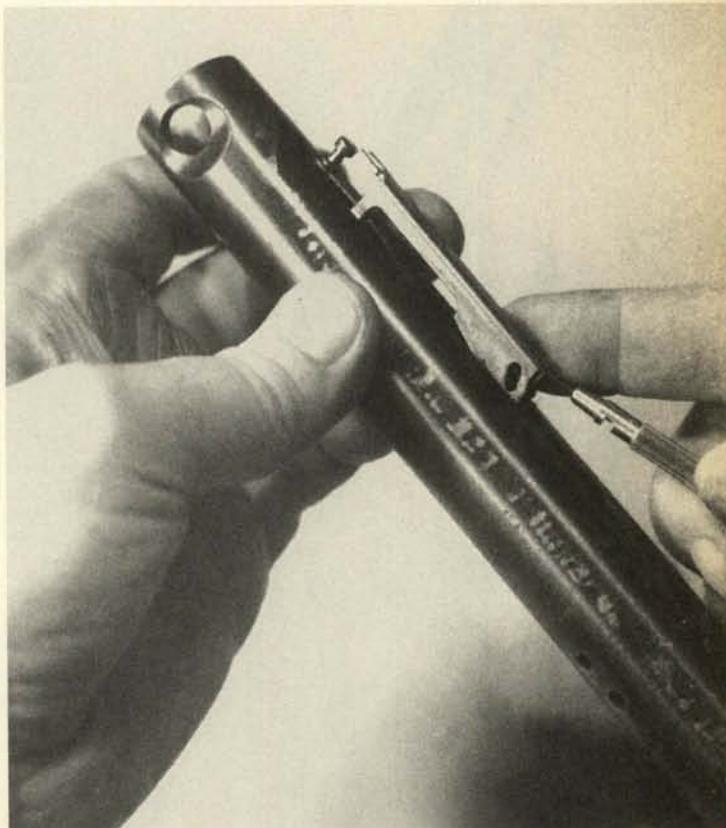
**11.** Backing out the screw/post at the rear of the disconnector slot will allow removal of the curved flat spring.
