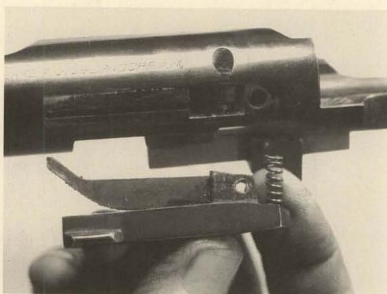
**11.** Take off the bolt stop assembly toward the left, and take care that the small coil spring isn't lost.
