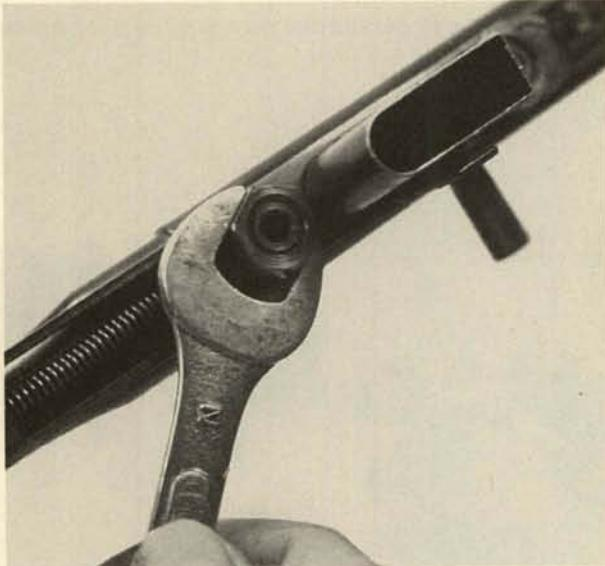
**10.** Remove the magazine housing. Take care that the two lock washers are not lost.
