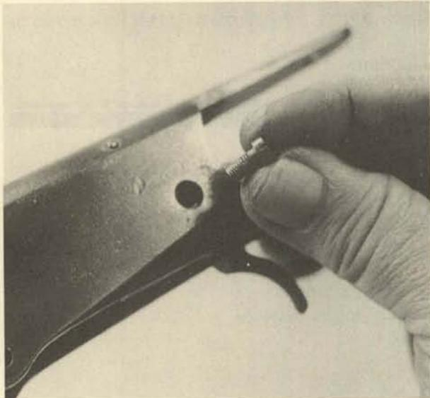
**4.** If the link has been removed from the lever, be sure it is installed with its lobe toward the rear, as shown.
