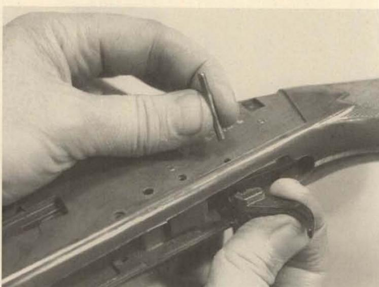
**13.** Push out the cross pin just below the ejector recess (arrow), and remove the cartridge stop and its flat spring from the bottom of the receiver.
