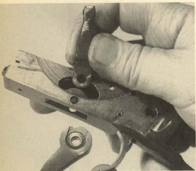
**15.** Push out the lever pivot pin toward the left, and remove the lever downward. Tip the upper lever arm toward the left as it is lifted out of its semi-circular opening and remove it.
