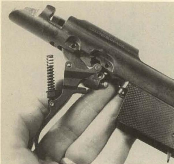
**10.** The magazine catch and its spring are pivoted and retained by a cross pin. **Caution:** Control the catch and its spring as the pin is drifted out. The magazine housing is retained on the receiver by two screws, at front and rear.
