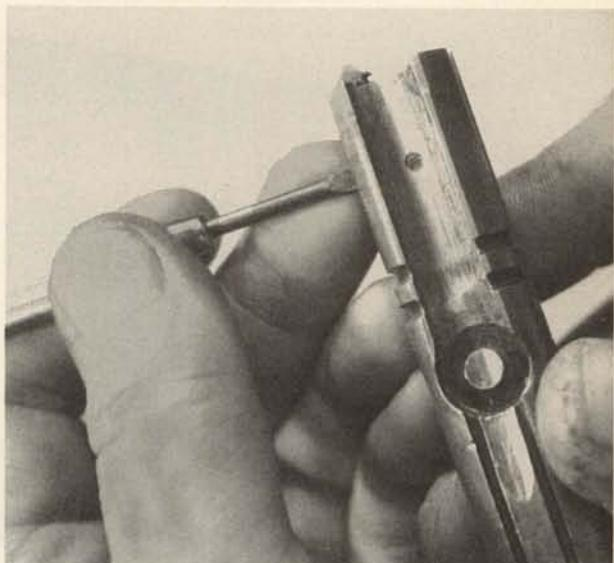
**4.** When replacing the disconnector, lift the spring with a small tool and be sure the tip of the spring enters the opening at the front of the disconnector.
