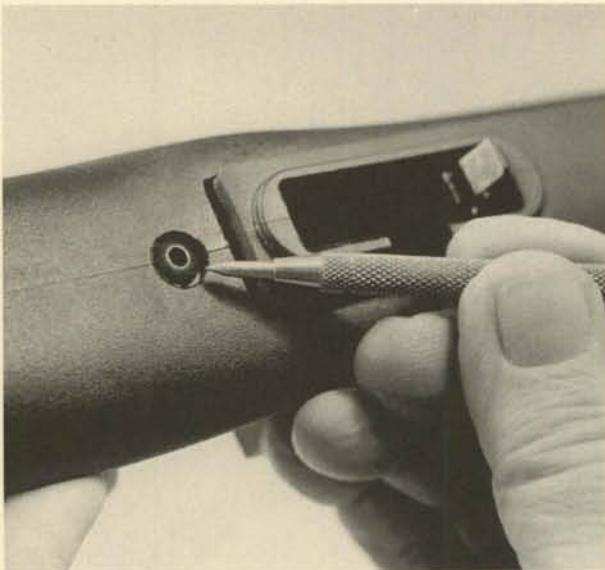
2. Remove the Allen screw at the rear of the trigger guard and take the action out of the stock.
