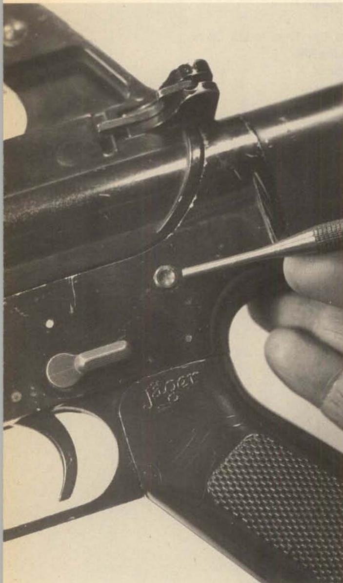
2. Tip the rear of the receiver upward, and pull back the charging handle to pull the bolt out of the rear of the receiver, and remove the bolt.
