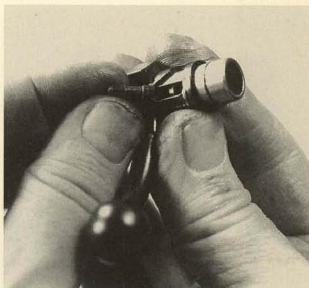
**5.** There is a tiny hole in the bolt body to accept the hooked end of the end piece retainer. The end piece is pushed into place against the spring tension, aligning the lock opening with this hole, and the tip of the retainer is inserted.
