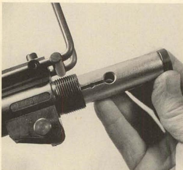
**7.** Use a tool to push the bolt assembly toward the rear, and remove the bolt assembly.
