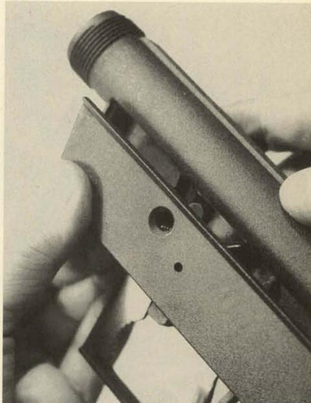
**6.** Restrain the magazine catch spring to prevent its loss, and remove the catch and spring toward the left.
