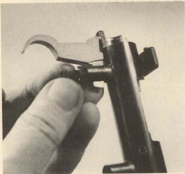
**6.** Remove the trigger downward.
