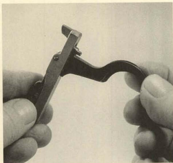
**15.** The trigger and sear can be separated by drifting out the cross pin. The trigger adjustment screw can be removed by turning it clockwise and backing it out upward. In normal takedown, it is best left in place.
