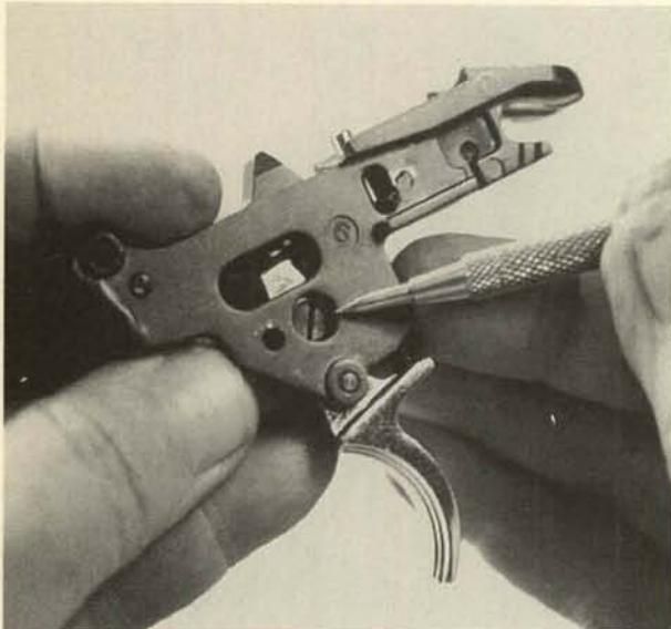
**21.** After the safety post is removed, drift out the trigger pin and take out the trigger and its spring downward. The sear contact stud in the top of the trigger is a separate part. In normal takedown, this system is best left undisturbed.
