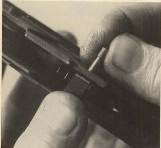
**15.** Move the safety to the off-safe position, restrain the hammer and pull the trigger, lowering the hammer to the fired position. Restraine the sear/disconnector assembly and remove its pivot pin toward the right.
