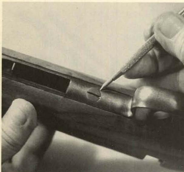
**3.** Remove the rear stock mounting bolt, located between the trigger guard and magazine well.
