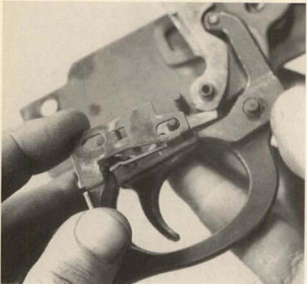
**12.** Use a small screwdriver to detach the sear spring from the rear of the sear and allow it to swing downward, relieving its tension.
