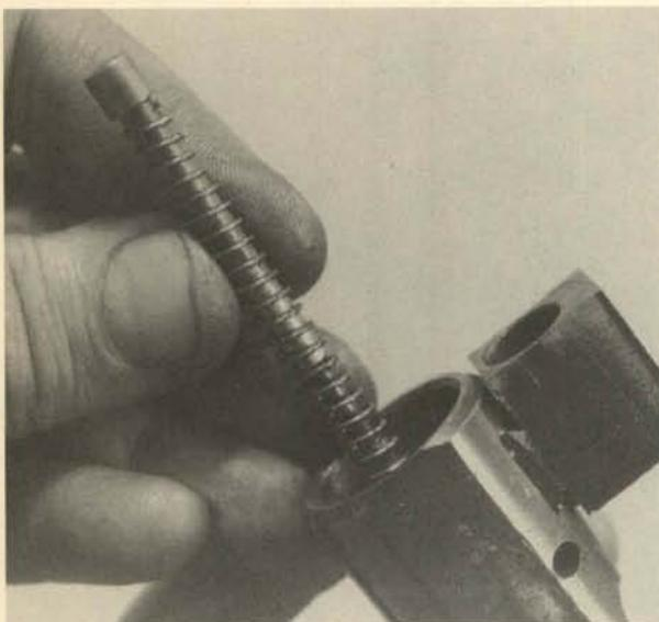
**18.** Remove the striker and its spring from inside the receiver. If they do not come out easily, pulling the trigger to relieve the sear tension should release them.
