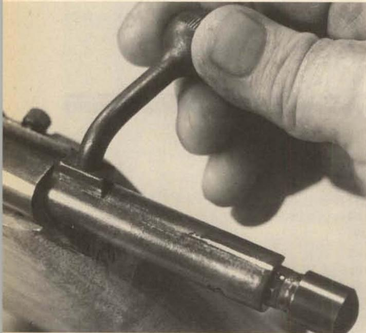
2. Turn the end piece counterclockwise (rear view) to drop the striker forward to the fired position. If the end piece can't be turned easily, tap the cam pin out of its engagement with its detent notch at the rear of the bolt.
