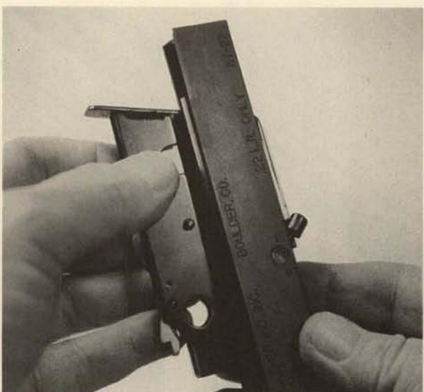
**24.** With the safety in off-safe position (forward), carefully move the trigger group sub-frame slightly upward and forward, taking the tip of the trigger through the recess in the safety cross-piece.
