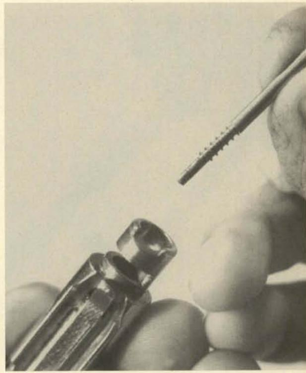
**8.** Remove the front firing pin and its return spring from the bolt head.
