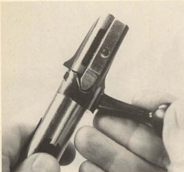
**25.** Restrain the bolt end piece and use an Allen wrench to remove the bolt sleeve retaining screw. **Caution:** Even in fired mode, the striker spring has some compression, so control the end piece.
