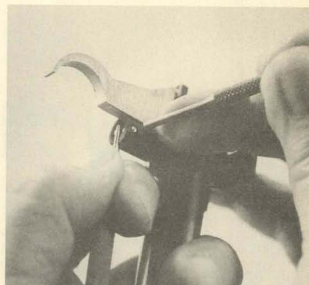
4. The cross pin that retains the combination sear and trigger spring is rebated at each end. To remove it, depress it upward with a tool or fingertip until its larger central portion is aligned with the exit hole on either side. Then, push it out. **Caution:** The spring is under tension, so control it.
