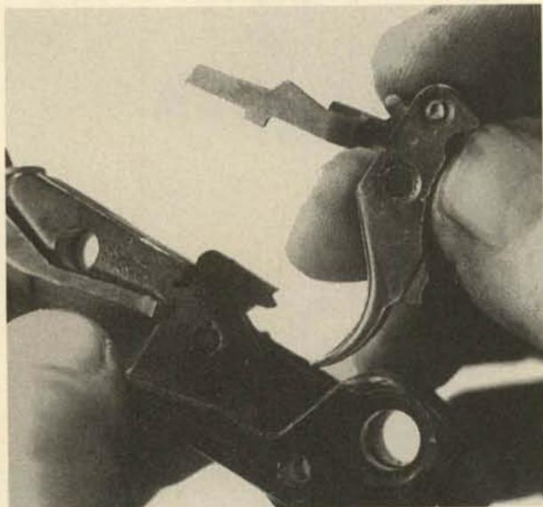
**6.** Drift out the trigger cross pin and remove the trigger, with its attached connector bar, upward. The two leaves of the connector are riveted at the top of the trigger and removal in normal takedown is not advisable.
