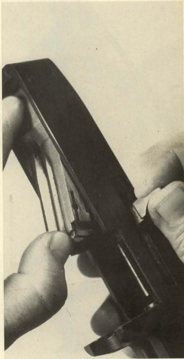
7. The bolt spring guide rod is staked at the forward end, ahead of the bolt handle, and if the stake lumps are filed off for disassembly, a new guide rod may be required. In normal disassembly, this unit is best left intact. If it is taken apart, be careful not to lose the small spacer (arrow) between the spring and the handle at the forward end.
