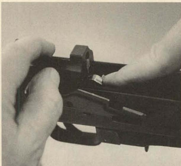
**5.** As the bolt is pushed back toward the front, it will be necessary to depress the hammer for clearance.
