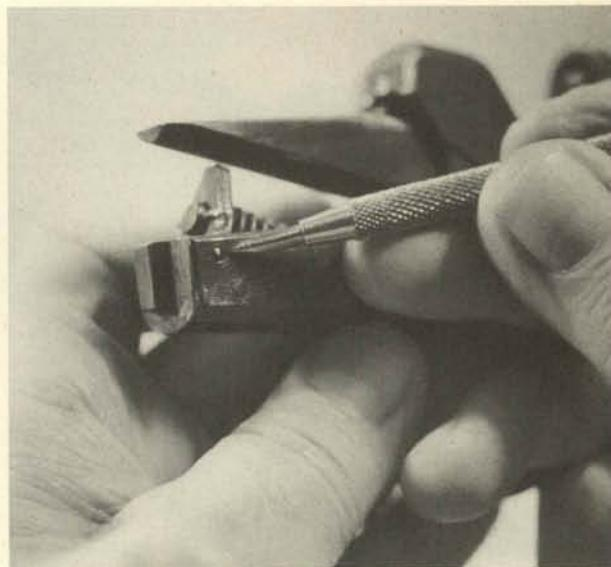
**20.** Drift out the hammer spring base lock pin.
