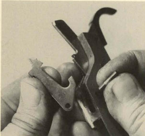
**14.** Note the relationship of the trigger and its spring before removal, to aid in reassembly. Push out the cross pin at the lower rear of the magazine housing, and remove the trigger and its spring toward the rear and downward. Take care that the trigger spring isn't lost. Restraine it, and ease it out.
