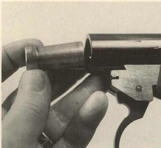
**8.** Cycle the bolt to nudge the striker toward the rear. Pull the trigger and remove the striker toward the rear.
