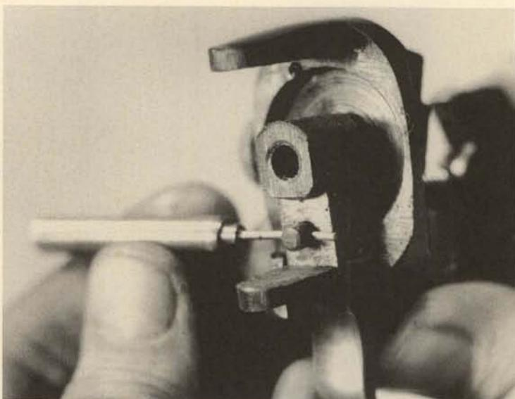
**17.** Depress the action slide lock to clear the left end of the hammer pivot and drift out the hammer pivot pin. This pin is also the pivot for the carrier. Note the relationship of these parts before removal.
