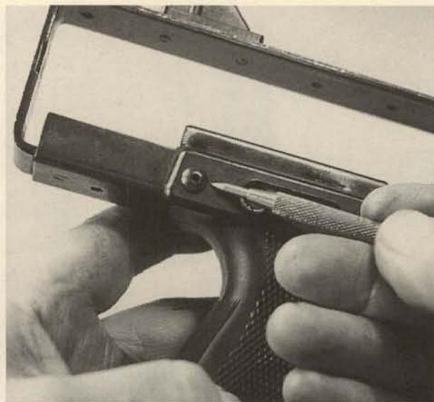
**27.** Remove the Allen screw on the right side at the rear of the grip frame.
