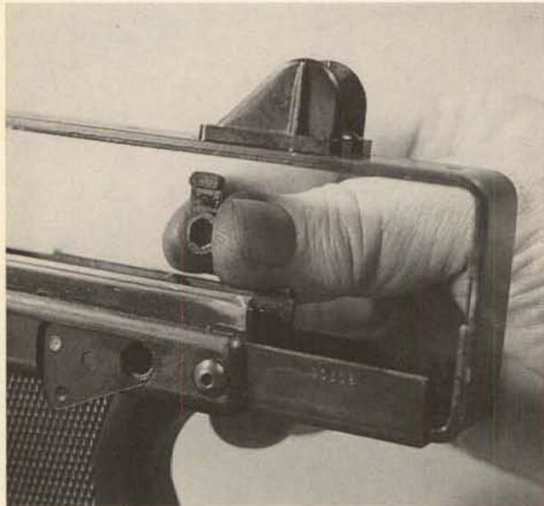
**25.** Remove the hammer spacer from inside the receiver, on the left side.
