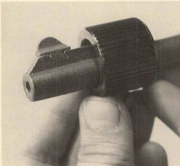
**3.** The barrel collar can be removed from the barrel only after the front sight is drifted out of its dovetail.
