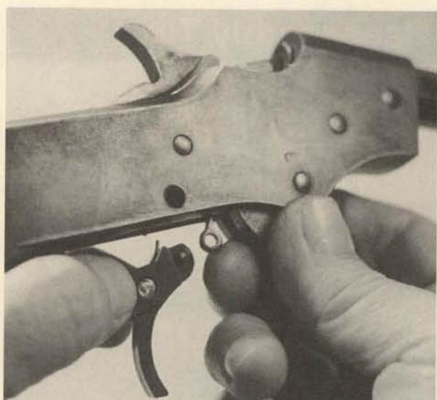
**6.** With the hammer pulled back, the hammer block is inserted at the top, its cross-piece lying in the "hook" at the back of the link. Its lower loop will protrude as shown to engage the post on the trigger.
