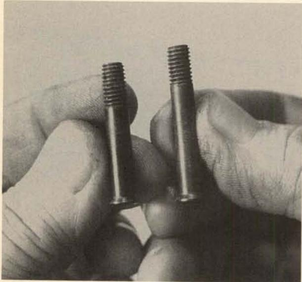
2. When replacing the sleeve and striker assembly, note that there is a flat on one side of the striker shaft, and this must be oriented to mate with the flat in the sleeve tunnel. Also note that the safety-lever must be in its midway or vertical position when the sleeve and striker assembly are turned back into the bolt.
