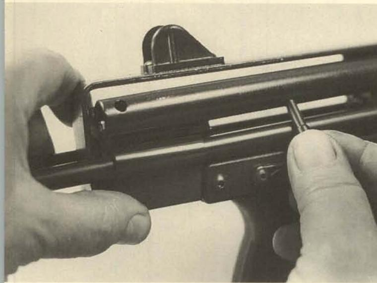
**8.** Use an Allen wrench to back out the screw which retains the firing pin and its spring. **Caution:** *The return spring is quite strong, so keep the firing pin under control.*
