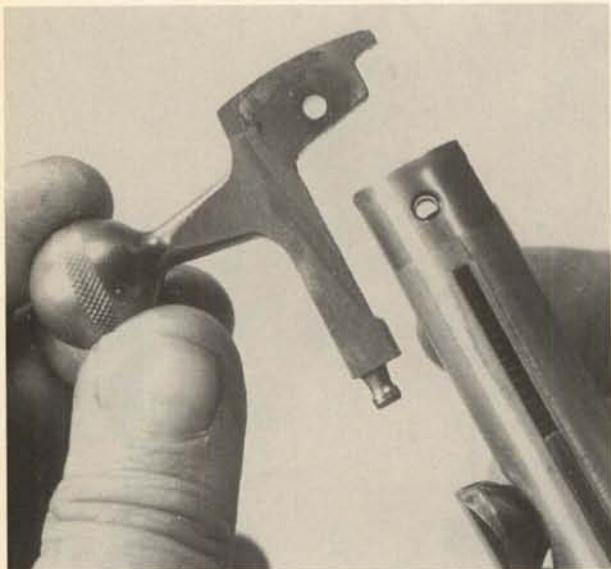
**6.** Remove the striker spring and its plunger toward the rear.
