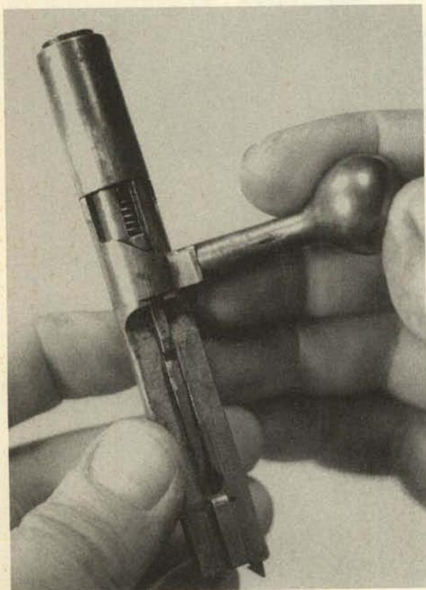
3. Grip the front portion of the bolt in a padded vise and turn the bolt handle to allow the striker to move forward to the fired position, partially easing the tension of its spring. The photo shows the bolt after the handle is turned, with the striker forward.
