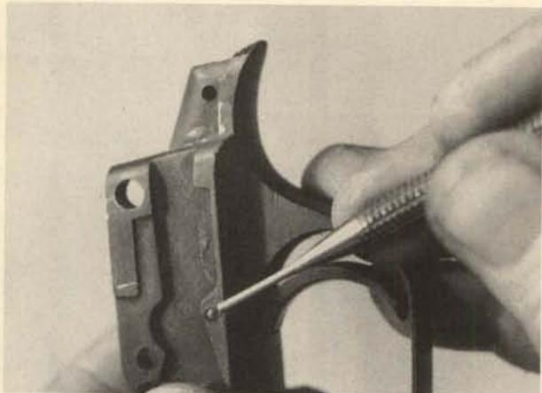
**7.** Drift out the trigger cross pin and remove the trigger and its spring upward.
