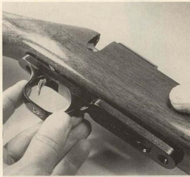
**4.** Remove the trigger guard assembly downward. The magazine catch and its spring, located in the guard forward of the trigger, are best left in place in normal takedown. If removal is necessary for repair, insert a drift or rod through the loop at the rear of the catch, and draw it back until its side wings align with the exit cuts; then lift it out. Control the spring.
