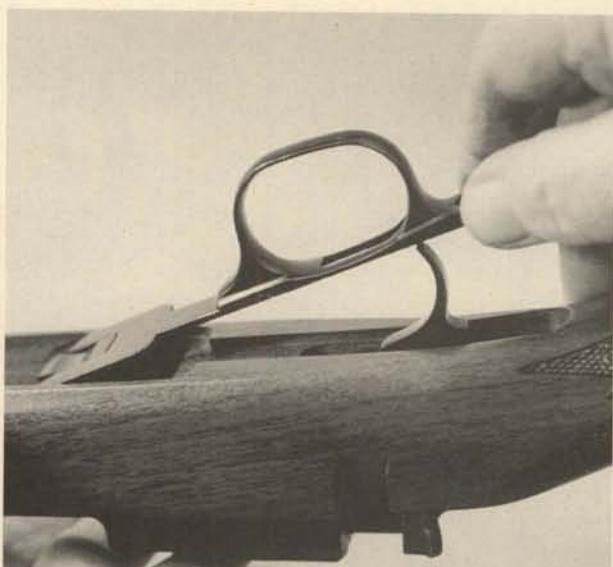
**9.** Restrain the magazine catch plunger and push out the catch lever cross pin.
