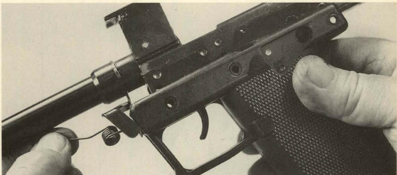
**30.** Remove the grip frame and the stock latch spring.
