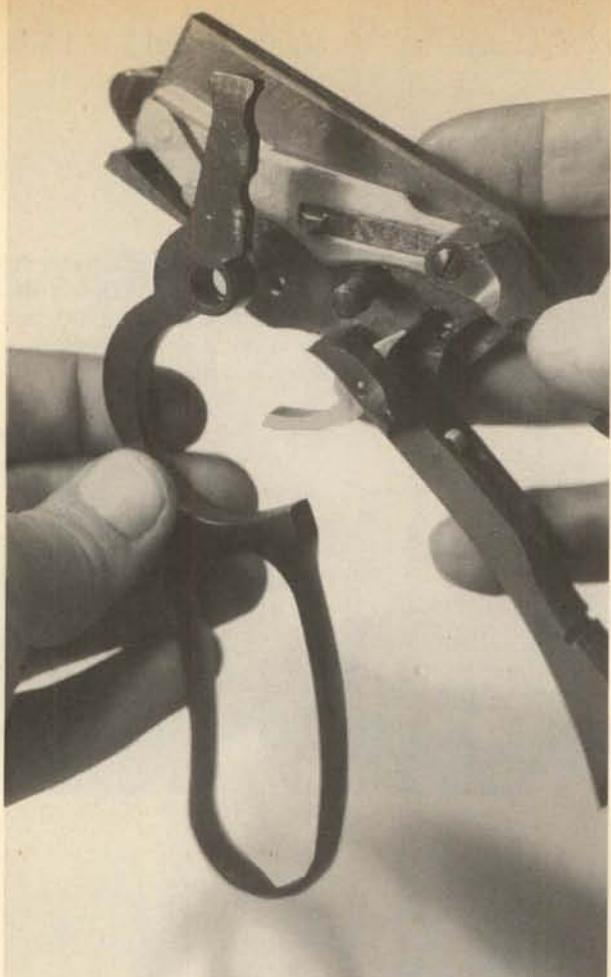
**16.** Take out the lever pivot screw and remove the lever toward the left.
