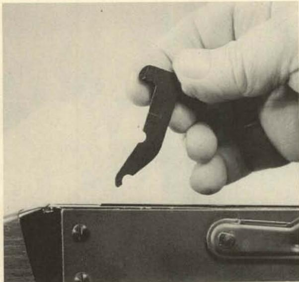
6. Move the bolt all the way to the rear, and lift it off upward.
