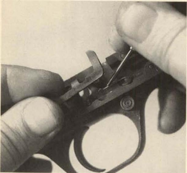
**6.** Drifting out the sear pivot pin toward either side will allow removal of the sear and its spring upward. Before removal, note the relationship of the sear and its spring to aid reassembly.
