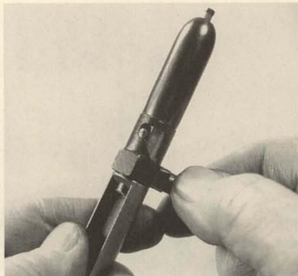
**8.** Before the bolt is put back into the receiver, it must be recocked. Hold the front portion of the bolt firmly in a shop cloth or a padded vise, and turn the bolt handle until the striker is in the position shown.
