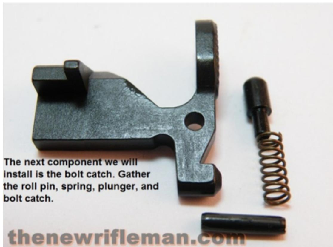
Drop the spring and plunger into the hole in the receiver before placing the bolt catch assembly in the slot
