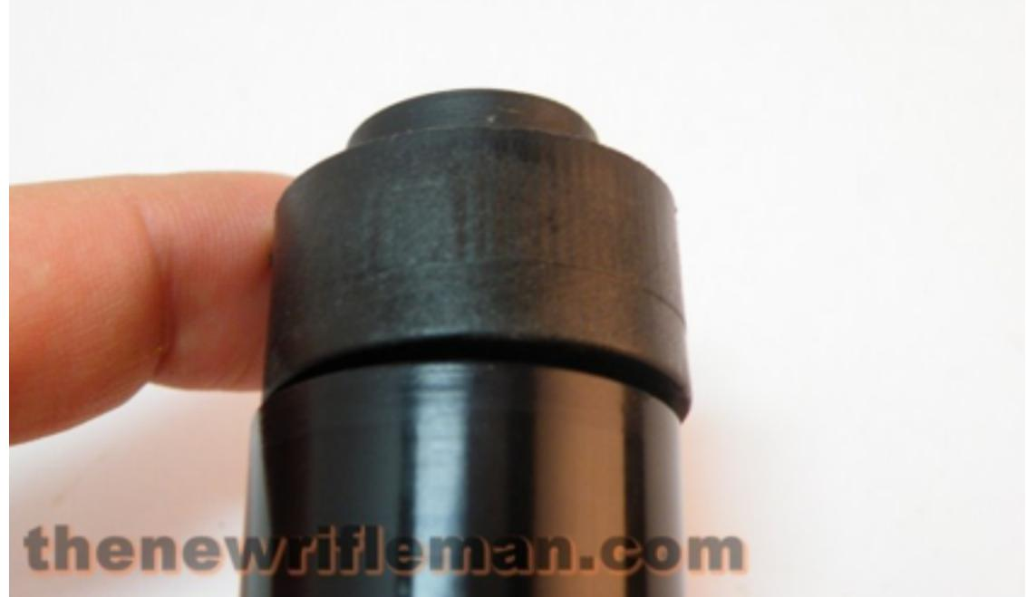
**Slide the A2 stock assembly over the receiver extension. It will trap the takedown pin's spring and detent assembly.**
