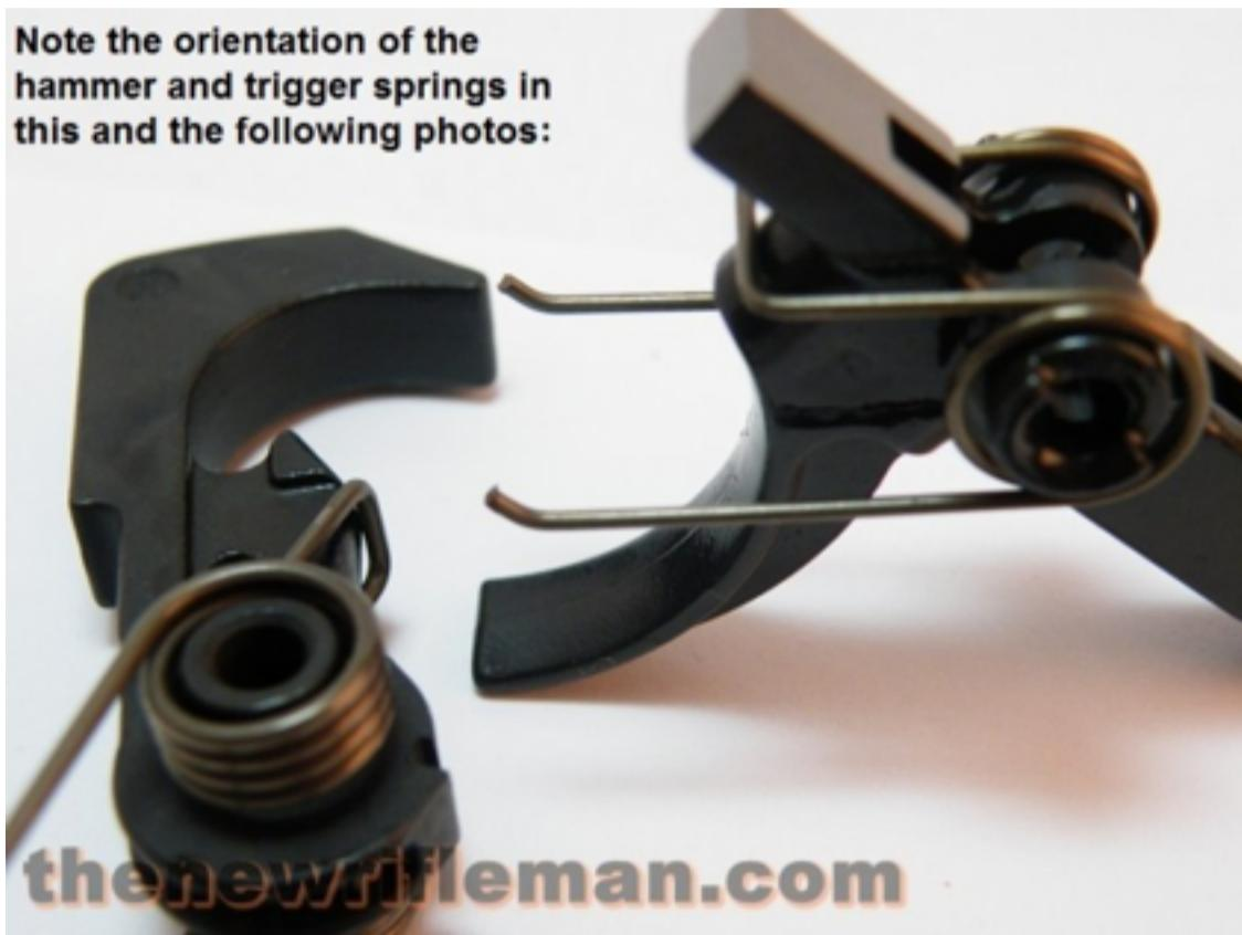
Push the disconnector spring into place here. The wide end goes down. Once installed it should be unable to fall out.
