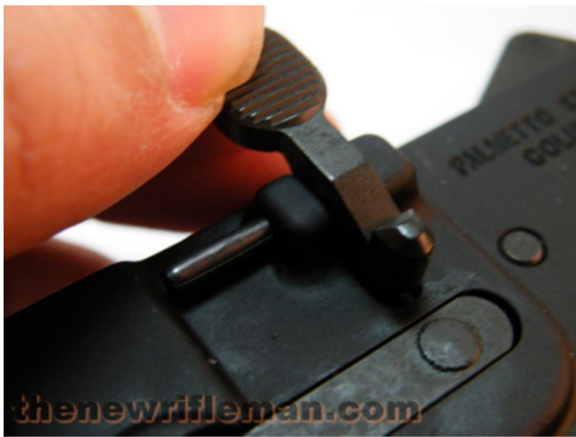
Wrap your pliers well with thick tape and pinch the roll pin in place. You can approach from the bottom...
