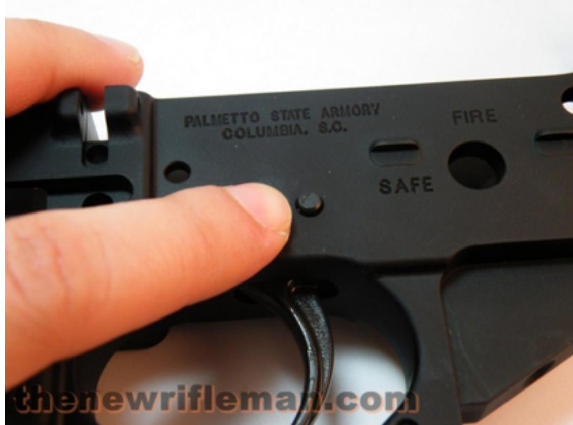
Push the hammer down into the receiver to align the pin holes. Make sure the ends of the spring lay on top of the trigger pin, not underneath.
