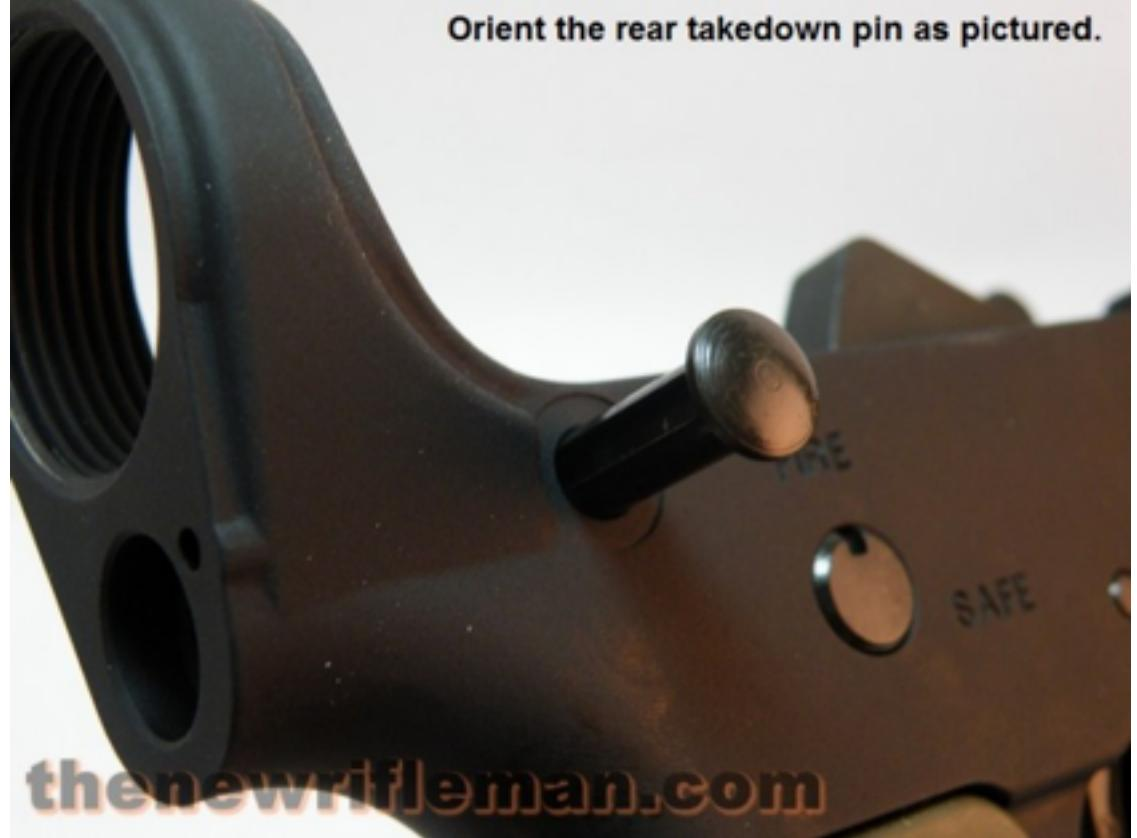
Drop the rear takedown detent into the hole followed by the detent spring.
