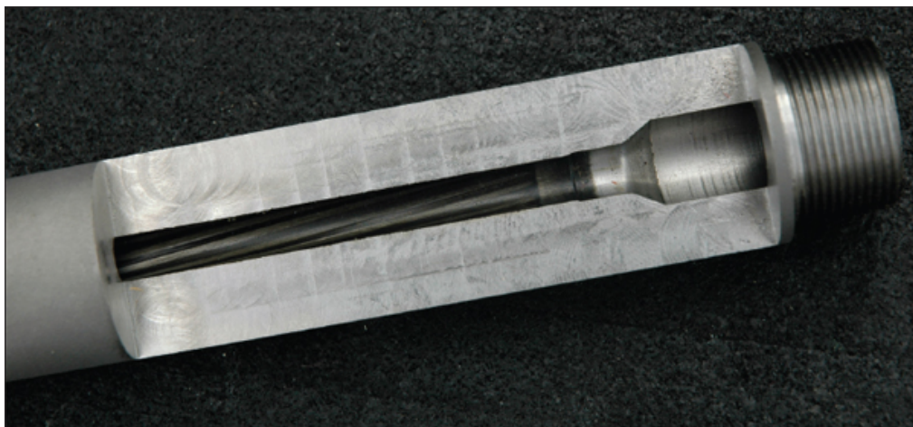
Chamber dimensions affect headspace and case expansion. The throat affects breech pressures.
