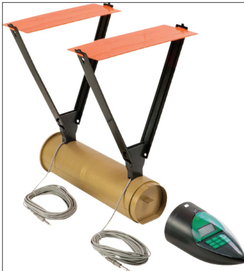
Chronographs (here an RCBS AmmoMaster) are now affordable, easy to use, a must for handloaders.
