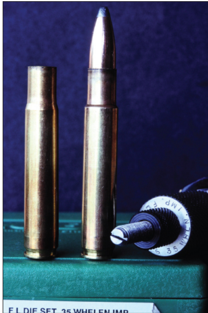
P. O. Ackley “improved” cartridges (here the .35 Whelen) by steepening the shoulder to 40 degrees.
