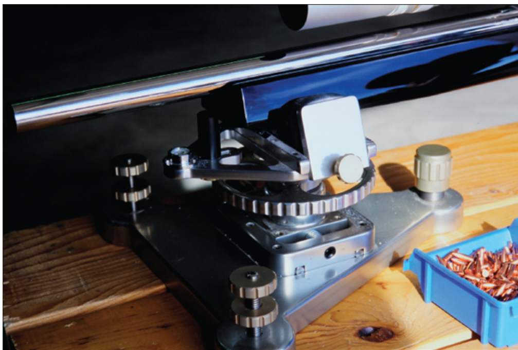
This benchrest forend cradle is fully adjustable, to ensure stability and consistent rifle support.
