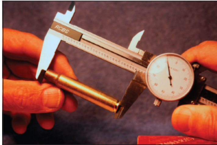
A dial calipers is exceedingly useful. Handloading wildcats, case length can be a crucial measure.
