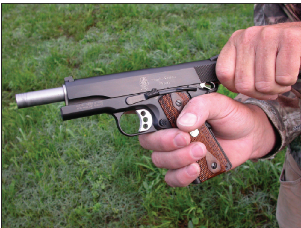
The .45 ACP case headspaces on the mouth, so case length matters a great deal in 1911 pistols.
