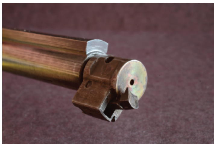
The Short Magazine Lee Enfield's bolt has a separate head, which can be changed to tune headspace.
