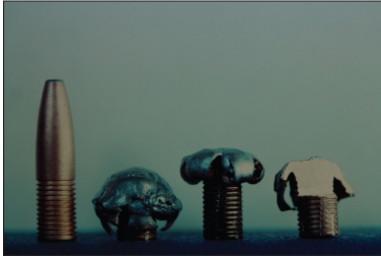
This experimental big game bullet has a lead nose that expands and a copper shank that drives deep.
