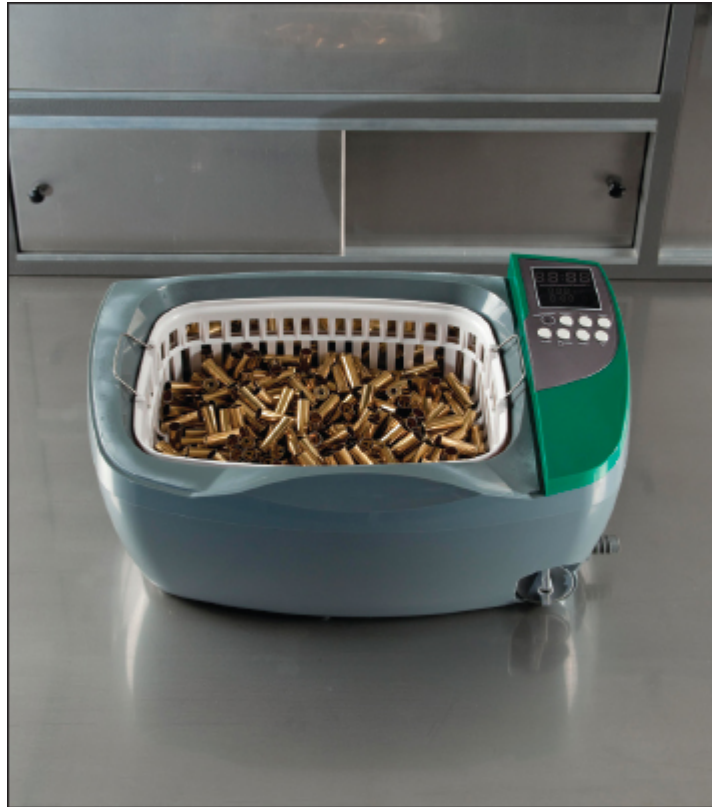
Ultrasonic case cleaners (here an RCBS) give wildcatters brilliant hulls to form into new cartridges.
