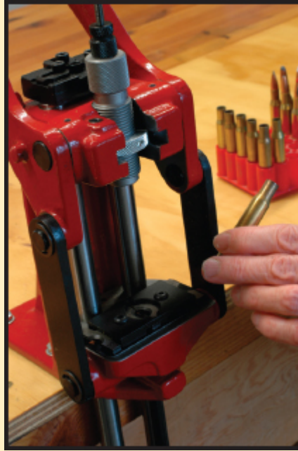
Neck-size to save unnecessary working of brass, and so cartridges fit more closely in the same rifle.
