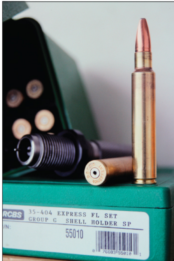
This husky wildcat was made by necking down the old .404 Jeffery (c. 1910) to take .358 bullets.
