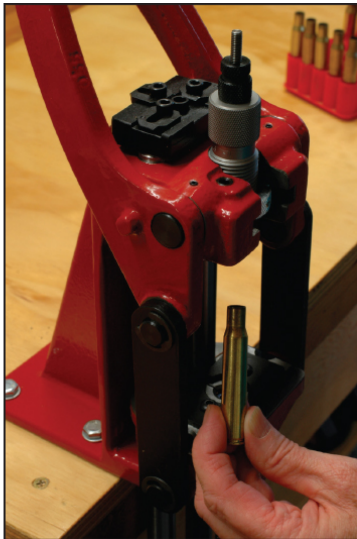
Straight cases like the .45-70 merit three-die sets. RCBS offers this one for Cowboy Action shooters.
