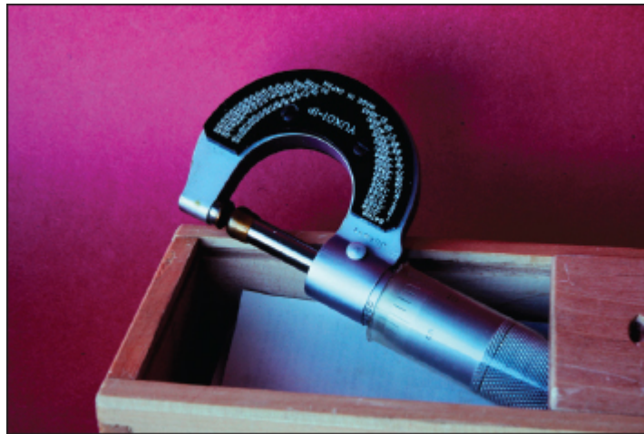
Case head expansion—a measure of pressure—can be done with a micrometer. Note protective caps.
