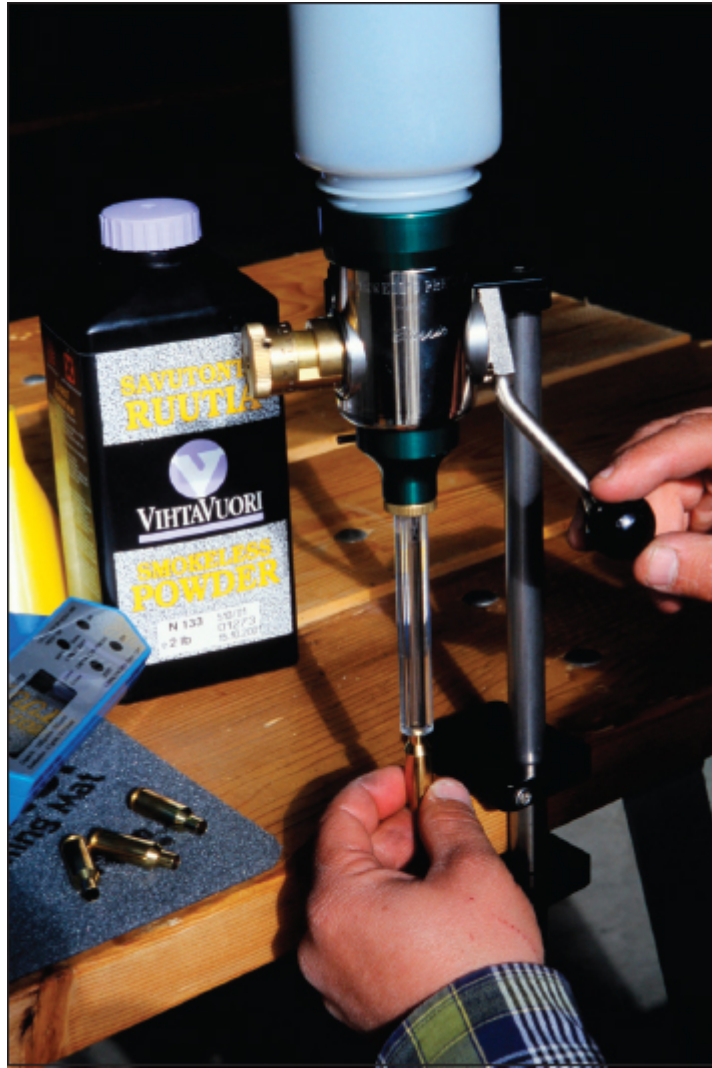
A well-made measure delivers powder in identical doses. A drop tube helps sift full-case charges.
