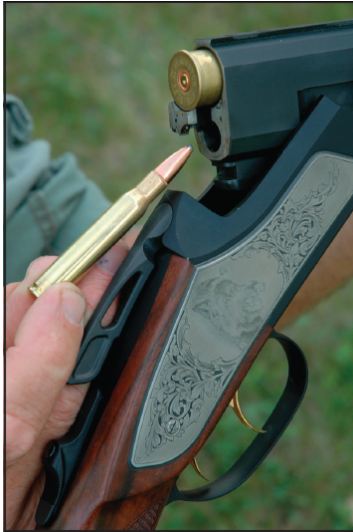
Ideally suited to rimmed cases, modern hinged-breech guns (here a Steyr Duett) also accept rimless.
