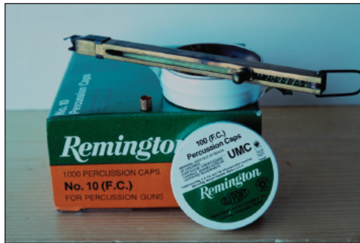
Percussion caps employ the muzzleloader's nipple as an anvil. The brass sleeve speeds capping.
