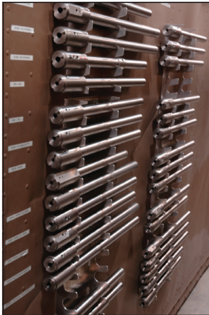
Rifle barrels at Black Hills Ammunition are used to measure pressures as well as check accuracy.
