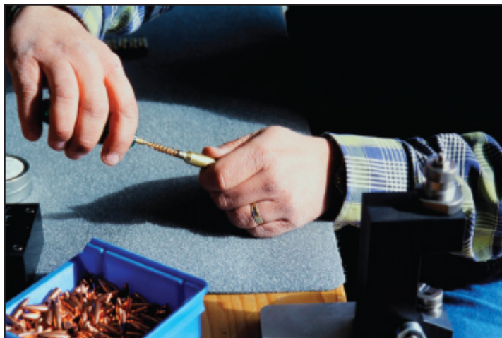
Not all useful tools are complex or costly. Here a simple brass brush cleans residue from case necks.
