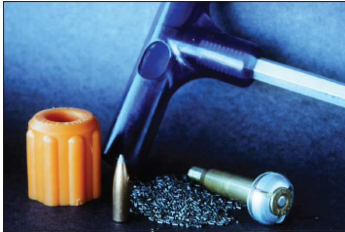
A bullet puller uses inertia to yank a bullet free, unscathed, and saves the powder. You'll want one.
