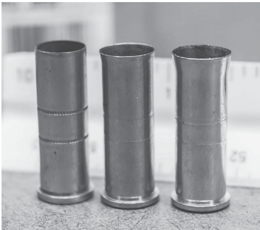
From left to right, the case before flaring, the properly flared case, and an over-flared case.
