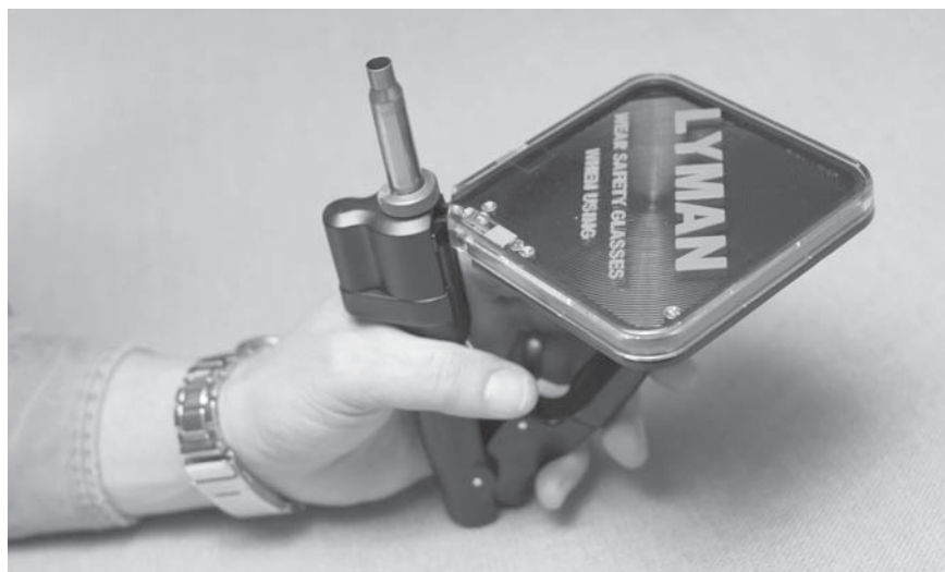
Hand priming can give a good "feel," when it comes to proper primer seating depth.
