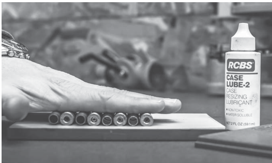
Rolling the cases to be resized across a lube pad.
