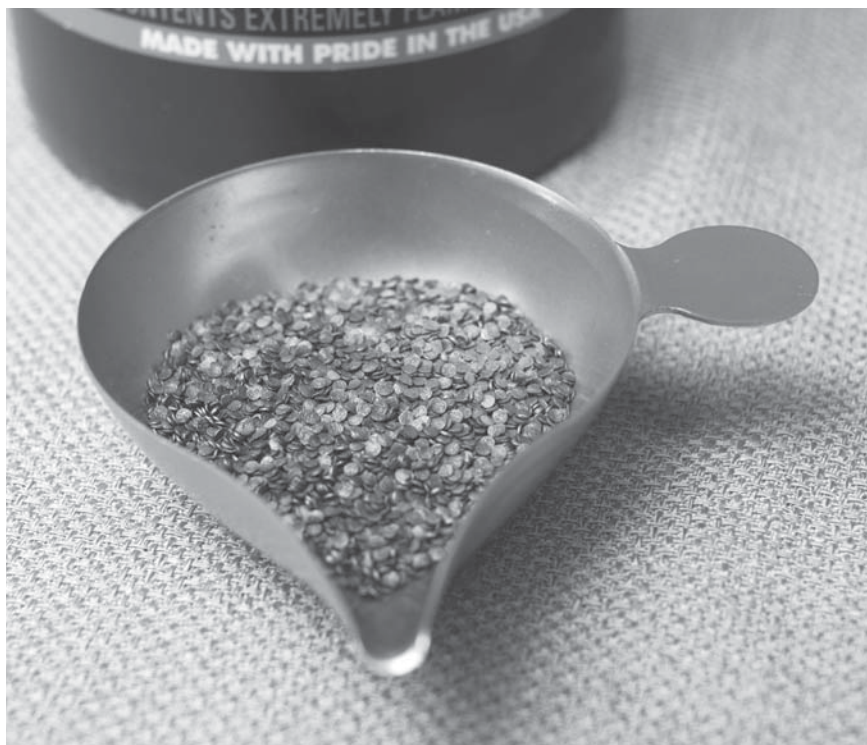
Flake powder grain structure.
