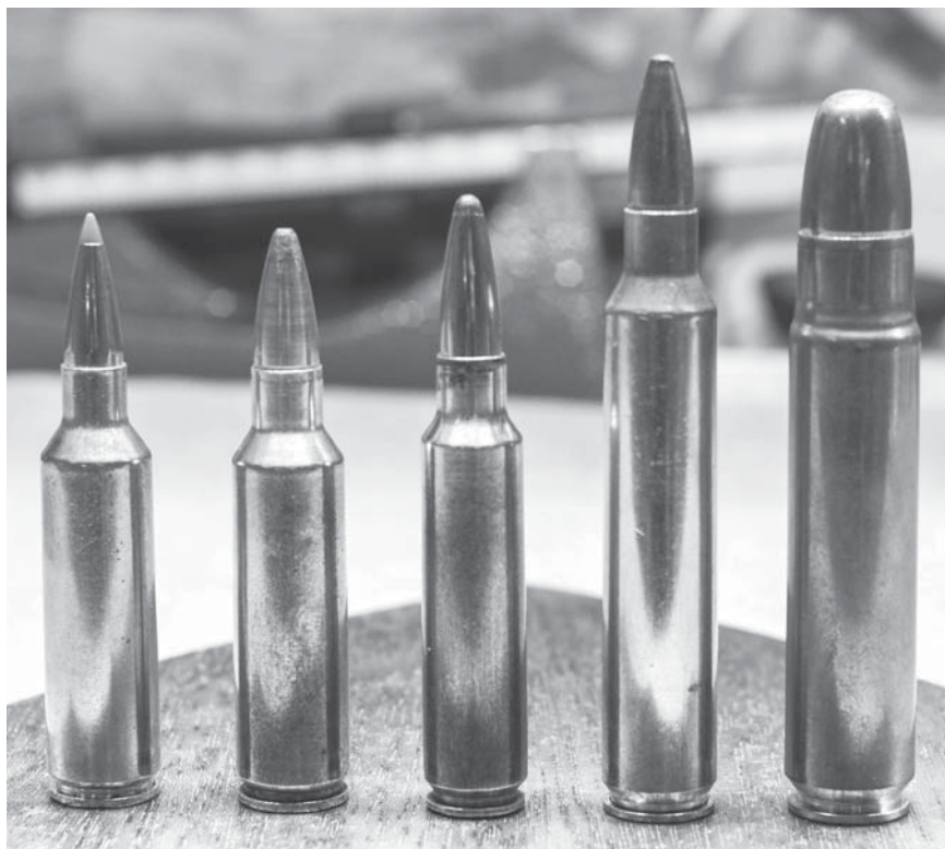
Rebated rim cartridges. Left to right, .270 WSM, .300 WSM, .284 Winchester, .300 Remington Ultra Magnum, and .500 Jeffrey.
