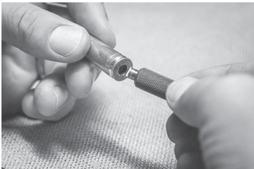
A clean primer pocket is an absolute necessity.
