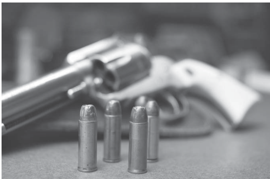
These .45 Colt cartridges were roll crimped, so the bullets won’t move out of the case under recoil, when fired in a revolver.
