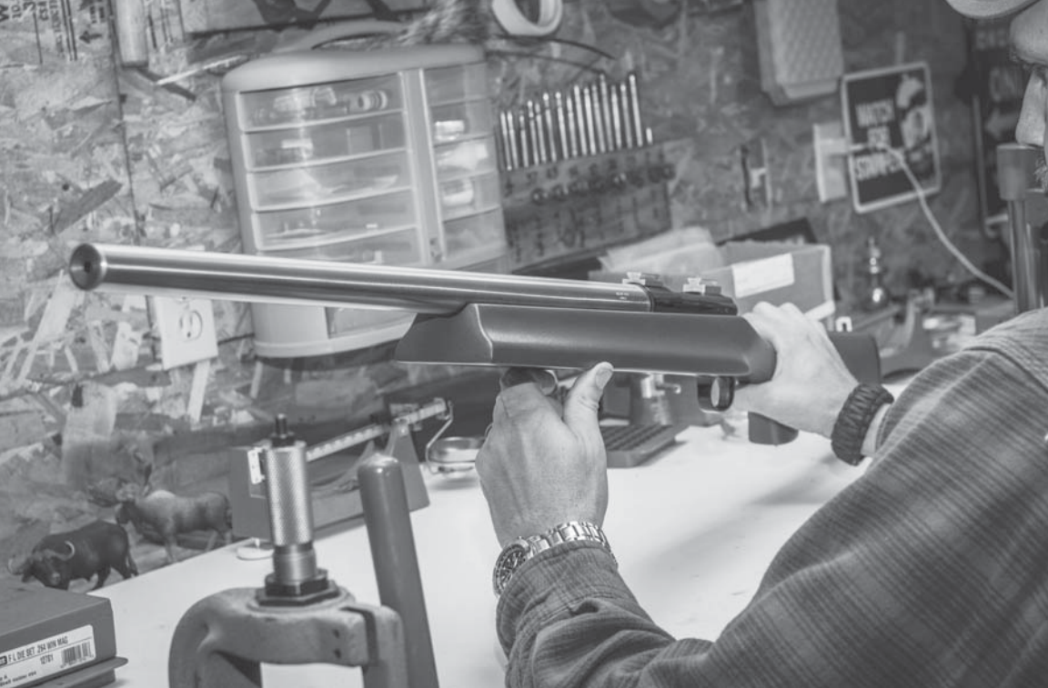
Large-diameter “bull” barrels are often employed on long-range target rifles.
