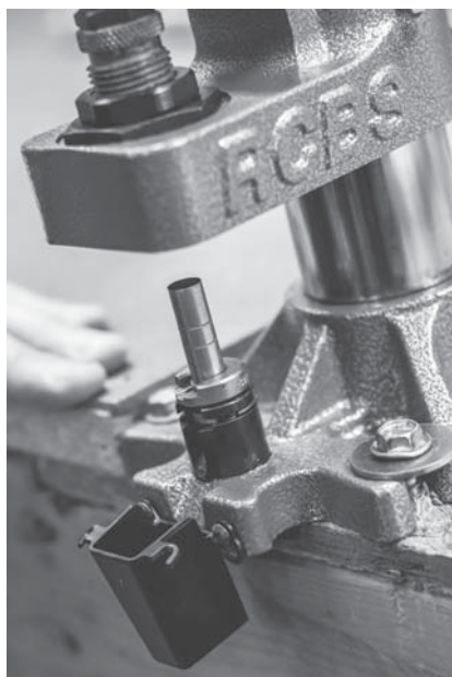
A .38 Special case before flaring.
