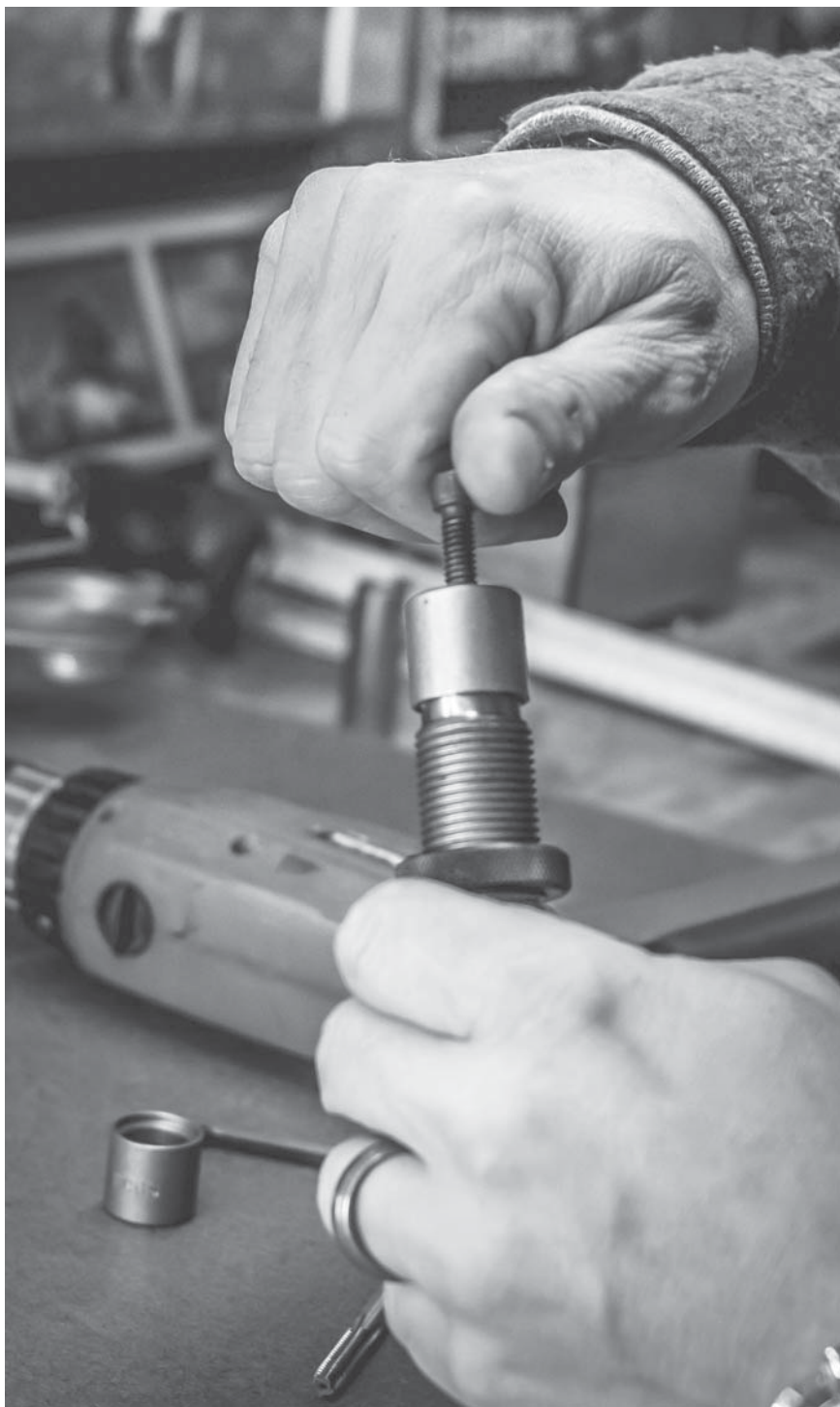
Using the case remover to back out a stuck case.
