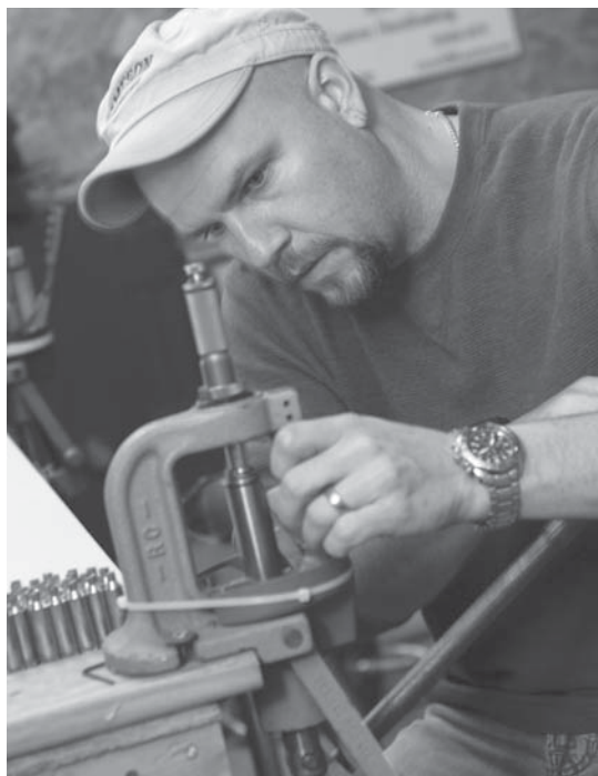
The strong frame of an “O”-style press.
