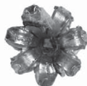
Expanded Speer GoldDot handgun bullet.
