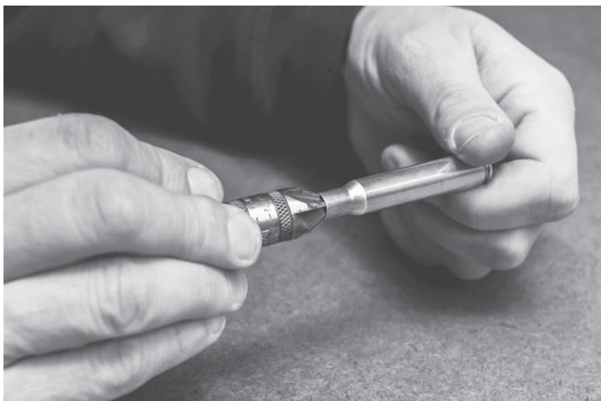
The inside of the case mouth should be chamfered, for smooth bullet seating.
