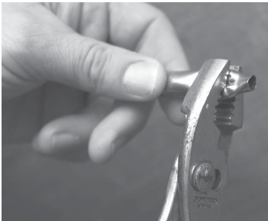
Crushing a case that is unusable prevents it from making it back into the “good brass” pile.
