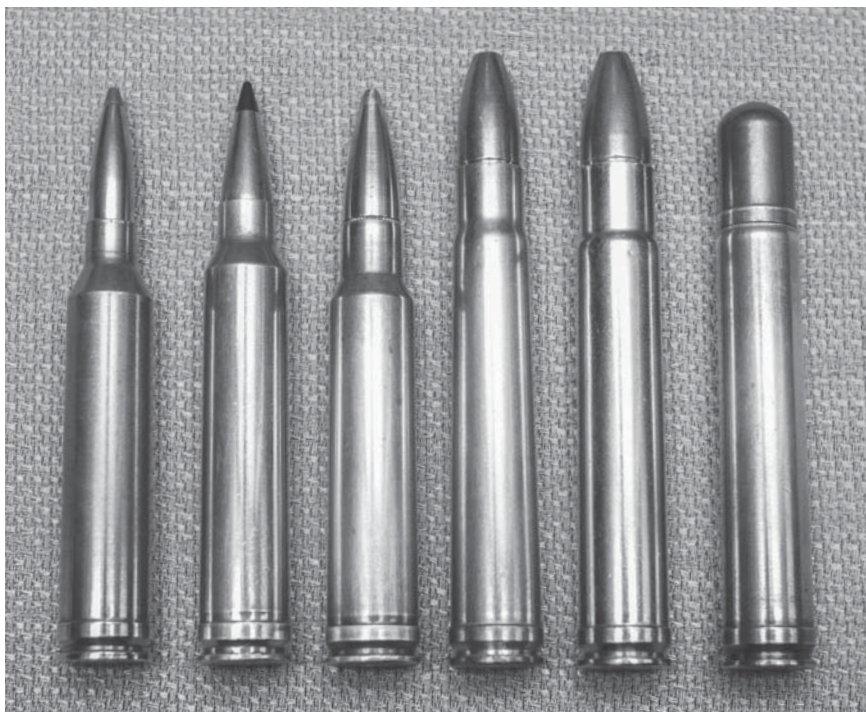
Belted magnums. Left to right, .264 Winchester Magnum, .300 Winchester Magnum, .338 Winchester Magnum, .375 H&H Magnum, .416 Remington Magnum, and .458 Winchester Magnum.
