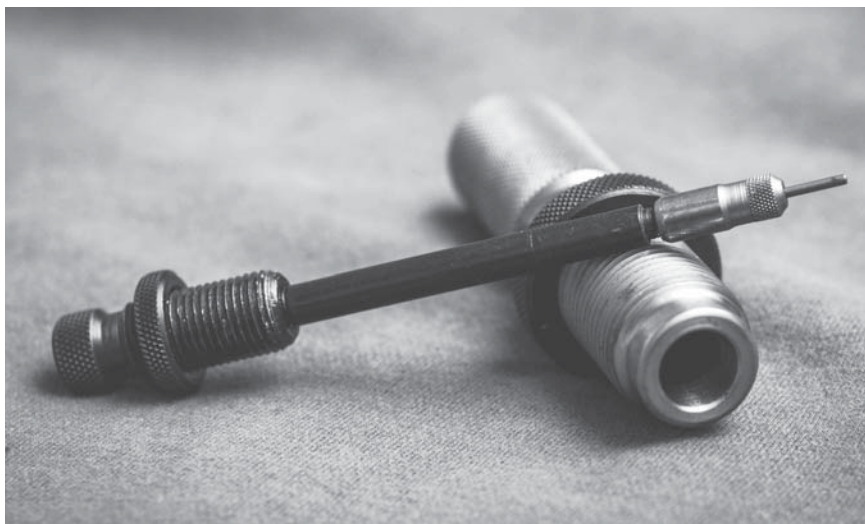
A disassembled resizing die, showing the expander ball and decapping pin.
