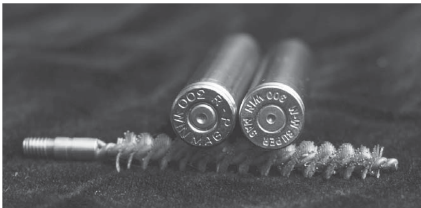
The primer on the left shows acceptable pressure. It has the same appearance as a new one, with the exception of the firing pin mark. The primer on the right has been flattened and the firing pin mark appears “cratered,” showing signs of excessive pressures.
