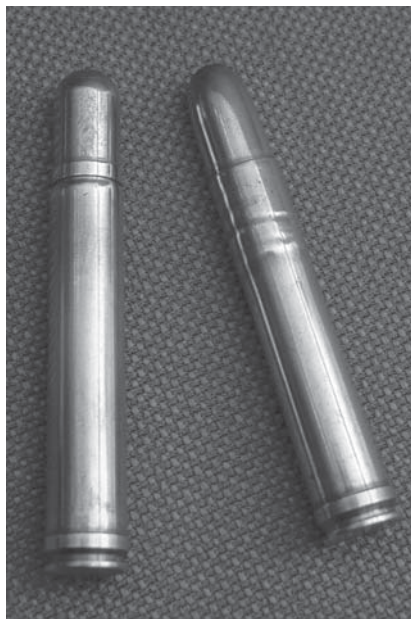
The .458 Winchester Magnum on the right is a victim of too much crimp and not enough flare. That caused the case to crumple.
