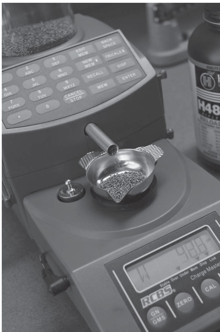
The digital display and powder pan of the ChargeMaster 1500.
