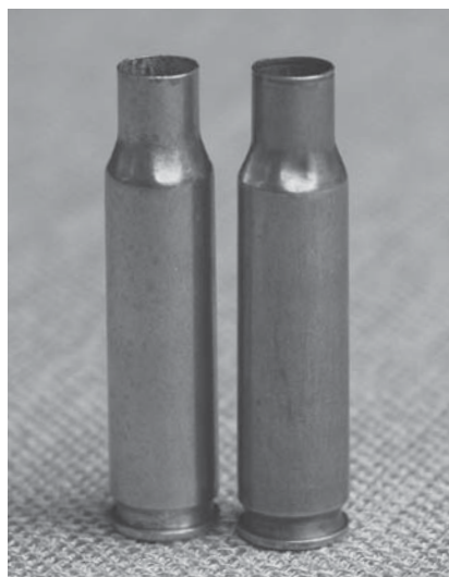
Unightly hydraulic dents in the shoulder portion of these .308 cases show signs of using too much case lube.
