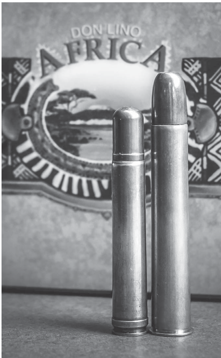
A heavy roll crimp was placed on the case mouths of this .458 Winchester Magnum (left) and the noticeably bigger .500 Nitro Express.
