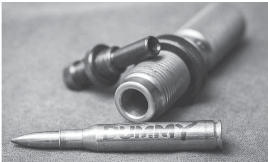
A disassembled seating die, with dummy round.
