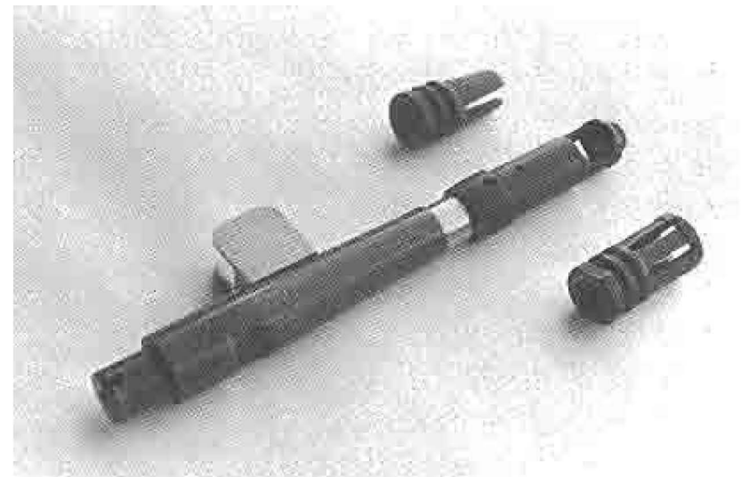
The short barrel with various types of muzzle brake and flash eliminators. The barrel end was threaded about 3/4 inch to take all current M16 barrel attachments including the Sionics silencer for the .223 cartridge. The thread-on-type silencer featured in the Home Workshop Silencers (Paladin Press, Boulder, CO) can be adapted for the 1022.
