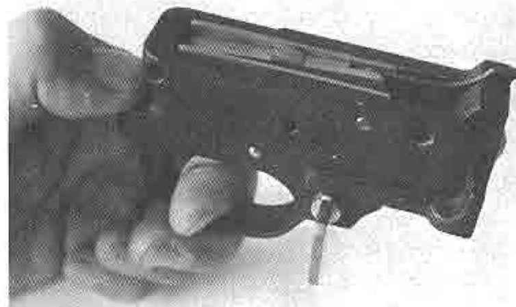
Photo showing the trigger not quite fully depressed. Note that the sear lug is now below the top level of the trigger housing and the bolt has been released. The remaining trigger pull will allow the disengagement of the trigger and sear trip.
