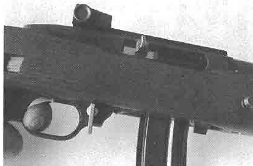
Close-up view showing the trigger fully pressed. In the shooting sequence, the weapon fires the first shot, the sear bounces back to its normal upward position after disengaging from the trigger and catches the bolt after it recoils to the rear once the shot is fired.
