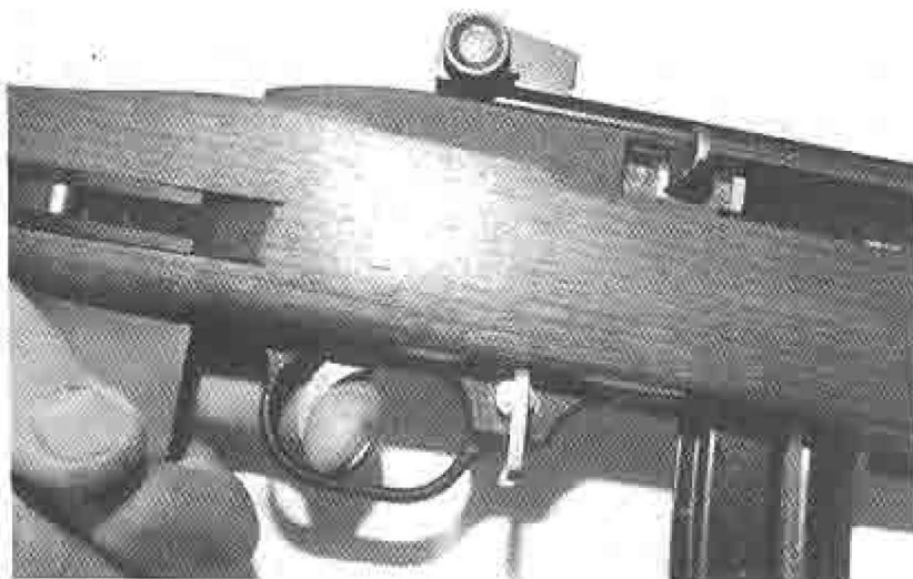
Close-up view showing the trigger being pressed. The selector is set at "semiauto." The bolt is still held in open position as engaged with the sear. Note that there is still about 3/16 of an inch left before the trigger is pressed fully to the rear. Further pull will release the bolt forward to fire the weapon. The trigger must be released forward for the trigger to reengage with the sear trip to fire the next shot.
