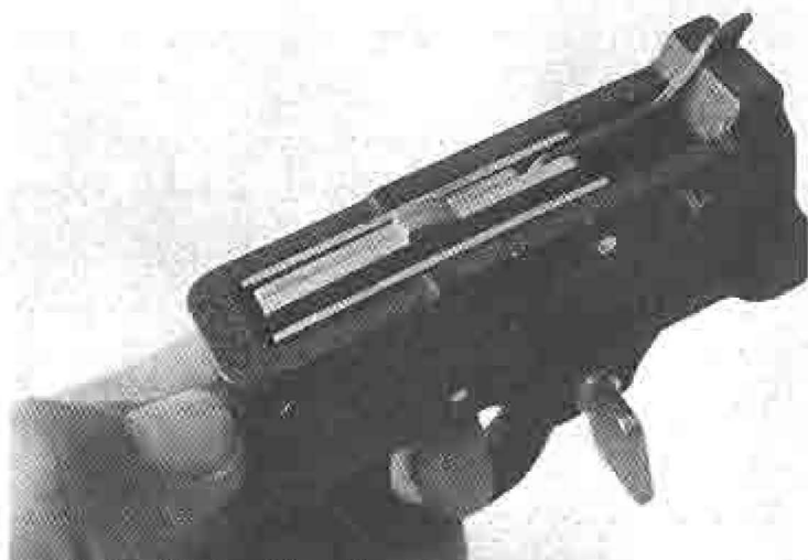
The trigger housing unit has been removed from the receiver to show the relationship of the trigger components when fired on "semiauto." The trigger is about to be pressed. The top of sear nose is well above the trigger housing frame.
